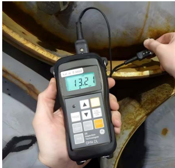
FIG. 34. Measuring corrosion attacks (courtesy of Urenco).
