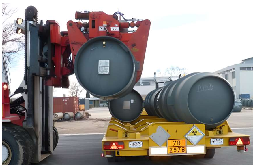
FIG. 20. Road trailer for on-site 48Y cylinder transport (courtesy of Orano).
