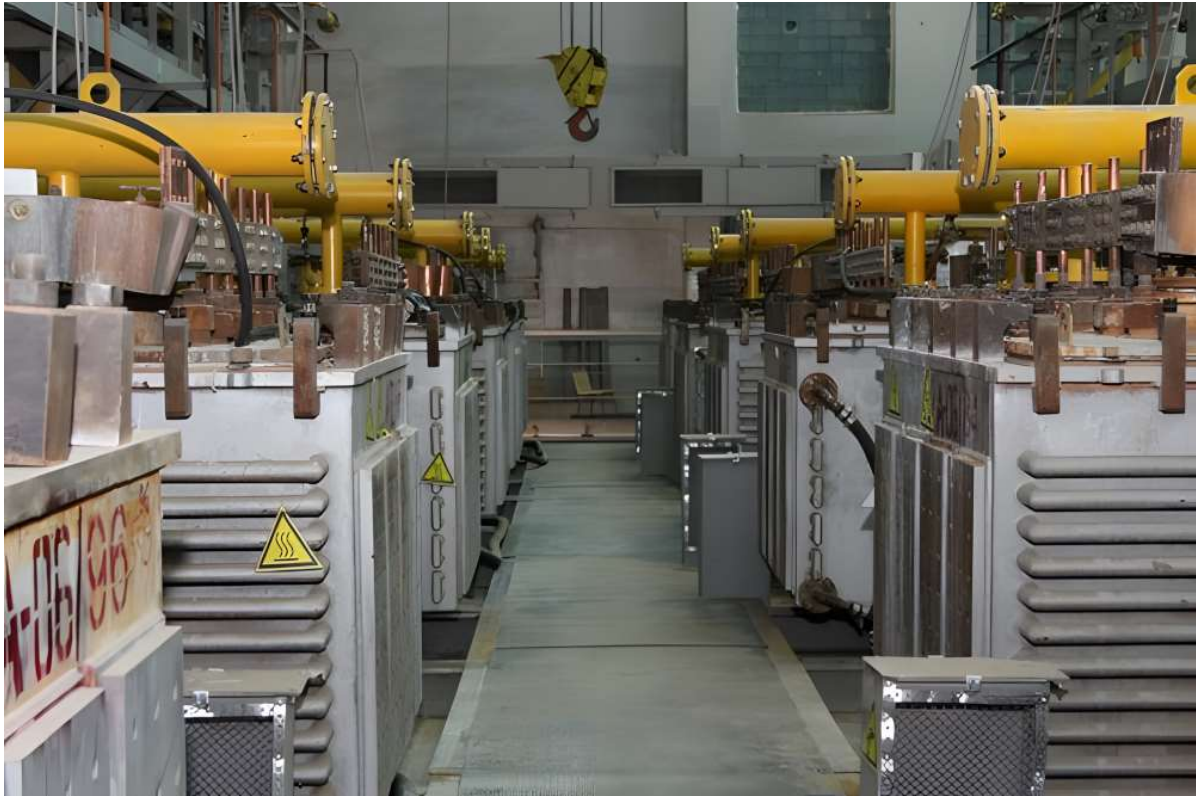
FIG. 22. Cells for fluorine generation (courtesy of TVEL).
