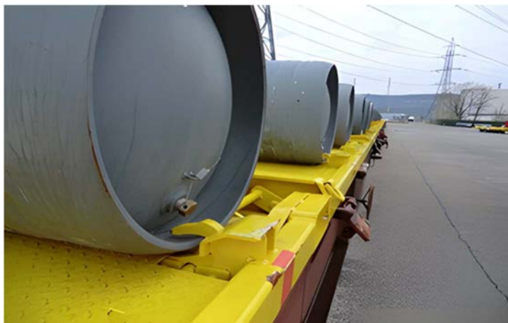
FIG. 19. Rail wagon for on-site 30B cylinders transport (courtesy of Orano).
