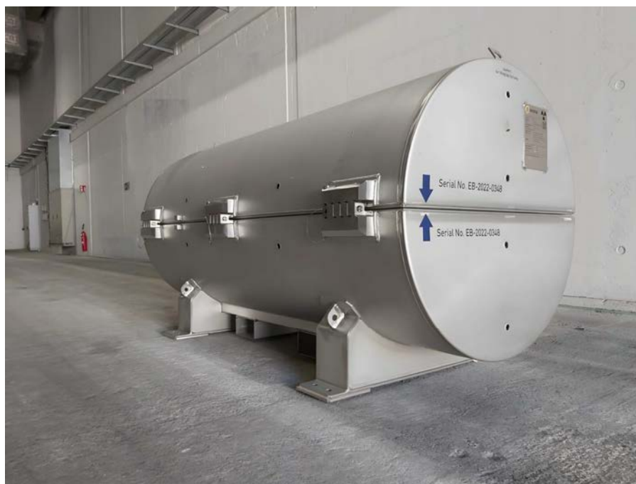
FIG. 24. DN30 outer protection containing a 30B cylinder (courtesy of Orano).
