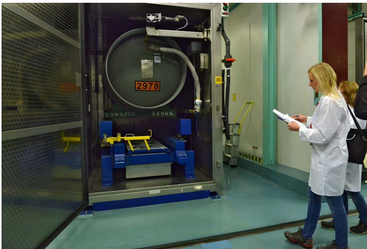
FIG. 23. \text{UF}_6 cylinder connected to heated pigtail.
