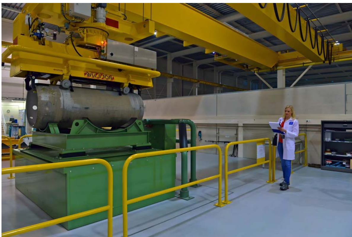
FIG. 18. UF 6 cylinder weighing operations.
