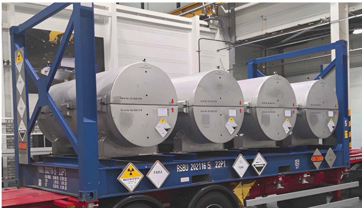
FIG. 30. DN30 outer protection on a flat rack (courtesy of Urenco).
