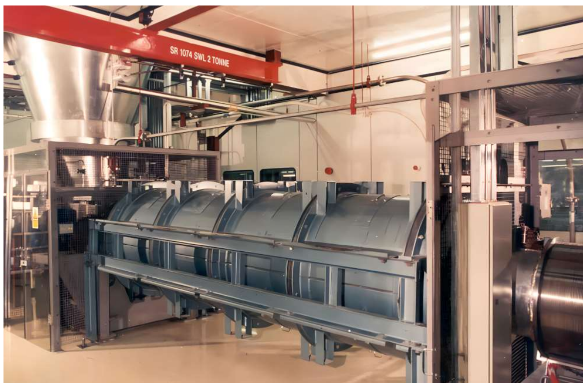
FIG. 8. Rotary kiln for reduction to \text{UO}_2 (courtesy of Westinghouse UK/Springfield Fuels Limited).
