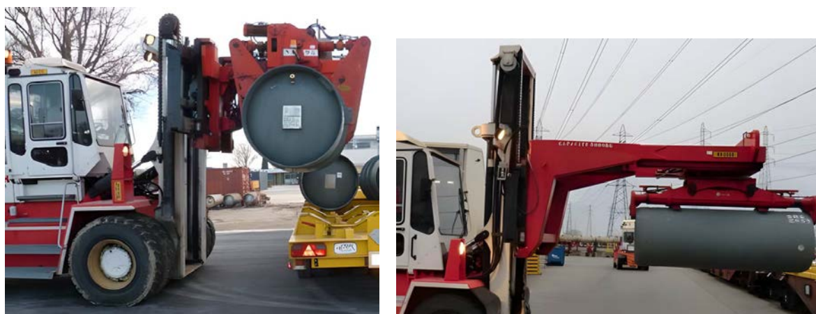
FIG. 21. UF 6 cylinders (48Y and 30B) handling (courtesy of Orano).
