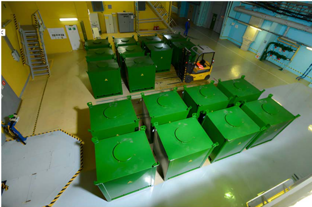
FIG. 10. Containers for long term storage of depleted oxides (courtesy of TVEL).
