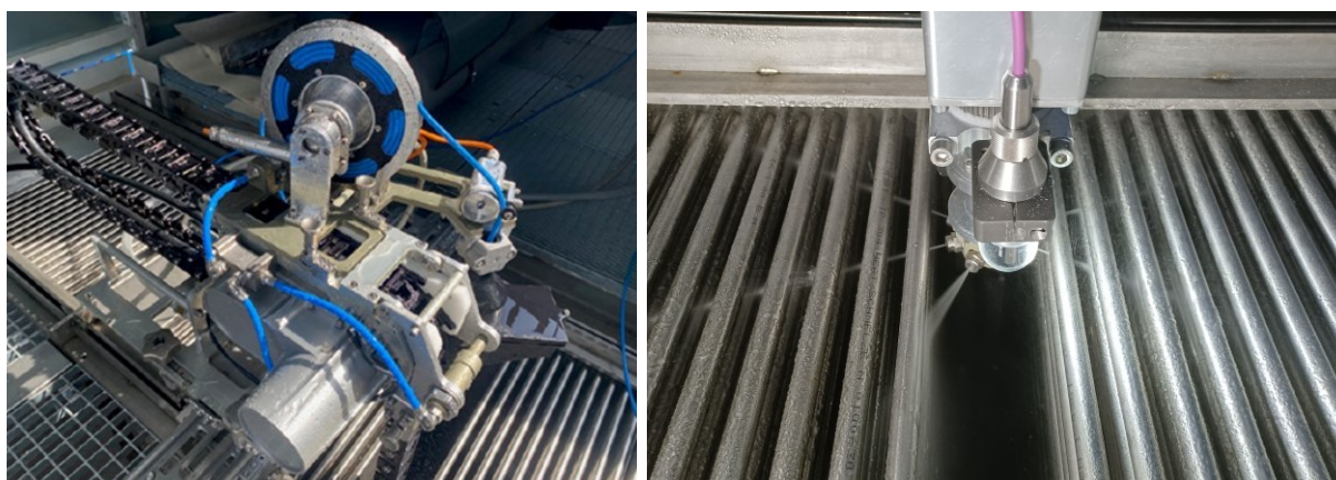
FIG. 51. Steam generator lancing equipment used at Dukovany NPP during qualification tests (courtesy of Framatome).
