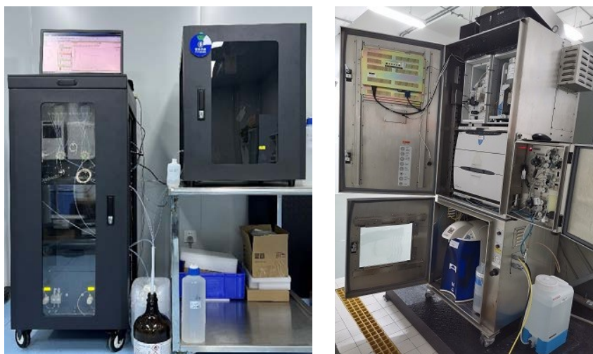
FIG. 64. Prototype of on-line zinc meter (left) and on-line ion chromatograph used in steam generator blowdown system (right) at Sanmen NPP (courtesy of CNNP).
