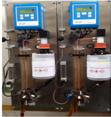
FIG. 69. On-line measurement of hydrazine in the feedwater at Bohunice NPP (Courtesy of Slovenské elektrárne, a.s.)
