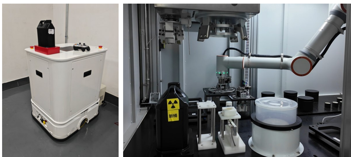
FIG. 78. Robot for transporting radioactive samples from the water treatment system (left) and preparing packages for measurement (right) being operated at Sanmen NPP (courtesy of CNNP).
