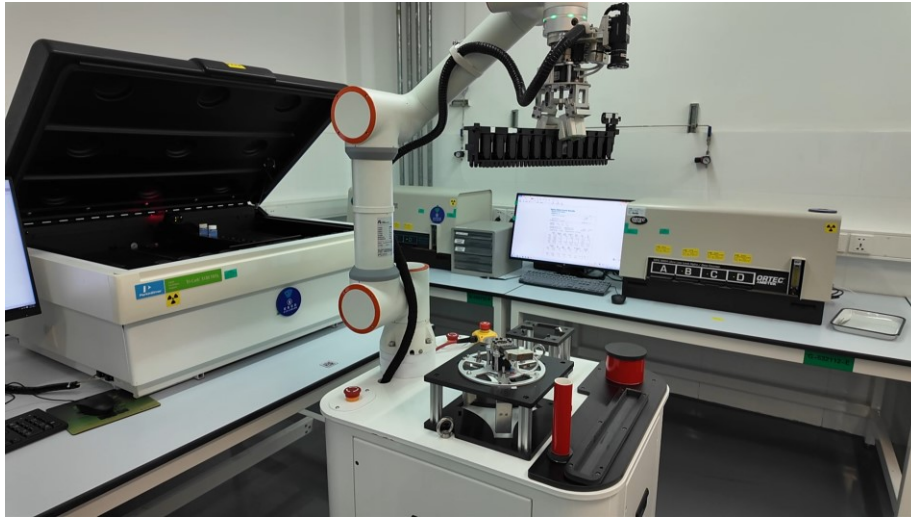
FIG. 79. Robot for preparing samples for a liquid scintillation counter being operated at Sanmen NPP (courtesy of CNNP).
