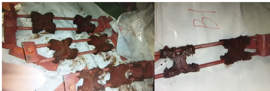
FIG. 48. Horseshoe magnet filters – original design in condenser of Daya Bay-B NPP (courtesy of CGN).
