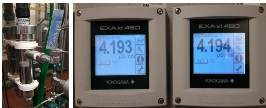
FIG. 71. Probe (left) and analyzers (right) for on-line measurement of conductivity in the feedwater at Bohunice NPP (Courtesy of Slovenské elektrárne, a.s.).
