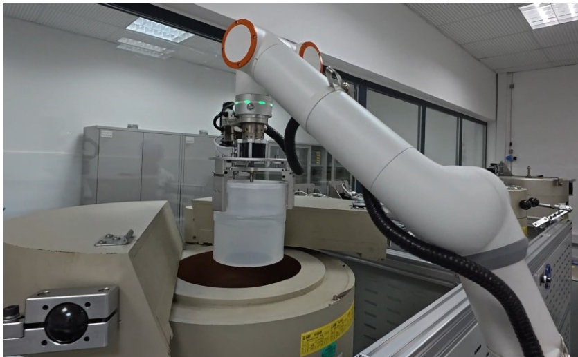
FIG. 80. Robot operating a high-purity germanium detector at Sanmen NPP (courtesy of CNNP).
