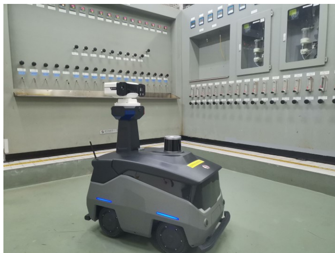
FIG. 81. Intelligent inspection robot for field acquisition of chemistry-related data being developed at Sanmen NPP (courtesy of CNNP).
