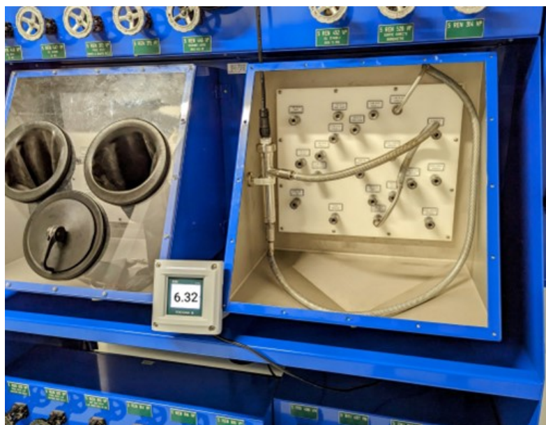
FIG. 66. On-line lithium monitor tested at Gravelines NPP (courtesy of EDF).
