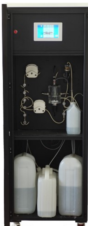
FIG. 65. Prototype of on-line boron meter installed at Sanmen NPP (courtesy of CNNP).
