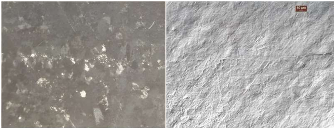
FIG. 8. Metallographic inspection of resistance welding zone of the bearing pad with the cladding.
