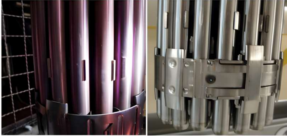
FIG. 2. CNA-2 FAs. Fuel rods with tabs welded to the cladding by resistance welding.
