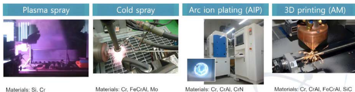
FIG. 3. Applied Coating Methods and Materials for Accident Tolerant Fuel (ATF) Cladding Development at KAERI.
