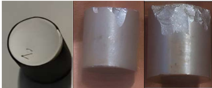
FIG.2. Different mechanical behaviour of pellets after percussion tests.
