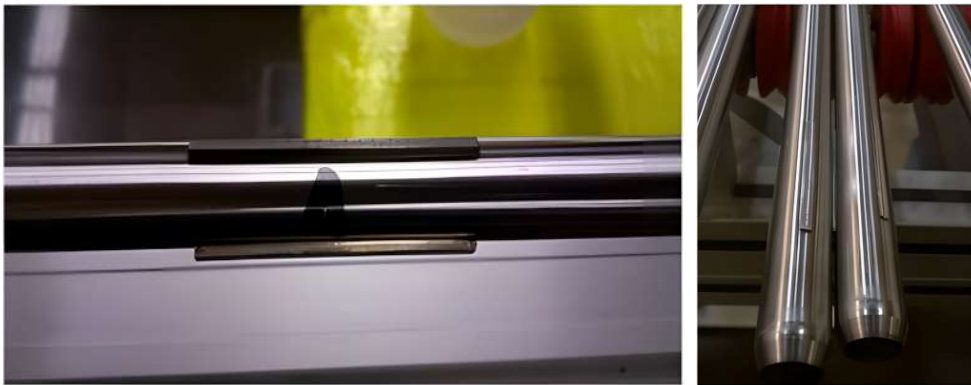
FIG. 3. CNA-1 bearing pads before and after final machining.
