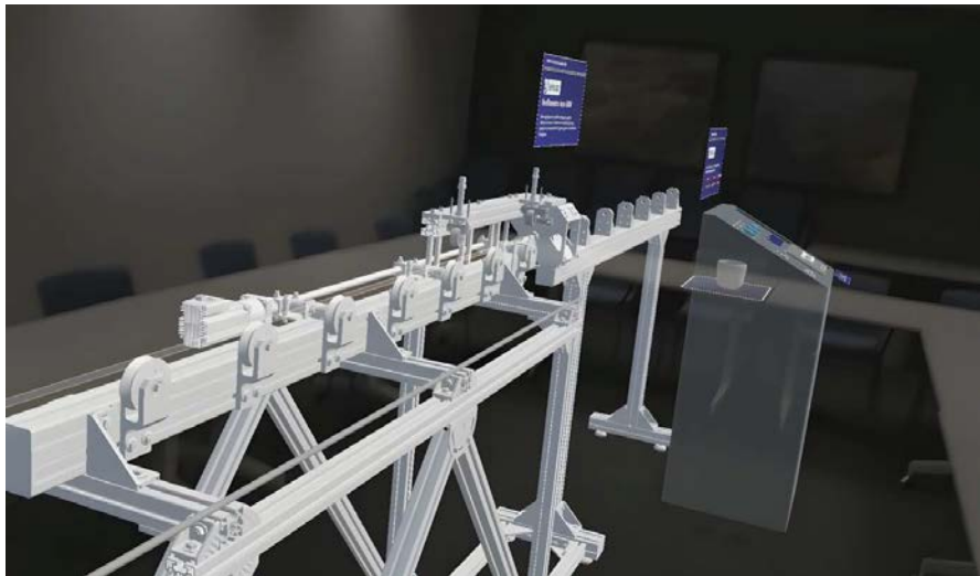
FIG. 5. Virtual model of laser profilometer inspection prototype in an Augmented Reality application.
