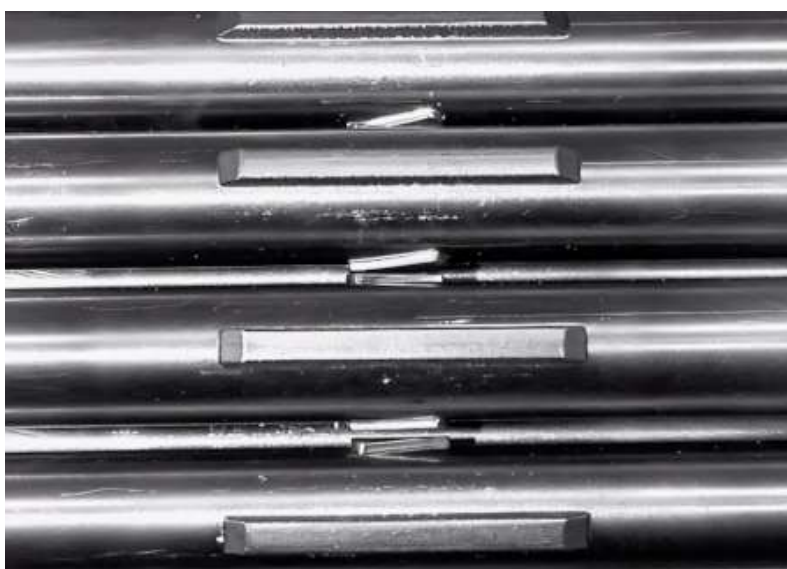
FIG. 2. Close-up view of bearing pads and spacer pads on fuel elements, attached using induction brazing.
