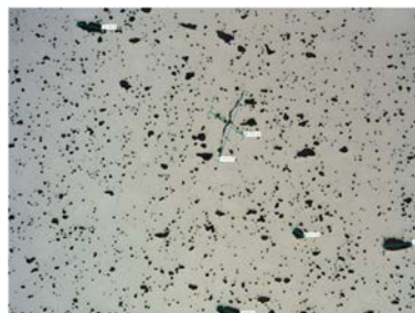
FIG. 6. Small cracks on Gd_2O_3 fuel pellets microstructure.
