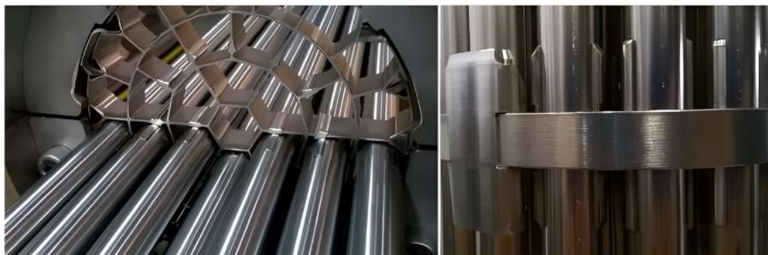
FIG. 1. CNA-1 fuel rods with bearing pads in contact with the spacer grid.
