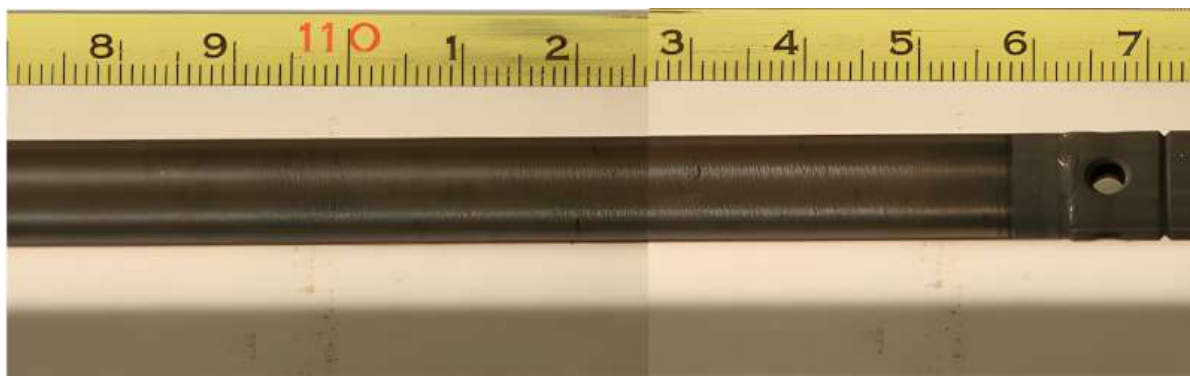
FIG. 11. Appearance of FeCrAl-coated Zircaloy-4 Cladding after One-cycle Irradiation Test in the Halden Reactor.
