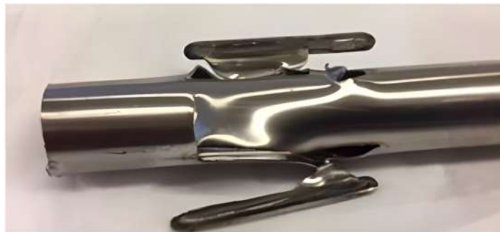
FIG. 9. Manual torque test showing no fracture in welding joints.
