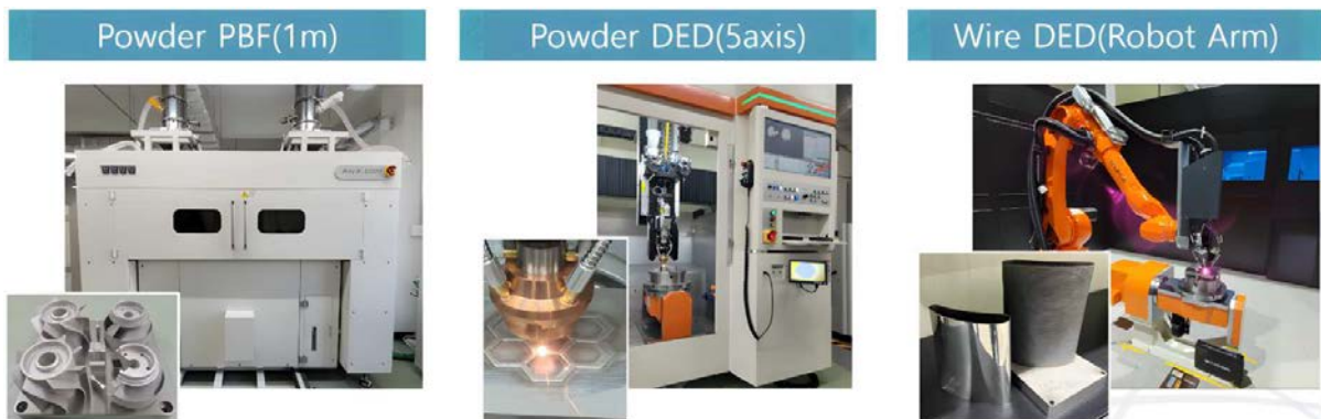
FIG. 15. Developing Various AM Devices after Considering the Material, Shape, Size, and Field Applicability of Parts/Components for Nuclear Application at KAERI.
