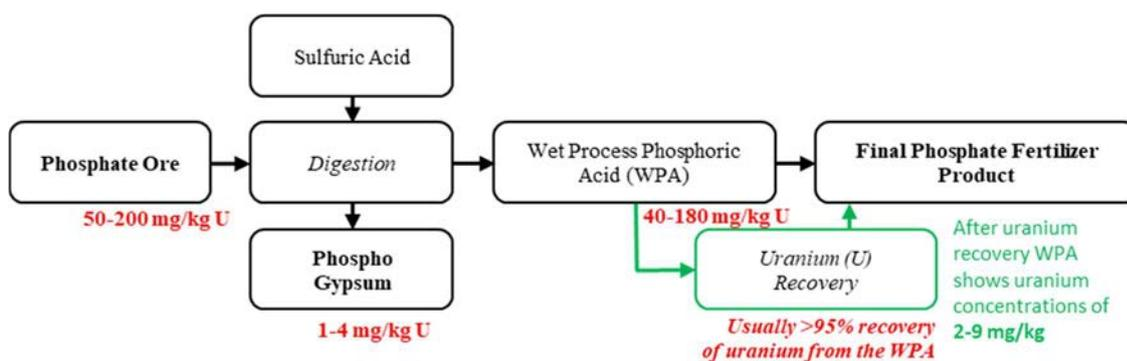
FIG. 3. Simple flow diagram of wet process phosphoric acid (WPA) production with uranium recovery as it was historically done.
