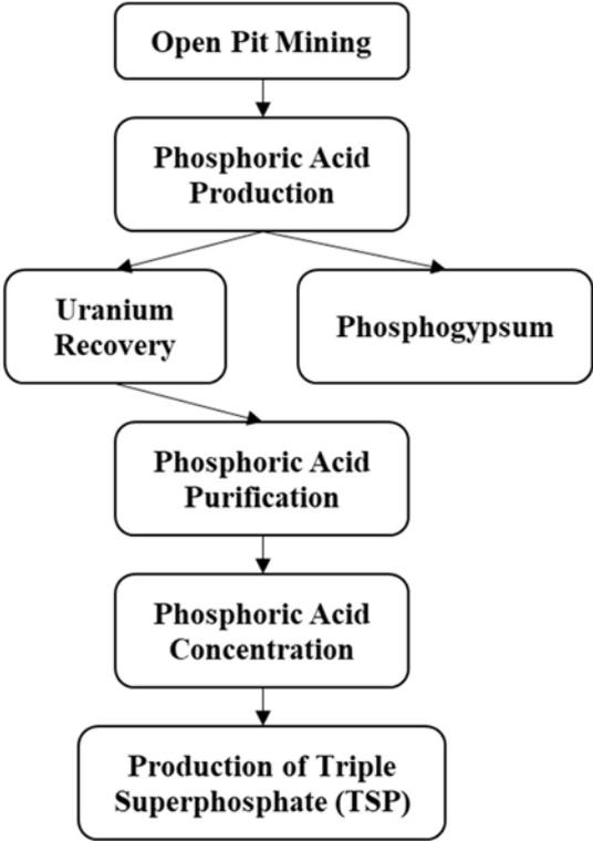
FIG. 12. Proposed flowsheet for developing the Itataia phosphate uranium ore in Northeastern Brazil (courtesy of L.M. da Silva, INB).
