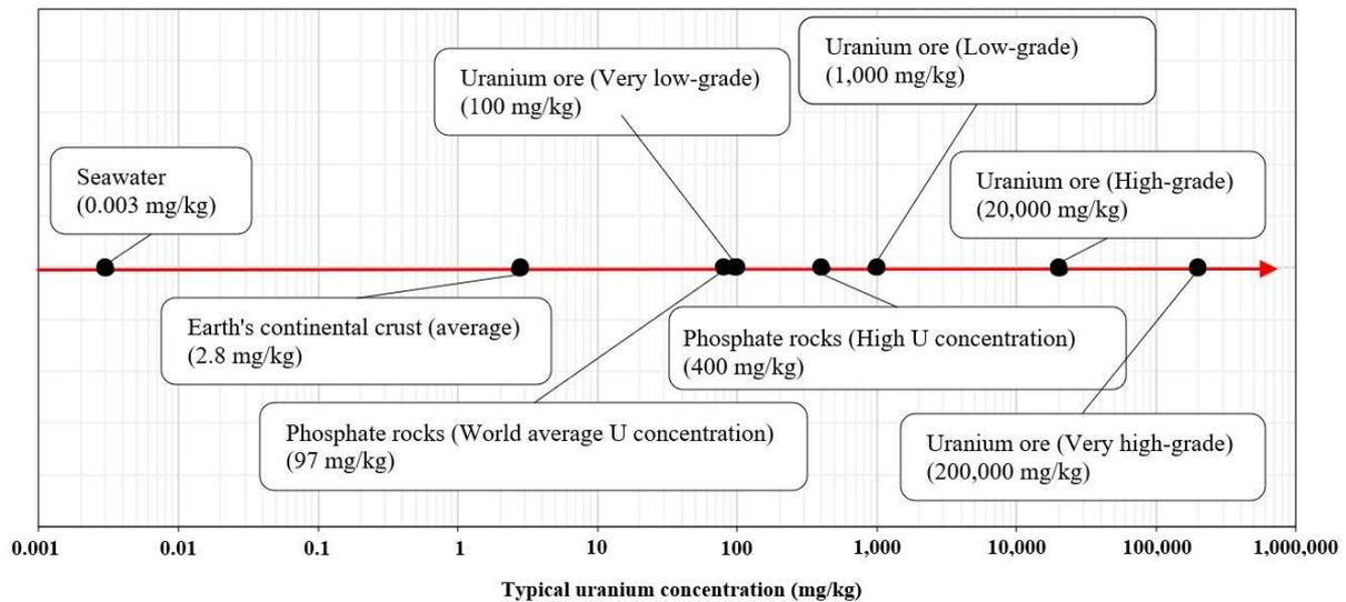
FIG. 1. Uranium concentrations in seawater, phosphates, and various uranium ores, expressed in part per million (ppm).
