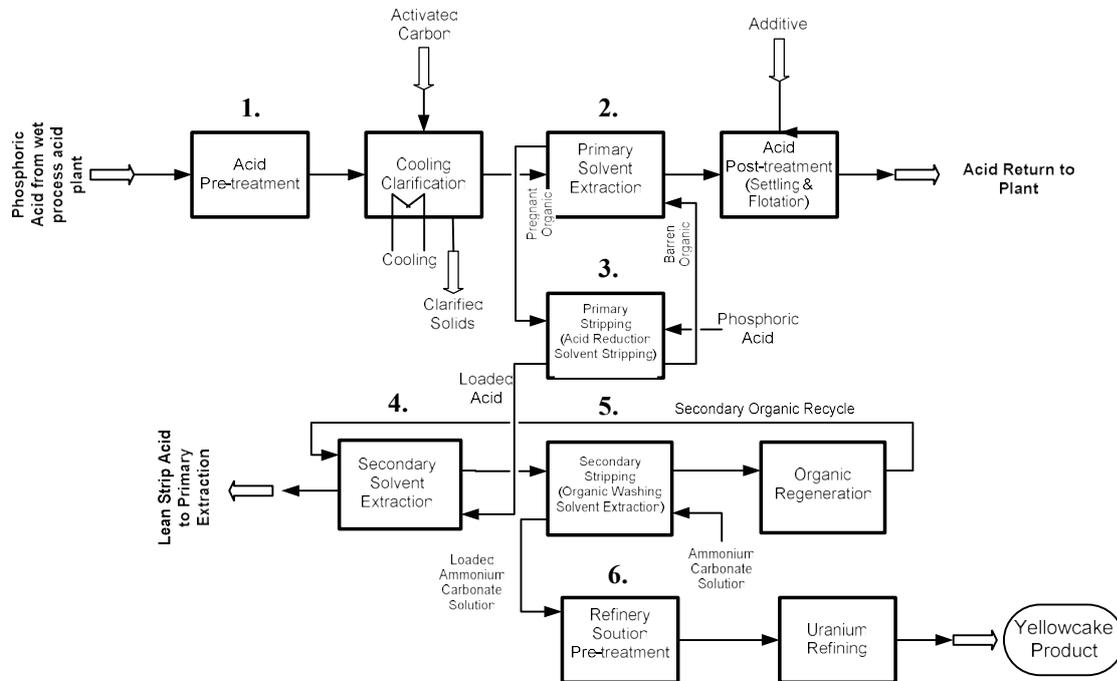
FIG. 4. 2-cycle solvent extraction process used for commercial uranium recovery from wet process phosphoric acid (WPA) in the past (courtesy of V. Astley, Dr. Phosphate Inc).
