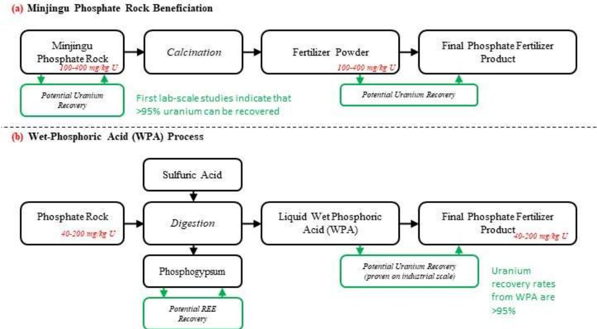
FIG. 17. Comparison of (a) the present Minjingu phosphate rock beneficiation process and (b) the wet phosphoric acid process with sulfuric acid that is commonly used in fertilizer production.
