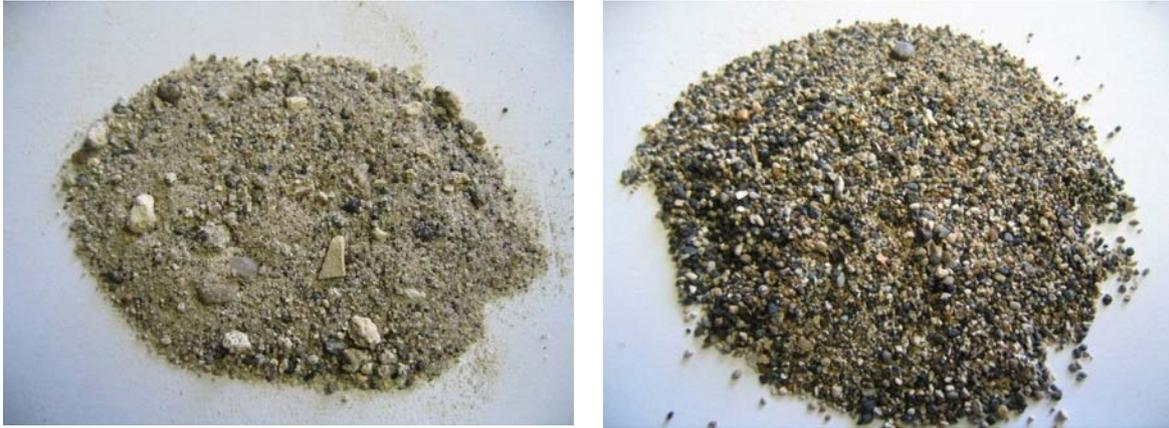
FIG. 2. Sedimentary phosphate ore from Florida (left) and concentrate of this ore after concentration using flotation (right) (courtesy of P. Zhang, Florida Polytechnic University).
