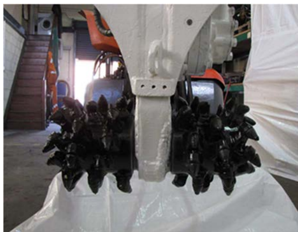
FIG. 5. Nibbling tool and partially removed graphite blocks in an experimental array. (Courtesy of Costain).
