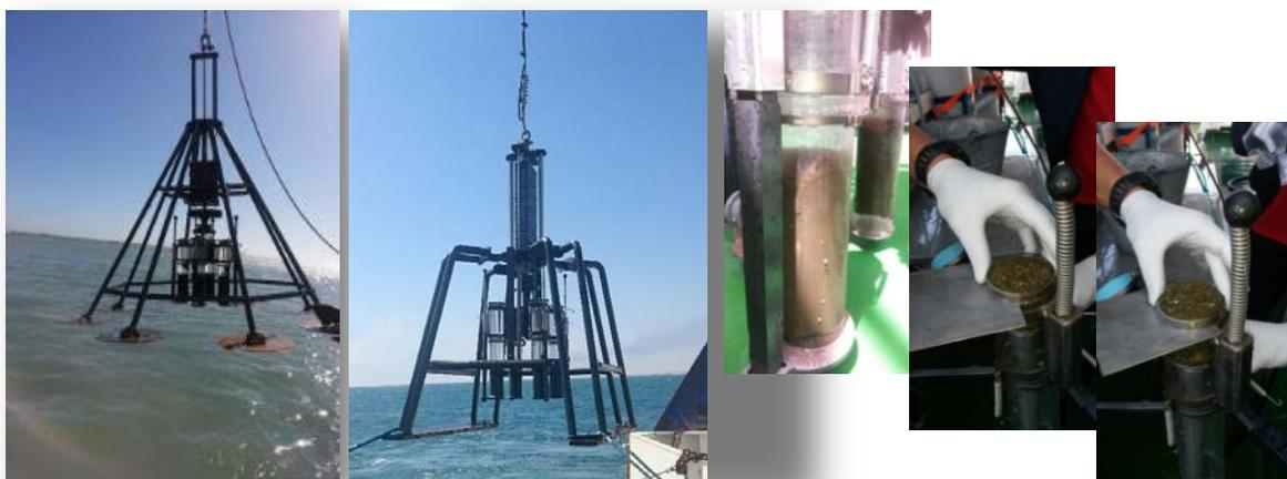
FIG. 3.2. Deployment of box corers on the RV Mirabilis and on board slicing of core sediments.
