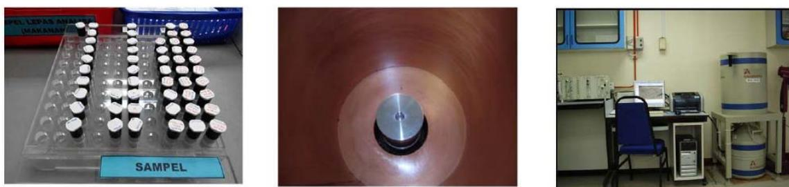
FIG. 6.5. Radioactivity measurement (from left to right): samples, well detector, gamma spectrometry system.
