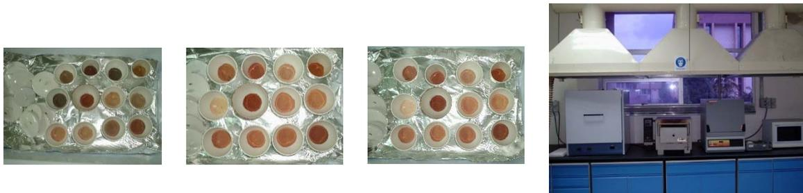
FIG. 6.4. a) LOI (from left to right) at 105°C, 550°C, and 1000°C. b) Furnace for LOI.
