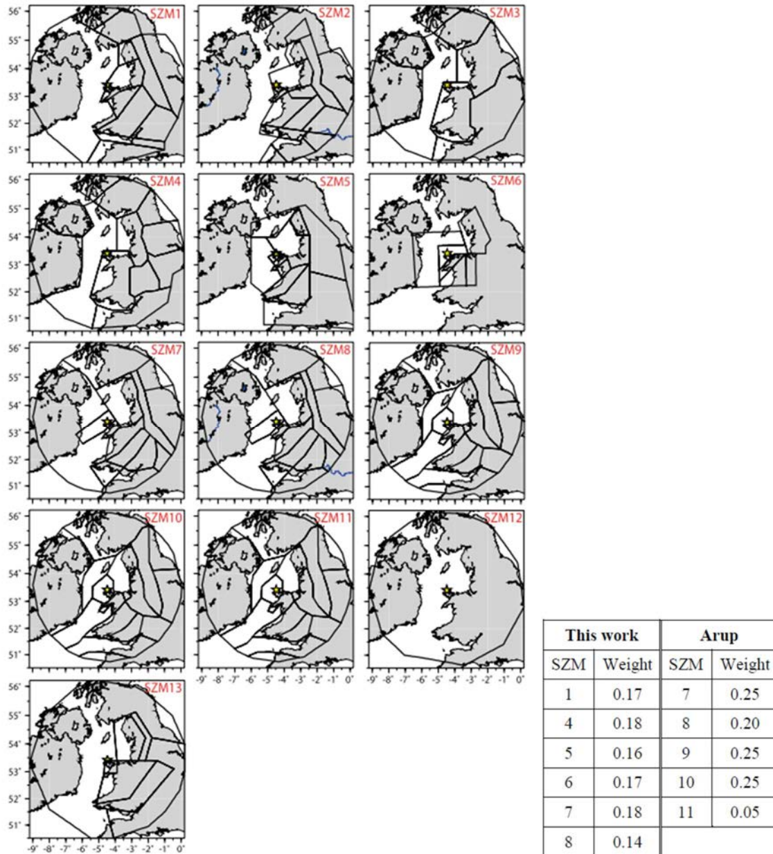
FIG. A–1. Thirteen possible seismic prior source models (left) and the final six posterior models and weights (right) (reproduced from Ref. [A–1] with permission).
