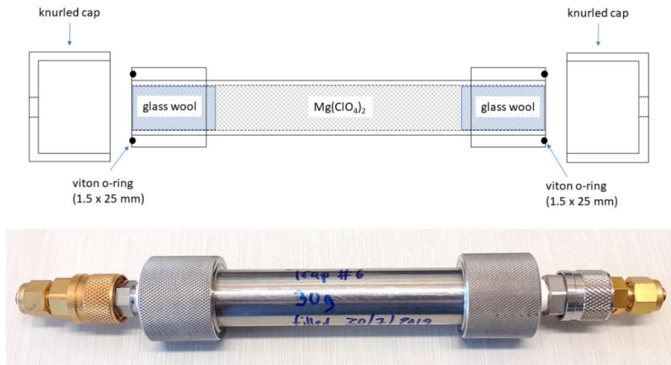
FIG. 14. Water trap design used at NIWA. Top: Schematic of the water trap, showing the position of the Viton o-ring and the extent of the glass wool. Bottom: Photo of filled water trap with quick connectors and brass caps on both ends to prevent moisture absorption while trap is not used.
