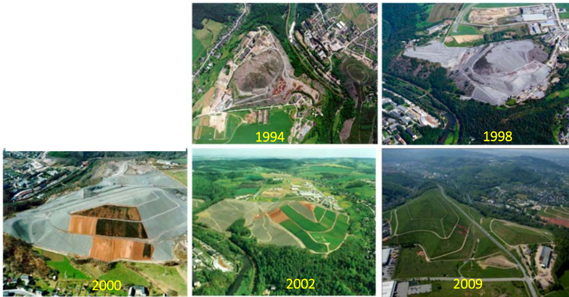
FIG. 3. Contouring and coverage of a big waste rock pile in Schlema-Alberoda (Aue site).
