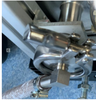
FIG. 30. A picture showing the bottom flange and clamp at the sampler's water inlet port.
