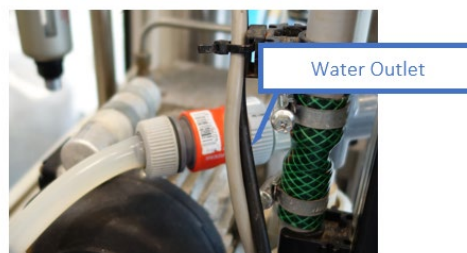
FIG. 11. Connection of water hose from the water outlet port
