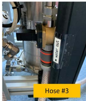
FIG. 31. A picture showing the water outlet port and the connection to the Hose #3.
