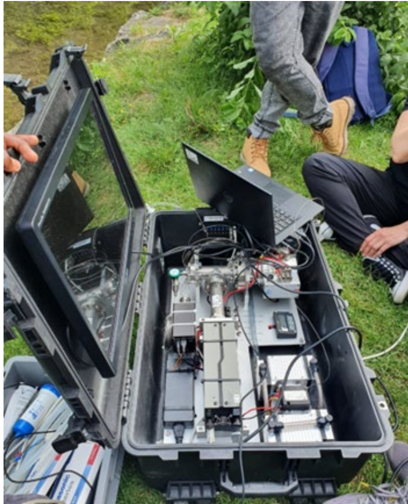
FIG. 6. Portable mass spectrometer system (miniRuedi, Gasometrix) being used in the field to analyze dissolved gases including ^4\text{He} .
