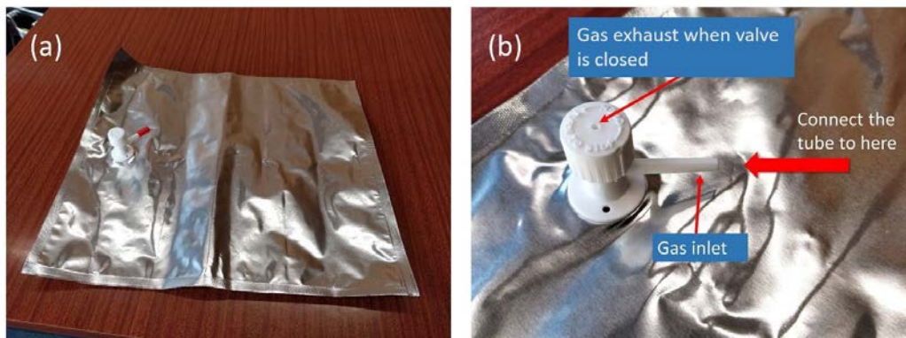
FIG. 2. Sampling Bag Validated for Field Gas Sampling for ATTA Analysis
