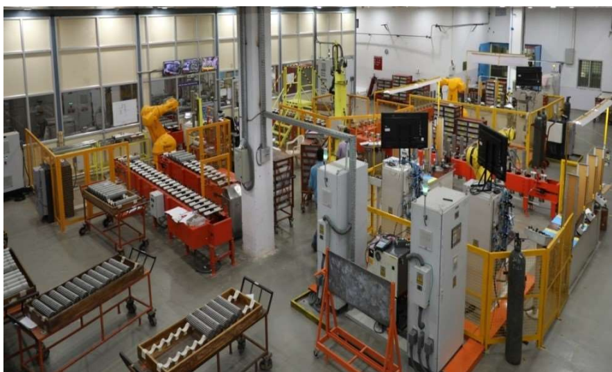
FIG. II-6. Robot aided Fuel Bundle handling and inspection system for 700 MWe PHWR fuel (courtesy of NFC, India)
