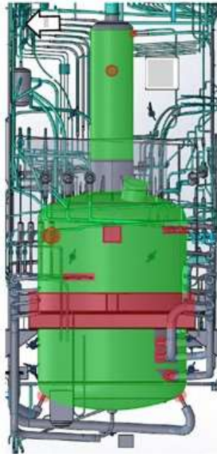
FIG.I-14. Evaporator accessible areas (courtesy of ORANO)
