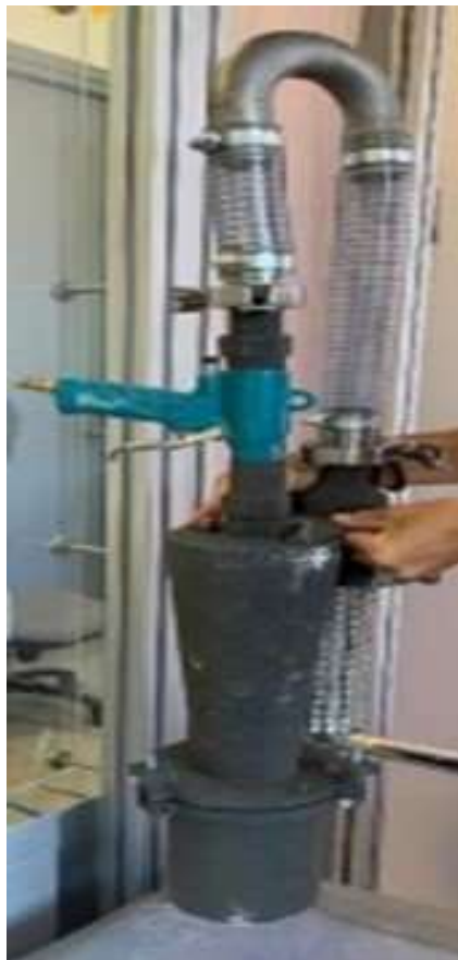
FIG. II-4. Venturi vacuum system to clean GBs without mechanical parts or engine inside (courtesy of ORANO, France)
