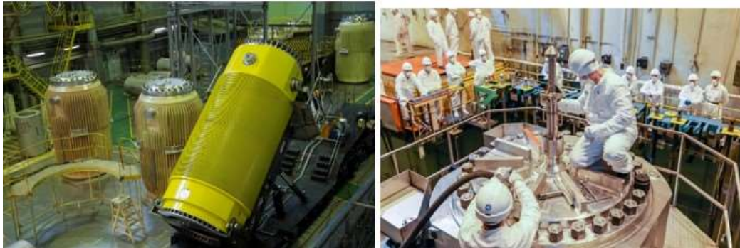
FIG. II–18. (a) Canisters for spent fuel (b) Sealed system (courtesy of ROSATOM, RF)
