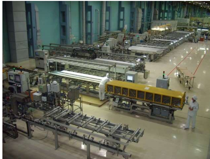
FIG. II–16. Combined manufacturing line for fuel rods and fuel assemblies (courtesy of TVEL, RF)
