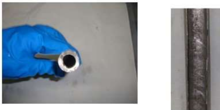
FIG. I-16. Tube thinning in failed TSE (courtesy of BARC, India)
