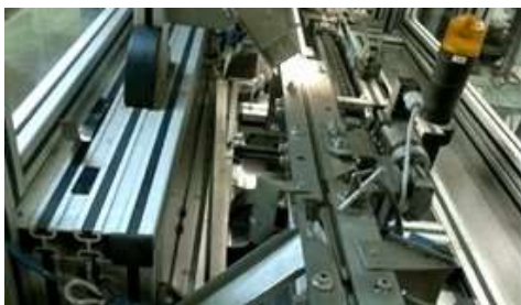
FIG. II–12. Automated circumference inspection (courtesy of TVEL, RF)
