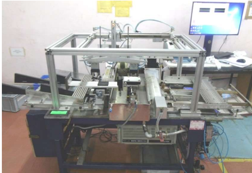
FIG. II-8. Automated UT system (courtesy of NFC, India)
