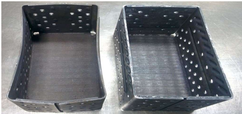
FIG. 8. (a) Pure Mo charge carrier boat (b) ODS Mo charge carrier boat (after 200 thermal cycles) (courtesy of NFC, India)
