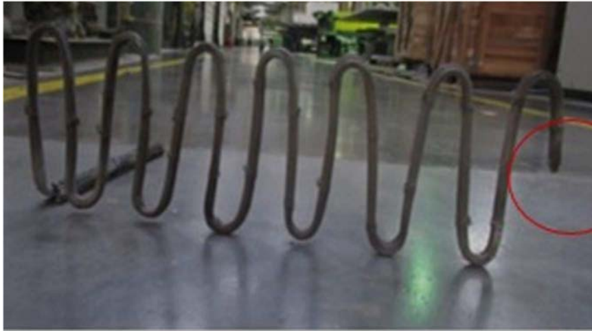
FIG.11. Failed pure Mo heating element (courtesy of NFC, India)
