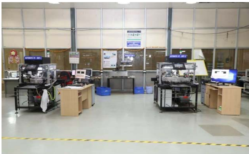
FIG. II-7. Ultra-sonic end cap weld scanning unit (courtesy of NFC, India)
