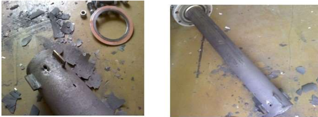
FIG. 7. Nitride scale formation on the outer surface of tube in contact with ammonia (courtesy of NFC, India)
