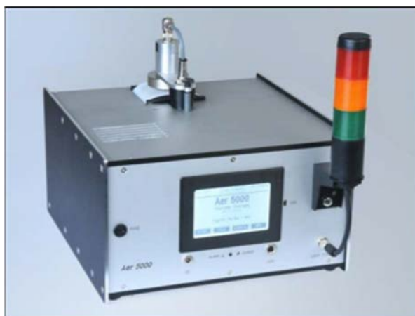
FIG. 20. Aerosol monitoring system used to measure ^{225}\text{Ac} presence in the air of laboratory dedicated to [^{225}\text{Ac}]\text{Ac} -radiopharmaceutical production (courtesy of C. D'Alessandria, TU Munich).
