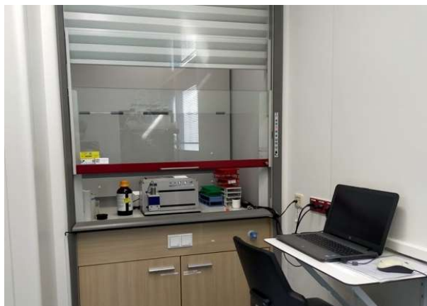
FIG. 8. An example of a fume hood where the TLC scanner is housed to perform ITLC scanning with high enough activity to obtain a good chromatogram (courtesy of E. de Blois, Erasmus MC).
