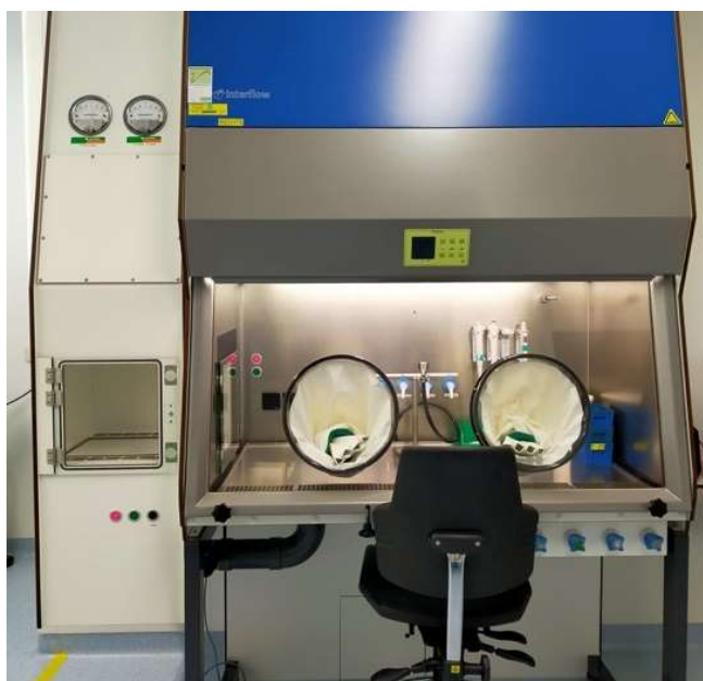
FIG. 6. An example of an isolator where radiolabelling of ^{225}\text{Ac} based radiopharmaceuticals occur (courtesy of E. de Blois, Erasmus MC).
