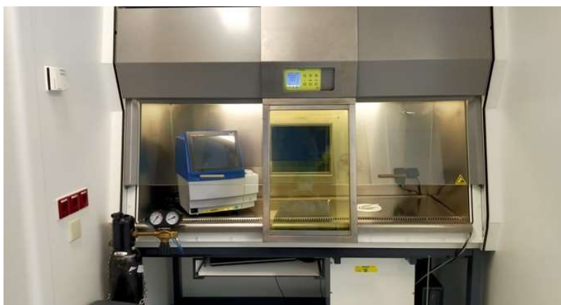
FIG. 7. An example of a LAF where the heating source (microwave) is housed used during production of ^{225}\text{Ac} radiopharmaceuticals, including the dose calibrator for measurement of ^{225}\text{Ac} activity (courtesy of E. de Blois, Erasmus MC).
