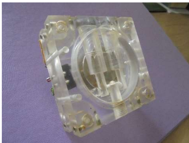
FIG. 3. Example of 1 direction rotation assembly with dual tube system connection, for use with 14 MeV neutron generator (courtesy of P. Bode, TU Delft).
