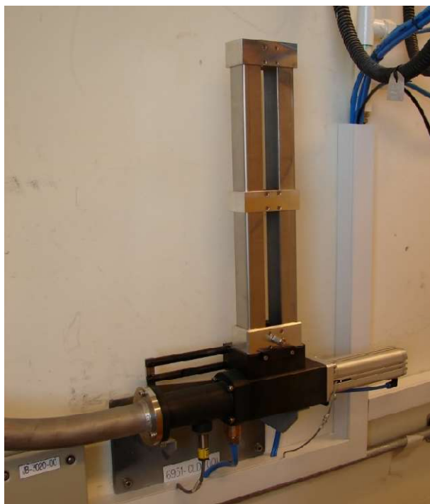
FIG. 14. Example of a vertical stack loader at the OPAL reactor (courtesy of A. Stopic, ANSTO).
