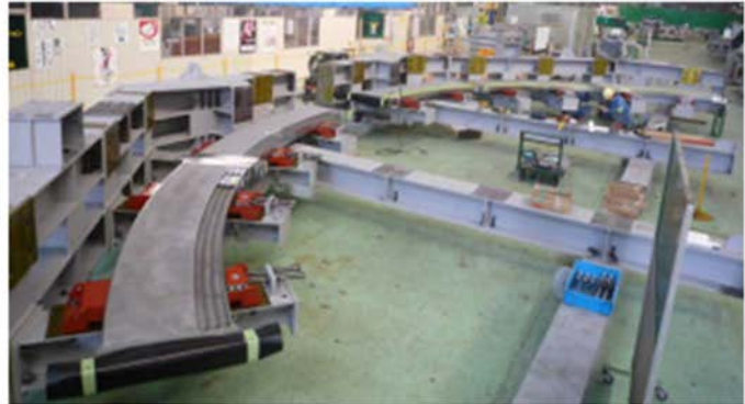
(Before machining groove at welding joints between RP segments)
