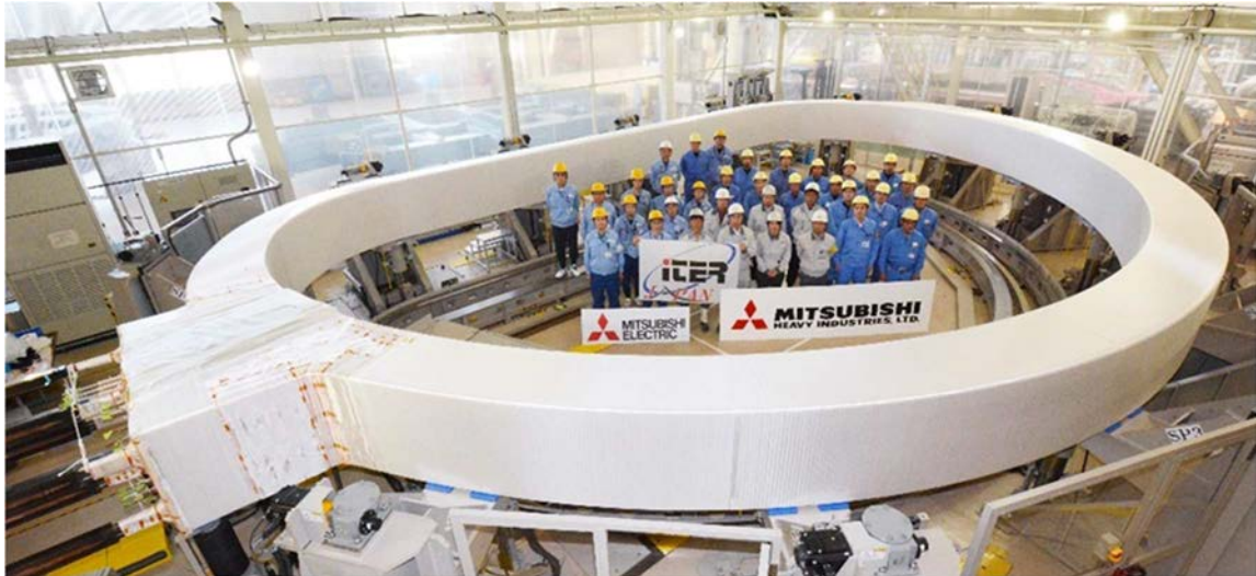
FIG. II-19. Winding pack after wrapping the ground insulation.
