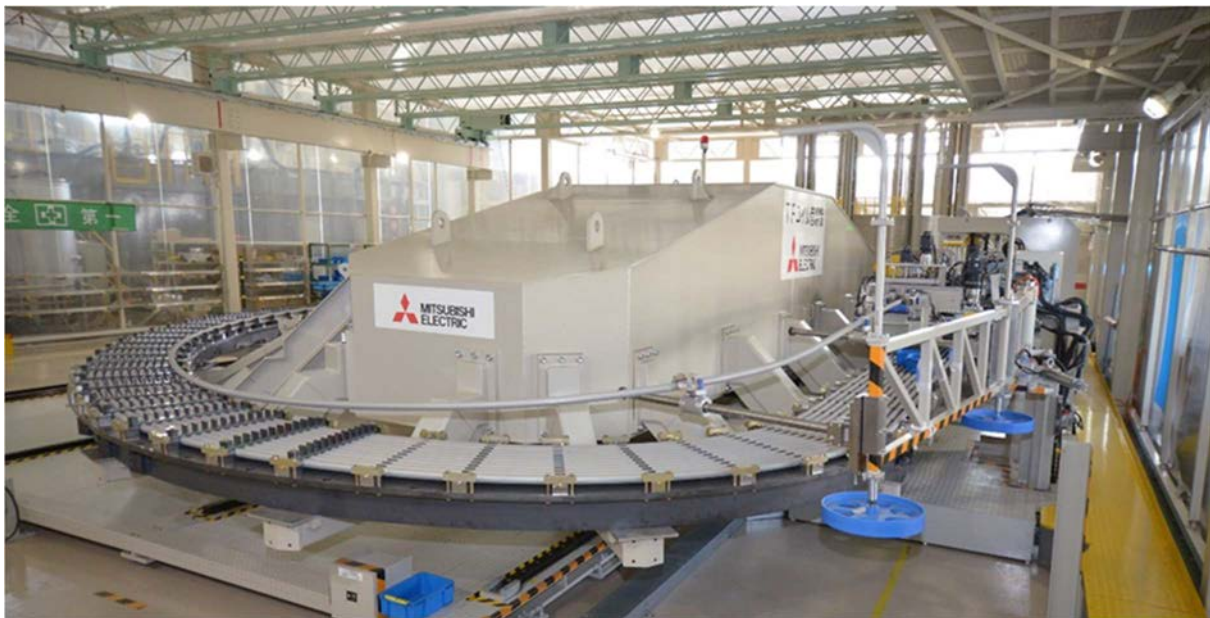
FIG. II-5. Winding toroidal field conductor.
