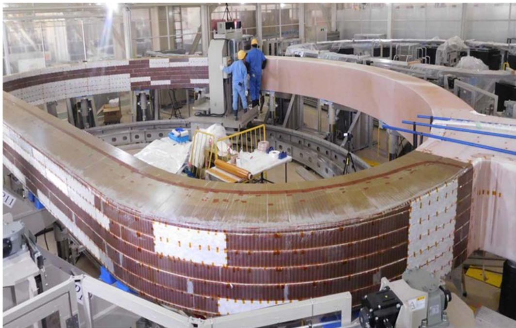
FIG. II-18. Winding pack ground insulation wrapping.
