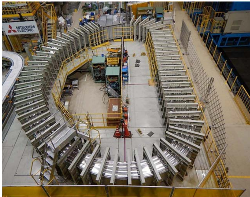
FIG. II-20. Winding pack before impregnation (winding pack is in mould).
