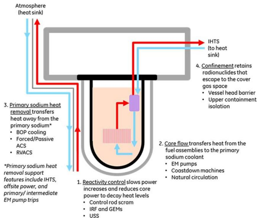
FIG. I-5. PRISM PSA safety functions<sup>2</sup>.
