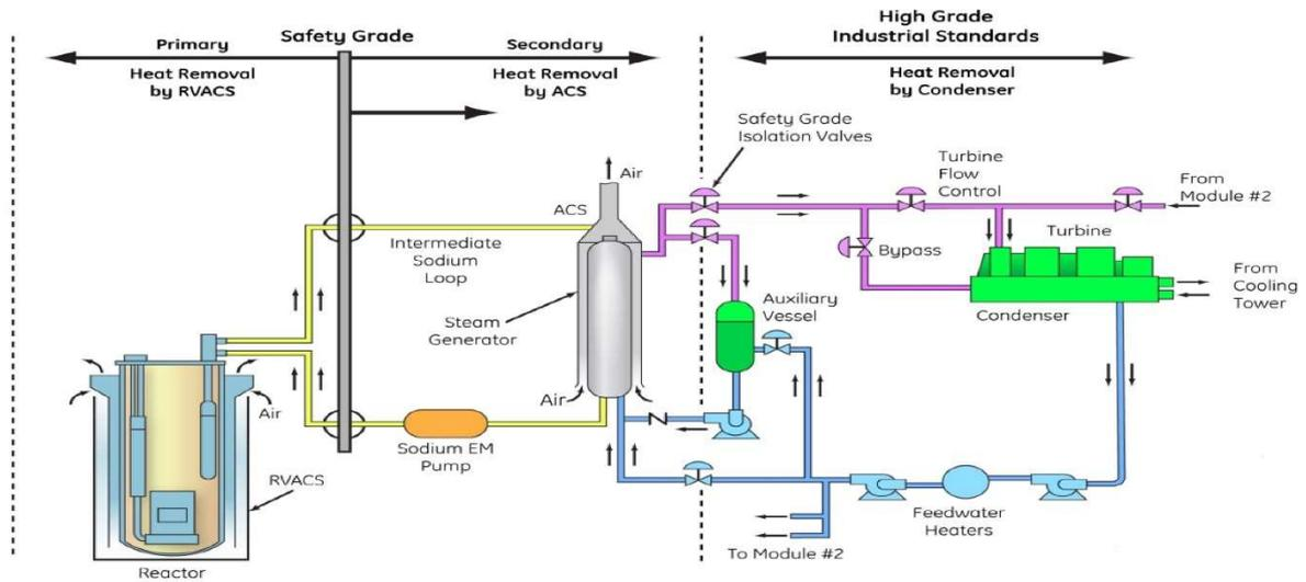
FIG. I-1. PRISM nuclear steam supply system.
