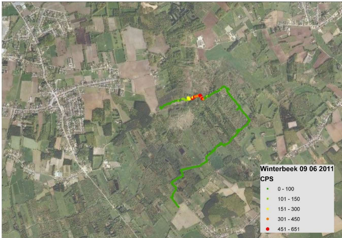
FIG. 71. Gamma flux measurements on the banks of the Winterbeek stream. These may reach 15 times background values.
