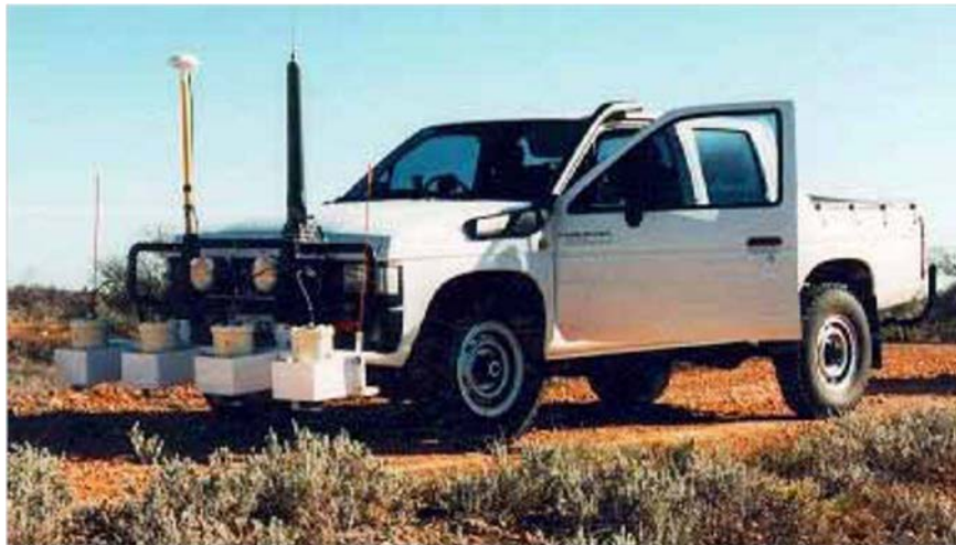
FIG. 39. The system used for measuring the number of particles per square metre.
