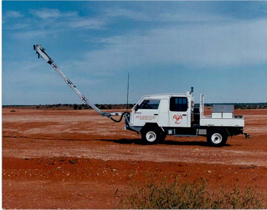
FIG. 38. The purpose-built system used for testing the area density of finely divided contamination.
