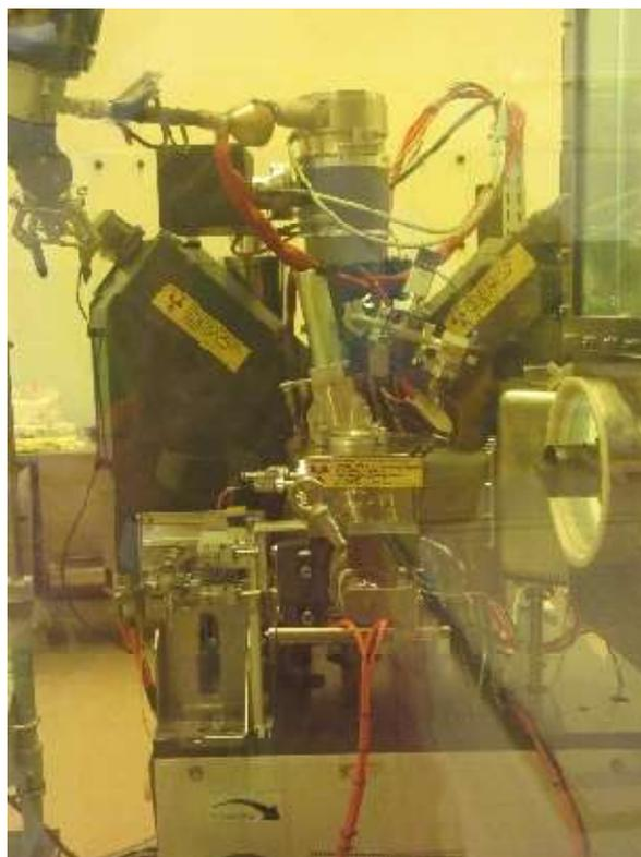
*FIG. 19. EPMA shown through a leaded glass confinement window at IMCL from INL (courtesy of INL)*
