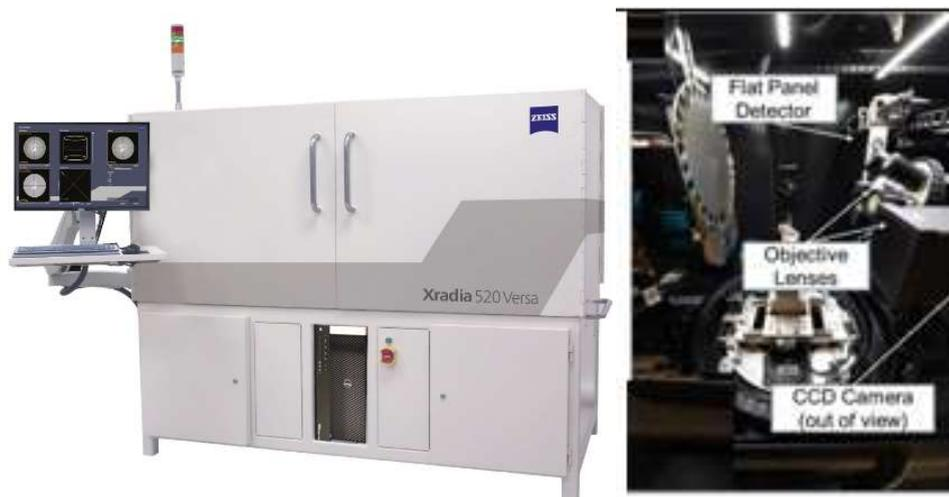
FIG. 9. ZEISS Xradia 520 Versa X-ray microscope located at INL (courtesy of INL)
