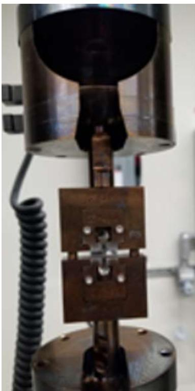
*FIG. 12. The actual subsize specimen fixture and the subsize specimen (courtesy of INL)*
