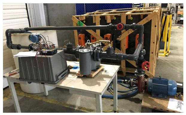
FIG. 17. Photo of duplex strainer dedication testing setup (Courtesy of Kinectrics).
