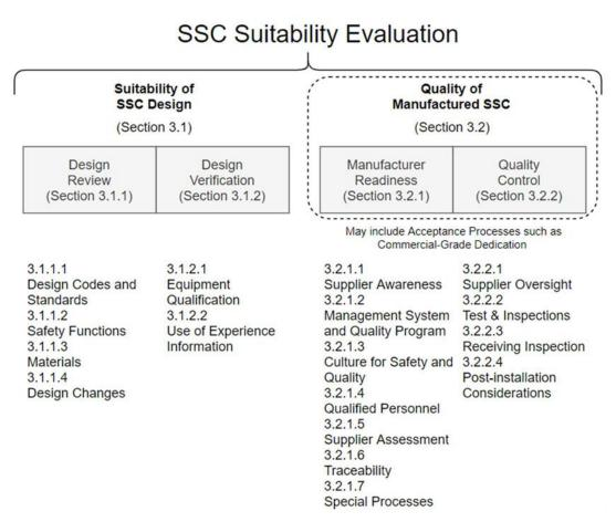
FIG. 2. Main elements of the suitability evaluation process for commercial grade items.
