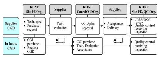
FIG. 8. CGD process steps for performance at supplier or in-house (Courtesy of KHNP).
