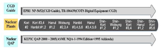
FIG. 7. Nuclear power plants and relevant codes, standards and guidelines for the use of commercial grade items in South Korea. Note Shin-Hanul 1,2 unit and Shin-Kori 5,6 unit are under construction (Courtesy of KHNP).
