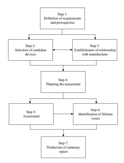
FIG. 3. The COTS device suitability evaluation process according to IAEA NR-T-3.31.
