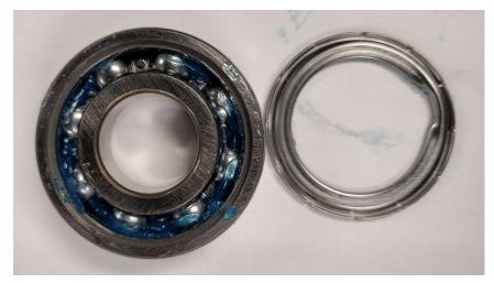
FIG. 12. Photo of commercial grade single-row double-shielded ball bearings (Courtesy of Kinectrics).
