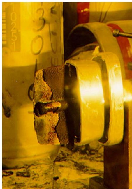
FIG. III-18. The build-up of 'carbon-like' deposits. This figure by the authors of Ref. [III-6] is licensed under CC BY-4.0.
