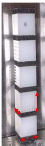
FIG. 31. Cubes of grooved PE moderators of 20 mm dimension (red arrows) used to test the effectiveness of ‘entry’ vs. ‘exit’ grooves (courtesy of K. Thomsen, PSI).
