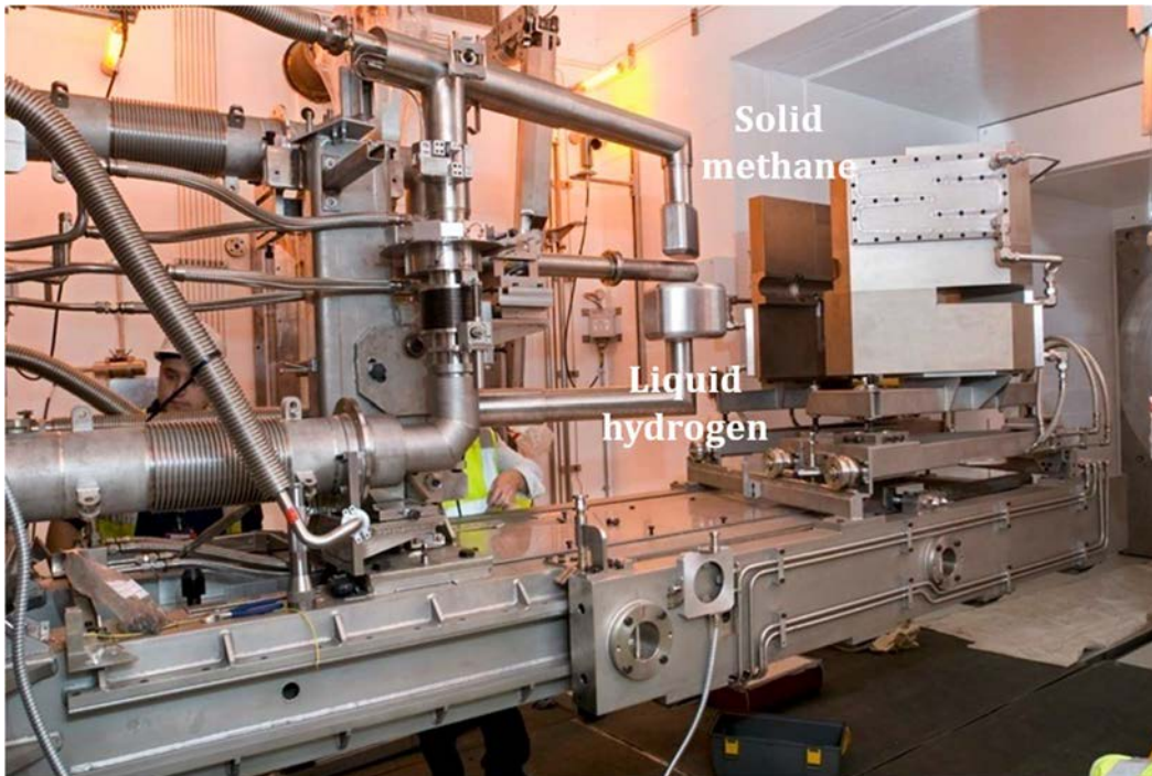
FIG. 13. A view of the ISIS Target Station 2 Target, reflector and moderator assembly showing the target (Ta-clad W cylinder), liquid hydrogen moderator, which operates at 20 K (below the target), solid methane moderator, which operates at 50 K (above the target), and the (split) Be reflector (courtesy of G. Škoro, ISIS Facility).
