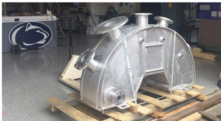
FIG. II-5. The D 2 O moderator tank as delivered for installation (courtesy of K. Ünlü, PSBR).
