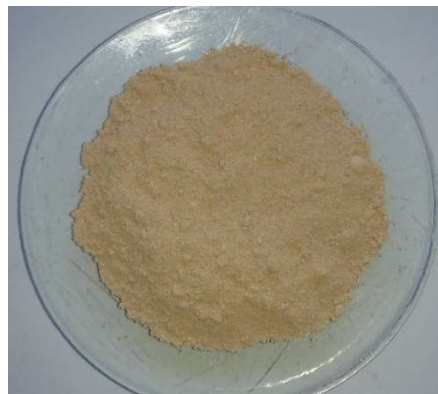
FIG. 3.14. REE(OH) 3 product from alkaline leaching of monazite in Indonesia.
