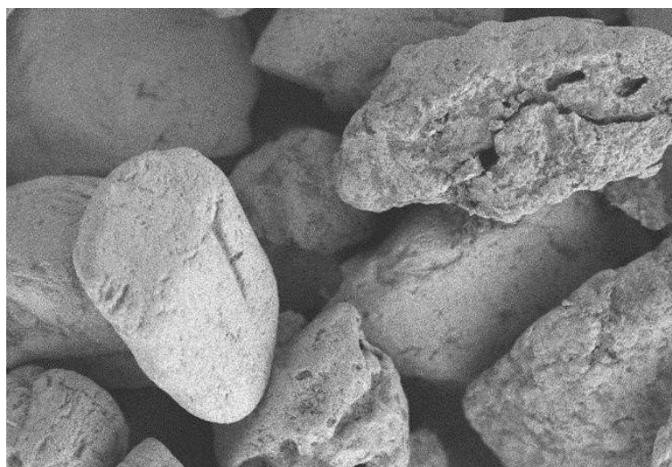
FIG. 3.16. SEM image of representative raw monazite sand from Malaysia.
