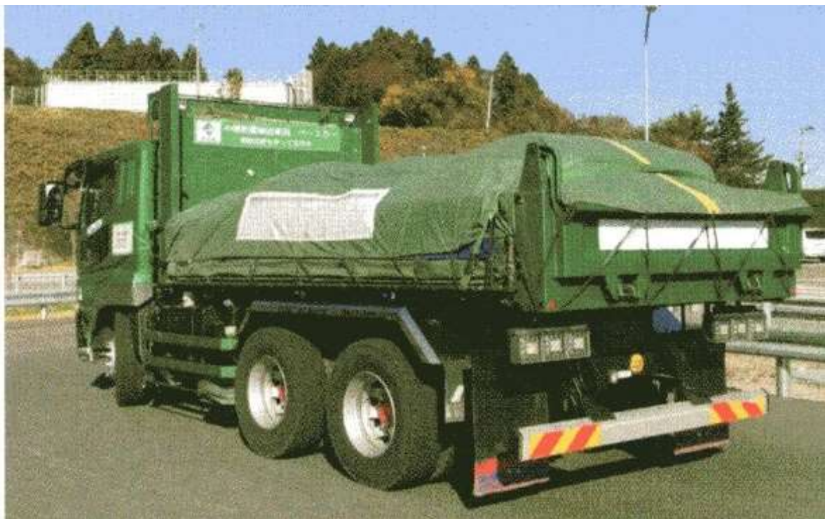
FIG. 26. Truck with waste covered by a protective sheet (reproduced from [31] with permission
