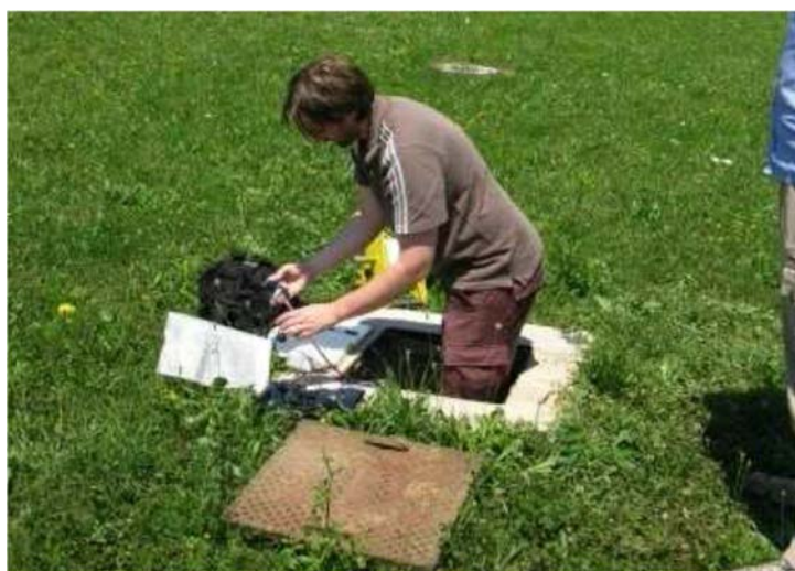
FIG. I-17. Borehole system around the CSF is equipped as piezometer.
