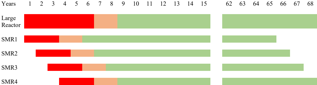
FIG. II-10. Construction and operation schedules with two-year construction delay for the large reactor and the SMRs.
