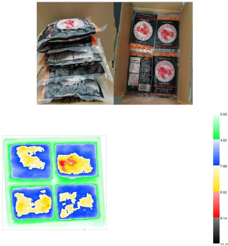
FIG. 18. Frozen shrimps and mass-thickness detection image.
