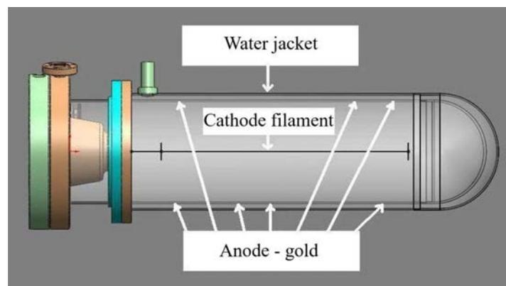
FIG. 1. The Rad Source 4-Pi X ray tube emits X rays in 360 degrees over a large surface area.
