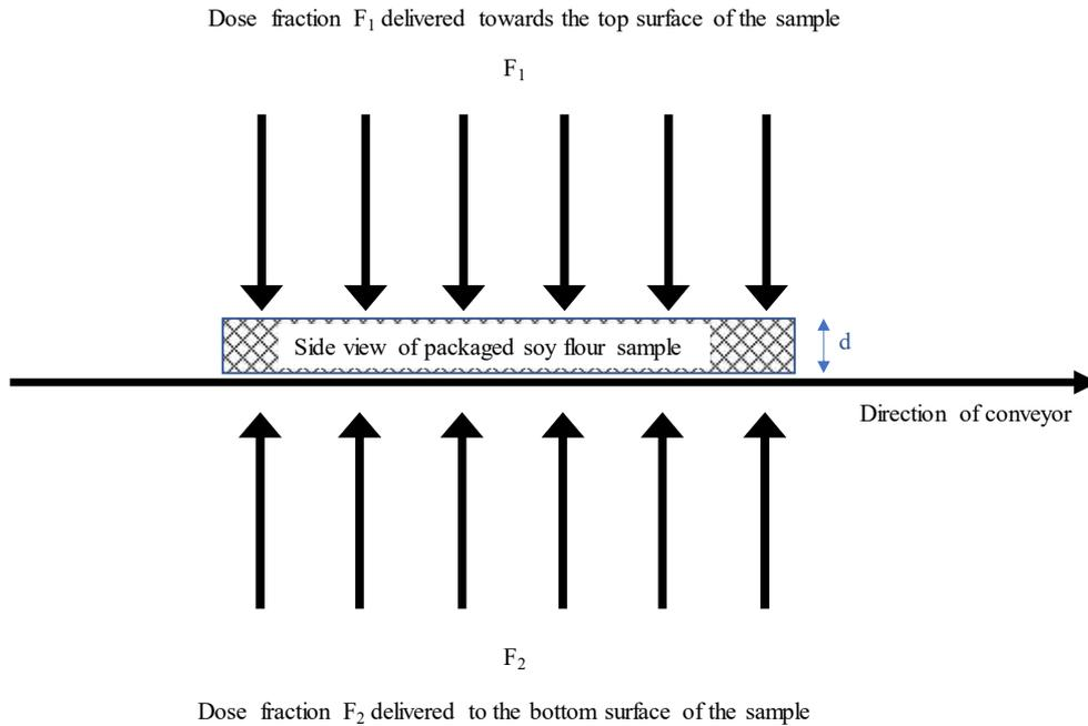
*FIG. 3. Two-sided irradiation,  $d$  is the thickness of the packet of soy flour and the sample is irradiated by dose fraction  $F_1$  from to the top side and then  $F_2$  to the bottom side (the packet is passed through the irradiation zone, flipped by  $180^\circ$  and passed a second time through the irradiation zone).*
