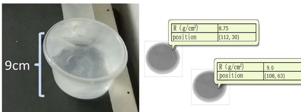
FIG. 10. Mass-thickness for water of 9 cm depth.
