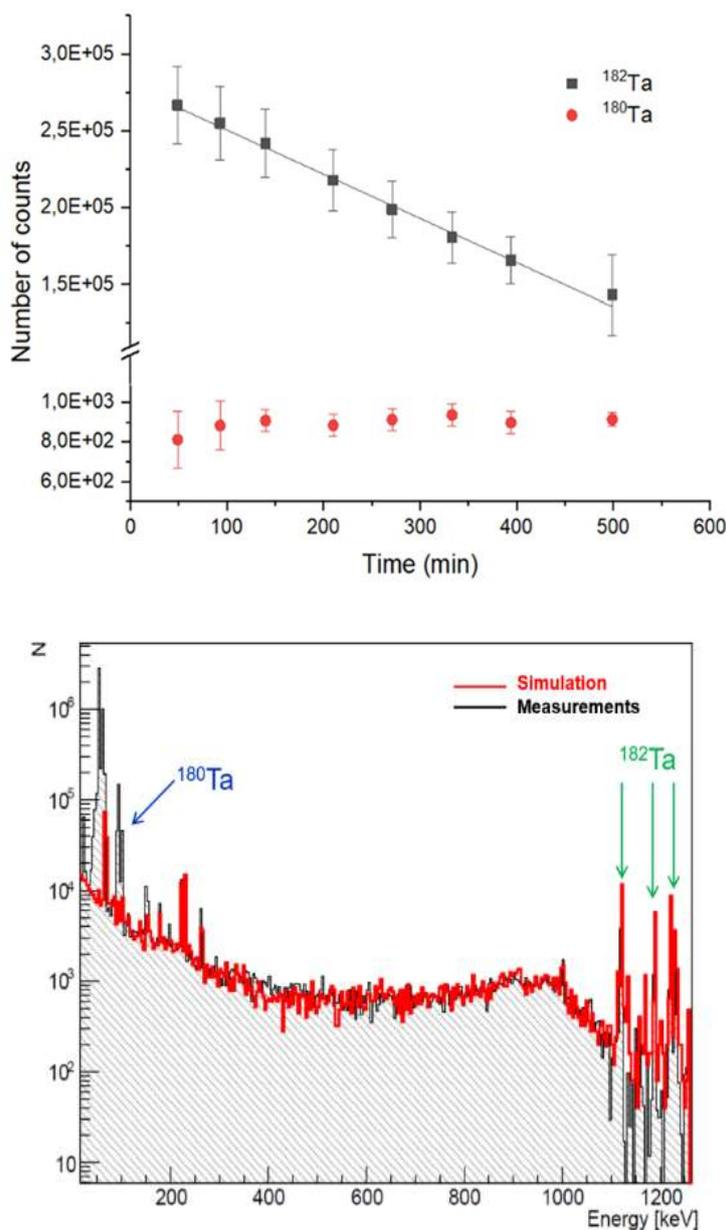
FIG. 3. Radioactive decay (top) and gamma emission spectrum (bottom) of  $^{180}\text{Ta}$  and  $^{182}\text{Ta}$  produced by the irradiation of tantalum plate with 15 MeV photons.
