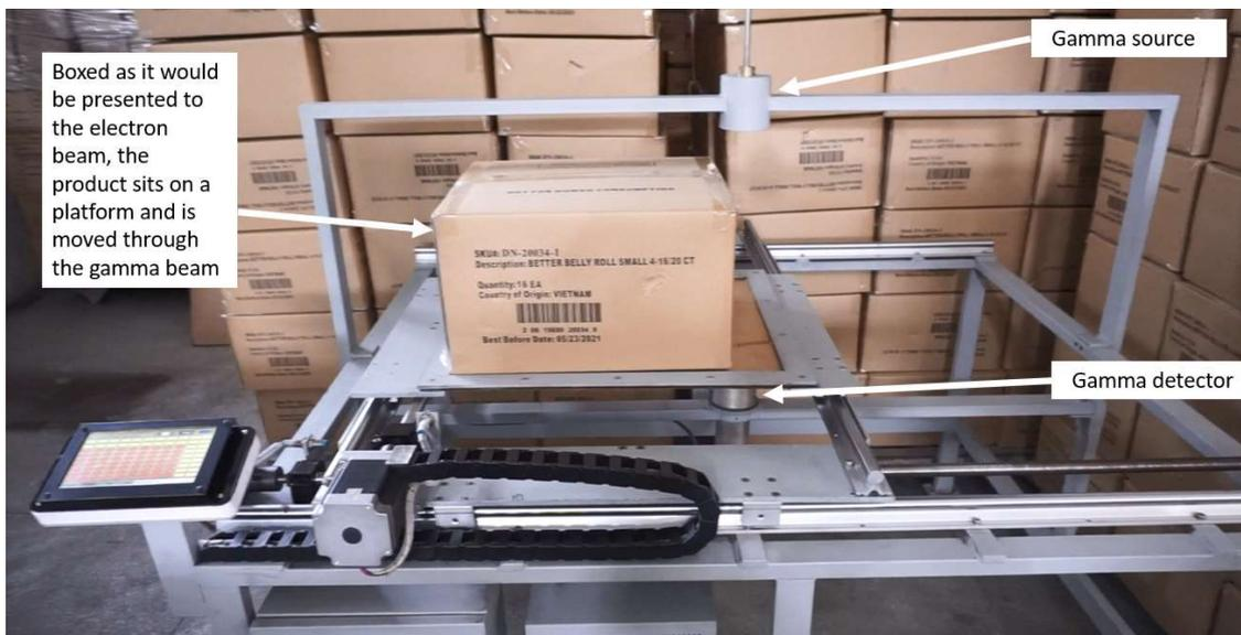
FIG. 9. Density detector device: the product in a standard box carton is passed through the gamma beam to measure mass thickness and predict the dose distributions that would result from electron beam irradiation.
