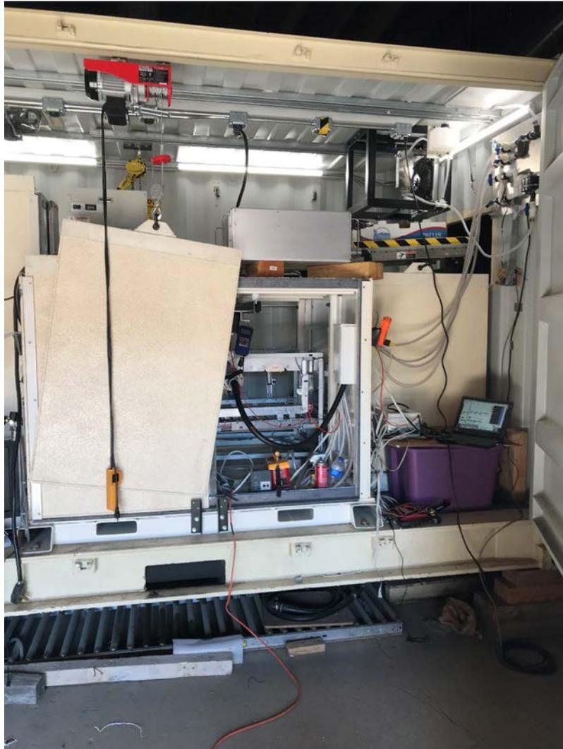
*FIG. 5. The cabinet treatment chamber of BUGS II is shielded using lead panels (February 2020). A pulley system allows for removal of the front panels for access to the X ray tubes and interior of chamber.*
