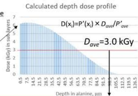
FIG. 10. Depth-dose profile and  $D_\mu$  estimation for 150-keV EB with Electron Beam Accelerator (Model EC250/15/10 mA, Iwasaki Electric, Co. Ltd). Density of alanine dosimeter ( $\rho_2$ ) is 1.482.
