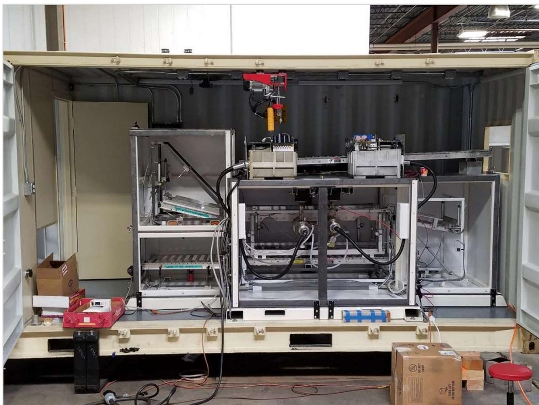
*FIG. 4. BUGS II cabinet X ray irradiator under construction by Applied Energy Devices (July 2018). The lead shielded treatment chamber with conveyor system is housed inside a 6.08 m shipping container.*
