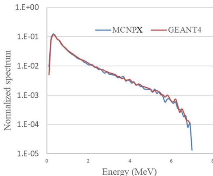
FIG. 6. X ray spectrum calculated from MCNPX and GEANT4 Monte Carlo codes for 7 MeV electron energy spectrum of the IBA Rhodotron.
