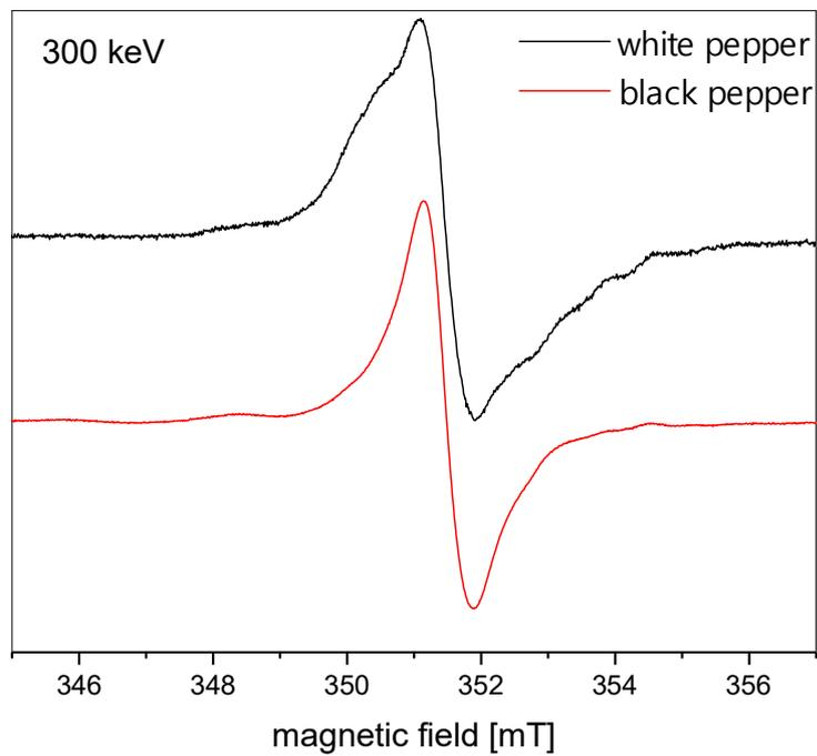
FIG. 10. EPR spectra of black and white peppercorns irradiated with 230 and 300 keV electron beams.
