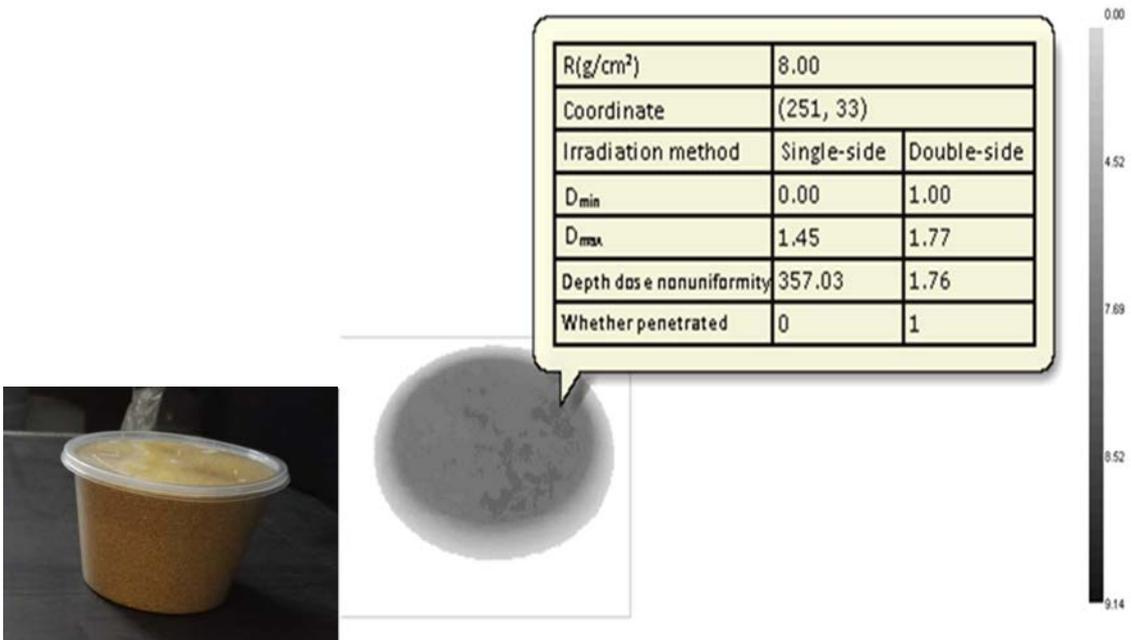
FIG. 14. Mass-thickness for millet of 9 cm depth.
