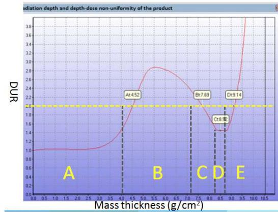
FIG. 7. DUR curve with mass thickness of 10MeV EB.
