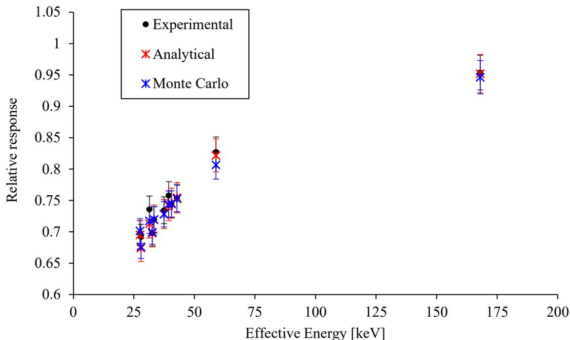
FIG.3. Relative responses of alanine dosimeters to kV X rays obtained by experimental measurements, Monte Carlo (MC) simulations and analytical calculations.
