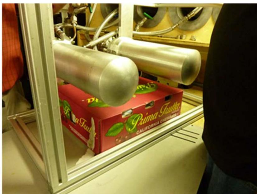
*FIG. 2. Experimental irradiation of sweet cherry boxes using two 4-Pi X ray tubes (Rad Source Technologies, Buford GA, USA).*
