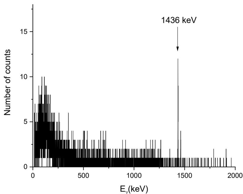
FIG. 9. Gamma ray spectrum of irradiated vanadium sample, with the main emission peak of  $^{52}\text{V}$  at 1436 keV.
