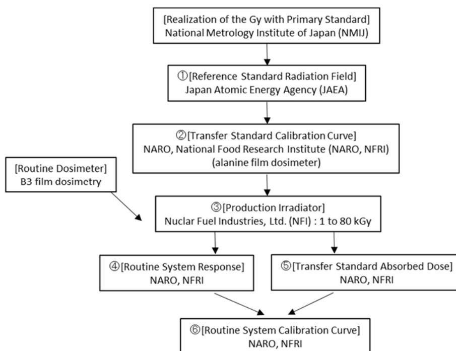
FIG. 1. Calibration procedure of the dosimetry system at NFRI/NARO, Japan and value traceability to the national/international standard.
