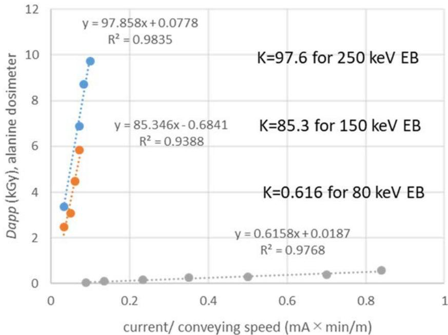
FIG. 7.  $K$  value observed for a low energy EB irradiator (EC 300/30/30 mA, Iwasaki Electric Co., Ltd.).
