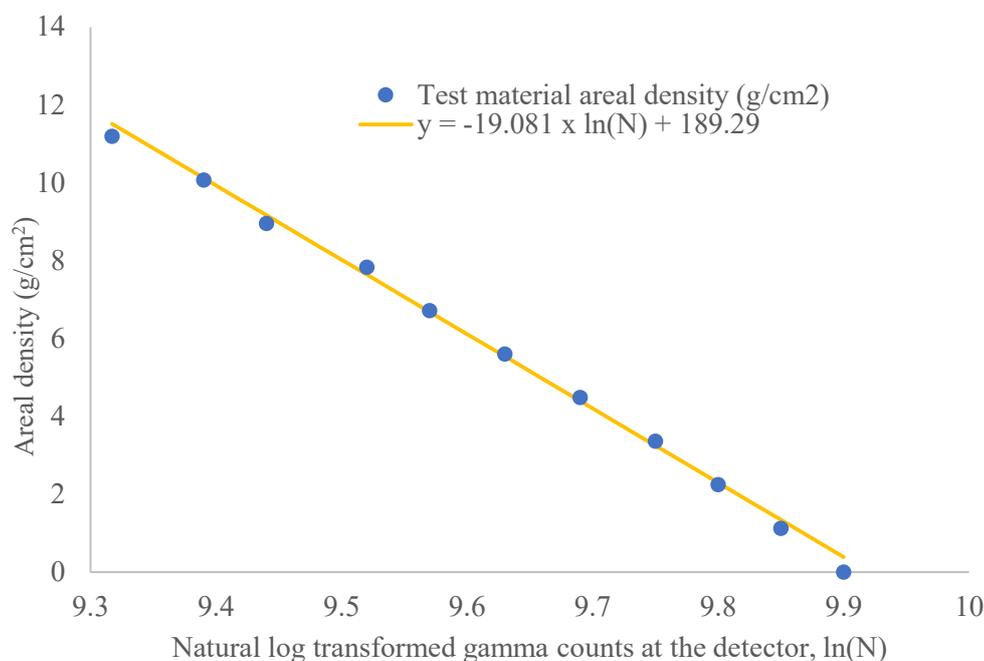
FIG. 10. Plot of gamma intensity at the detector against areal density.
