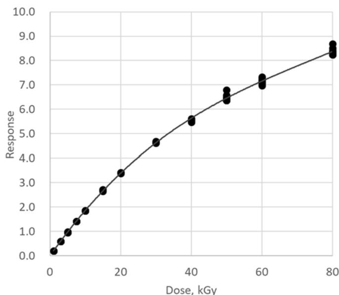
FIG. 2. The ESR signal response from the gamma irradiated alanine dosimeter.
