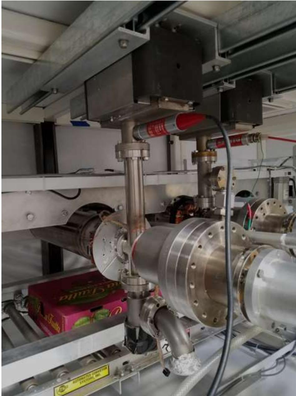
*FIG. 3. The capsule-type X ray emitters in BUGS II. The conveyer system moves boxes of fruit over and then under the X ray tubes for treatment from the bottom and then the top of the box. The over-and-under design improves dose uniformity of the treatment and doubles the volume of fruit that can be treated per unit time compared to a point source X ray tube. The large surface area of the X ray emitter allows for complete coverage of the fruit box during each pass at close range.*
