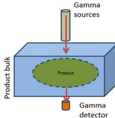
FIG. 1. Experiment layout for areal density detection system via gamma attenuation.
