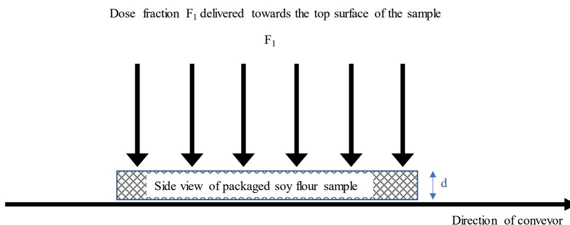
FIG. 2. One-sided irradiation,  $d$  is the thickness of the packet of soy flour and  $F_1$  is the dose fraction. Imparted by the electron beam as it is shone onto the top surface of the sample and passes through the soy flour, perpendicular to the direction of travel through the irradiation zone.
