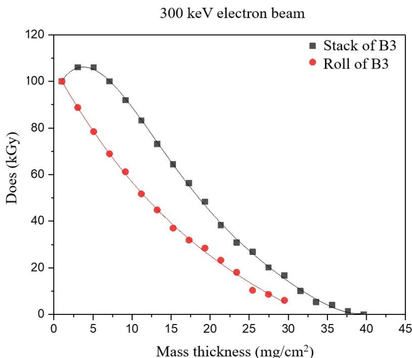
FIG. 5. Depth dose distribution of low energy electron beam determined for flat and round samples under the experimental conditions.
