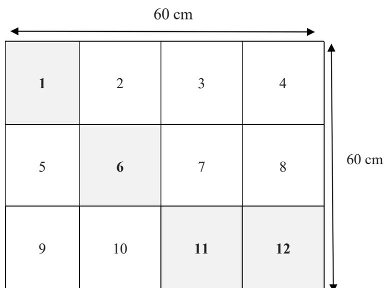
FIG. 1. Top view of sample tray and the placement positions of bagged soy flour samples. Four locations (1, 6, 11 and 12). on the sample tray were used for electron beam irradiation treatments of flat packets of soy flour.
