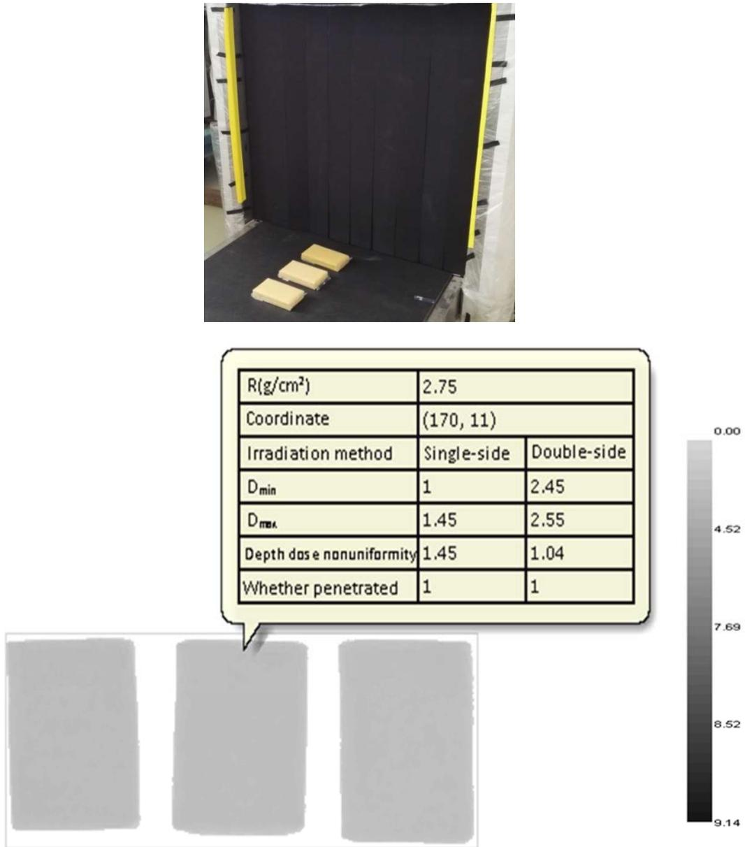
FIG. 11. Mass-thickness for millet of 3 cm (The darker the colour of the scanned image in the figure, the greater the mass thickness calculated) Using a density of  $0.92 \text{ g/cm}^3$  for the millet the mass thickness is  $3 \times 0.92 = 2.76 \text{ g/cm}^2$ .
