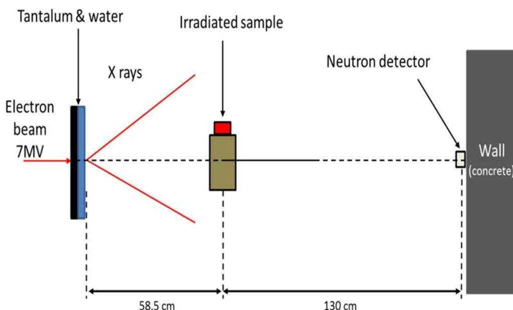
FIG. 5. Setup of the STERIS experiments.
