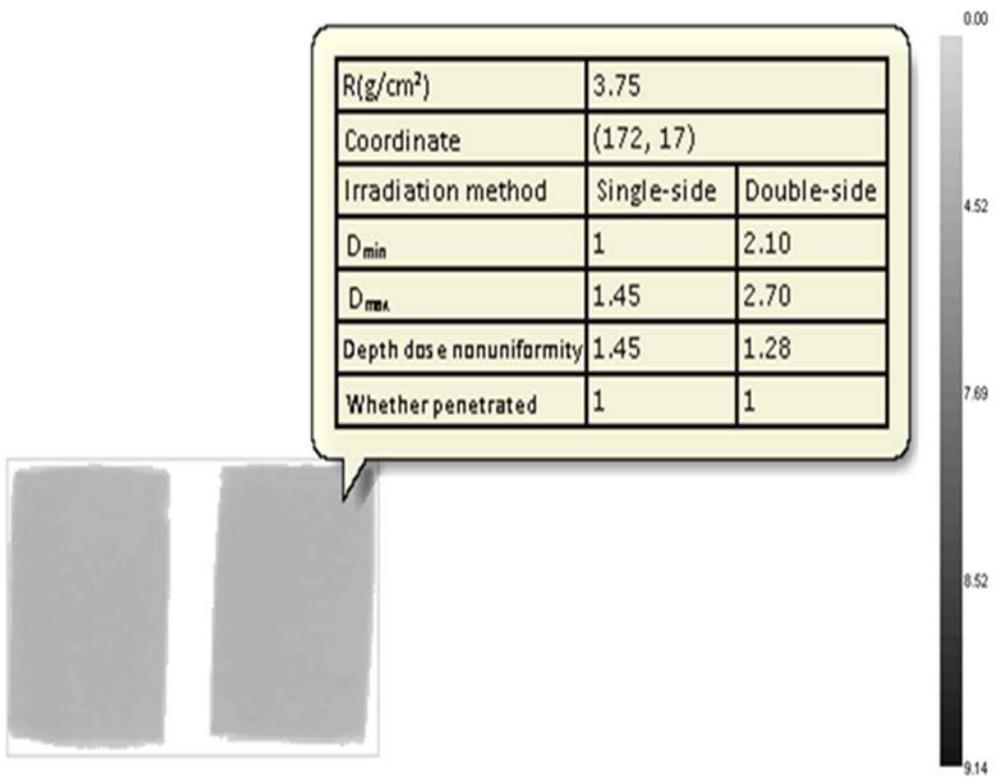
FIG. 12. Mass-thickness for millet of 4 cm depth.
