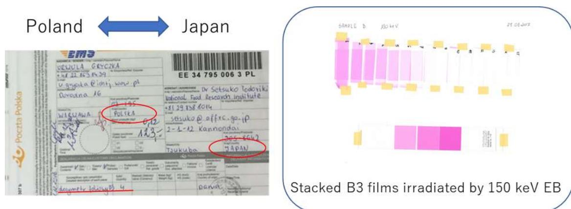
FIG. 8. Photo of the B3 films irradiated by 150-keV electron beam. The films shielded were shipped par avion (blank control film simultaneously shipped showed no colour development).
