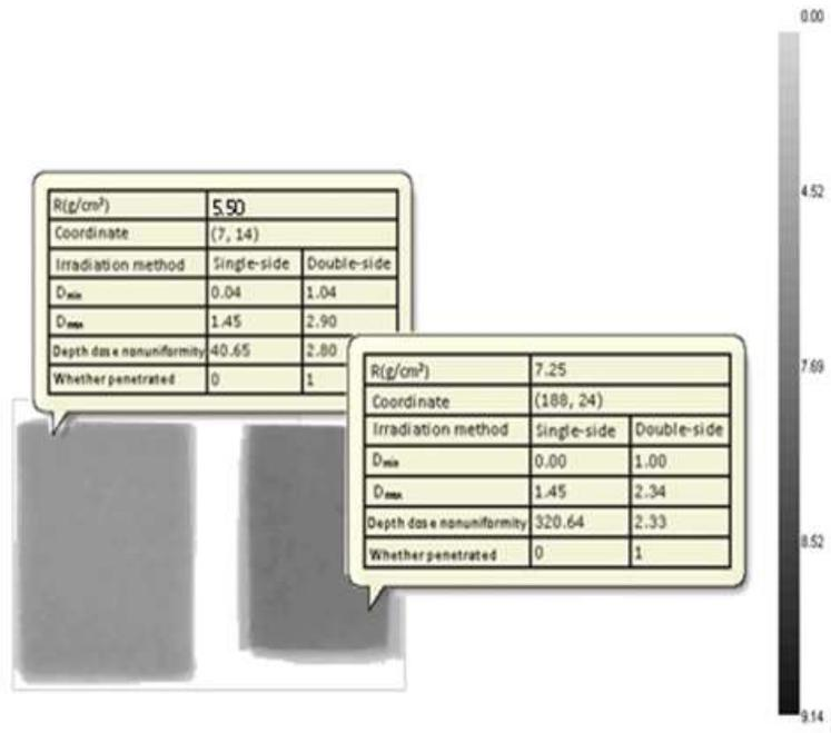
FIG. 13. Mass-thickness measurement of millet samples. On the left is a stack of two 3 cm depth samples with a total depth of 6 cm ( $6 \times 0.92 = 5.52 \text{ g/cm}^2$ ) and on the right is a stack of two 4 cm depth samples with a total depth of 8 cm ( $8 \times 0.92 = 7.36 \text{ g/cm}^2$ ).
