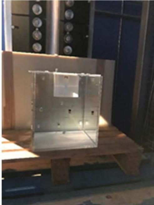
*FIG. 4. View of the 35 x 35 x 35 cm<sup>3</sup> water phantom and solid-state nuclear track detectors (SSNTD).*
