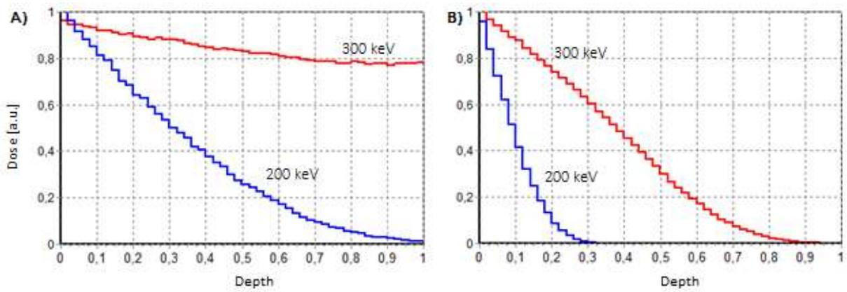
FIG. 7. Simulated depth dose distribution in A) bay leaves ( $x: l = 0,025\text{cm}$ ;  $y: l = 5\text{ kGy}$ ) and B) dried onion flakes ( $x: l = 0,038\text{ cm}$ ;  $y: l = 5\text{ kGy}$ ) irradiated with electrons having energy 300 keV and 200 keV.
