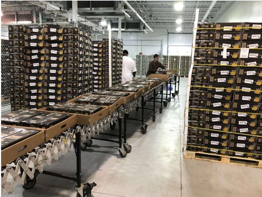
*FIG. 1. Photo showing the Mexican mangos arriving on pallets, then “de-palletized”, and single cases placed on carriers on the eBeam processing conveyor system.*
