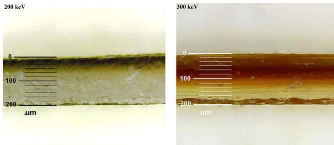
FIG. 3. Visualization of the irradiated layer thickness, observed as darkening in a photograph of the cross-section of PVC film that had been exposed to the electron beam.
