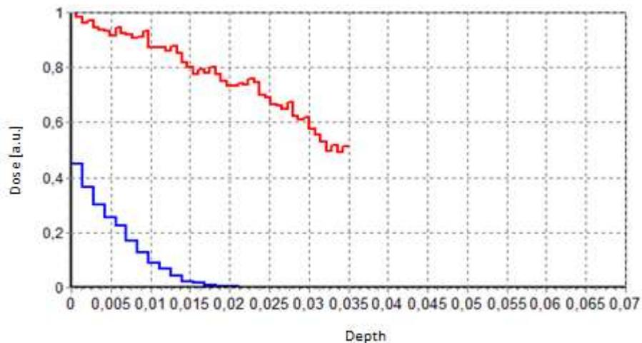
FIG. 8. Simulated depth dose distribution in surface layer of pepper and allspice grains irradiated with electrons having energy 300 keV (red line) and 200 keV (blue line) ( $x: \text{cm}$ ;  $y: l = 5\text{ kGy}$ ).
