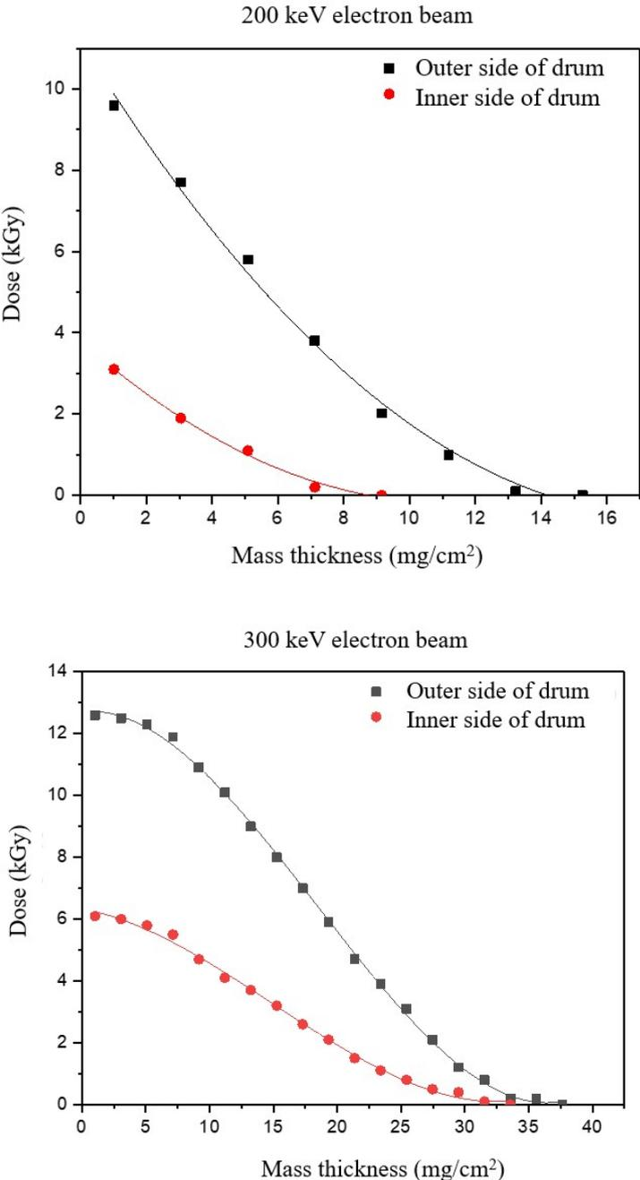
FIG. 4. Depth dose curves of 200 and 300 keV electron beam measured using B3 dosimetric foil.
