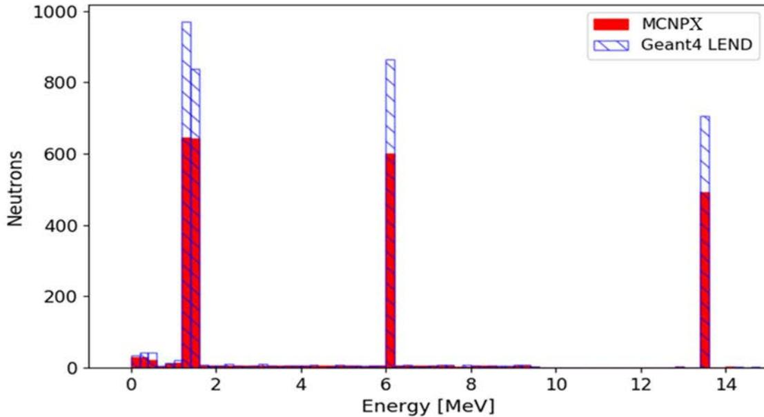
FIG. 2. Comparison of GEANT4 (LEND models) and MCNPX photoneutron spectrum corresponding to the irradiation of a  $^9\text{Be}$  cube ( $1\text{ mm}^3$ ) with 20 MeV photons.
