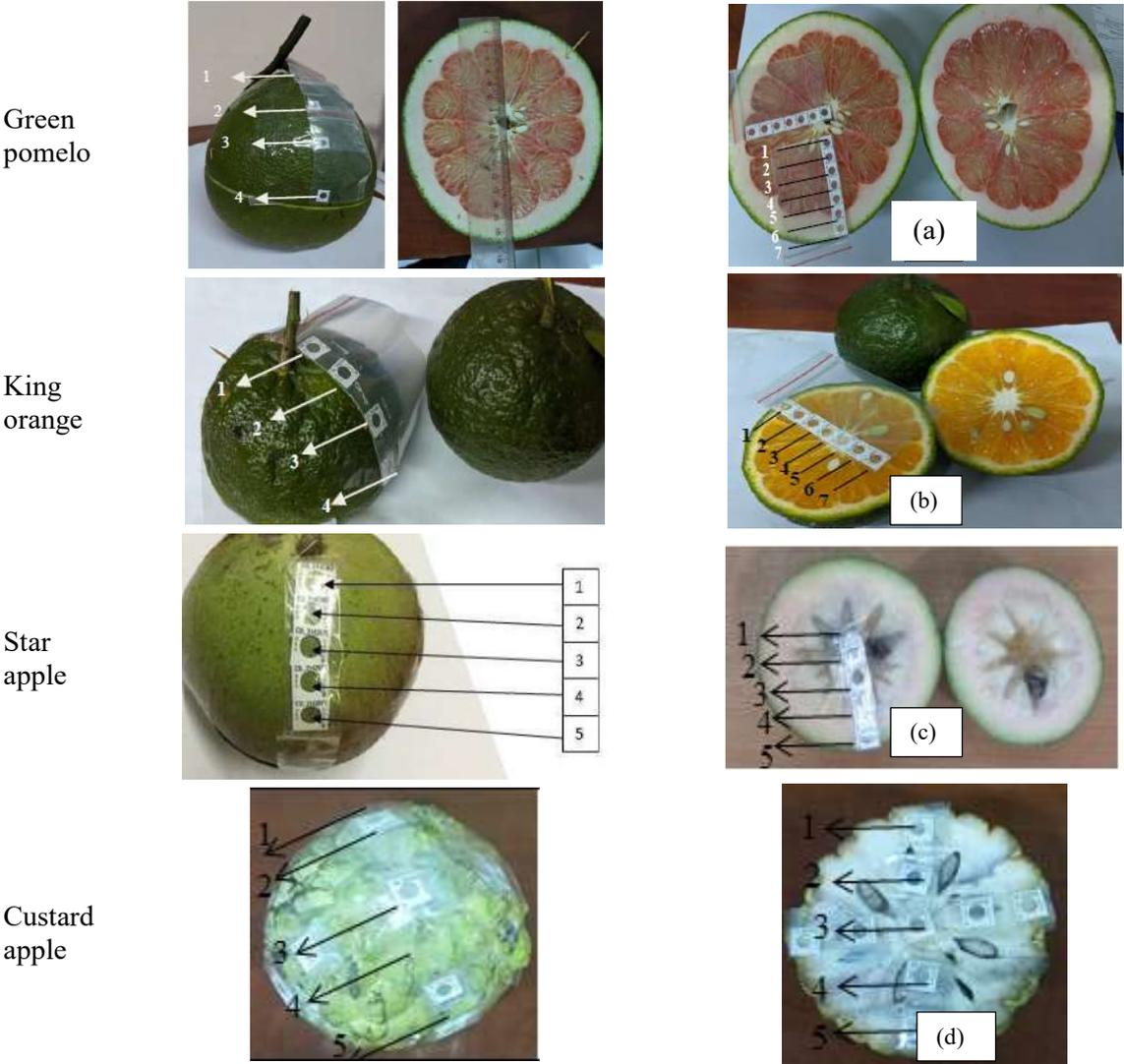
FIG. 13. Dose mapping of fruits for EB irradiation. Dosimeters were placed at locations on the outside, and inside of green pomelo (a), king orange (b); Lò Rèn star apple (c) and custard apple (d).
