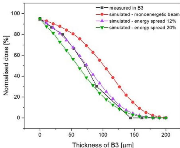
FIG. 2. Measured and simulated depth dose curves for 150 keV electron beam in B3 dosimetric foil.
