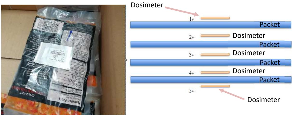
FIG. 20. Dosimeters deployment for frozen shrimps.
