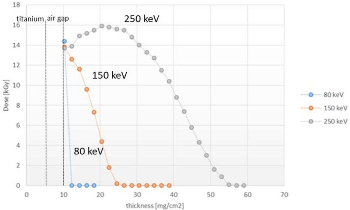
FIG. 9. Depth-dose profile in the stack of B3 films irradiated with low energy EB of energies 80, 150 and 250 keV.
