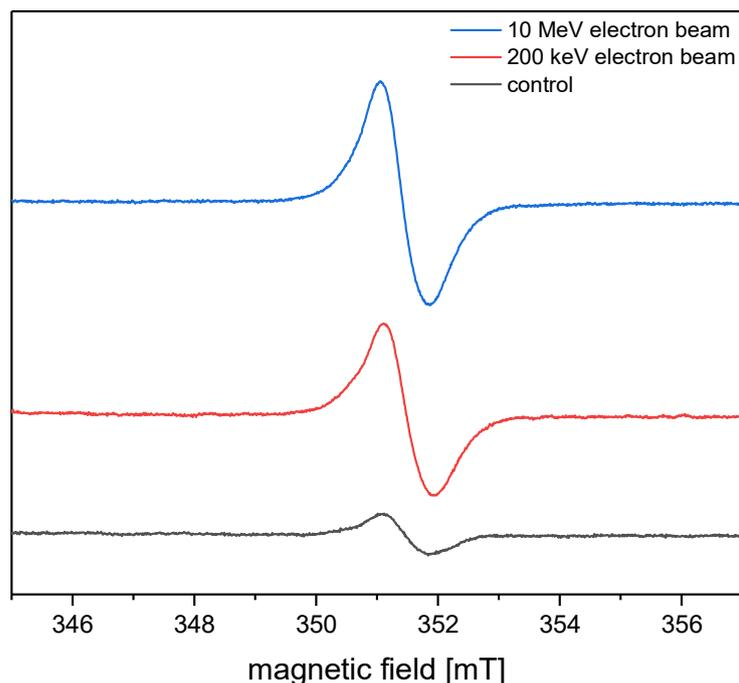
*FIG. 9. EPR spectra of bay leaves irradiated with low and high energy electron beam.*
