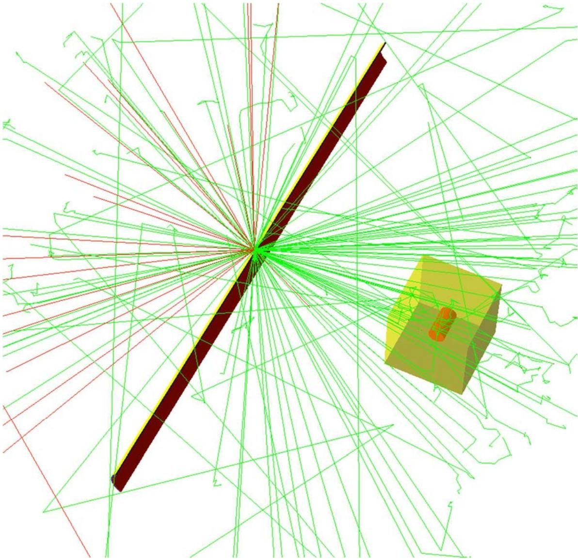
*FIG. 7. GEANT4 simulation for 7 MeV X ray irradiations of food sample inside a cardboard box.*
