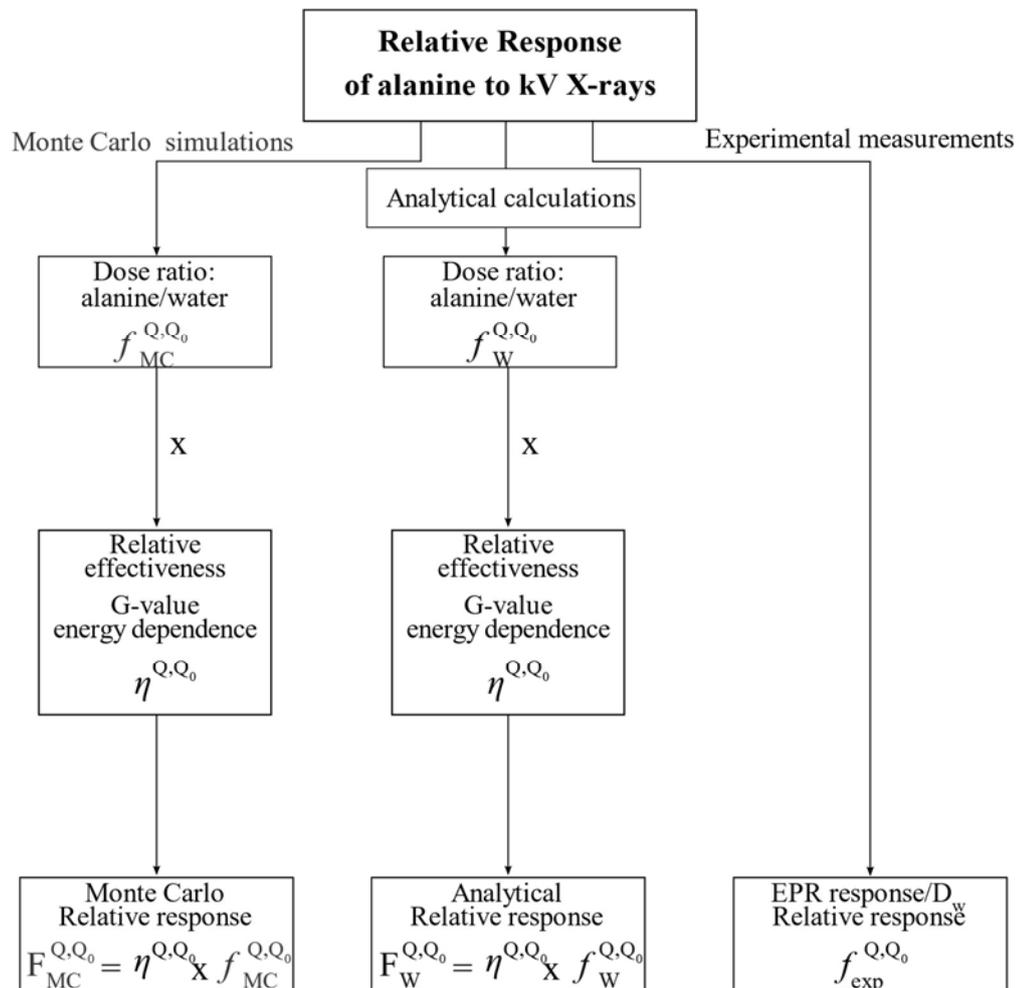
FIG. 1. Diagram of the three studied methods to determine the relative response of alanine to kv X rays.
