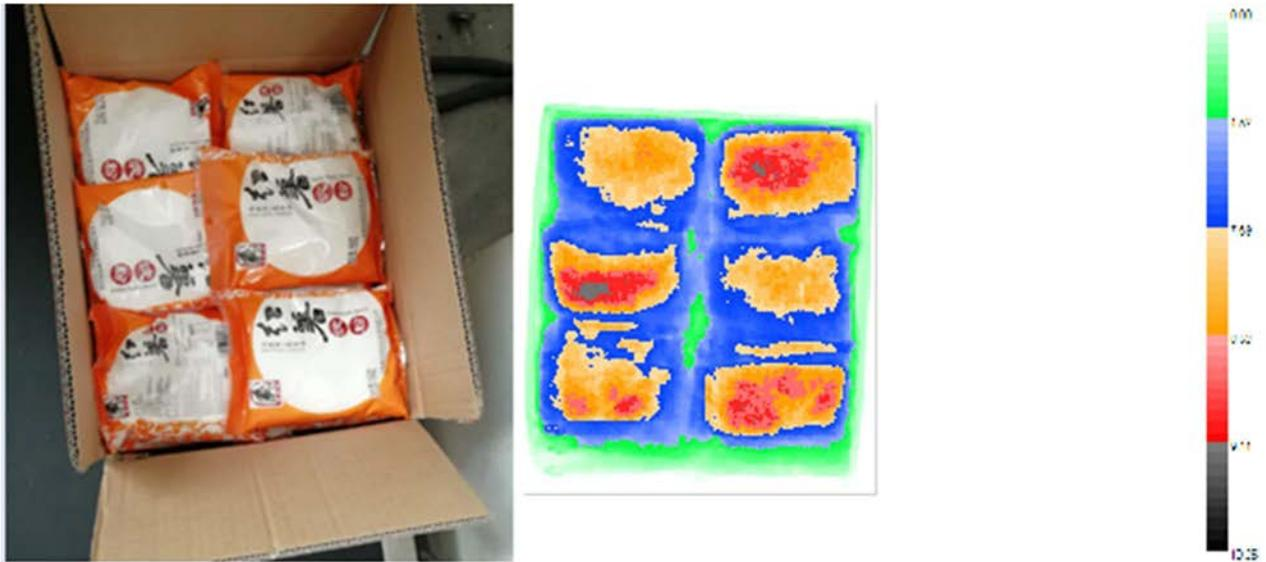
FIG. 22. Mass-thickness detection output image of potato starch.
