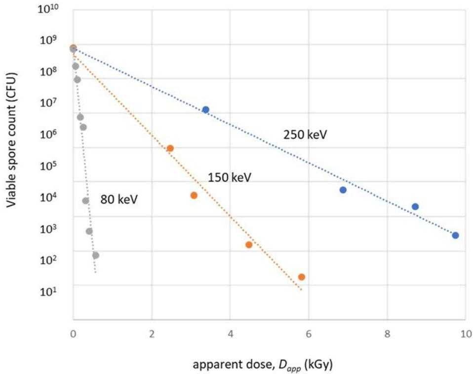
FIG. 6. The viable spore count and apparent dose ( $D_{app}$ ) measured by alanine dosimeter.
