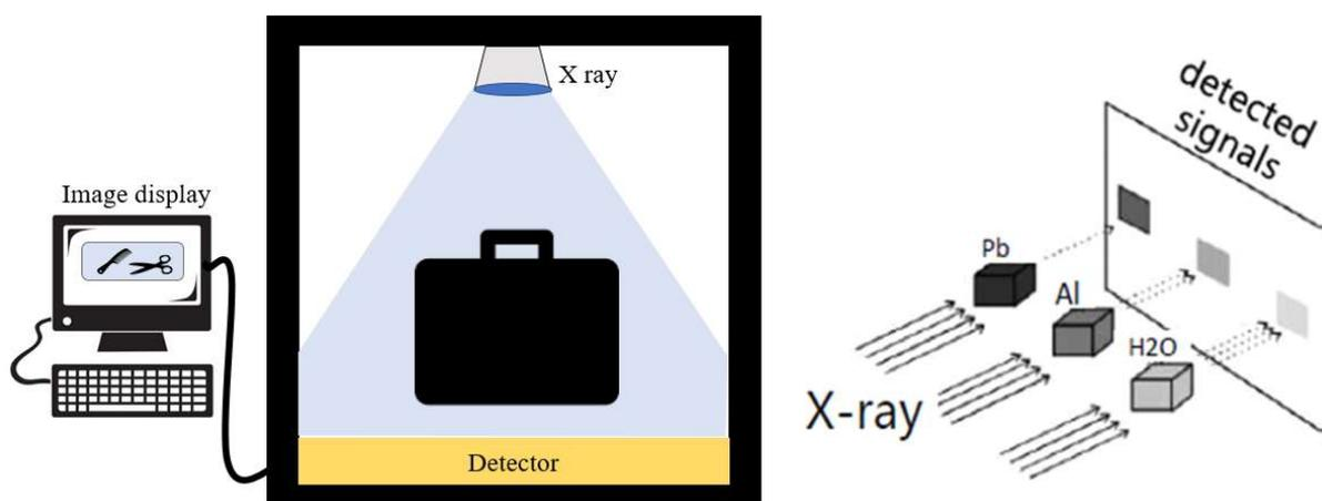
FIG. 1. X ray imaging technique.
