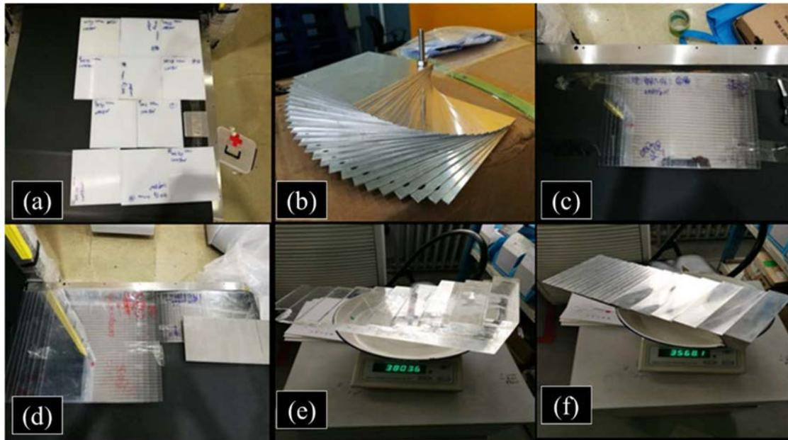
FIG. 2. Test materials (a) polyethylene sheet, (b) aluminium sheet, (c) polymethyl methacrylate (PMMA) sheet, (d) PMMA sheet, (e) step block of PMMA, (f) step block aluminium.
