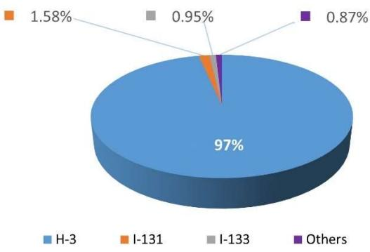
FIG. VI-2. Inhalation dose contribution per radionuclide, %. Atmospheric case A
