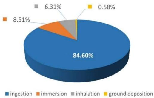
FIG. III-12. Total dose contribution per pathway, %, Atmospheric case B
