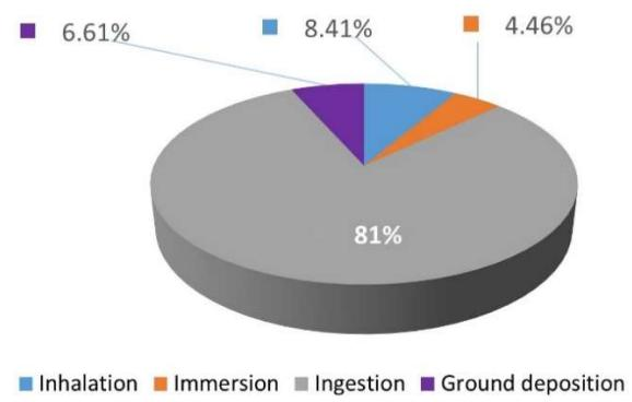
FIG. V-6. Total dose contribution per pathway, %, Atmospheric case A
