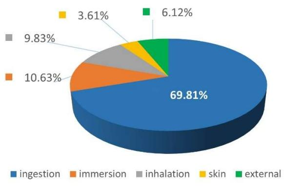
FIG. II-18. Total dose contribution per pathway, %, Atmospheric case C
