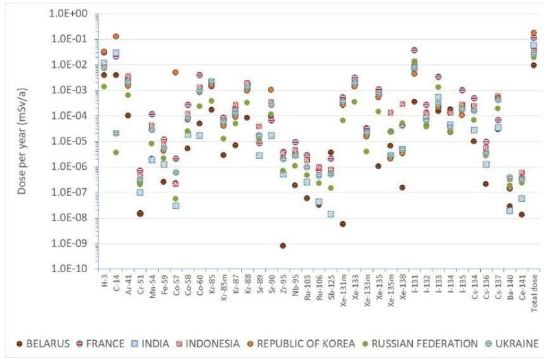
*FIG. 15. Summary of results showing dose for each nuclide and the total dose for each participant (logarithmic scale). Atmospheric case C*
