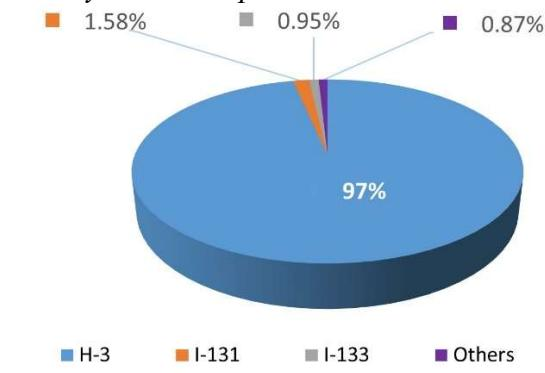
FIG. VI-8. Inhalation dose contribution per radionuclide, %. Atmospheric case B
