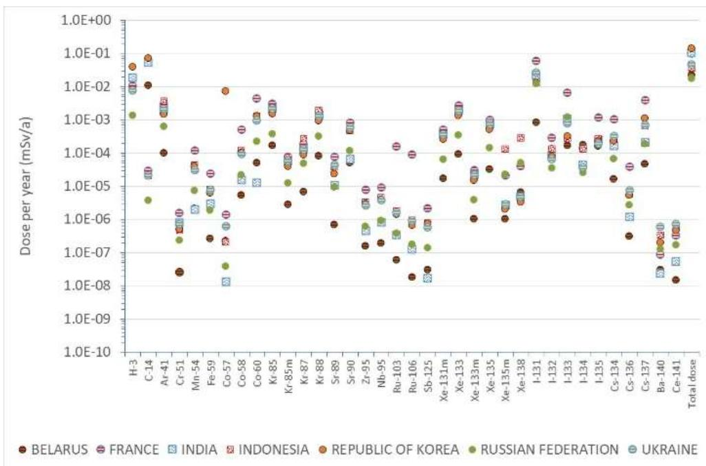
*FIG. 3. Summary of results showing dose for each nuclide and the total dose for each participant (logarithmic scale). Atmospheric case A*
