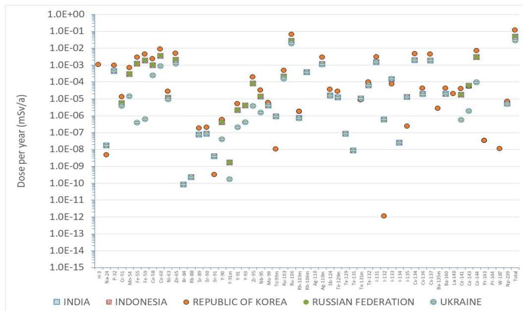
FIG. 46. Summary of results showing dose for each nuclide and the total dose. Marine case A
