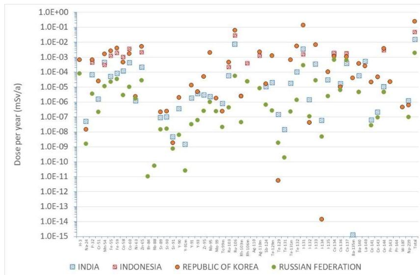
*FIG. 51. Summary of results showing dose for each nuclide and the total dose. Marine case B*
