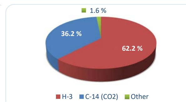
FIG. I-7. Inhalation dose contribution per radionuclide, %. Atmospheric case B
