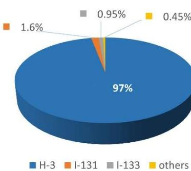
FIG. IV-8. Inhalation dose contribution per radionuclide, %. Atmospheric case B
