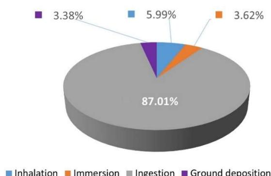
FIG. V-18. Total dose contribution per pathway, %, Atmospheric case C
