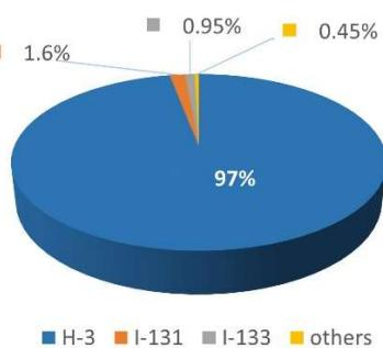
FIG. IV-14. Inhalation dose contribution per radionuclide, %, Atmospheric case C
