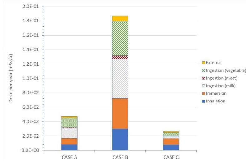
*FIG. 24. Comparison of the results for each case showing the breakdown by pathway. Ukraine*
