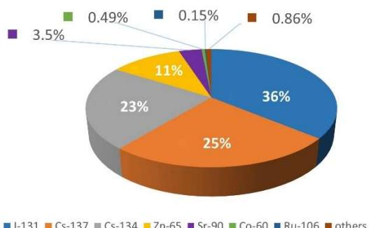
FIG. IV-21. Ingestion dose contribution per radionuclide, %, Riverine case B
