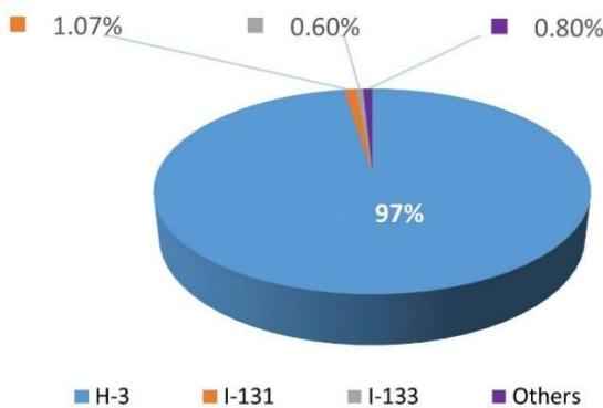
FIG. V-8. Inhalation dose contribution per radionuclide, %. Atmospheric case B
