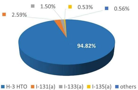
FIG. II-8. Inhalation dose contribution per radionuclide, %. Atmospheric case B.
