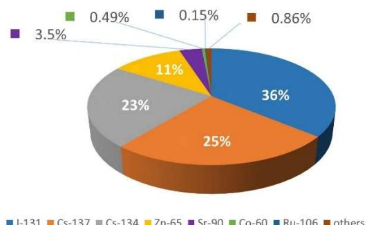
FIG. IV-20. Ingestion dose contribution per radionuclide, %, Riverine case A
