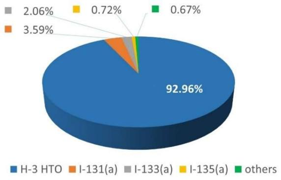
FIG. II-2. Inhalation dose contribution per radionuclide, %. Atmospheric case A
