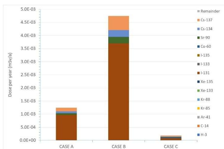
FIG. 44. Comparison of the results for each case showing the breakdown by nuclide (meat ingestion – Ukraine)
