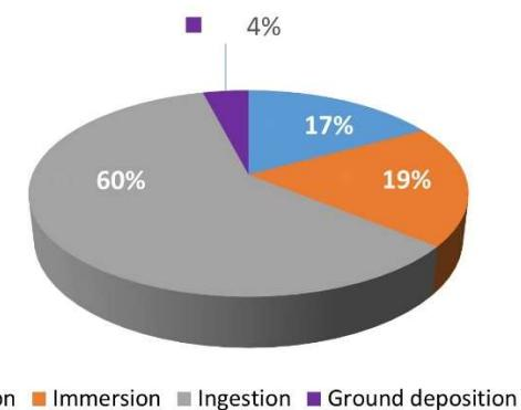
FIG. VII-6. Total dose contribution per pathway, %. Atmospheric case A
