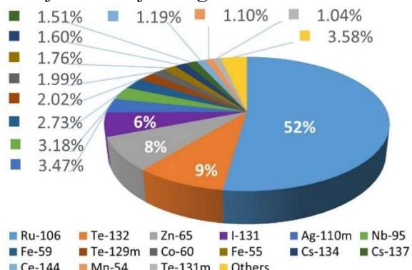
FIG. V-23. Contribution of radionuclides to the total dose from ingestion excluding algae. Marine case B
