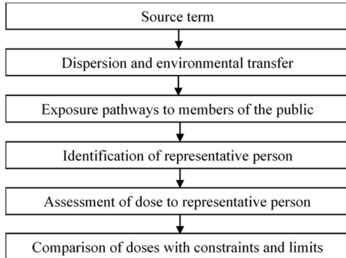
*FIG. 1. Basic stages of assessment of radiological impact from a nuclear energy system (adapted from [2]).*
