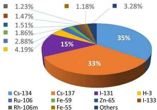
FIG. VI-22. Contribution of radionuclides to the total dose. Marine case B
