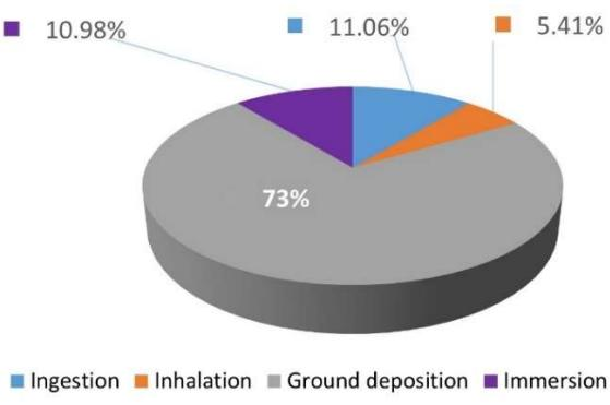
FIG. V-12. Total dose contribution per pathway, %, Atmospheric case B
