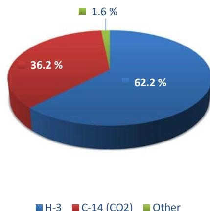
FIG. I-12. Inhalation dose contribution per radionuclide, %. Atmospheric case C
