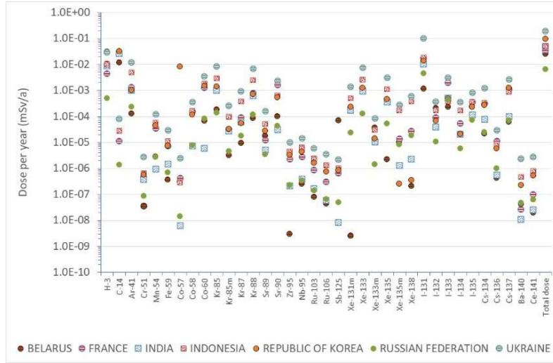
*FIG. 12. Summary of results showing dose for each nuclide and the total dose for each participant (logarithmic scale). Atmospheric case B*
