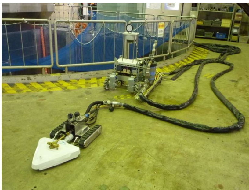
FIG. 10. Decontamination robot used in Unit 2 of the Fukushima Daiichi NPS (courtesy of TEPCO).
