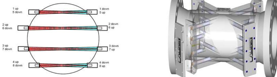
FIG. 105. Multipath transit-time UFM pipe section (courtesy of Caldon. Inc)
