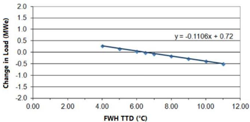
FIG. 39. Resulting curve of relationship between load and feedwater heater
