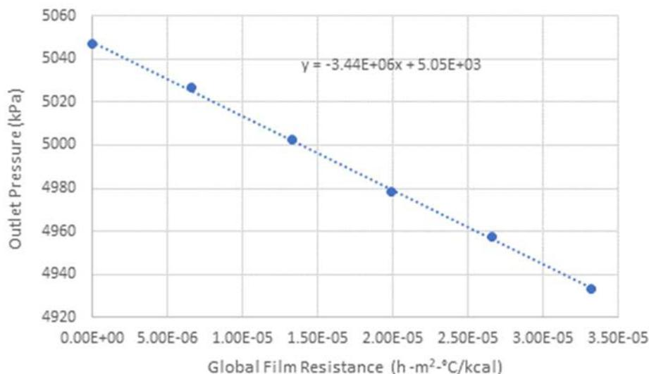
FIG. 112. Effect of fouling on SG pressure
