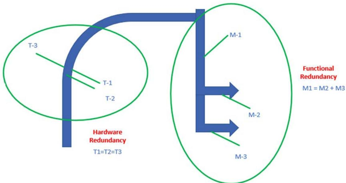
FIG. 28. Two types of measurement redundancies
