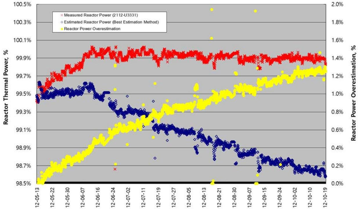
FIG. 73. Trending of the RTP measurement drift
