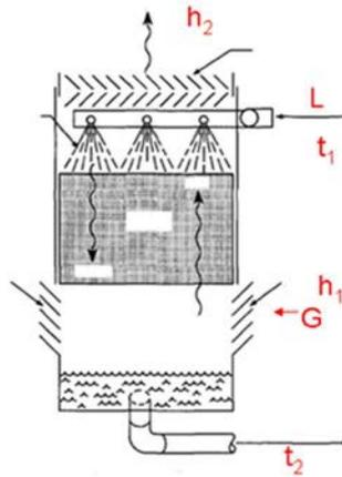
FIG. 87. Cooling tower energy exchange
