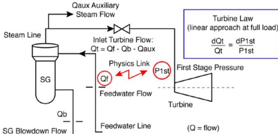
FIG. 53. EDF's  $\Delta P/P$  method for the RTP measurement drift monitoring [25]
