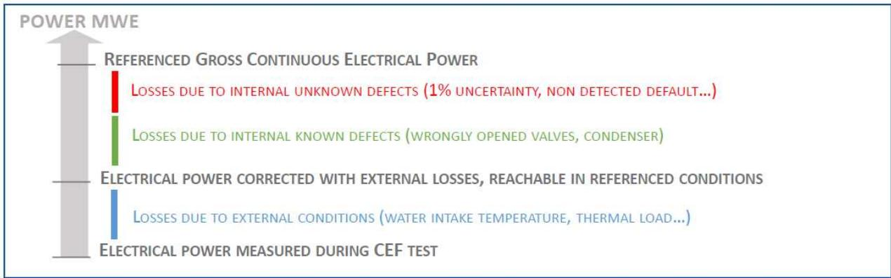
FIG. 34. Losses identification
