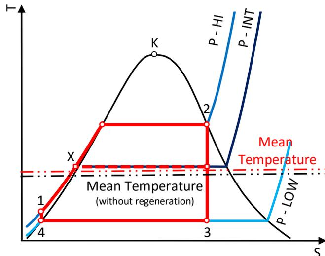
FIG. 82. Ideal regenerative Rankine cycle with closed feedwater heater
