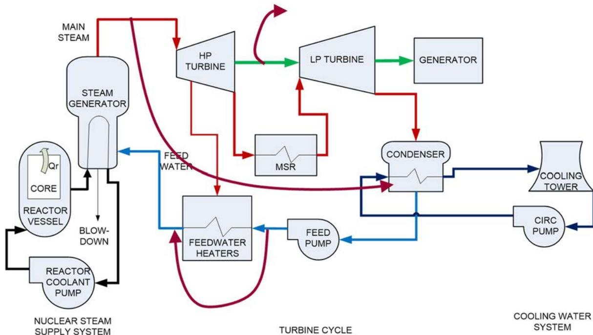
FIG. 16. Cycle isolation leakages for PWR schema [1]
