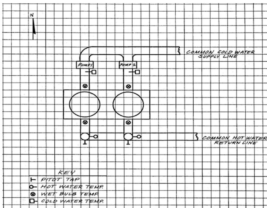
FIG. 90. Performance test measurement locations
