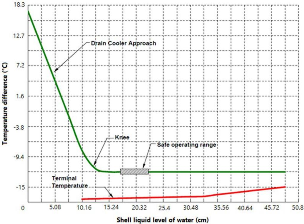
FIG. 128. Typical DCA and TTD vs. internal liquid level (courtesy ASME PTC 12.1 [4])
