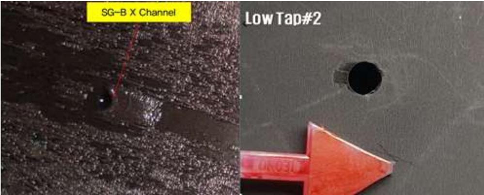
FIG. 102. Case of deposit (left) and erosion (right) on low pressure tap
