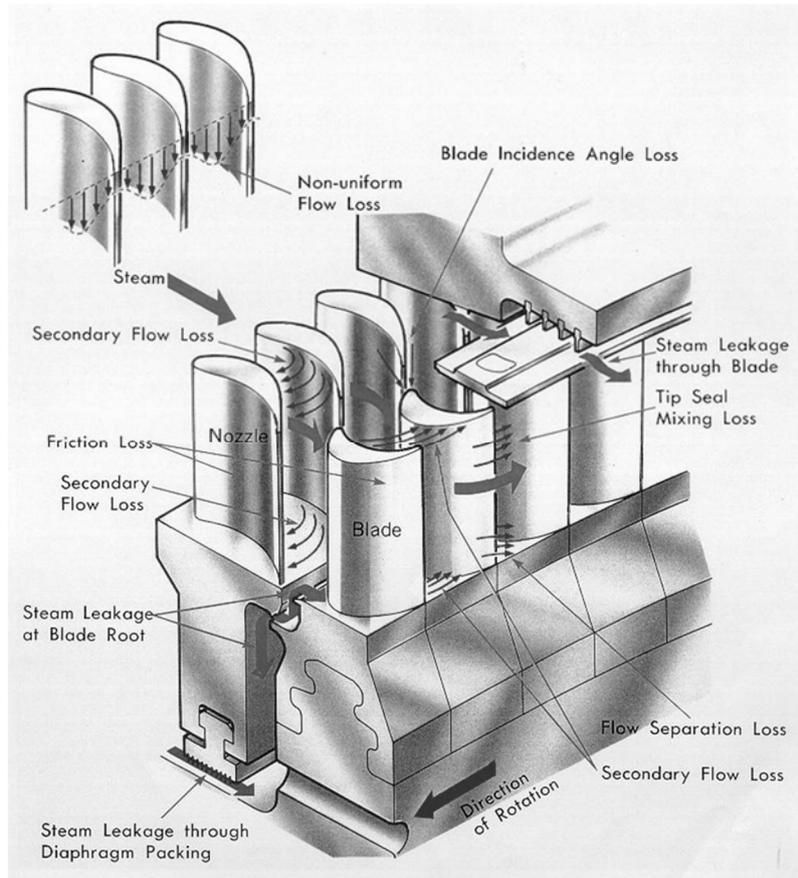
FIG. 139. Turbine stage performance losses (impulse turbine)
