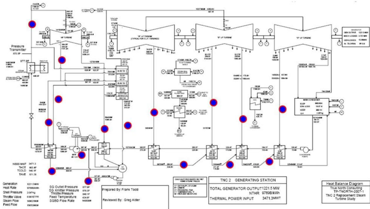
FIG. 17. Cycle isolation leakage valve detection
