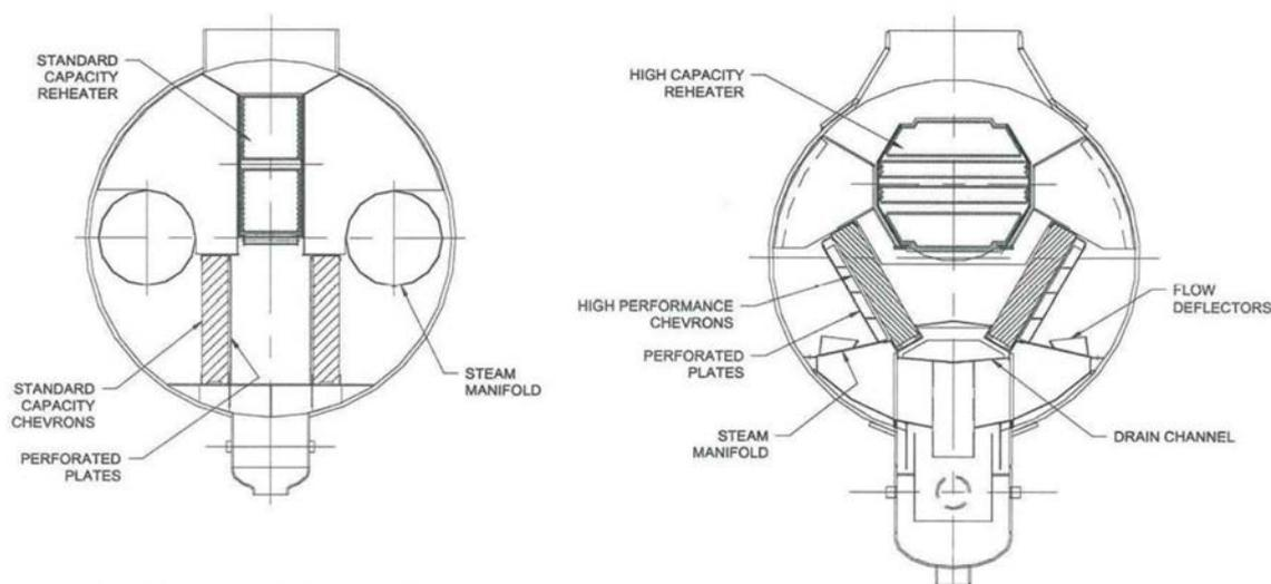
FIG. 141. Old (left) and new (right) MSR designs
