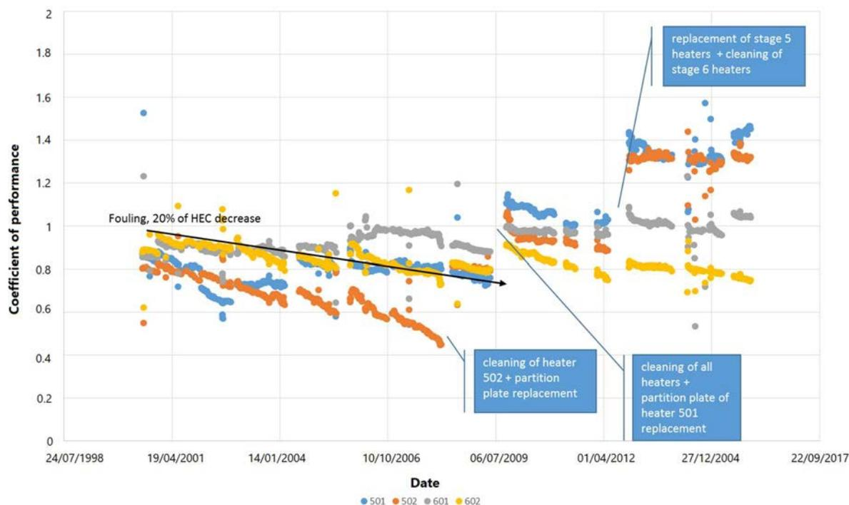
FIG. 133. Fouling factor for HP heaters
