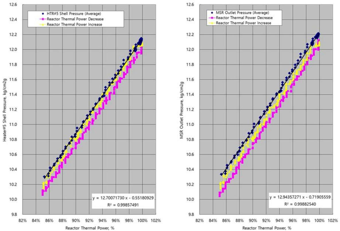
FIG. 60. RTP vs HTR#5 shell pressure(left); RTP vs MSR outlet pressure(right)
