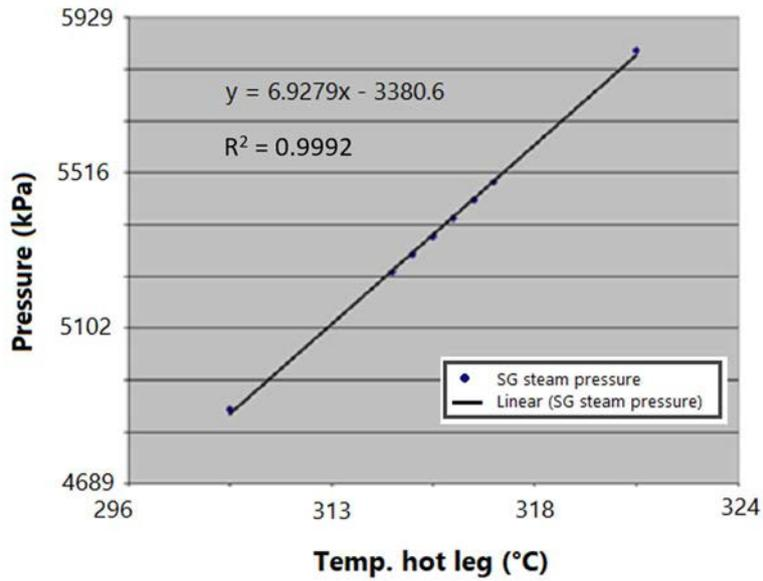
FIG. 116. SG outlet steam pressure vs primary hot leg temperature
