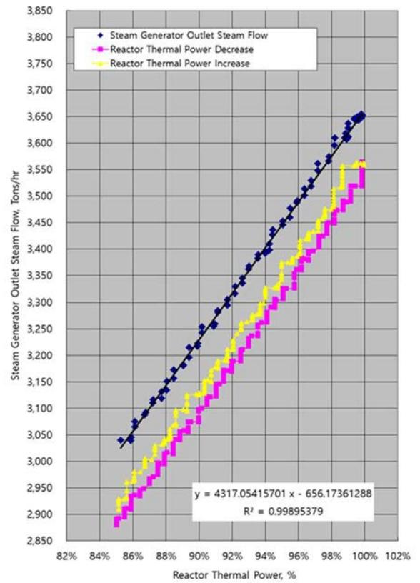
FIG. 57. RTP vs final feedwater flow(left); RTP vs SG outlet steam flow (right)
