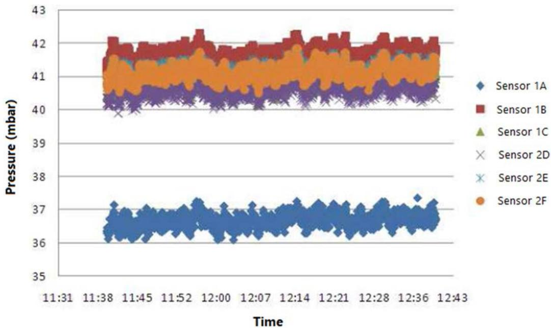
FIG. 13. Example of cross comparison between condenser vacuum sensors
