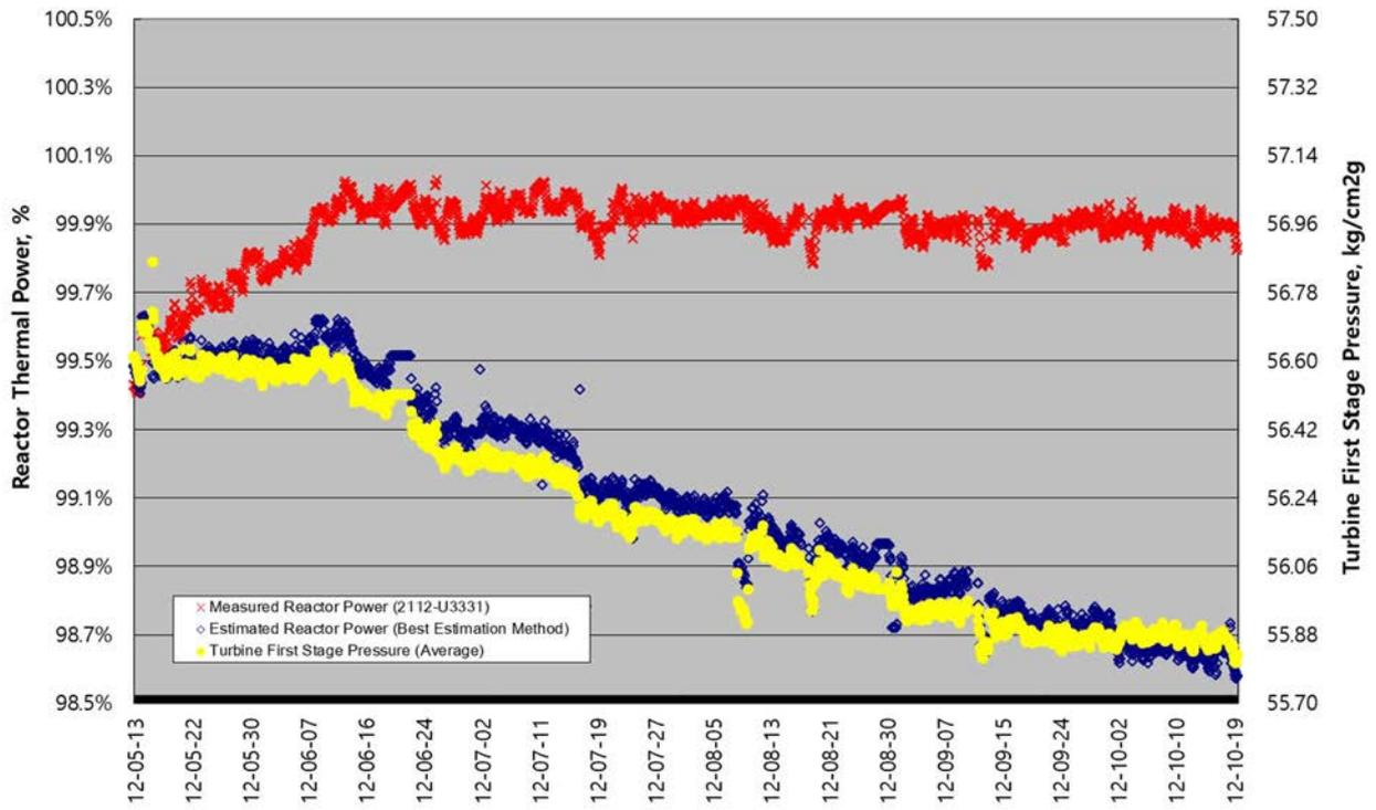
FIG. 67. Trending of RTP vs HP turbine 1st stage pressure
