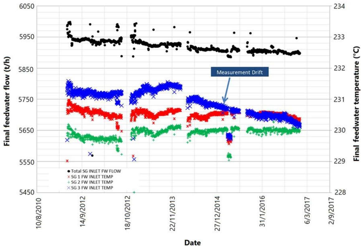
FIG. 108. Monitoring of final feedwater measurement drift
