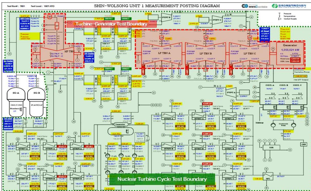
FIG. 84. Turbine cycle and turbine-generator control (or test) boundary
