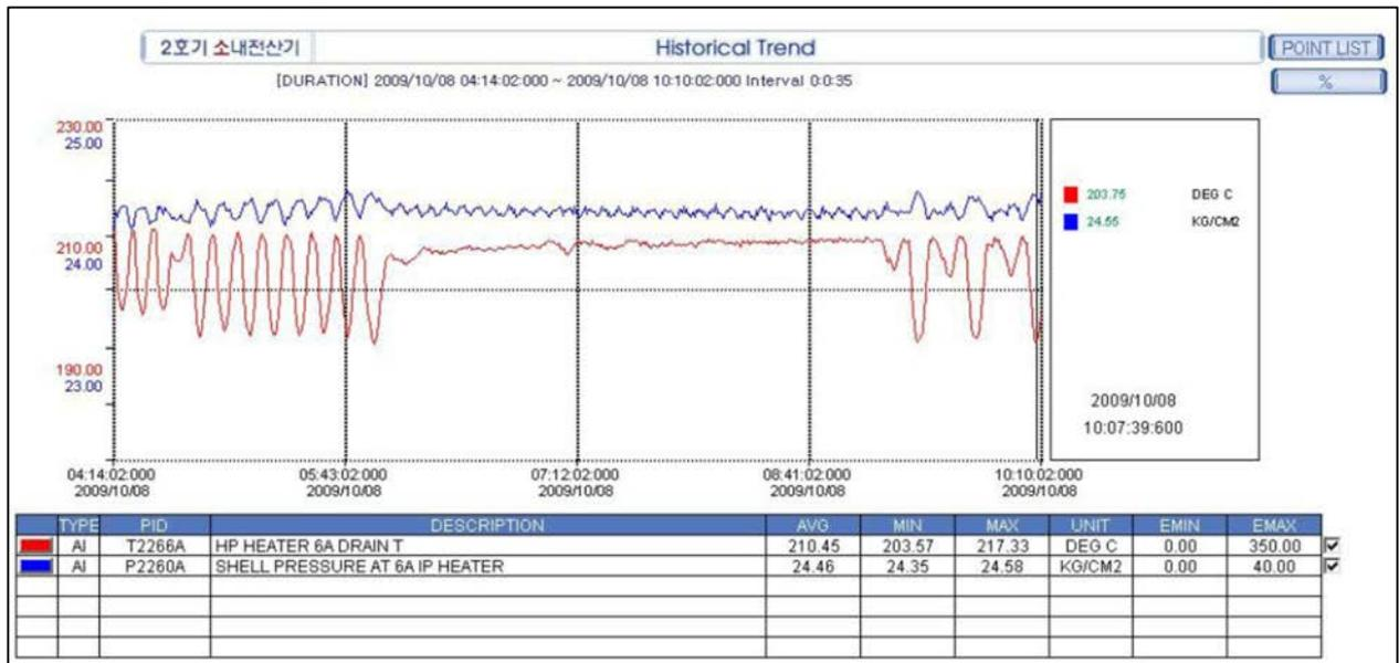
FIG. 130. Oscillation of heater drain temperature
