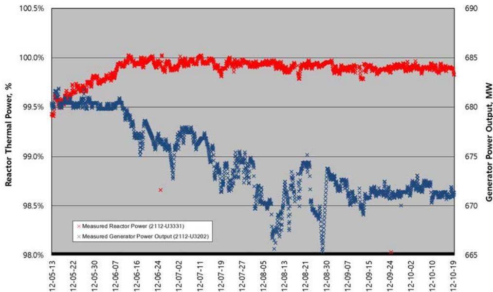
FIG. 56. RTP vs Generator Power Output
