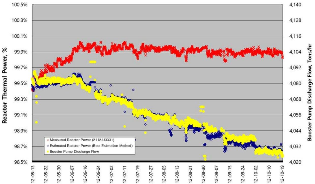
FIG. 66. Trending of booster feed pump discharge flow
