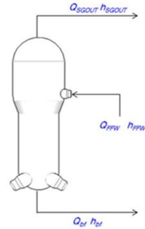
FIG. 100. Calculation of SG thermal power (PWR)
