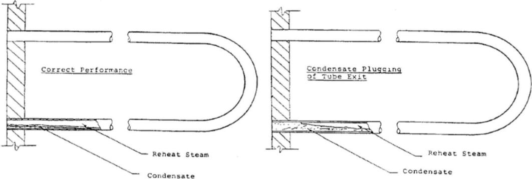
FIG. 134. Reheater tube inside condensation (two pass type reheater)
