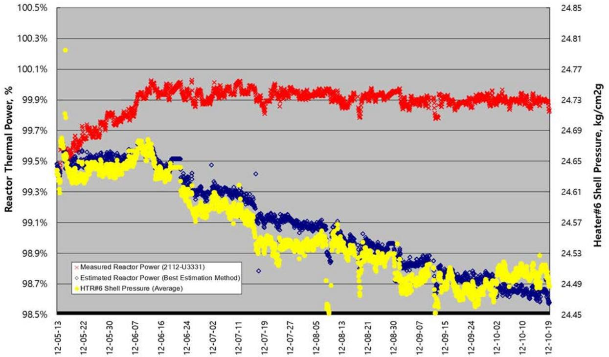
FIG. 68. Trending of RTP vs feedwater heater 6 shell pressure
