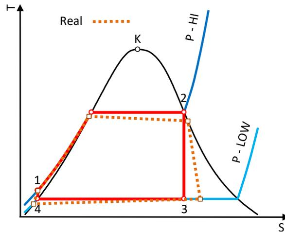
FIG. 78. Real Rankine cycle
