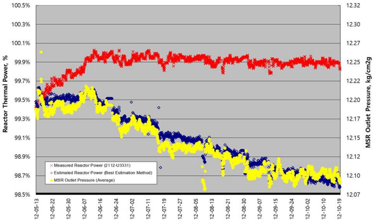
FIG. 70. Trending of RTP vs MSR outlet steam pressure
