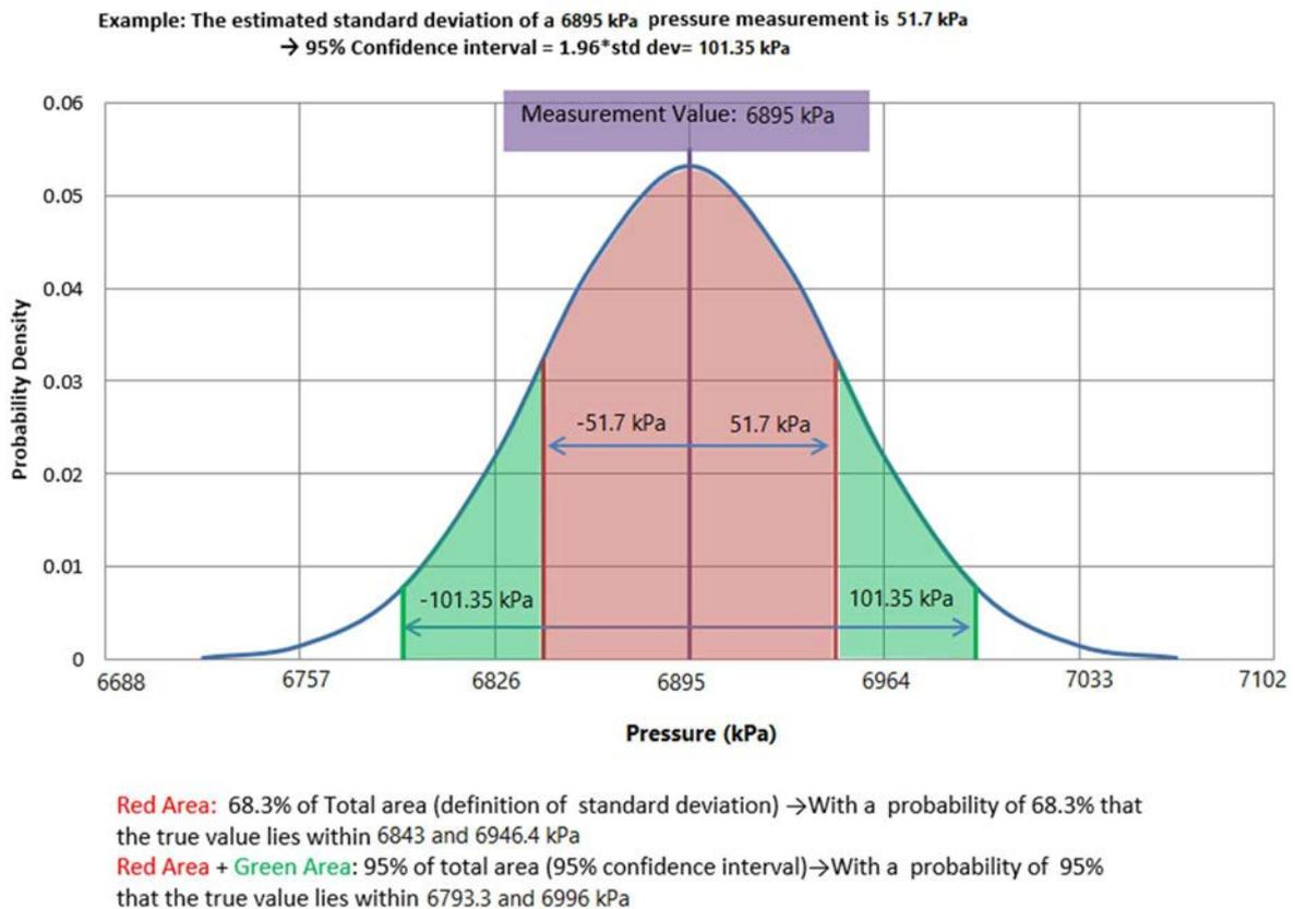
FIG. 29. The relationship between the standard deviation  $\sigma$  and the 95% confidence level of the plant measured values
