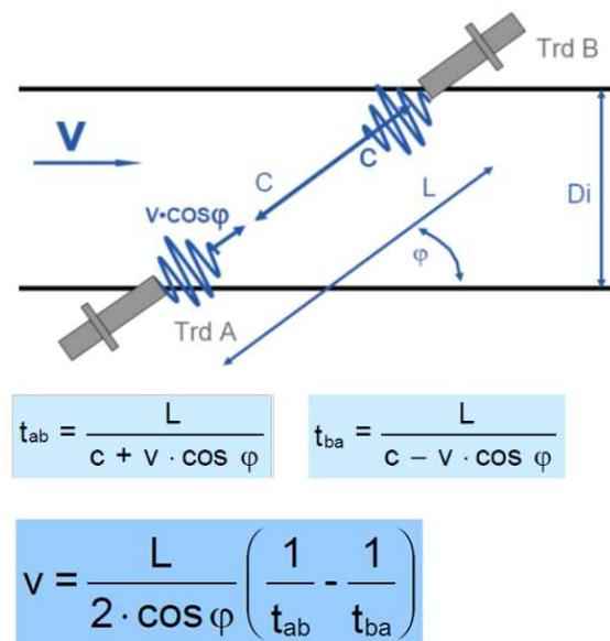
FIG. 104. Flow measuring principal of the transit-time UFM
