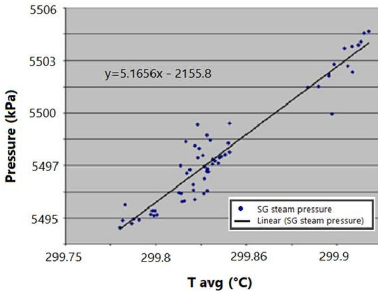
FIG. 117.  $T_{avg}$  vs SG outlet steam pressure
