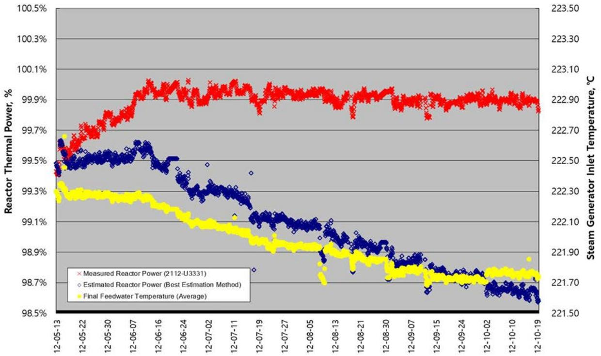
FIG. 71. Trending of RTP vs final feedwater temperature
