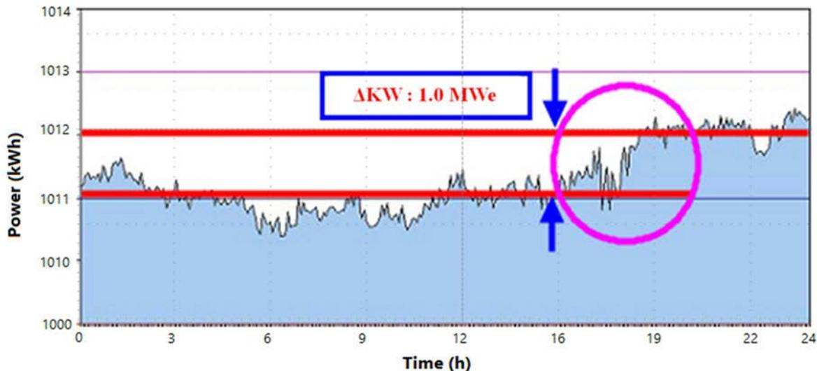
FIG. 136. Change of kW output from excessive heating steam optimization
