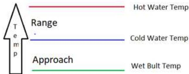
FIG. 89. Approach and range temperatures
