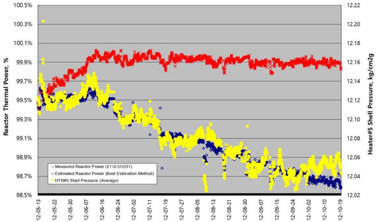
FIG. 69. Trending of RTP vs feedwater heater 5 shell pressure
