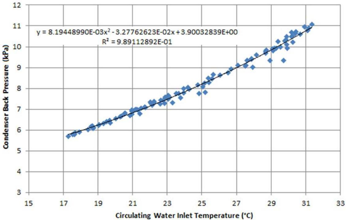
FIG. 51. Expected condenser pressure curve for condenser cooling water inlet temperature
