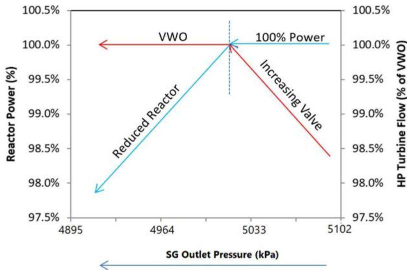
FIG. 119. Limitation of RTP due to SG pressure reductions
