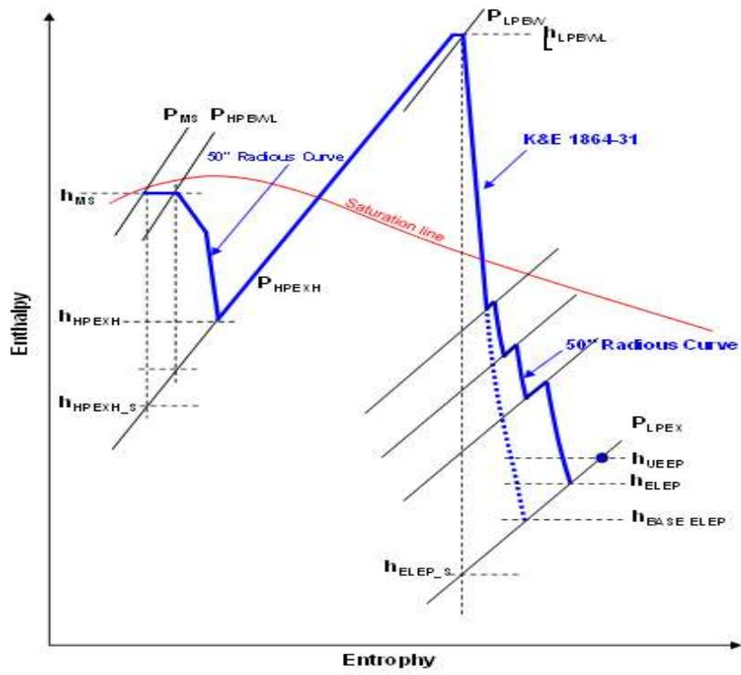
FIG. 25. Typical HP-LP turbine steam expansion line
