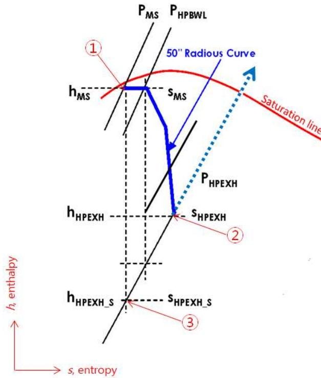
FIG. 85. HP turbine expansion line
