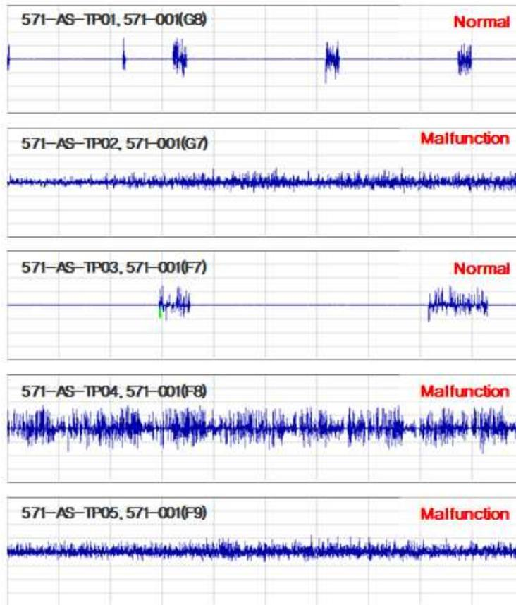
FIG. 111. Check for steam trap malfunctioning
