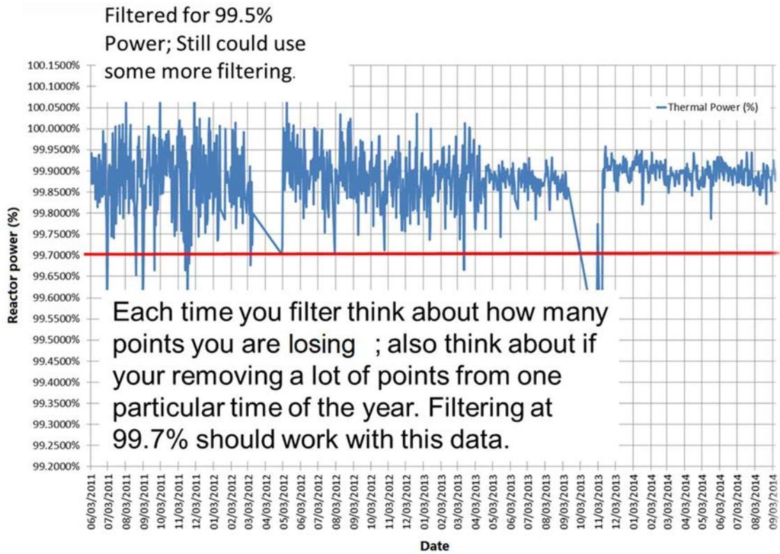
FIG. 47. Filtered data for power vs time
