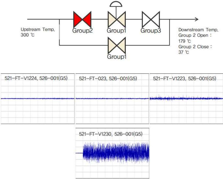
FIG. 110. Check for valve leakage at drain valve train
