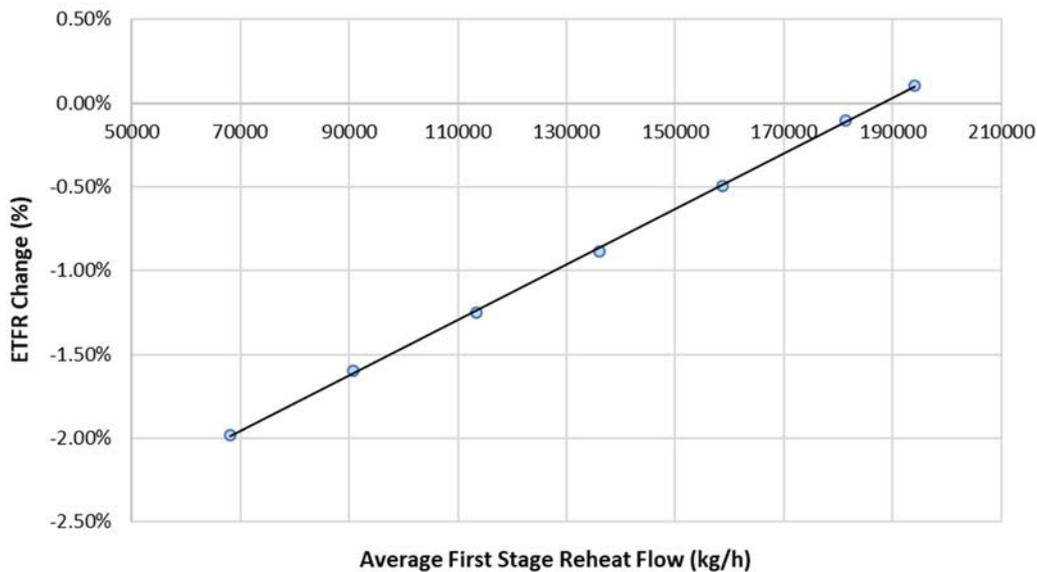
FIG. 125. First stage reheater flow vs ETFR
