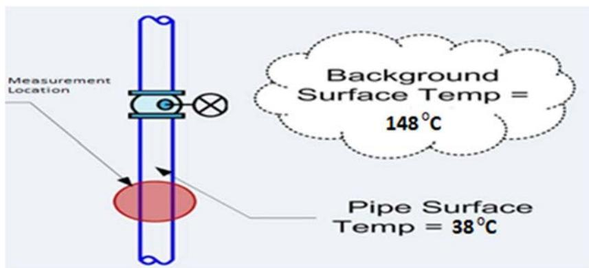
FIG. 19. IR thermometer false reading condition [1]
