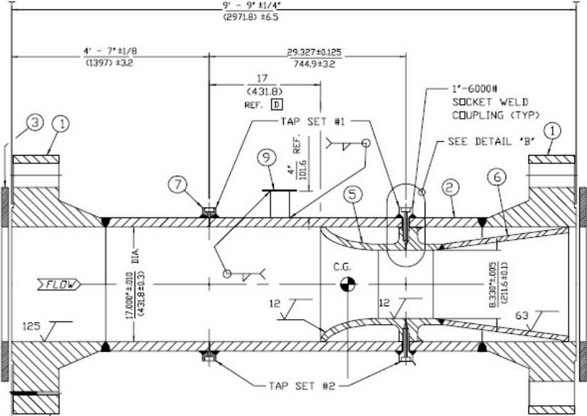
FIG. 101. Cross-section of typical ASME PTC 6 [3] throat tap nozzle for nuclear application
