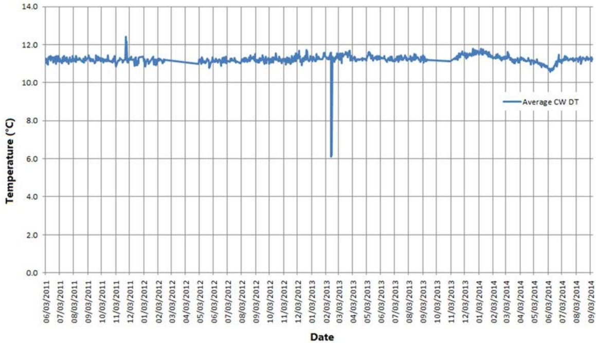
FIG. 49. Average circulating water temperature
