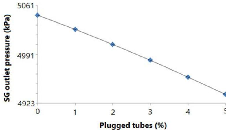
FIG. 115. Effect of SG tube plugging on SG outlet pressure
