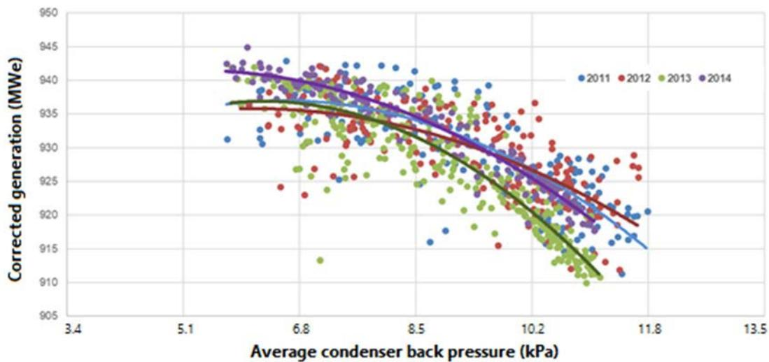
FIG. 46. Condenser back pressure vs gross generation
