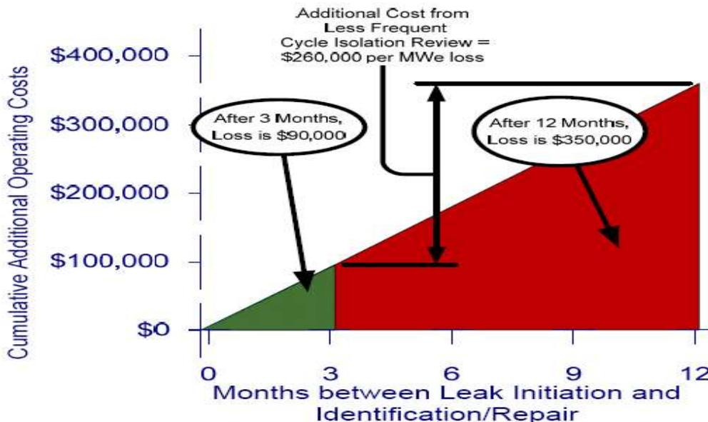
FIG. 15. Cycle isolation losses [1]
