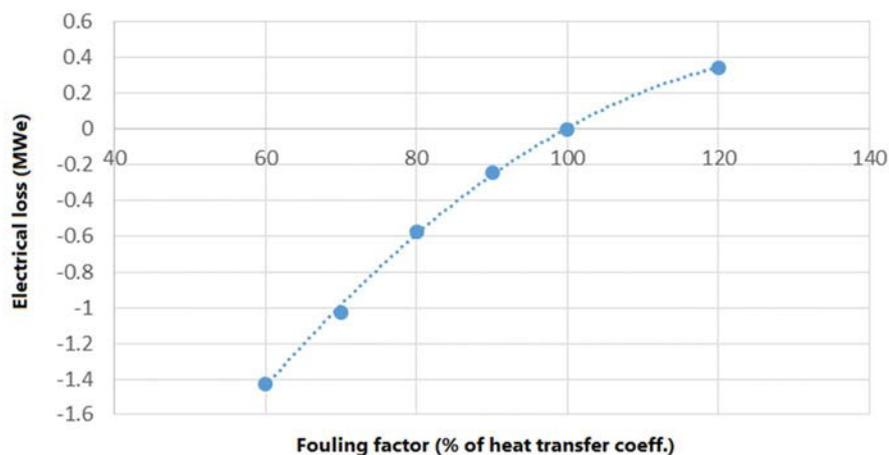
*FIG. 132. Electrical losses vs fouling factor curve*
