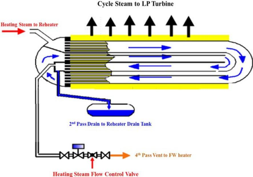
FIG. 135. Four pass type reheater
