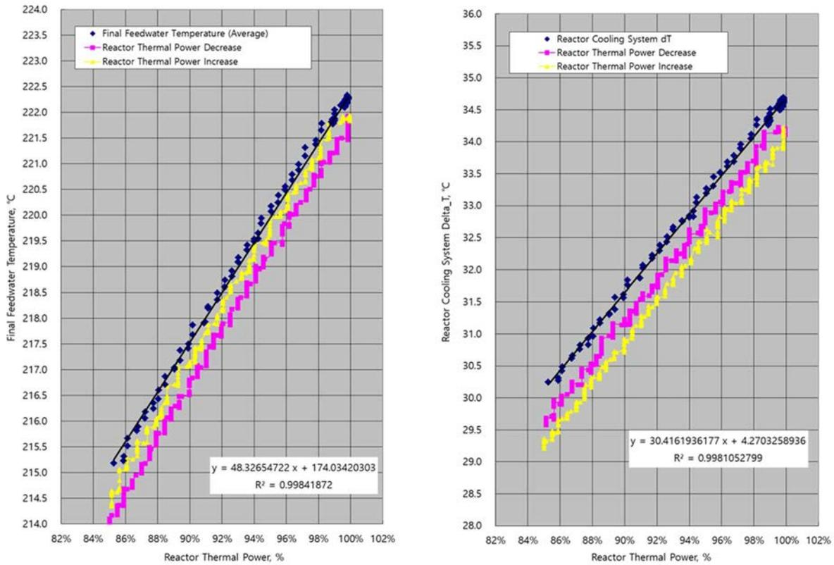
FIG. 61. RTP vs final feedwater temperature (left); RTP vs RCS  $\Delta T$  (right)
