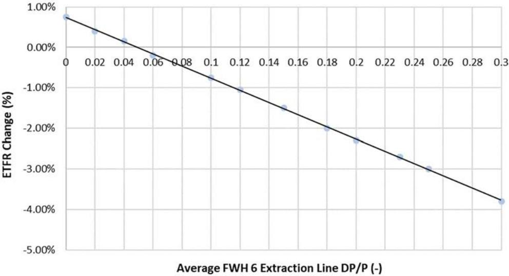
FIG. 126. Throttle extraction steam vs ETFR
