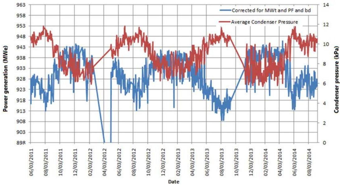
FIG. 44. Power corrected generation
