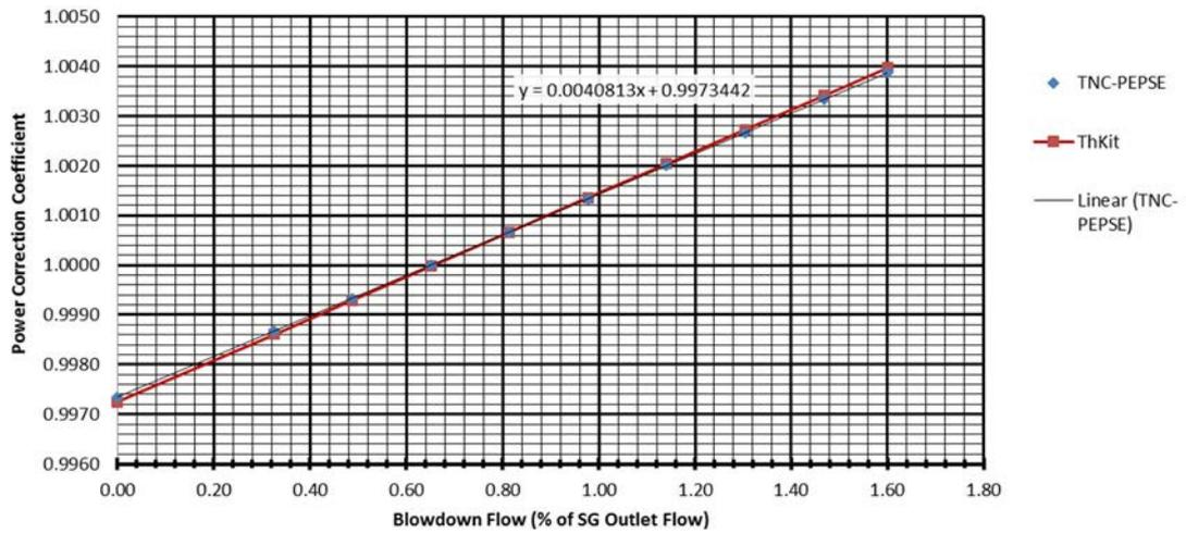
FIG. 42. Resulting curve of relationship between power correction and blowdown flow
