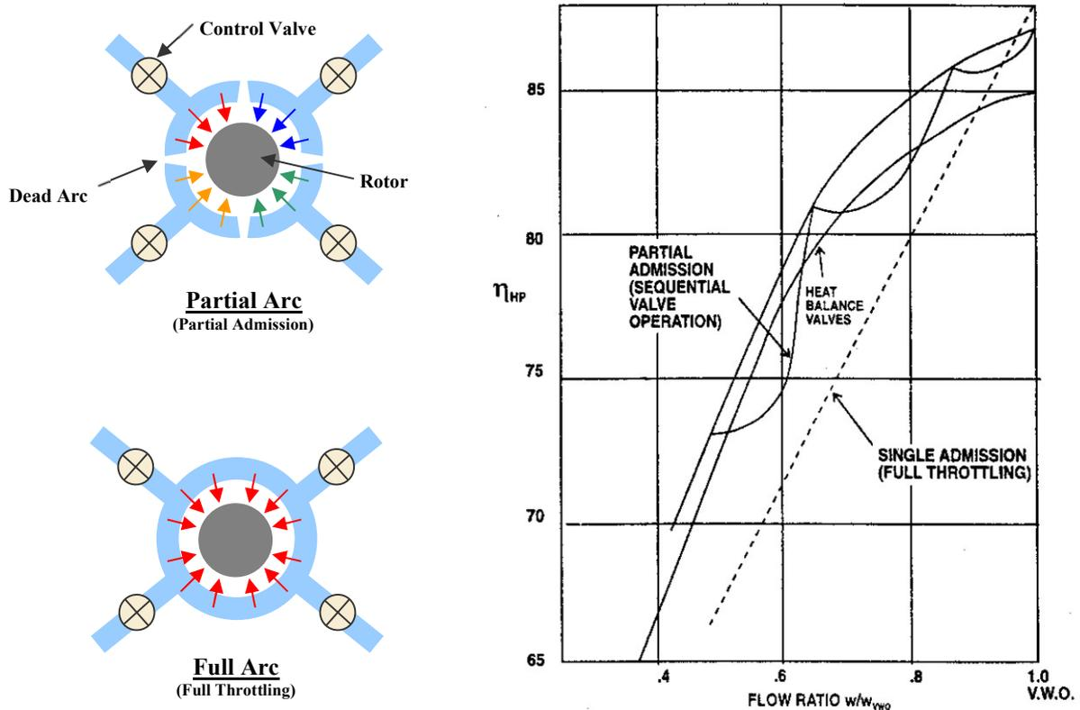
FIG. 140 HP Turbine Efficiency Characteristic – Full Arc vs. Partial Arc
