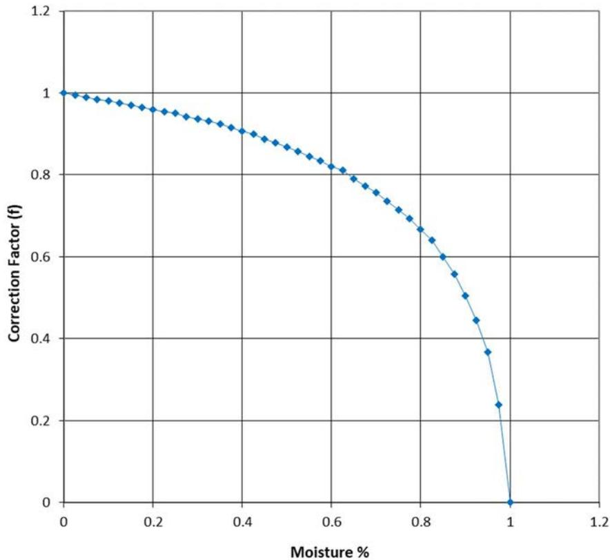
FIG. 23. Curve for correcting the calculated flow [1]
