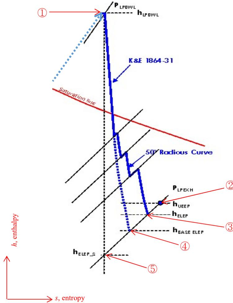
FIG. 86. LP turbine expansion line
