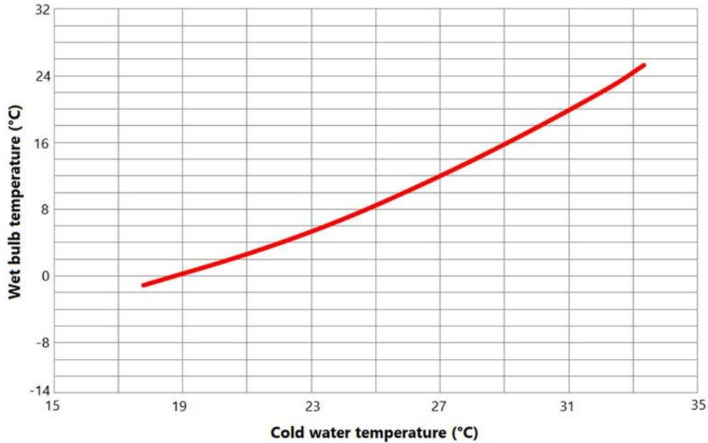
FIG. 88. Wet-bulb temperature vs cold water temperature
