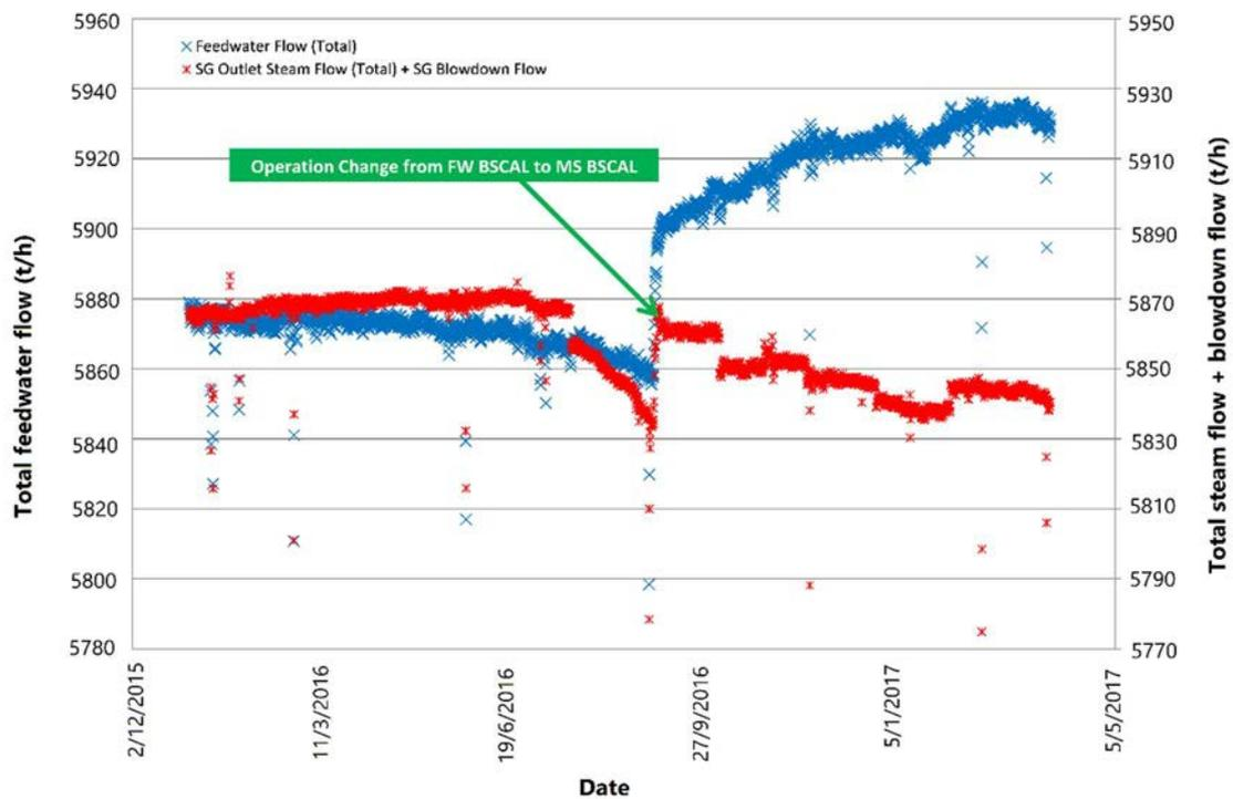
FIG. 106. Trend of FW and MS flows before and after operation change
