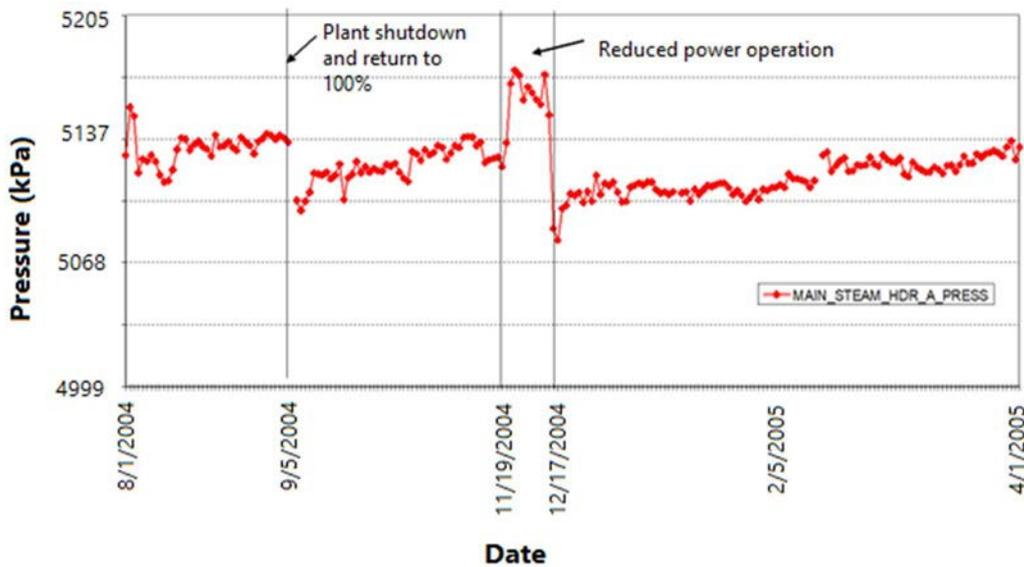
FIG. 114. Steam header pressure (PWR)
