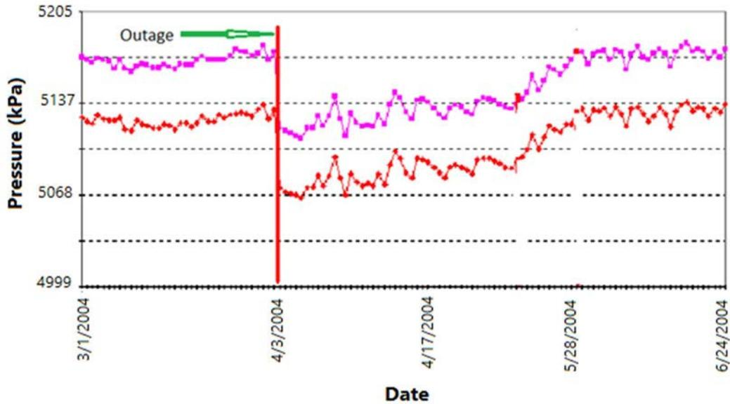
FIG. 113. Steam generator pressure changes
