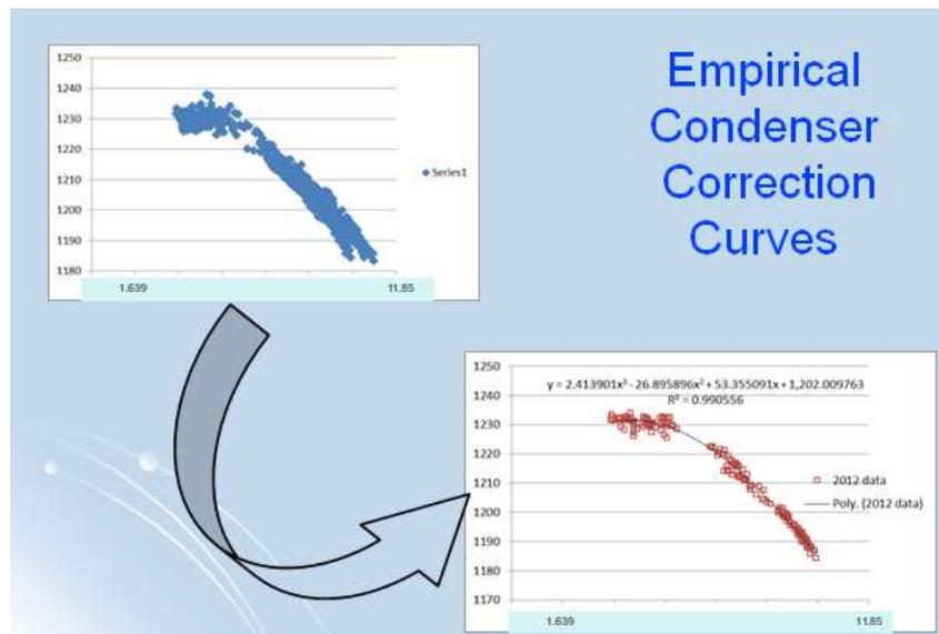
FIG. 45. Empirical condenser correction curves [1]
