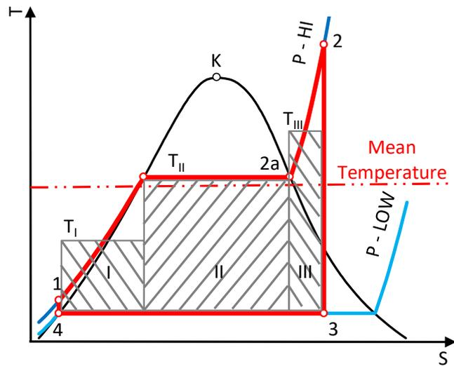
FIG. 80. Partial cycles of Rankine cycle
