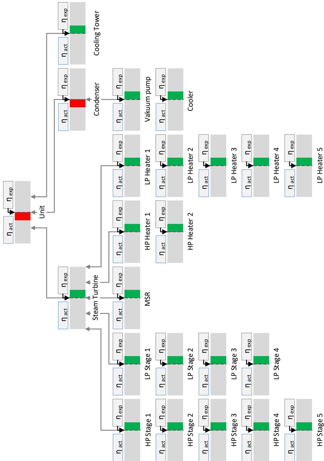
FIG. 32. Identifying the origin of performance deviation – simplified NPP
