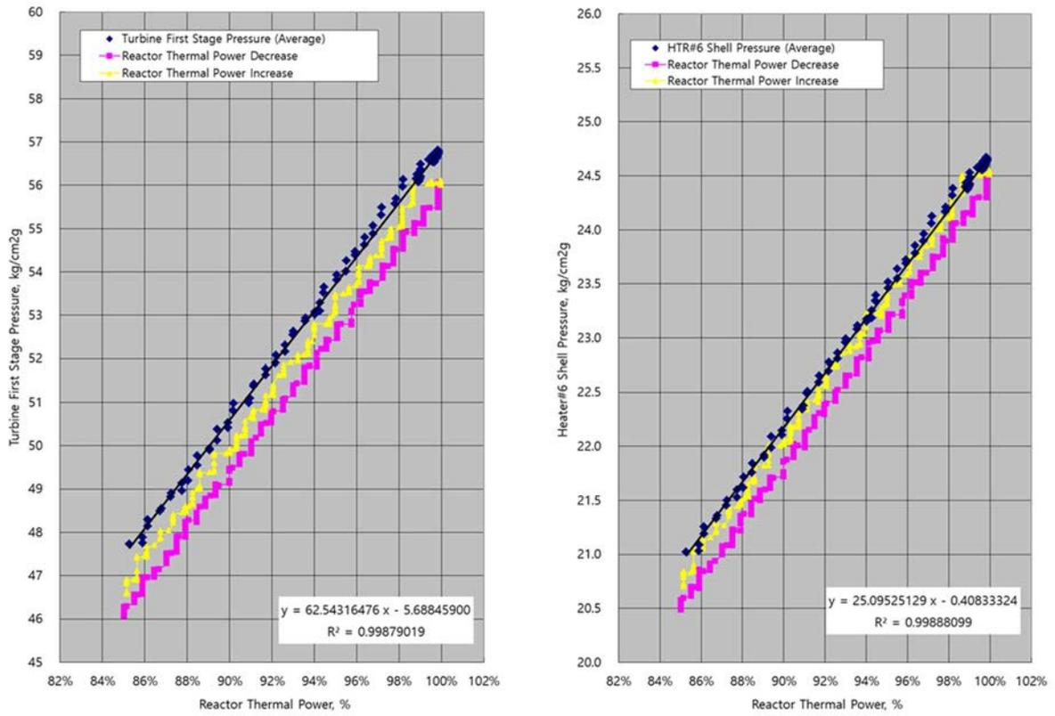
FIG. 59. RTP vs Turbine 1<sup>st</sup> stage Pressure(left); RTP vs HTR#6 Shell Pressure(right)
