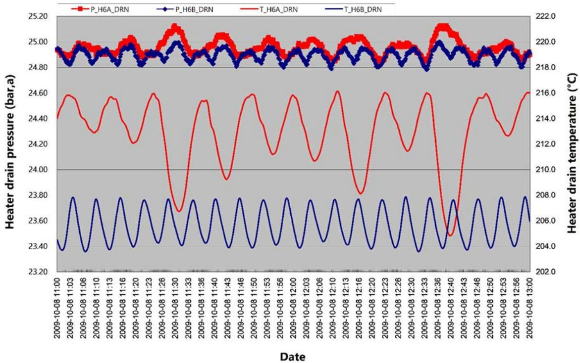
FIG. 129. Oscillation of feedwater heater drain temperature
