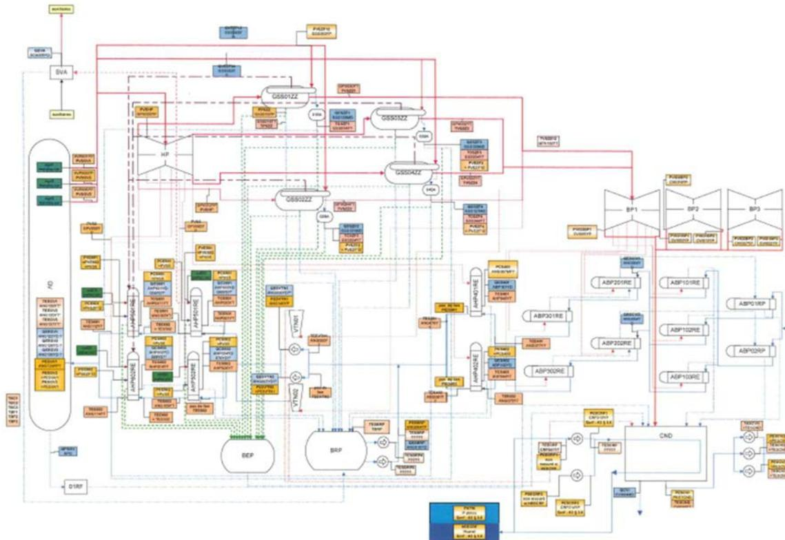
FIG. 33. Thermal model (with sensors)
