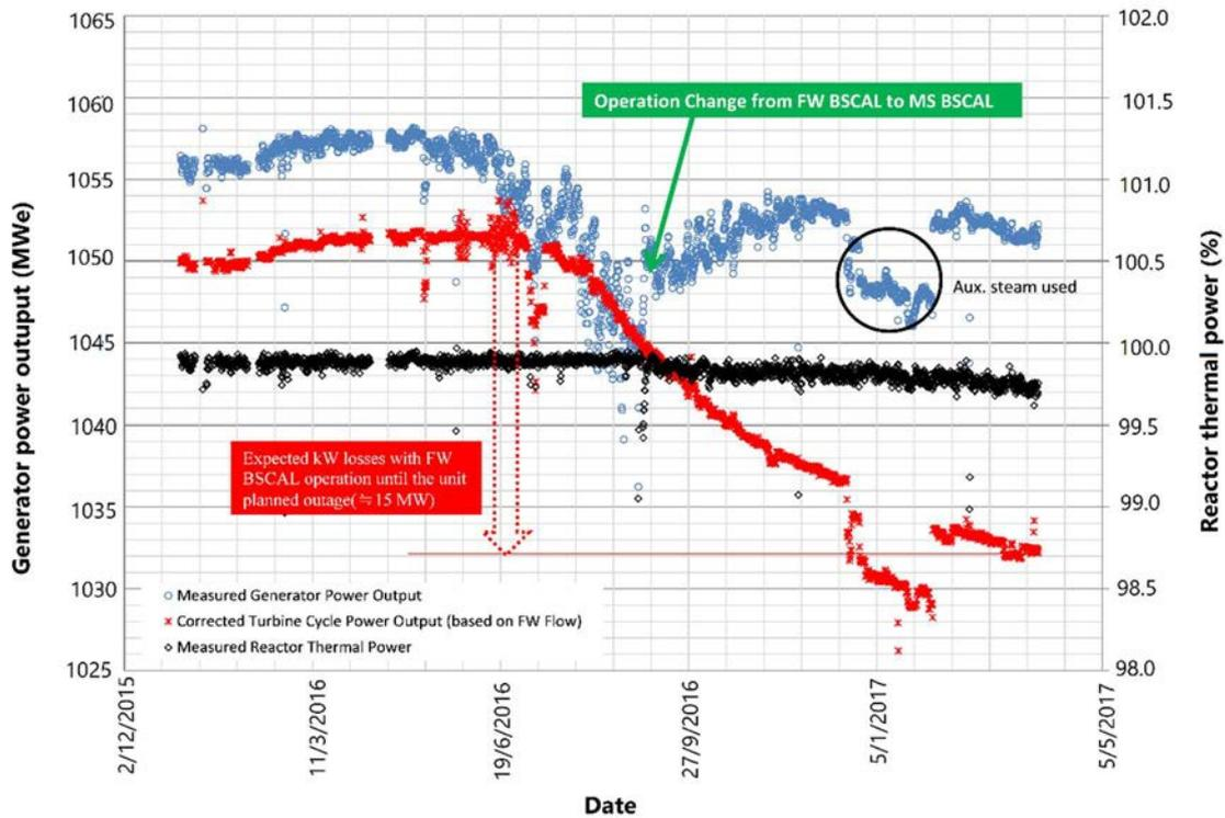
FIG. 107. Trend of electrical power output before and after operation change
