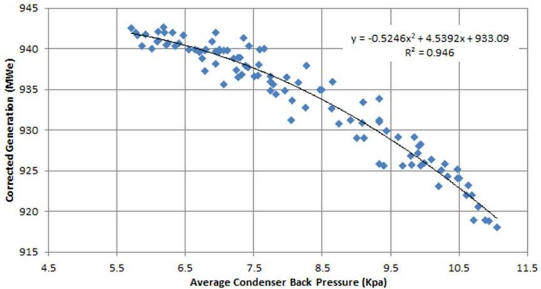
FIG. 50. Correct gross generation for reactor power
