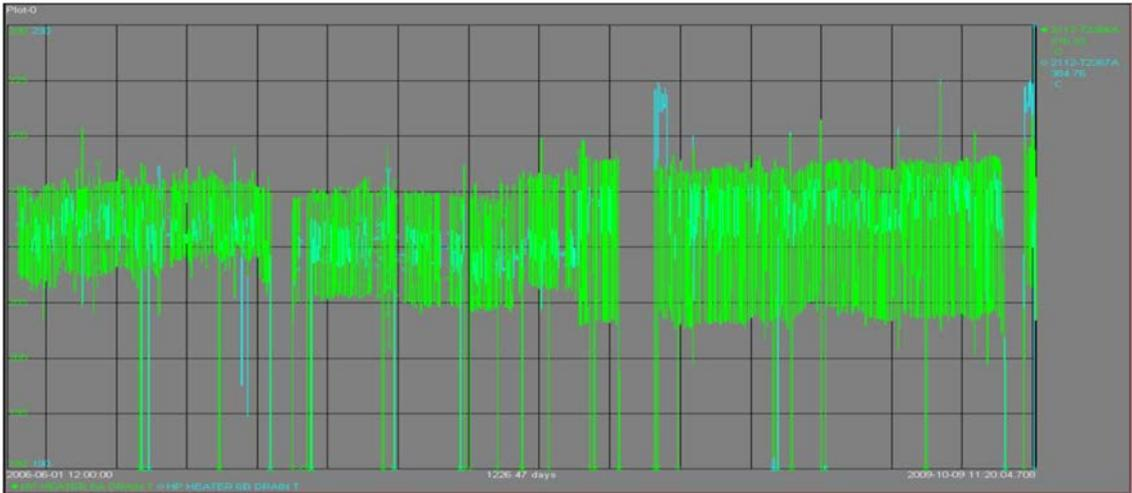
FIG. 131. Trending of heater drain temperature for 5 years
