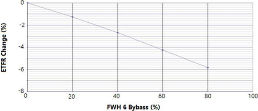
FIG. 127. Bypass FW heater vs ETFR
