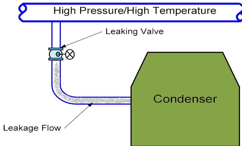
FIG. 14. Cycle isolation condition [1]
