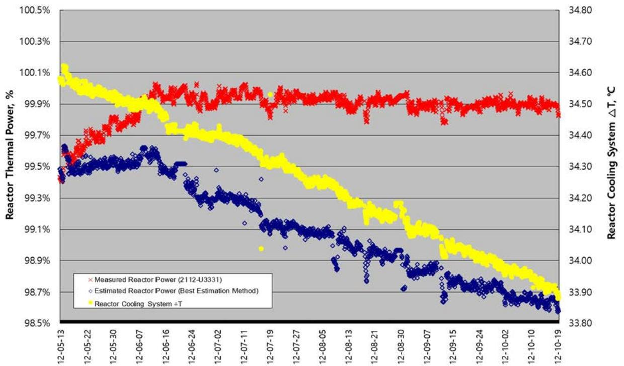
FIG. 72. Trending of RTP vs reactor cooling system  $\Delta T$
