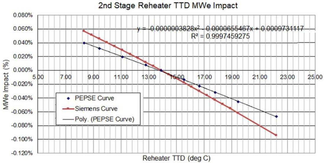
FIG. 41. Resulting curve of relationship between power correction and average MSR TTD
