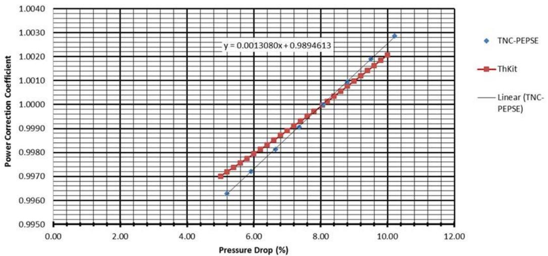
FIG. 43. Resulting curve of relationship between power correction and pressure drop
