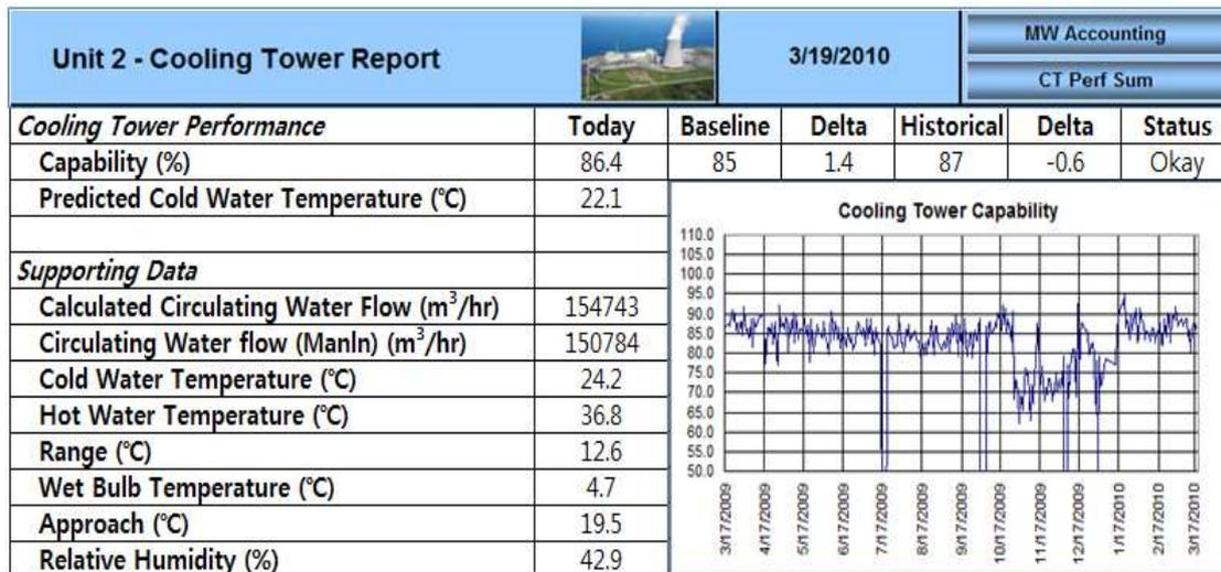
FIG. 99. Example cooling tower monitoring
