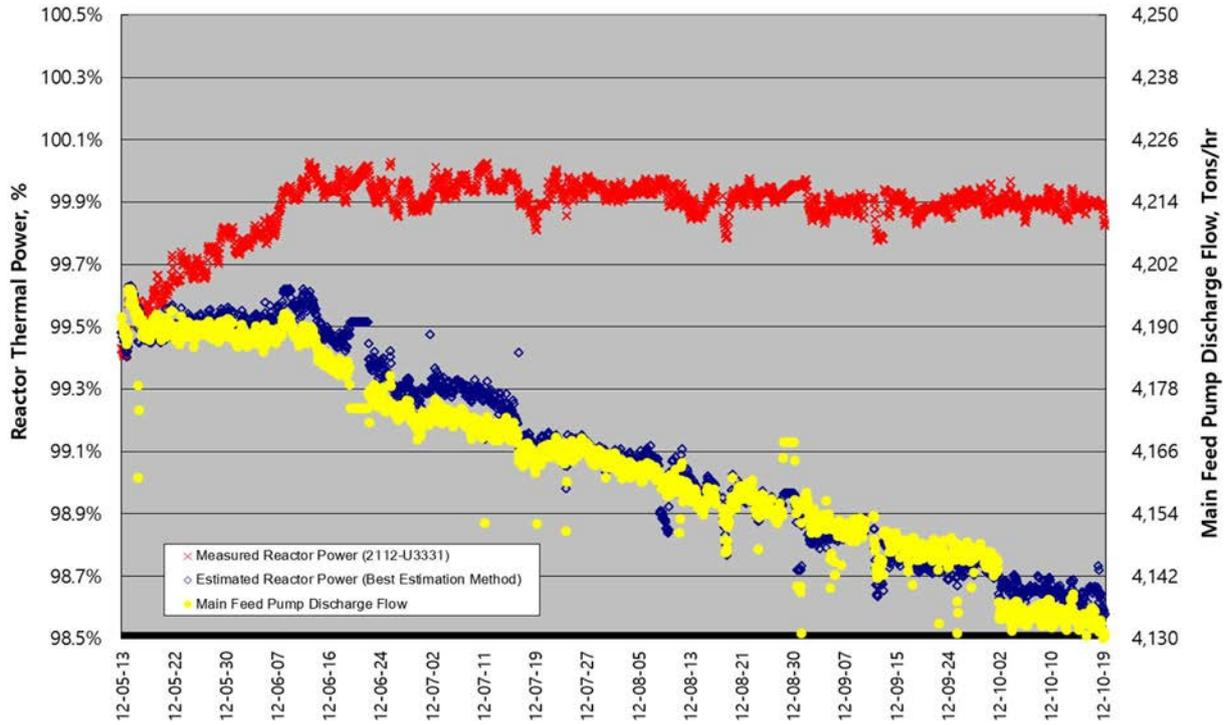
FIG. 65. Trending of RTP vs main feed pump discharge flow
