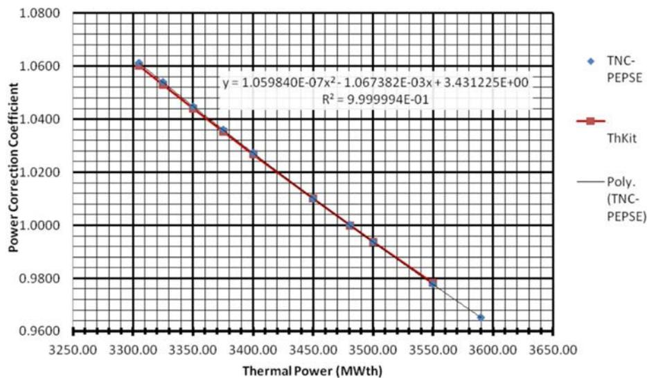
FIG. 40. Resulting curve of relationship between power correction and thermal power
