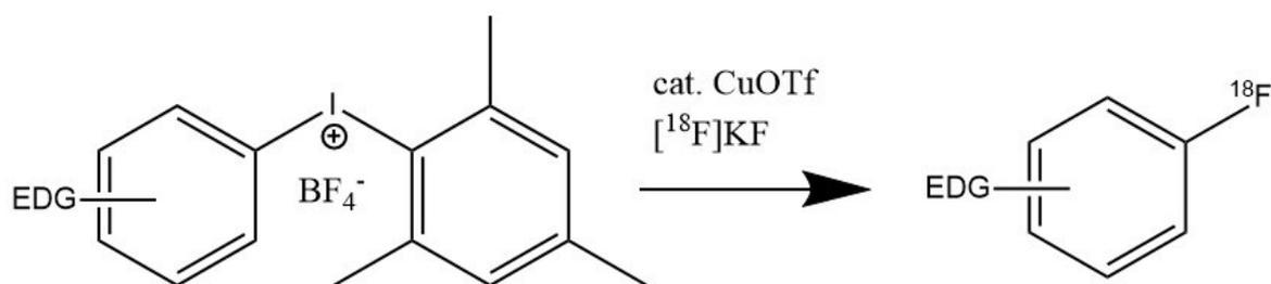
FIG. 65. General reaction scheme for Cu-catalyzed [<sup>18</sup>F]radiofluorination of iodonium salts (courtesy of P. Scott, University of Michigan).
