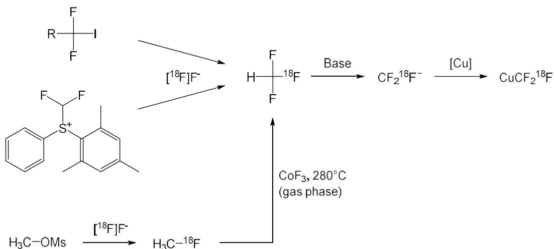
FIG. 79. Preparation of  $[^{18}\text{F}]\text{CuCF}_3$  via  $[^{18}\text{F}]\text{Fluoroform}$  (courtesy of M. Huiban, Invicro LLC).
