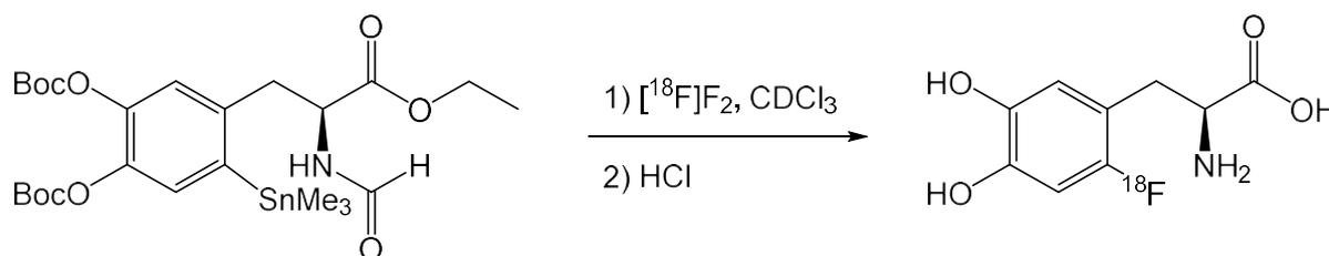
FIG. 35. Preparation of [ $^{18}\text{F}$ ]FDOPA via electrophilic aromatic substitution (courtesy of M. Huiban, Invicro LLC).
