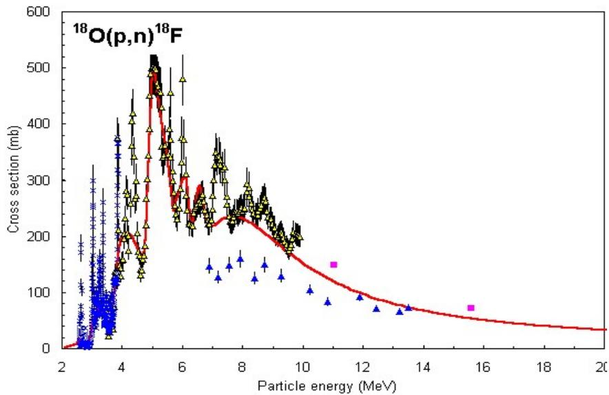
FIG. 11. Cross section for the  $^{18}\text{O}(p,n)^{18}\text{F}$  reaction (reproduced from Ref. [21]).
