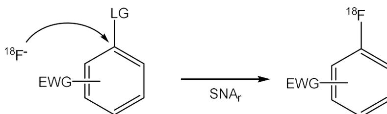
FIG. 38. General principle of nucleophilic aromatic substitutions (electron withdrawing group on ortho or para position) (courtesy of M. Huiban, Invicro LLC).
