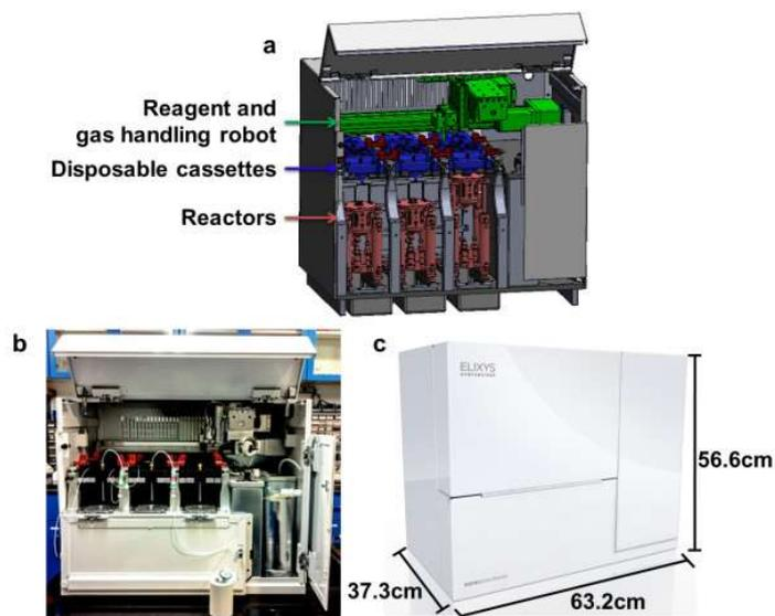
FIG. 31. Hybrid synthesis units (reproduced from Ref. [41] with permission).
