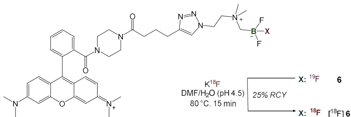
FIG. 71. Direct radiofluorination of a zwitterionic  $\text{AmBF}_3$ -conjugate through  $^{19}\text{F}$ - $^{18}\text{F}$  isotopic exchange (courtesy of R. Schirmacher, University of Alberta).
