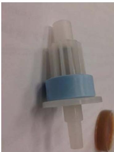
*FIG. 16. Silver release problem in silver body target. Recovered  $\text{H}_2[^{18}\text{O}]\text{O}$  (left), QMA Cartridge with silver ion contamination (right) (courtesy of E. Cazzola, Sacro Cuore Hospital).*
