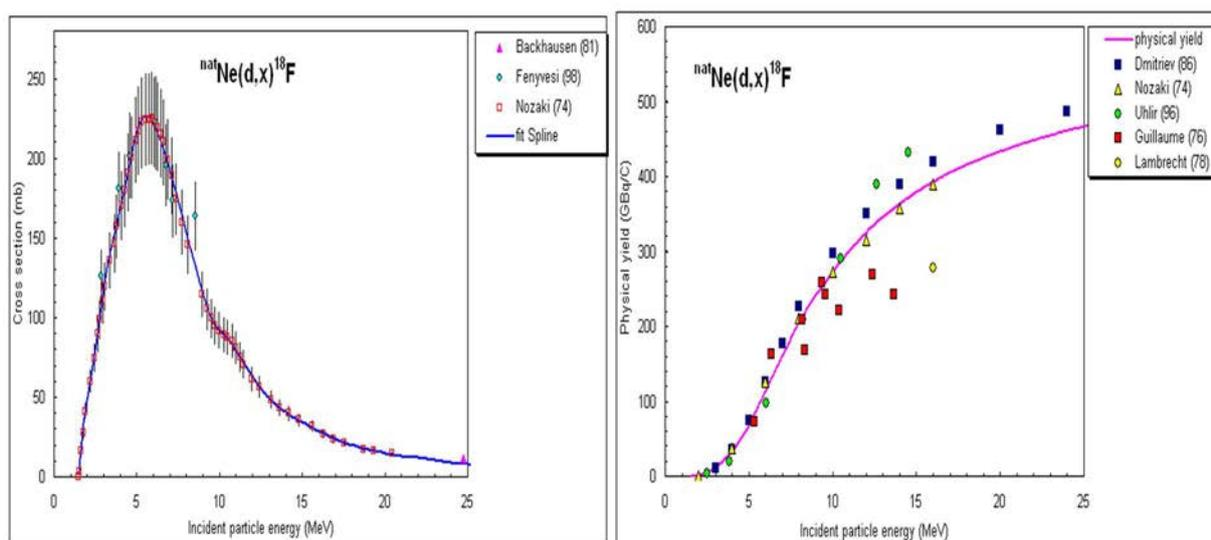
FIG. 10. Cross section and yield curves for the  $^{20}\text{Ne}(\text{d},\alpha)^{18}\text{F}$  reaction.
