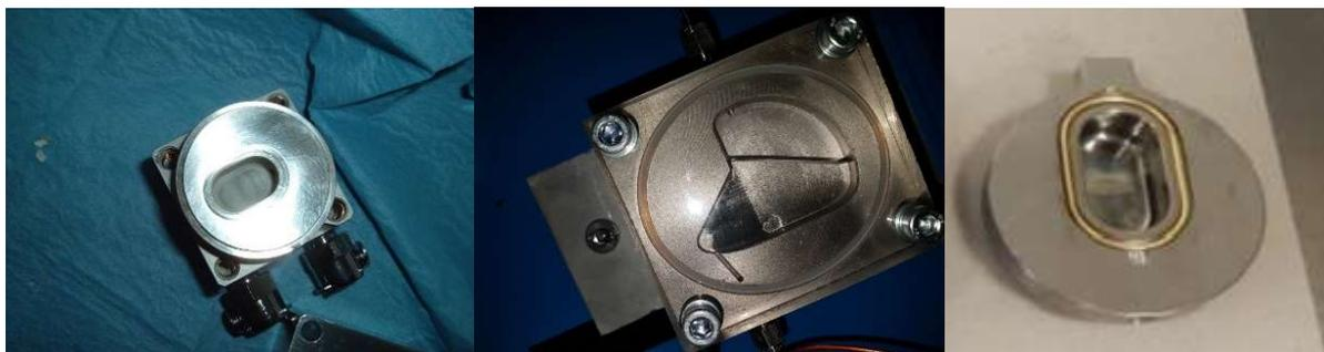
FIG. 17. Vertical target body of MINITrace, angled target body shape from ACSI, PETtrace vertical body target (courtesy of E. Cazzola, Sacro Cuore Hospital).
