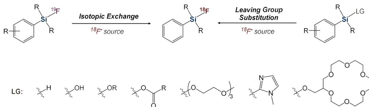
FIG. 69. General scheme for radiofluorination of SiFA compounds (courtesy of R. Schirmacher, University of Alberta).
