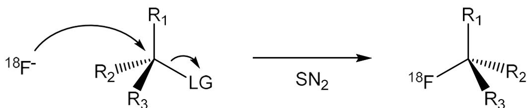
FIG. 36. General principle of nucleophilic aliphatic substitutions (courtesy of M. Huiban, Invicro LLC).
