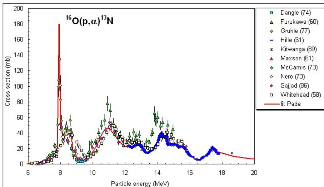
FIG. 21. Excitation function of the nuclear reaction  $^{16}\text{O}(p,\alpha)^{13}\text{N}$  from 6–20 MeV protons (reproduced from Ref. [15]).
