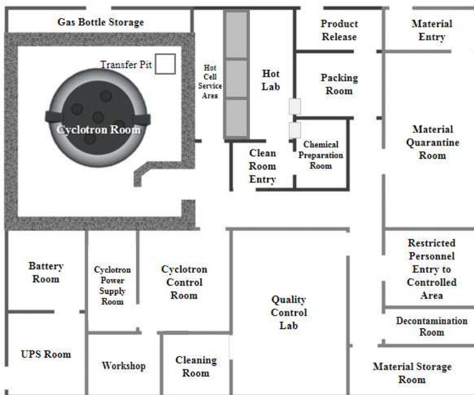
FIG. 93. The layout of a typical cyclotron PET radiopharmaceuticals production facility used for the manufacture of [ $^{18}\text{F}$ ]FDG and  $^{18}\text{F}$  radiopharmaceuticals (courtesy of Ajith, J., Molecular Cyclotrons).
