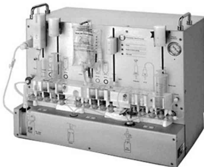
FIG. 27. Early cassette-based synthesis module (reproduced from Ref. [35] with permission).
