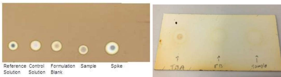
FIG. 33. Colorimetric assays for  $K_{222}$  (left) and TBA (right) testing (courtesy of M. Huiban, Invicro LLC).
