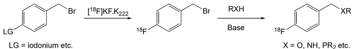
FIG. 52. 4- $^{18}\text{F}$ fluorobenzyl bromide building block (courtesy of P. Scott, University of Michigan).
