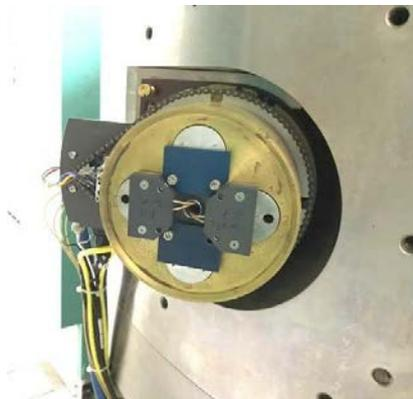
FIG. 15. A target carousel having two targets and two Faraday cups used in a Siemens HP cyclotron (courtesy of M. Anees, Molecular Cyclotrons).
