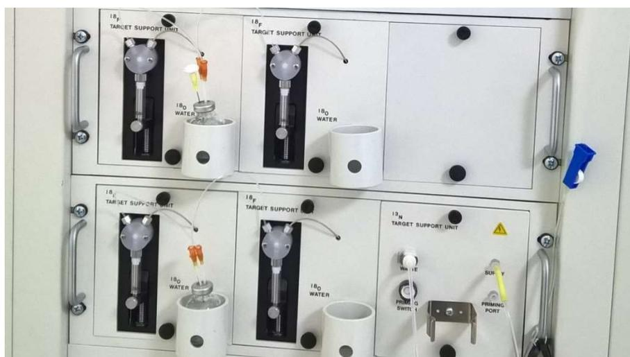
FIG. 20.  $^{18}\text{O}$ -enriched water loading station (courtesy of M. Anees, Molecular Cyclotrons).
