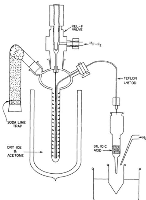
FIG. 24. Early laboratory set-up for the synthesis of  $[^{18}\text{F}]\text{FDG}$  (reproduced from Ref. [31] with permission of [© 1983 John Wiley & Sons, Ltd.]).
