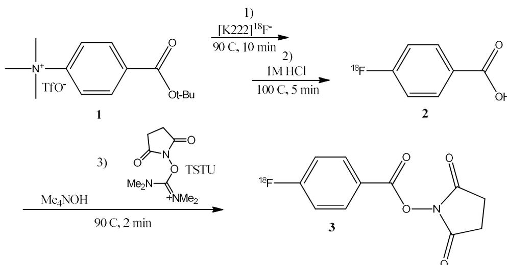
FIG. 59. Synthesis scheme of the automated [<sup>18</sup>F]SFB synthesis (courtesy of R. Schirmacher, University of Alberta).
