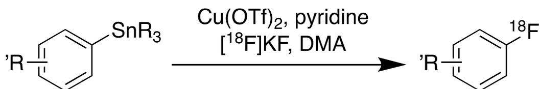
FIG. 64. General reaction scheme for Cu-catalyzed [<sup>18</sup>F]radiofluorination of arylstannanes (courtesy of P. Elsinga, University of Groningen).
