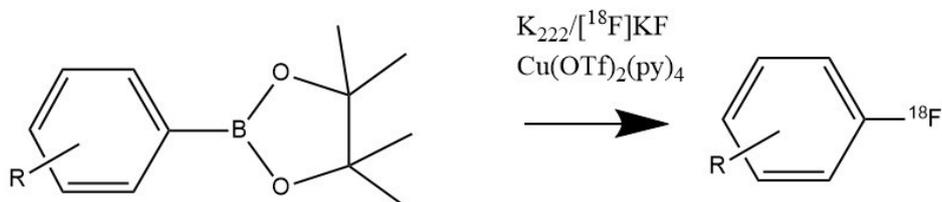
FIG. 62. General reaction scheme for Cu mediated  $[^{18}\text{F}]$ fluorination of boronic pinacol ester precursors (courtesy of P. Elsinga, University of Groningen).
