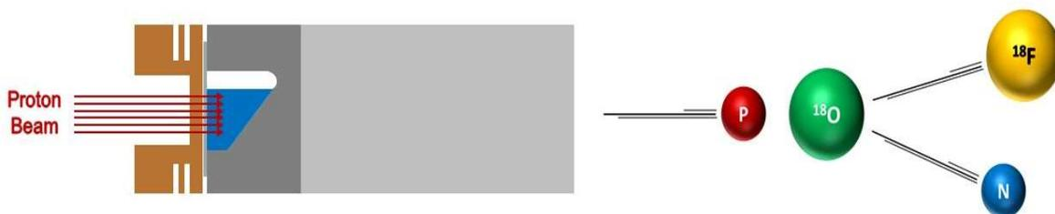
FIG. 19. The sequence for the production of  $^{18}\text{F}$  using a  $^{18}\text{O}$ -water target (top). Schematic of the targetry and the proton beam (bottom, left). Schematic representation of the nuclear reaction (bottom right). (Courtesy of N. Raviteja, Molecular Cyclotrons,).
