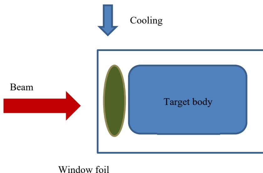
FIG. 13. Simplified target drawing (courtesy of E. Cazzola, Sacro Cuore Hospital).
