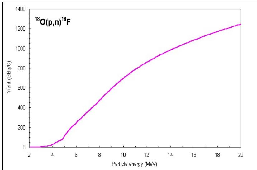
FIG. 12. The yield curve for the  $^{18}\text{O}(p,n)^{18}\text{F}$  reaction from 2-20 MeV (reproduced from Ref. [21]).
