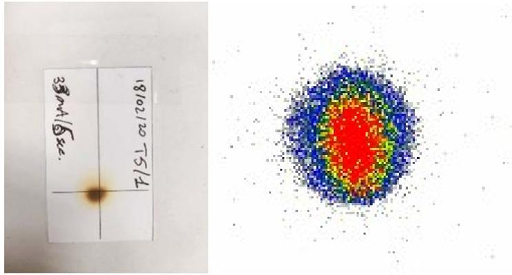
FIG. 18. Paper burn beam shape from PETtrace cyclotron, Metal burn beam shape from TR19 cyclotron (courtesy of E. Cazzola, Sacro Cuore Hospital).
