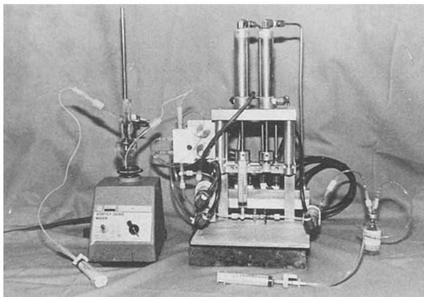
FIG. 25. Early homemade radiosynthesizer (reproduced from Ref. [32] with permission of [© 1983 John Wiley & Sons, Ltd.]).
