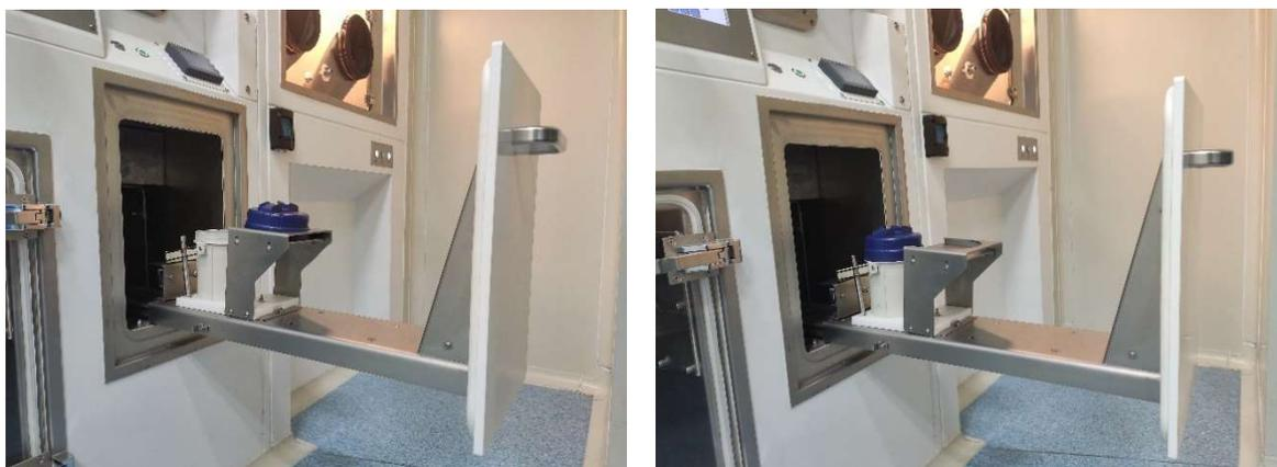
*FIG. 98. Packaging of dispensed radiopharmaceuticals inside lead/tungsten containers (courtesy of K. Dilshad, Molecular Cyclotrons).*
