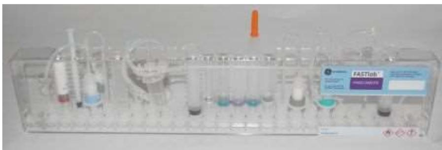
FIG. 29. A sample of a radiopharmaceutical cassette (courtesy of GE).
