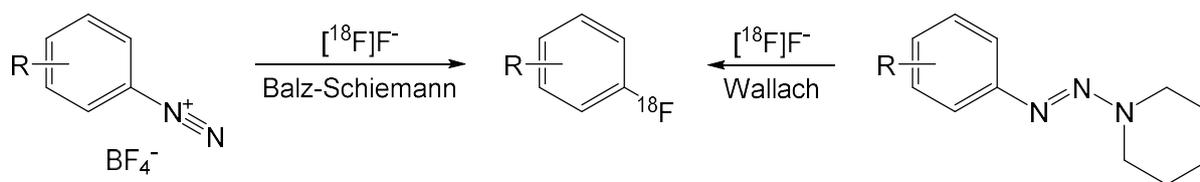
FIG. 40. Balz–Schiemann and Wallach reactions (courtesy of M. Huiban, Invicro LLC).
