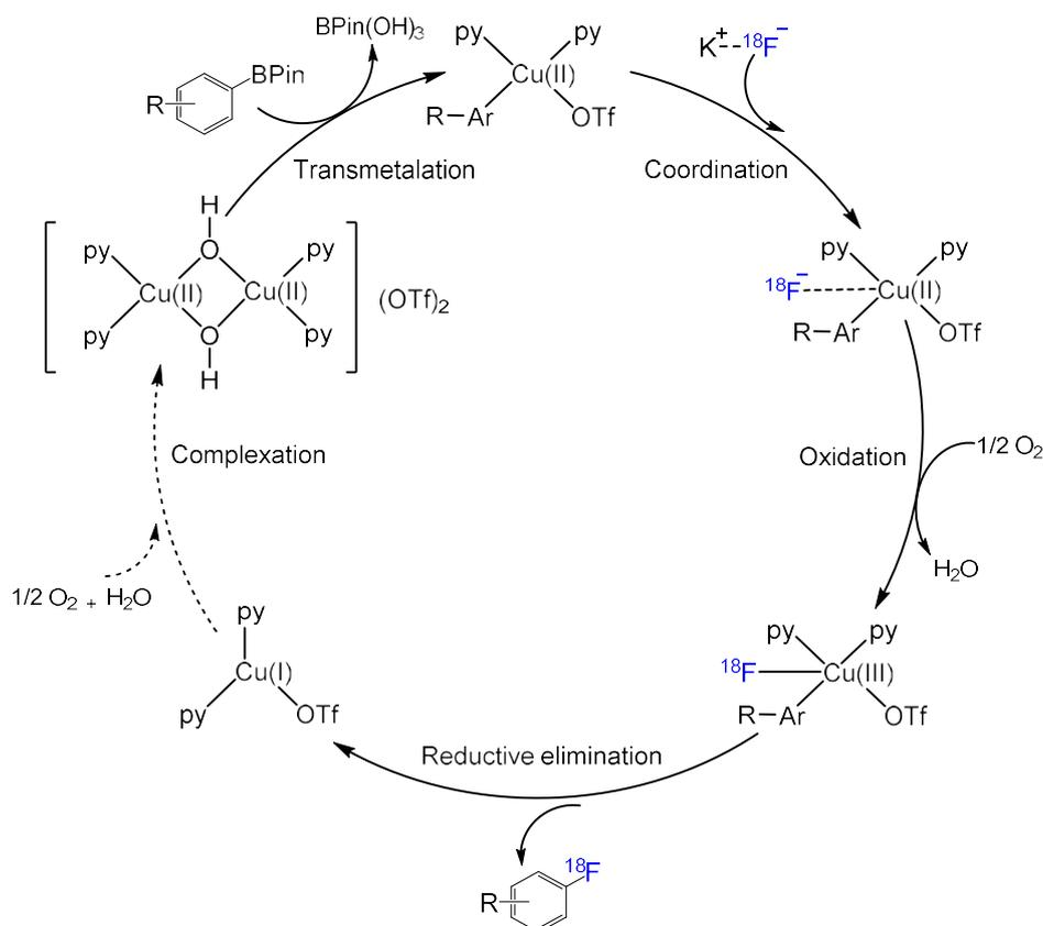
FIG. 63. Proposed mechanism for Cu mediated oxidative  $[^{18}\text{F}]$ fluorination of arylboronic esters (reproduced from Ref. [88] with permission).
