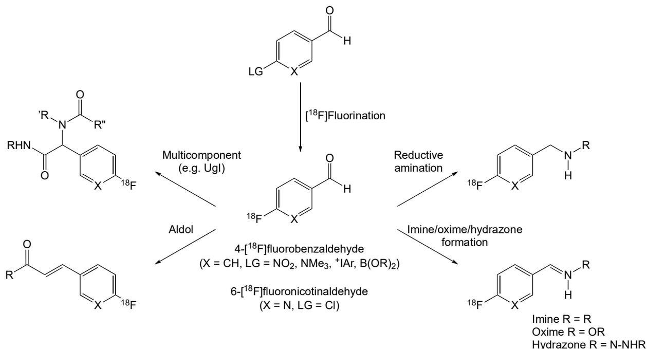
FIG. 50.  $^{18}\text{F}$ fluorobenzaldehyde building block (courtesy of P. Scott, University of Michigan).
