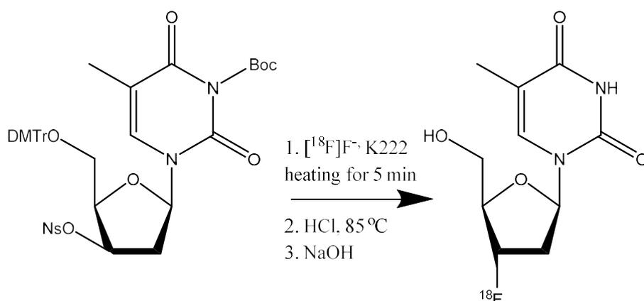
FIG. 115. Synthesis of [ $^{18}\text{F}$ ]FLT via the DMTr-nosyl-lyxothymidine approach.
