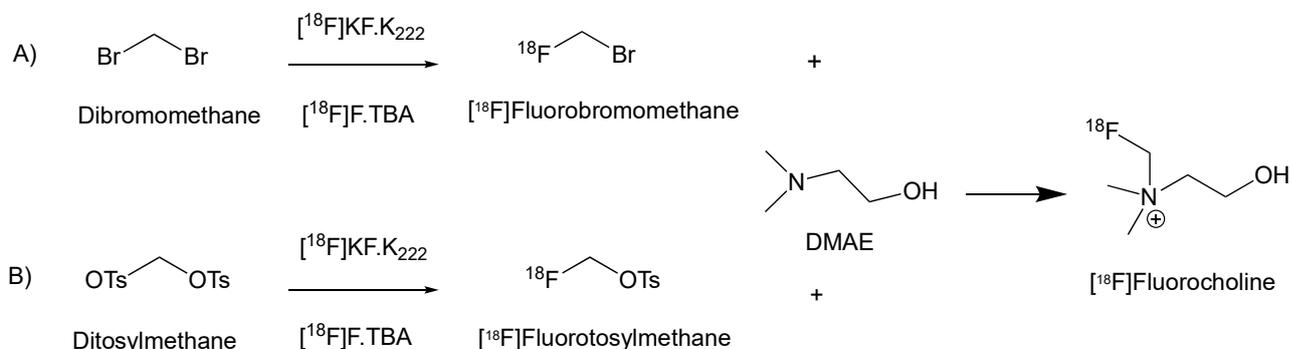
FIG. 108. Reaction scheme for the synthesis of  $^{18}\text{F}$ Fluorocholine ( $^{18}\text{F}$ FCH) (courtesy of E. Cazzola, Sacro Cuore Hospital).
