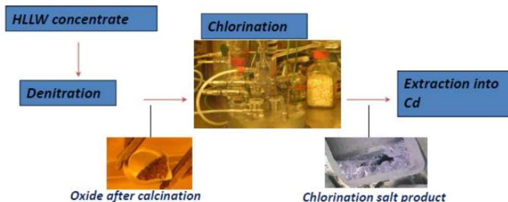
FIG. 29. TRUs recovery from HLLW prepared by SNF dissolution [44].
