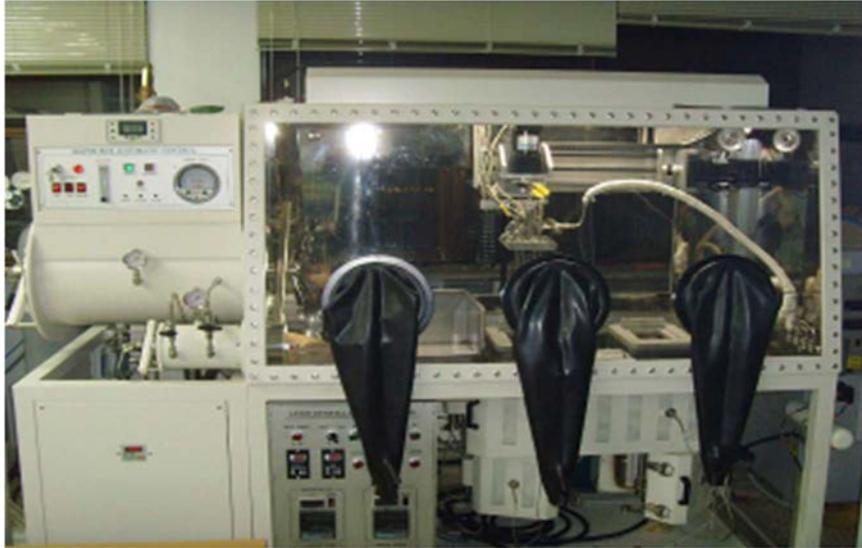
FIG. 37. Laboratory scale layer crystallization apparatus [88].
