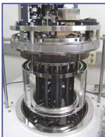
FIG. 35. High throughput electrorefiner equipped with graphite cathode [85].
