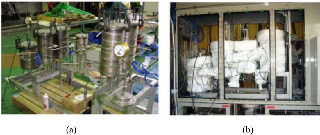
FIG. 30. (a) Four staged counter-current extractor with  $KCl-LiCl/Cd$  system for separation of actinides from lanthanides [77]; (b) The equipment of the left hand side was covered with heat-shielding in a glove-box (reproduced courtesy of CRIEPI).
