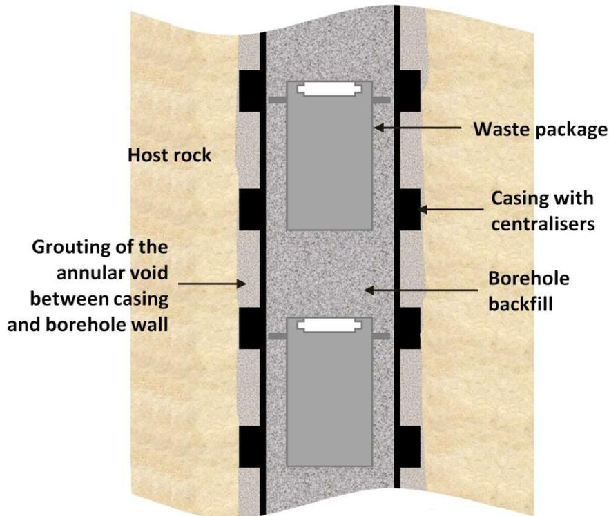
FIG. 34. Cross-section of the borehole in the disposal zone.
