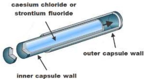
FIG. 39. Schematic drawing of the Cs and Sr capsules (modified from [83]) (Courtesy of SANDIA NL).
