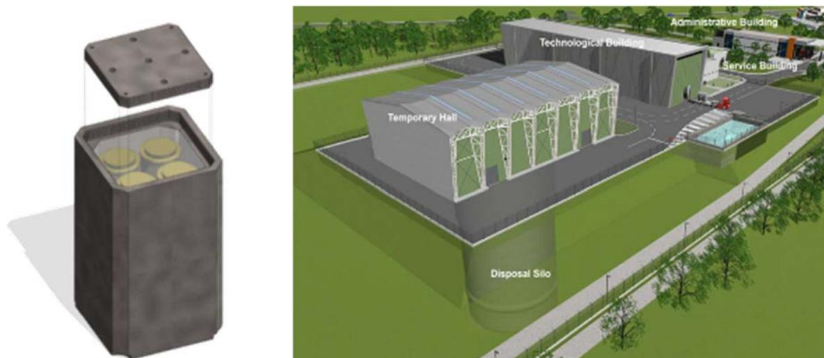
FIG. 9. Drawings of the concrete disposal container (left) and disposal silo during the operational phase (right) (Courtesy of ARAO).
