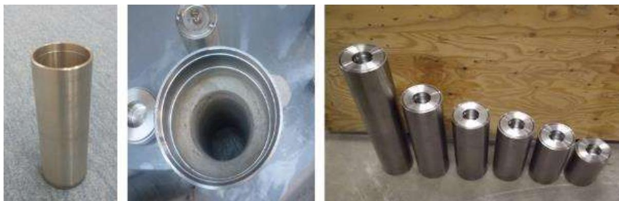
FIG. 33. Design of the waste package: sources are placed in 3 mm thick stainless-steel capsules (left) which are placed in a 6 mm thick stainless steel disposal container which is backfilled with a cementitious material (middle). A set of disposal containers with different lengths is available (right).
