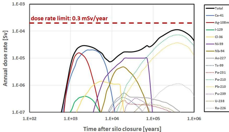
FIG. 11. Calculated dose rates based on a safety assessment for a normal evolution scenario.
