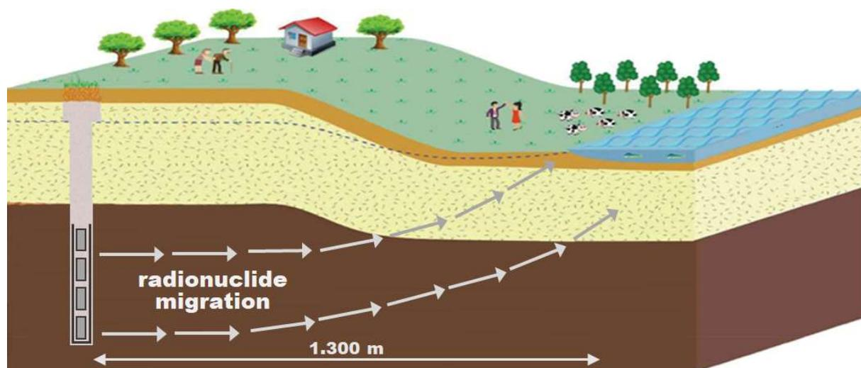
FIG. 35. Conceptual model of the normal evolution scenario: liquid radionuclide release in the saturated zone with the river as the geosphere-biosphere interface (figure is not to scale) (modified from [67]).
