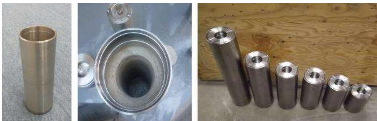
FIG. 33. Design of the waste package: sources are placed in 3 mm thick stainless-steel capsules (left) which are placed in a 6 mm thick stainless steel disposal container which is backfilled with a cementitious material (middle). A set of disposal containers with different lengths is available (right).
