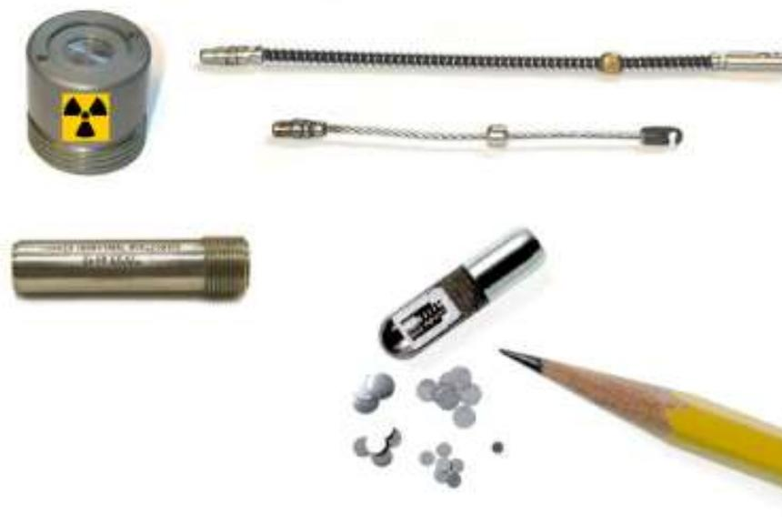
*FIG. 1. Some examples of sealed radioactive sources (the pencil indicates the scale).*
