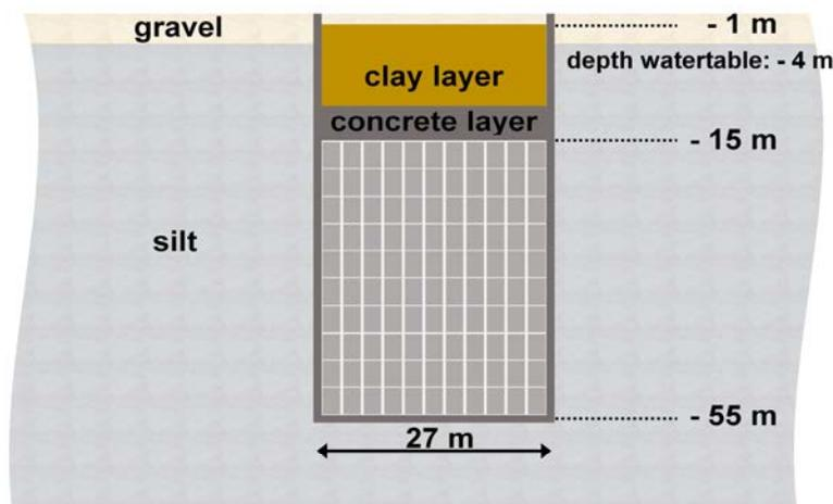
FIG. 10. Schematic view of the disposal silo.
