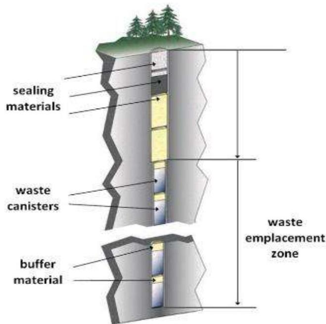
FIG. 37. Very deep borehole disposal concept (modified from [70]) (Courtesy of SKB).
