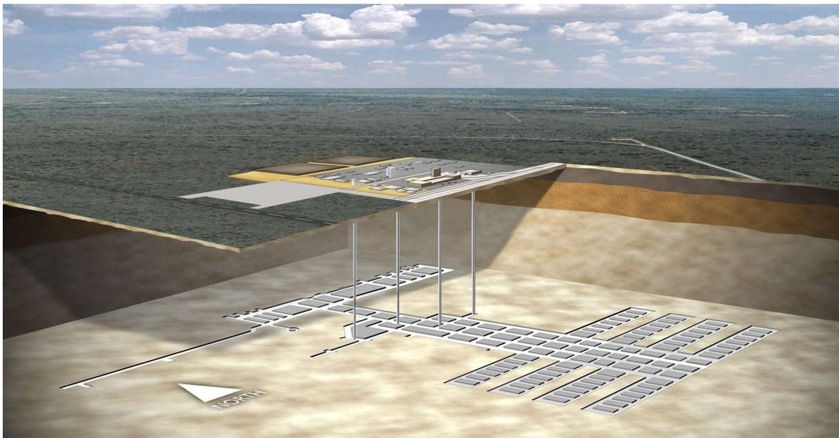
FIG. 4. Schematic picture of the WIPP facility at a depth of ca. 650 m in a salt formation in New Mexico (USA) (Courtesy of USA DOE).
