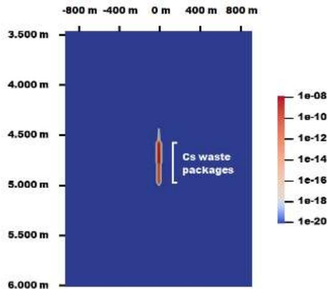
FIG. 43. Calculated dissolved Cs-135 concentrations around the disposal zone after 10 million years (modified from [86]) (Courtesy of SANDIA NL).
