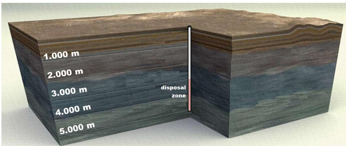
FIG. 38. The deep borehole disposal concept considered in the Deep Borehole Field Test studies (modified from [83]) (Courtesy of SANDIA NL).
