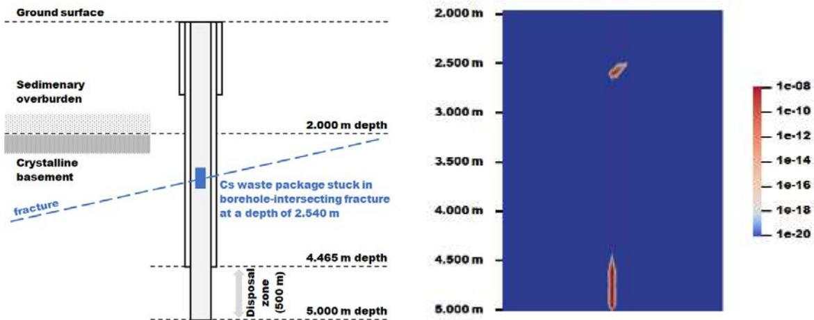
FIG. 44. Alternative scenario of a Cs-containing waste package that got stuck at a borehole-intersecting fracture at a depth of 2.500 m (left) and the calculated Cs-135 concentrations along this fracture after 10 million years (right) assuming a regional flow gradient of 0.1 mm/m (modified from [86]) (Courtesy of SANDIA NL).
