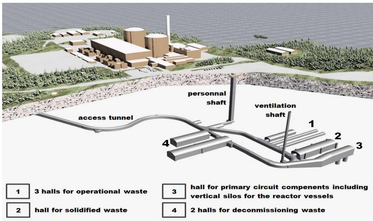
FIG. 19. Layout of the disposal facility consisting of several waste caverns (halls or silos) for different waste types. The caverns for the decommissioning waste will be excavated prior to decommissioning phase of the reactor unit; other parts of the facility have been already built (Courtesy of FORTUM).
