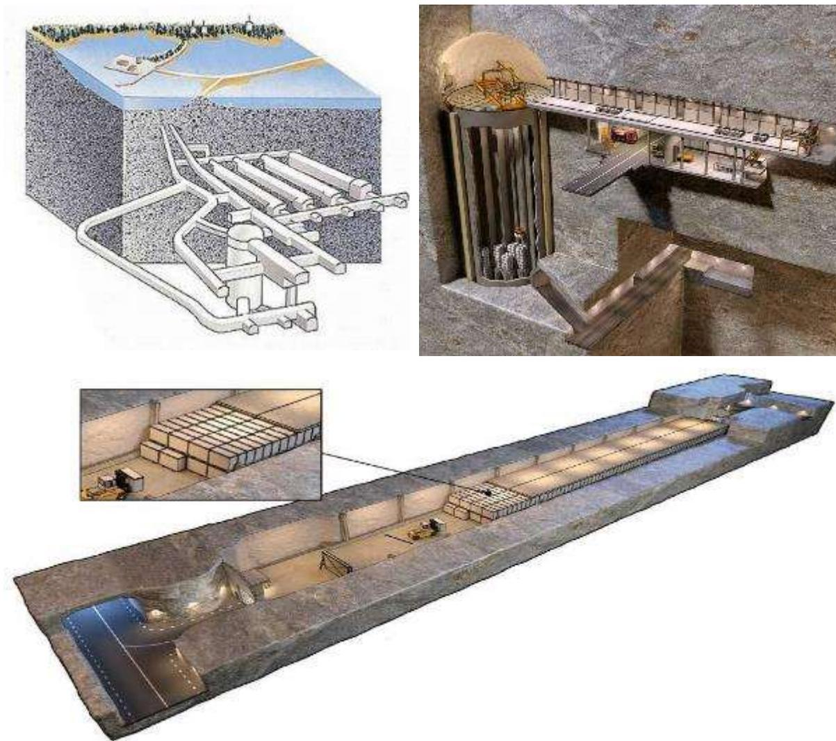
FIG. 14. Schematic picture of the current layout of the SFR disposal facility (top left), the disposal silo (top right) and a disposal cavern (bottom) [54] (Courtesy of SKB, Illustrator LAJ illustration).
