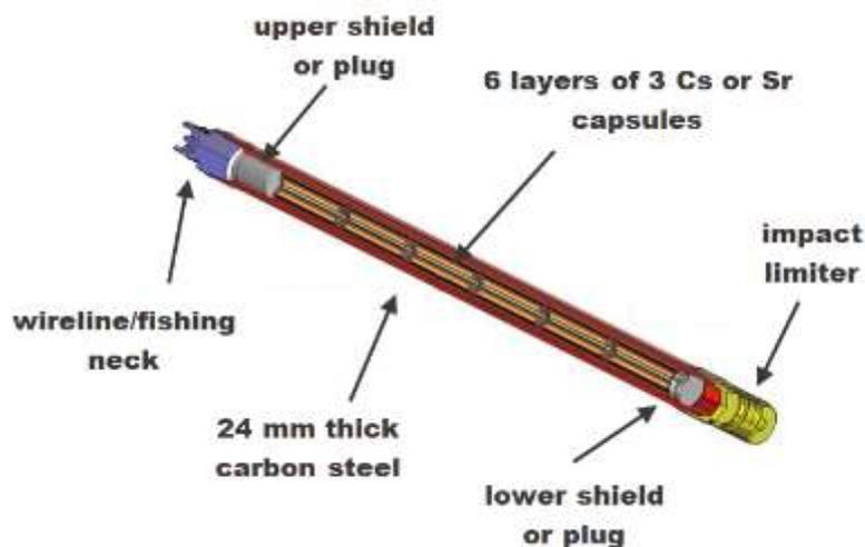
FIG. 40. Schematic drawing of the Cs and Sr capsules (modified from [83]) (Courtesy of SANDIA NL).
