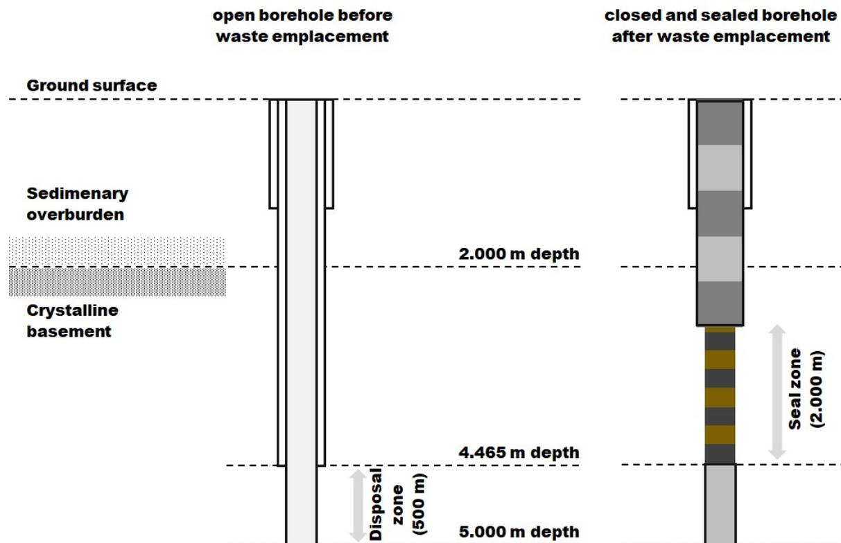
FIG. 41. Conceptual design of the disposal borehole: open borehole before waste emplacement (left) and closed borehole with the sealed zone consisting of an alternating sequence of bentonite and cement plugs and the part above this zone with alternating concrete and cement plugs (right) (modified from [82]) (Courtesy of SANDIA NL).
