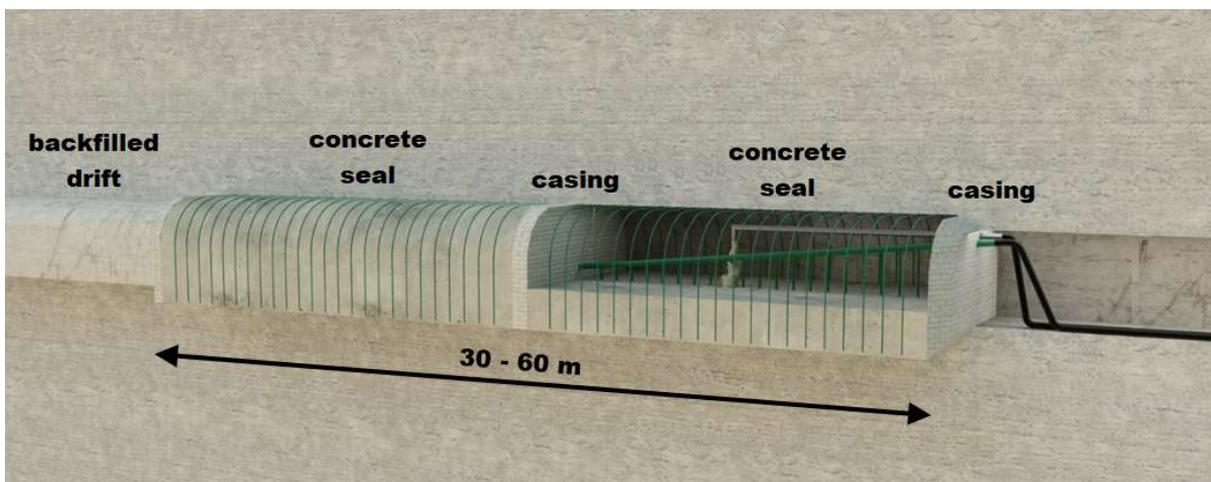
FIG. 31. Drift seals consisting of a long body of concrete (Courtesy of BGE).
