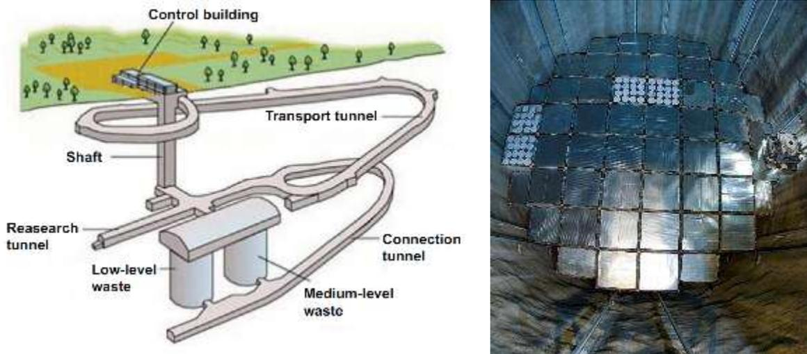
FIG. 16. Schematic drawing of the current layout of the VLJ repository for LLW and ILW (left) and top view of a silo (right) (modified from [56]) (Courtesy of POSIVA).
