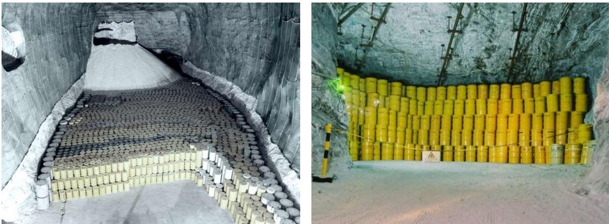
FIG. 29. Disposal of solid waste by stacking waste drums (Courtesy of BGE).
