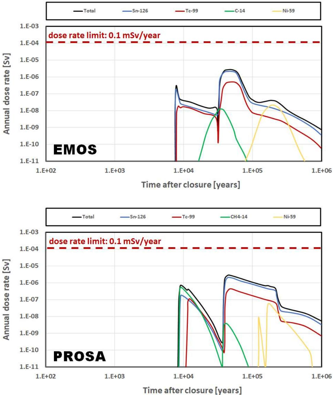
FIG. 32. Calculated dose rates from the Morsleben repository disposal facility using the EMOS model (top) and PROSA (bottom) models.
