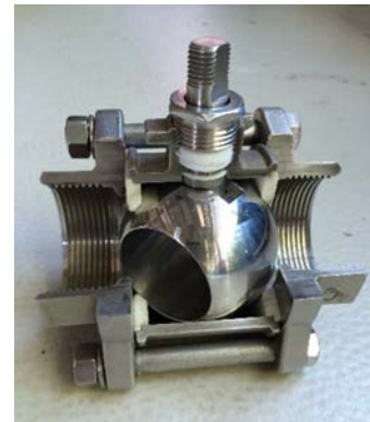
FIG.9. BALL VALVE INTERNAL COMPONENTS
