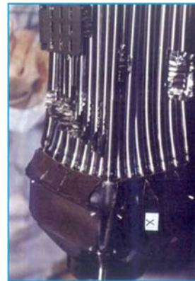
FIG. 35. Fresh BWR FA after 9 m drop test (picture courtesy of TN International and INS Ltd. [7]).
