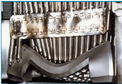
FIG. 34. Fresh PWR FA after 9 m drop test (picture courtesy of TN International and INS Ltd. [7]).
