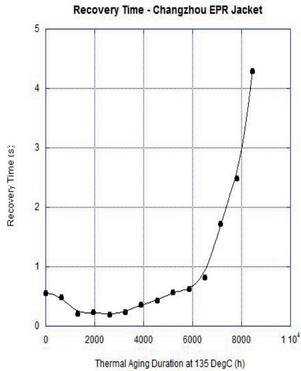
FIG. 88. IM and recovery time results for unaged and thermally aged Changzhou EPR jacket samples.
