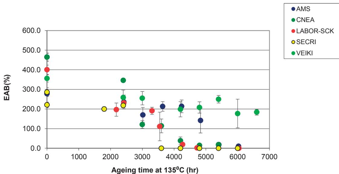
FIG. 75. EAB data for XLPO insulation (Shanghai).
