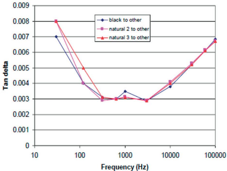
FIG. 28. Tan  $\delta$  Data on unaged PEEK cable with sweep frequency 30 Hz – 105 Hz provided by VEIKI-VNL.
