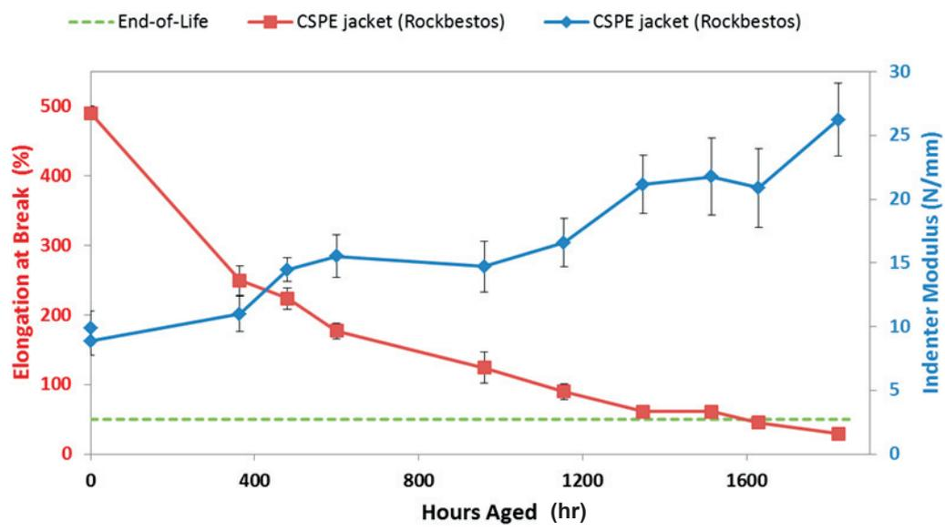
FIG. 8. Indenter modulus correlated with EAB using 50% EAB end of life designator (Reproduced with permission courtesy of AMS corporation).
