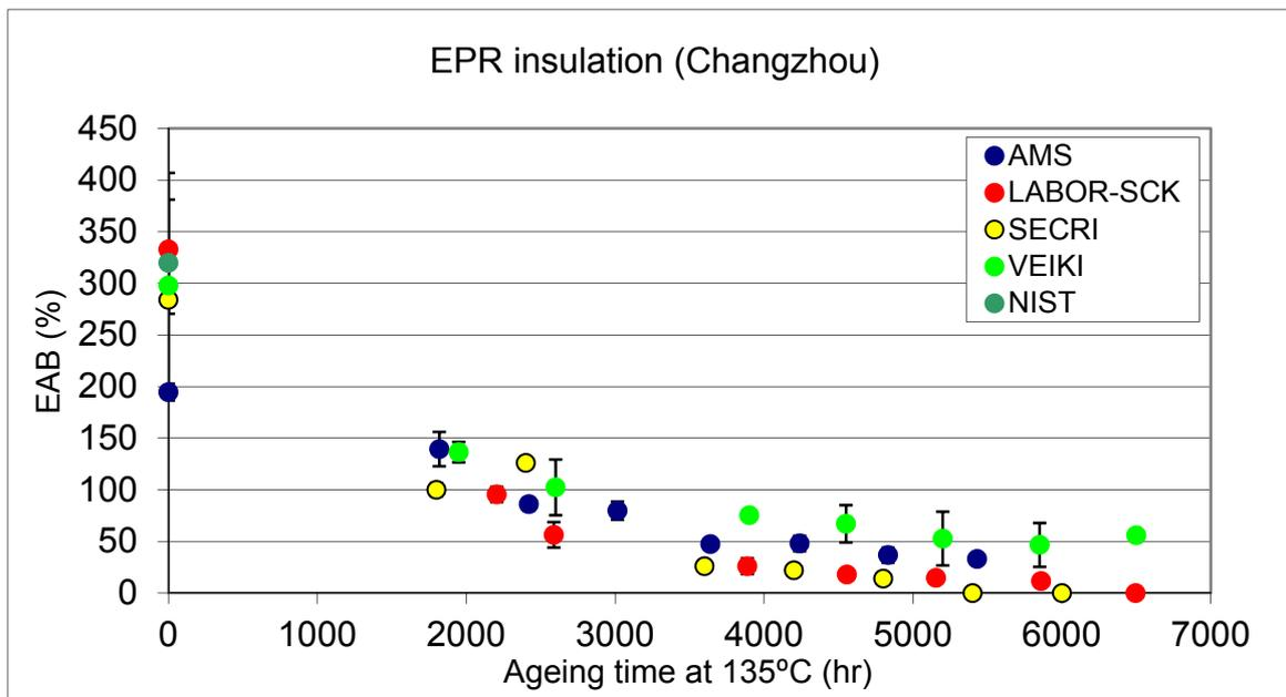
FIG. 66. EAB data for EPR insulation (Changzhou).
