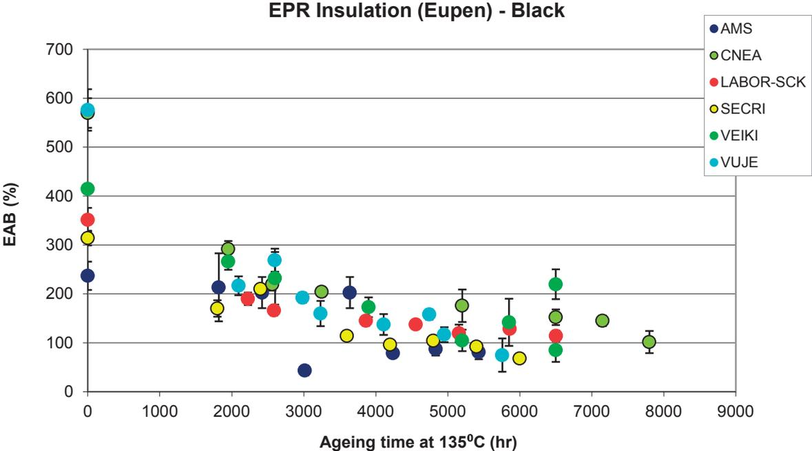
FIG. 51. EAB data for thermal ageing of EPR insulation (Eupen) – black colour.
