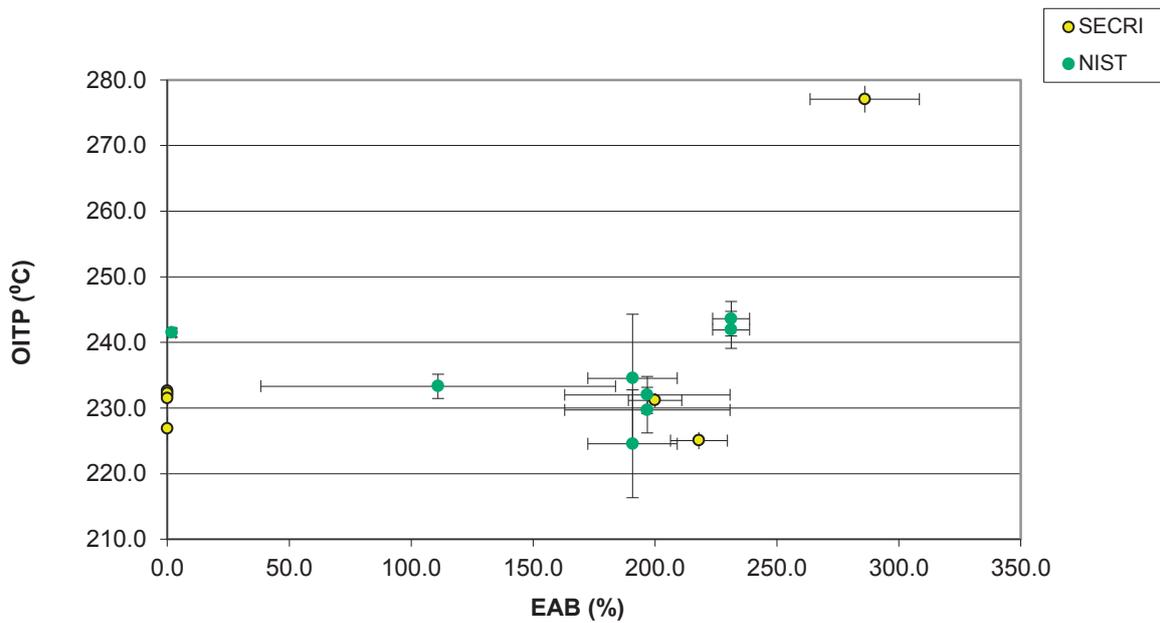
FIG. 78. Cross-plot of OITP vs. EAB for XLPO insulation (Shanghai).
