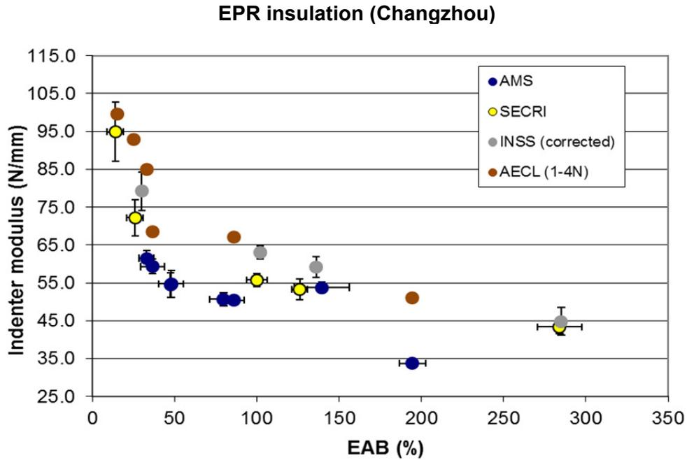
FIG. 67. Cross-plot of IM vs. EAB for EPR insulation (Changzhou).
