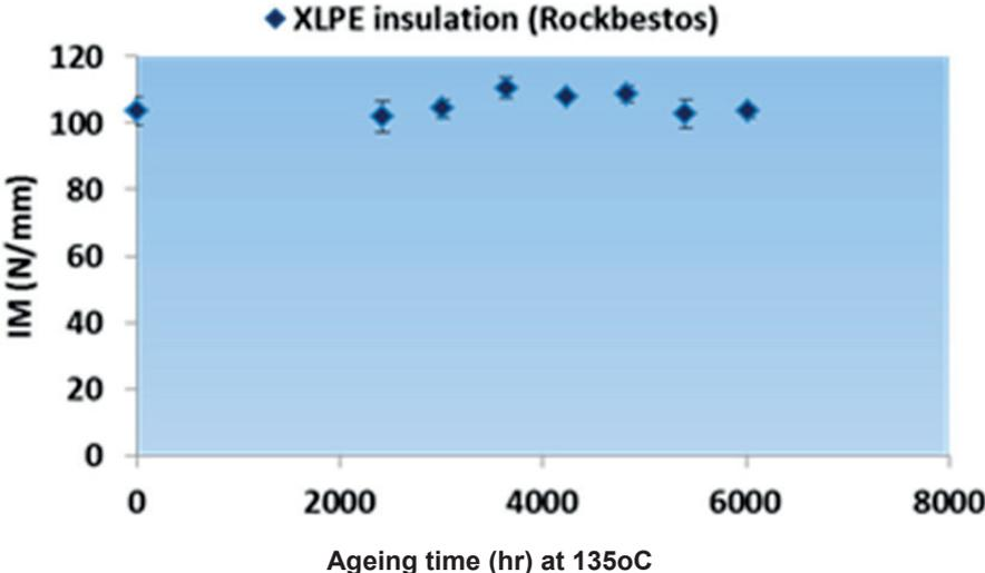
FIG. 123. XLPE insulation IM test.
