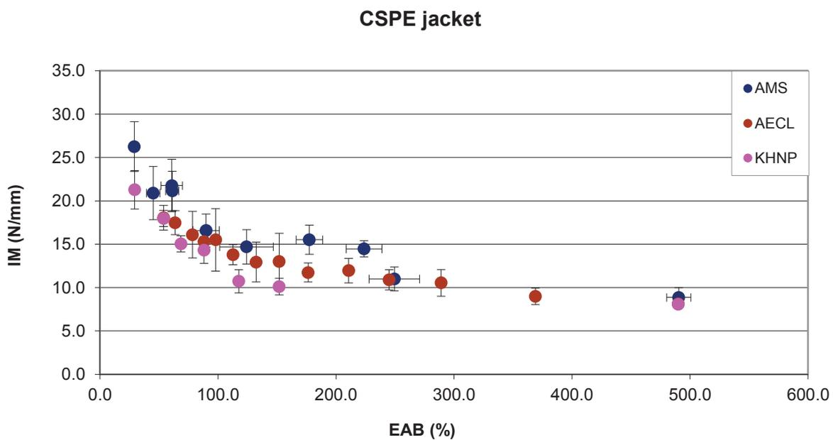
FIG. 61. Cross-plot of IM vs. EAB for CSPE jacket (Rockbestos).
