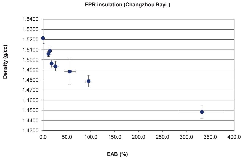
FIG. 115. Density changes in aged EPR insulation (EAB).
