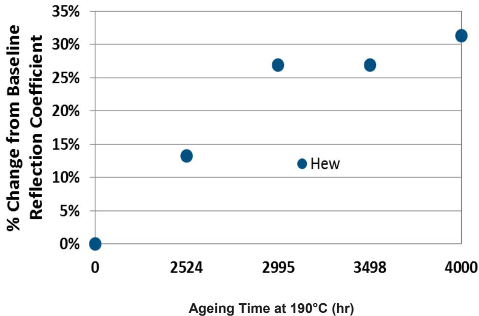
FIG. 47. FDR data for thermally aged Hew insulation (SiR).
