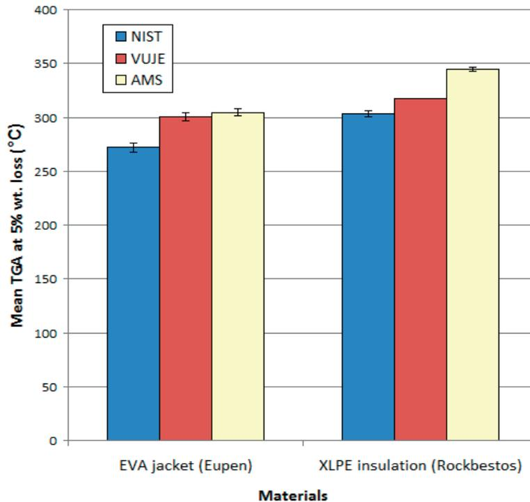
FIG. 24. Example of variability of TGA data for unaged samples.
