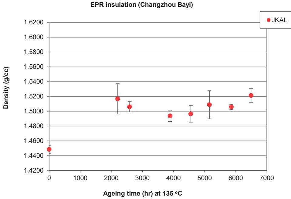
FIG. 114. Density changes in aged EPR insulation (Ageing time)
