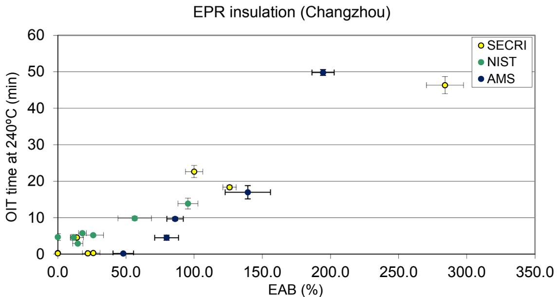
FIG. 68. Cross-plot of OIT vs. EAB for EPR insulation (Changzhou).
