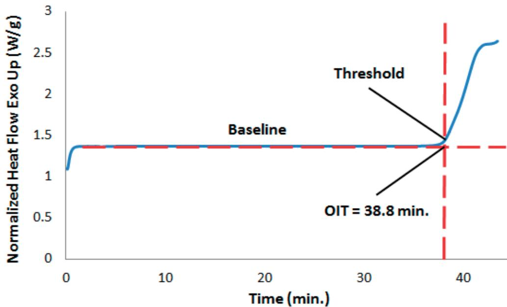
FIG. 11. OIT measurement of PE (215 °C) (Reproduced with permission courtesy of AMS corporation).
