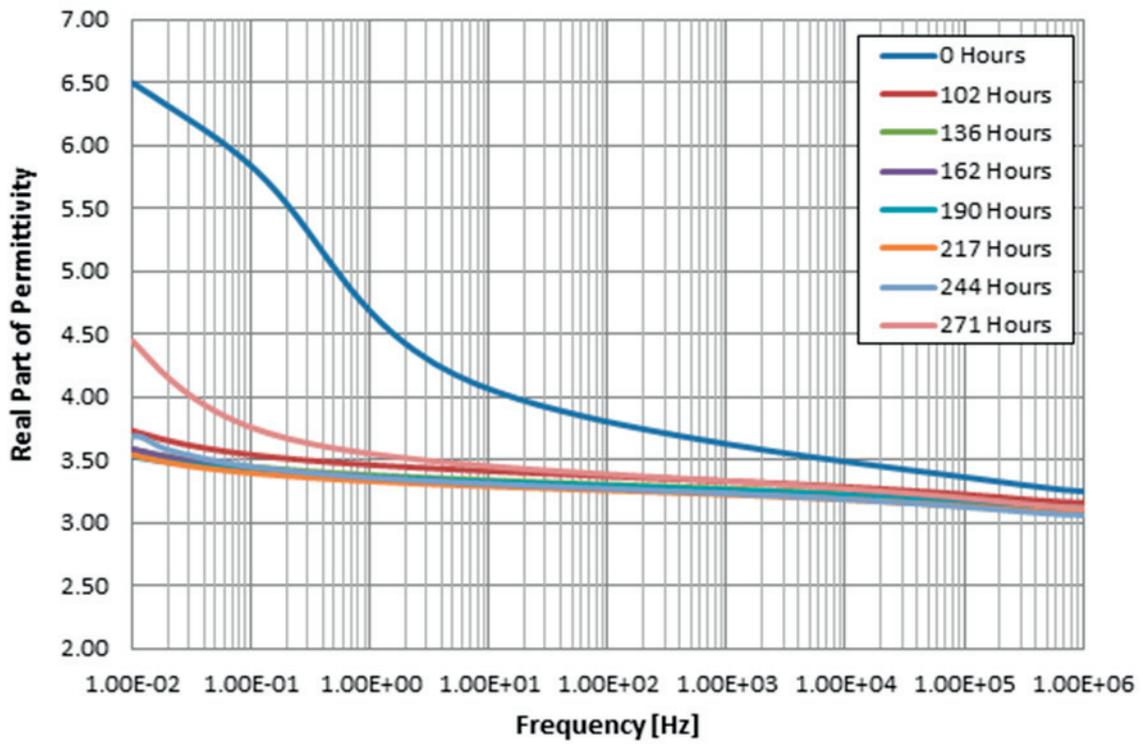
FIG. 44. Real part of permittivity vs frequency of Eupen (EPR/EVA) cable after thermal ageing at 135°C.
