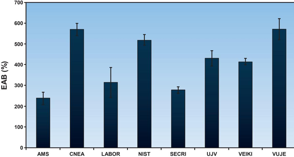
FIG. 16. Elongation data for Eupen EPR insulation (error bars are ± one standard deviation).
