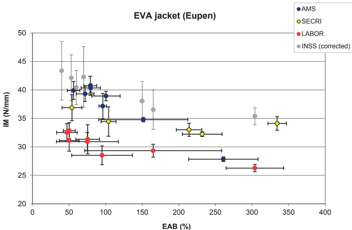
FIG. 54. Cross-plot of IM vs. EAB for EVA jacket (Eupen).
