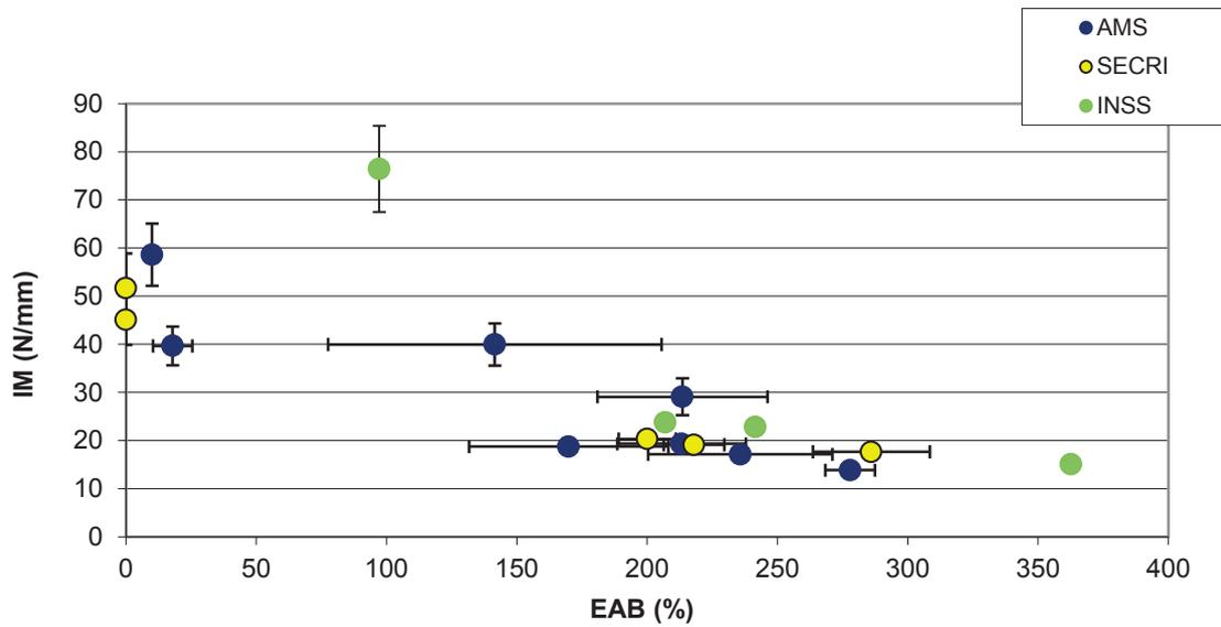
FIG. 76. Cross-plot of IM vs. EAB for XLPO insulation (Shanghai).
