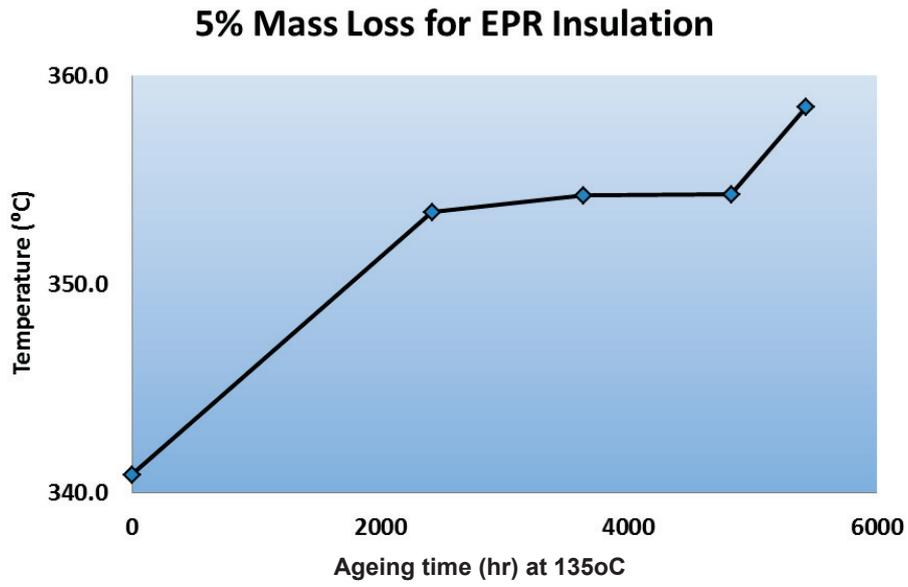
FIG. 126. Thermogravimetric analysis in case of 5% mass loss.
