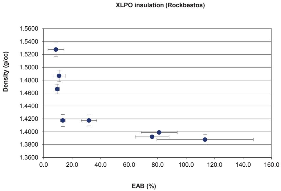
FIG. 117. Density changes in XLPO insulation (EAB).
