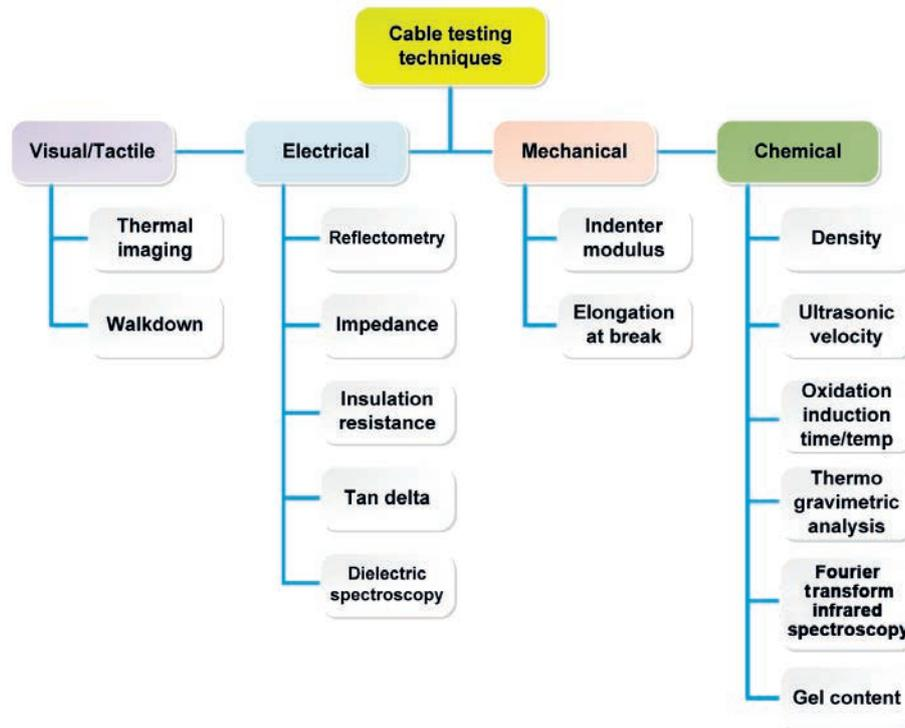
FIG. 2. Four types of testing techniques (Reproduced with permission courtesy of AMS corporation).
