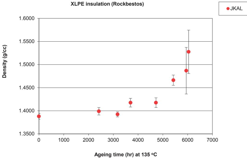
FIG. 116. Density changes in XLPE insulation (Ageing time).
