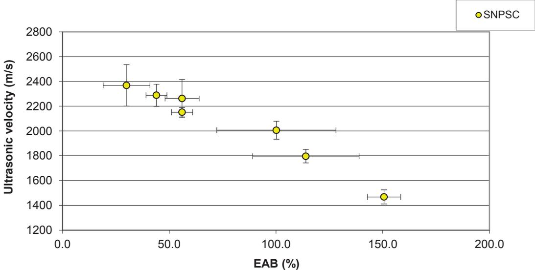
FIG. 82. Cross-plot of ultrasonic velocity vs. EAB for XLPO insulation (Shanghai).
