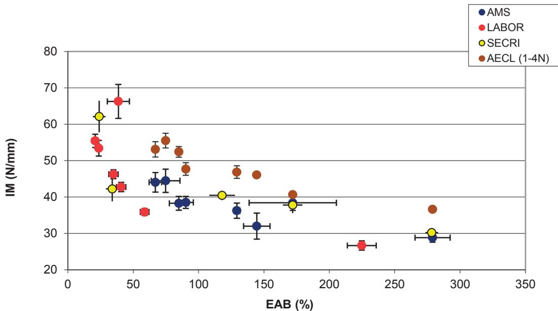
FIG. 72. Cross-plot of IM vs. EAB for EPR jacket (Changzhou).
