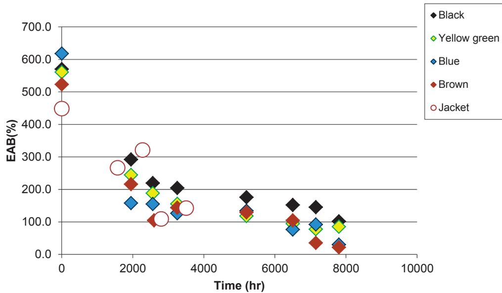
FIG. 92. EAB vs time for Eupen insulation and jacket materials.
