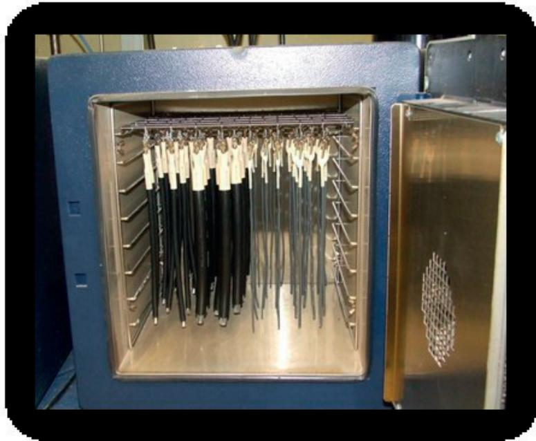
*FIG. 15. Ageing chamber with mechanical test samples (Reproduced with permission courtesy of AECL).*
