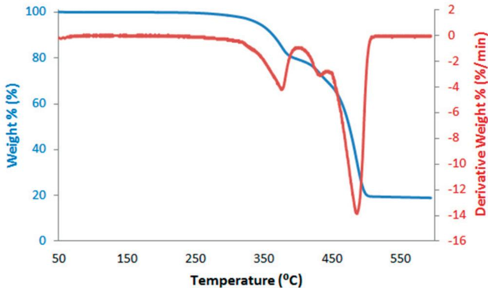
FIG. 14. TGA curve showing decomposition characteristics of the Rockbestos XLPE insulation (Reproduced with permission courtesy of AMS corporation).
