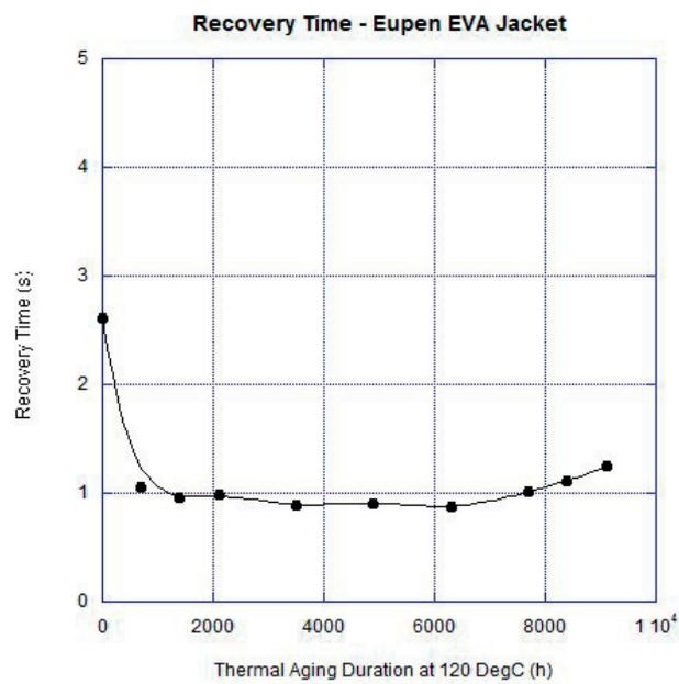
FIG. 89. IM and recovery time results for unaged and thermally aged Eupen EVA jacket samples.
