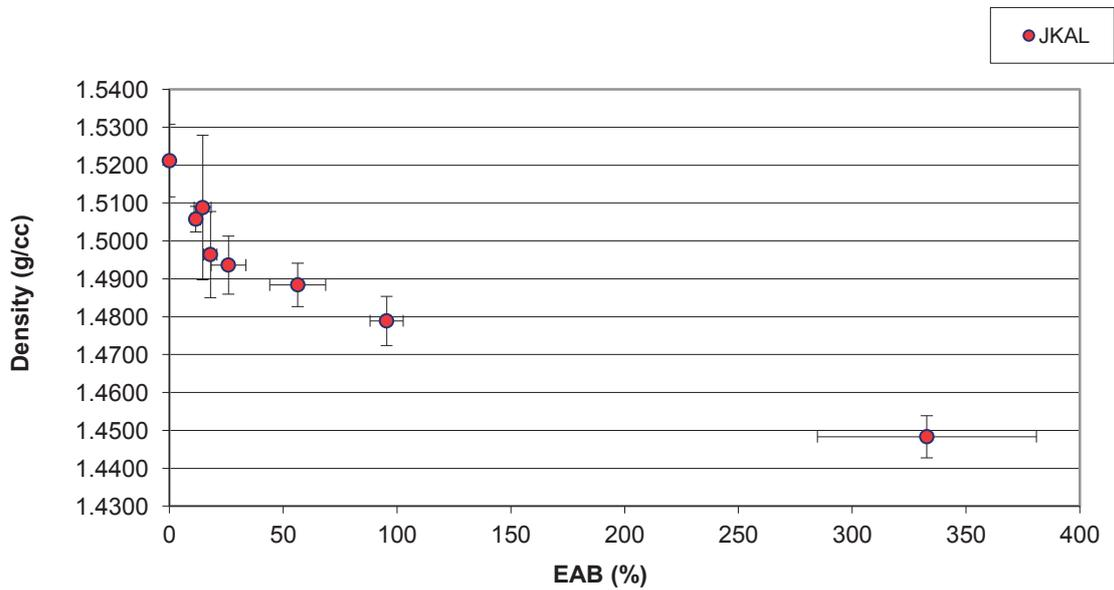
FIG. 70. Cross-plot of density vs. EAB for EPR insulation (Changzhou).
