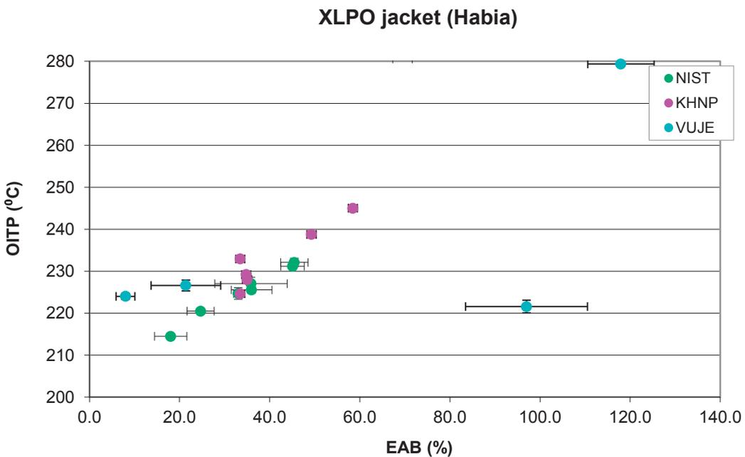
FIG. 50. Cross-plot of OITP vs. EAB for XLPO jacket (Habia).
