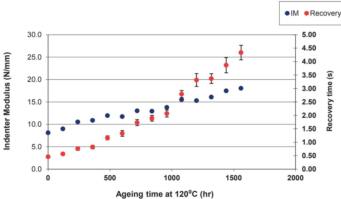
FIG. 10. Comparison of recovery time and indenter modulus measurements on CSPE (Rockbestos) jacket.
