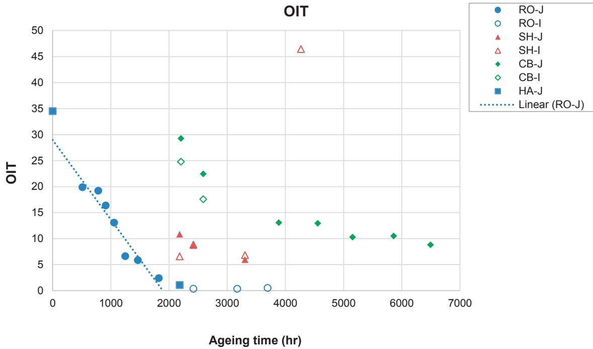
FIG. 120. OIT results for a series of thermally aged cable insulation and jackets.
