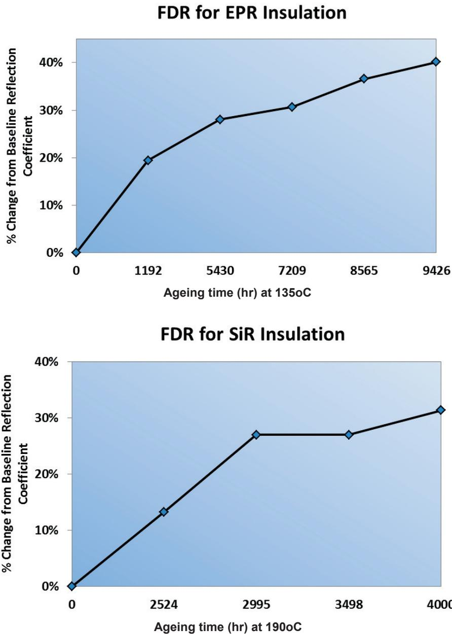
FIG. 129. Thermal ageing conclusions for TDR and FDR a) 135°C, b) 190°C.
