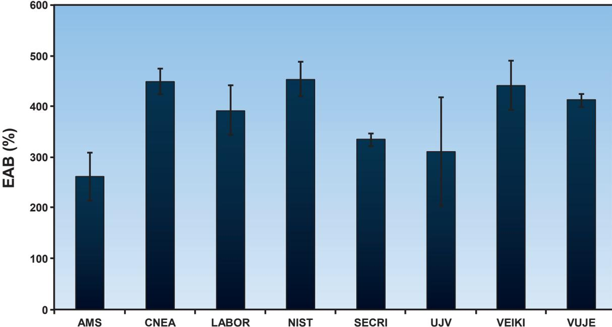
FIG. 17. Elongation data for Eupen EVA jacket (error bars are ± one standard deviation).
