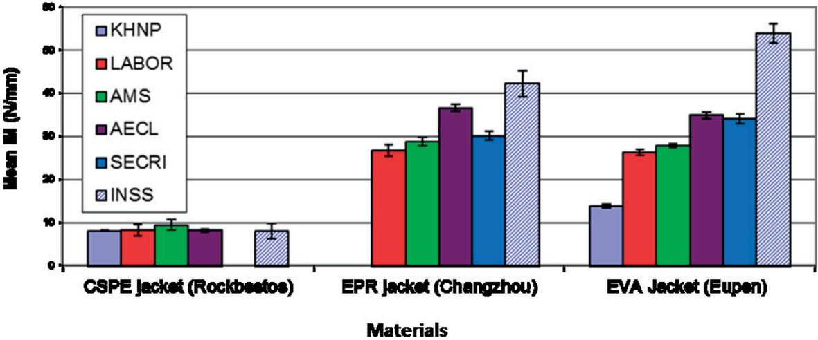
FIG. 21. Indenter data on as-received samples for jackets.
