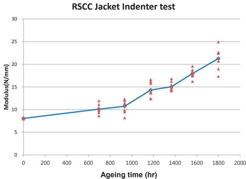
*FIG. 112. RSCC jacket indenter test results.*
