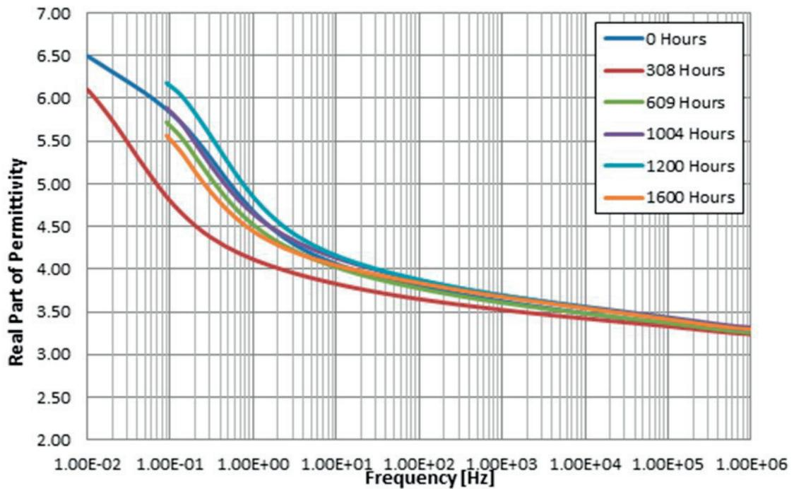
FIG. 45. Real part of permittivity vs frequency of Eupen (EPR/EVA) cable after irradiation at room temperature (0.3 kGy/h).
