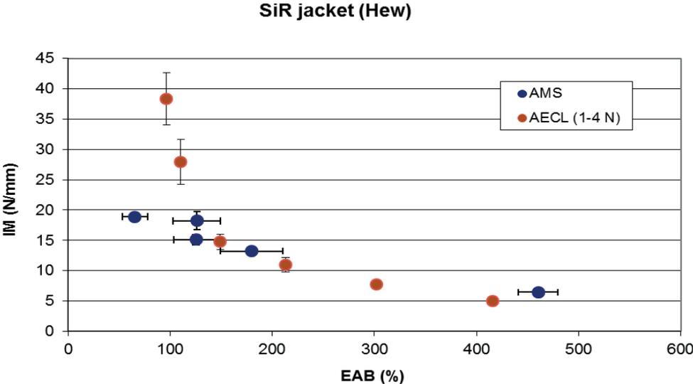
FIG. 58. Cross-plot of IM vs. EAB for SiR jacket (Hew).
