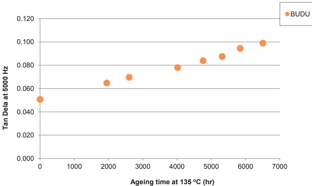
FIG. 43.  $\tan \delta$  data for thermally aged EPR insulation (Changzhou).
