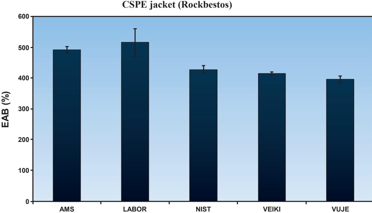
FIG. 18. Adjusted data for CSPE jacket (Rockbestos).
