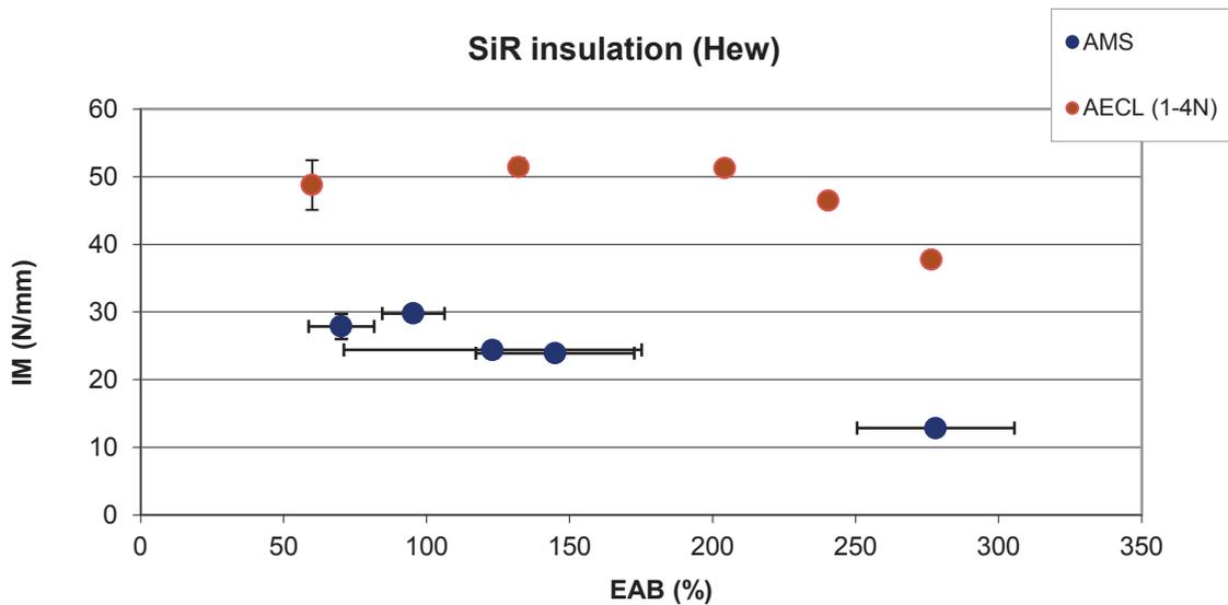
FIG. 57. Cross-plot of IM vs. EAB for SiR insulation (Hew).
