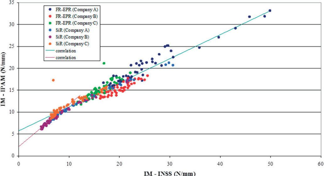
FIG. 35. Correlation curve for indenter measurements using the INSS indenter, compared with the IPAM 4 indenter.
