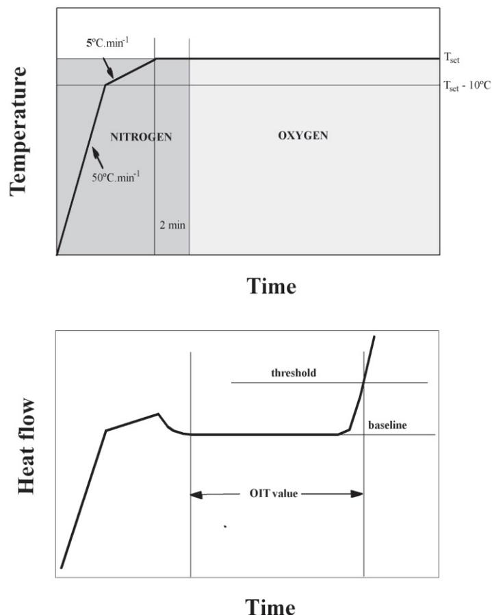
FIG. 132. Oxidation induction time measurements.
