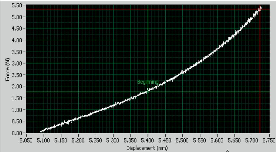
FIG. 84. Force-displacement curve for indentation of unaged Rockbestos CSPE Jacket.
