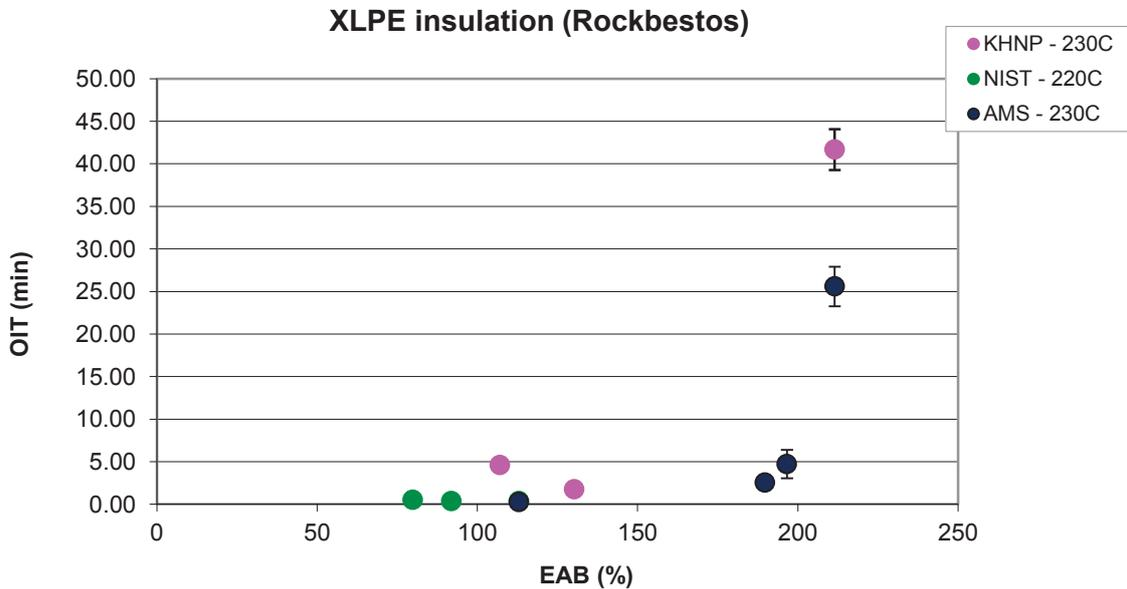
FIG. 60. Cross-plot of OIT vs. EAB for XLPE insulation (Rockbestos).
