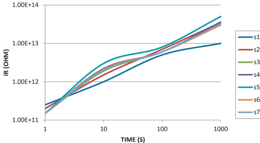
FIG. 30. Insulation Resistance Test Results for Seven Unaged Shanghai XLPO Cable Samples (reproduced with permission of Budapest University).
