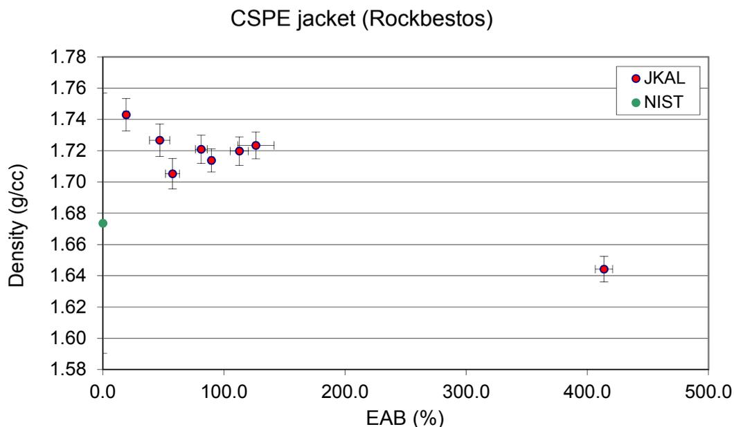
FIG. 64. Cross-plot of density vs. EAB for CSPE jacket (Rockbestos).
