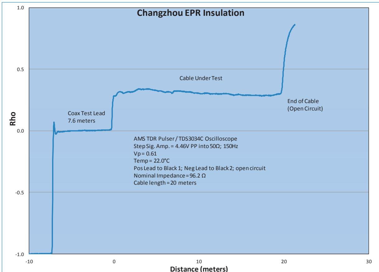
FIG. 31. TDR example data on unaged Changzhou EPR cable (reproduced with permission of AMS corporation).
