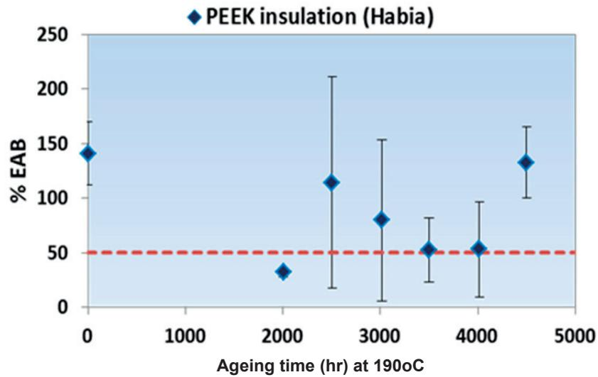
FIG. 125. PEEK insulation EAB test.
