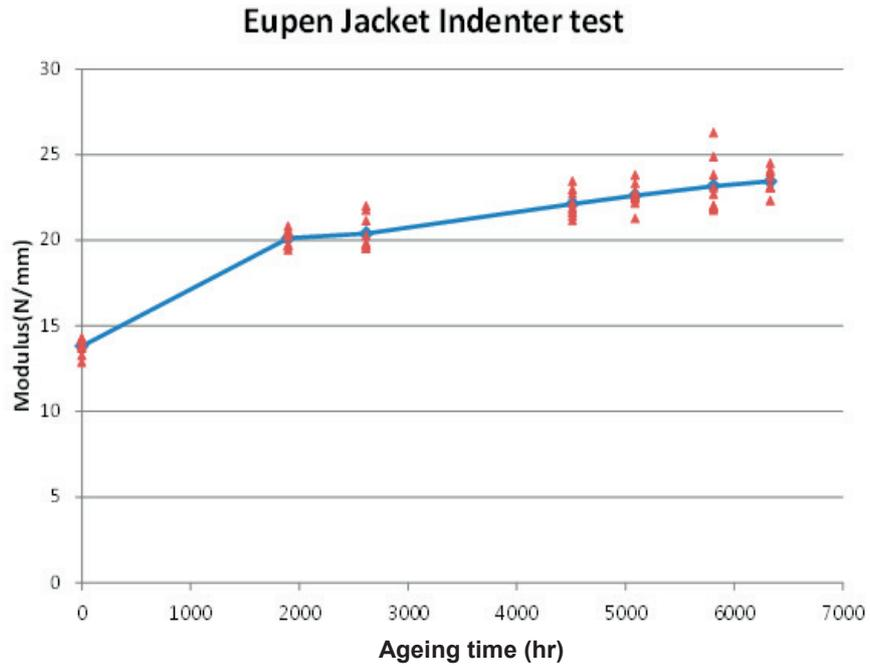
FIG. 110. Eupen jacket indenter test results
