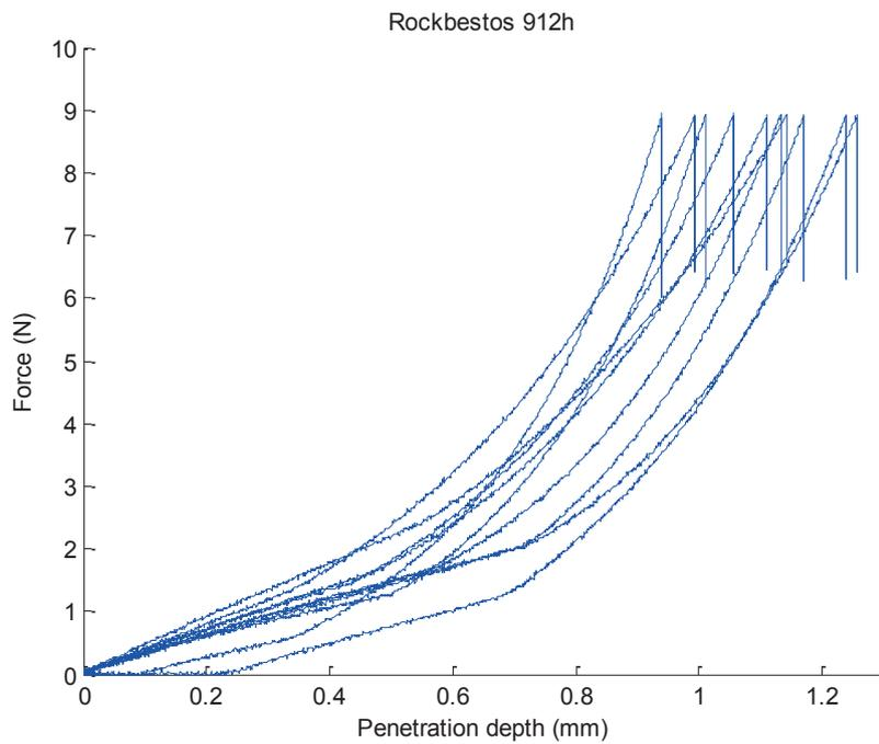
FIG. 108. Rockbestos jacket 912h without reprocessing.
