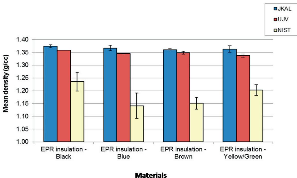
FIG. 25. Variability of density measurements (Example is for different coloured EPR insulations, Eupen).
