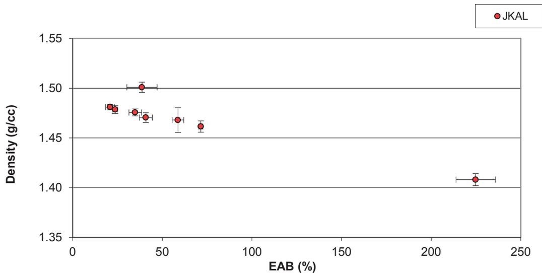
FIG. 73. Cross-plot of density vs. EAB for EPR jacket (Changzhou).
