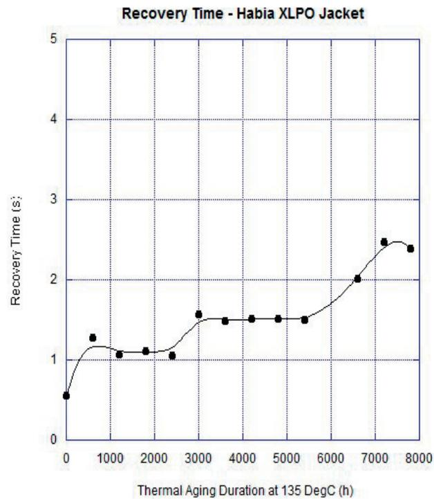
FIG. 90. IM and recovery time results for unaged and thermally aged Habia XLPO jacket samples.
