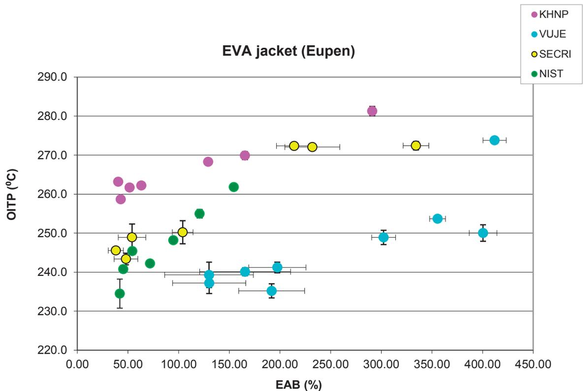
FIG. 55. Cross-plot of OITP vs. EAB for EVA jacket (Eupen).
