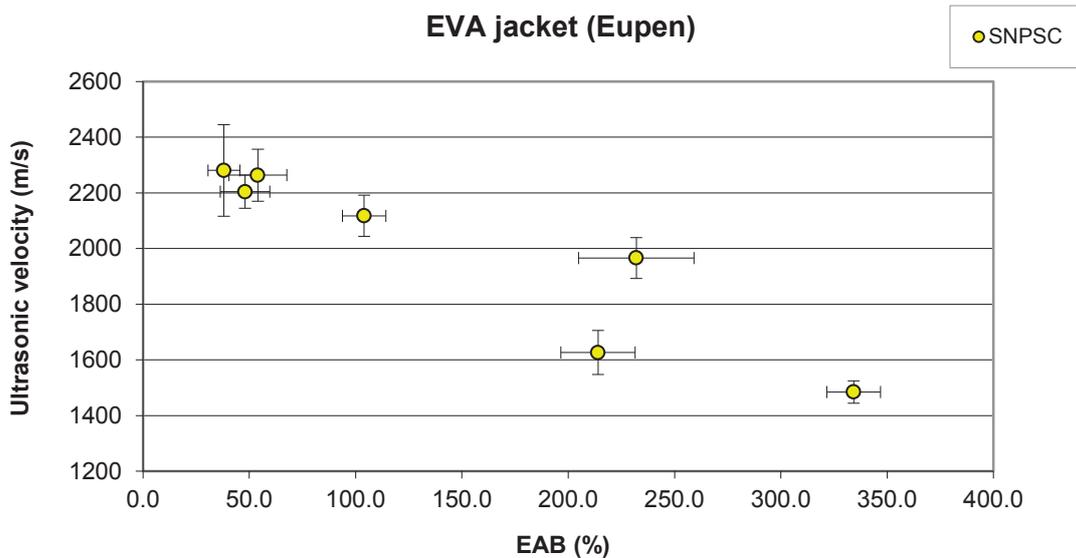
FIG. 56. Cross-plot of ultrasonic velocity vs. EAB for EVA jacket (Eupen).
