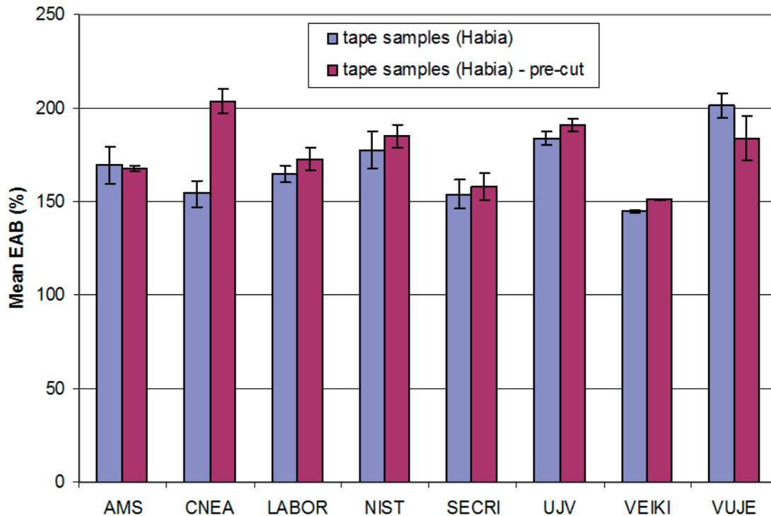
FIG. 19. EAB results for additional baseline tests on tape samples.
