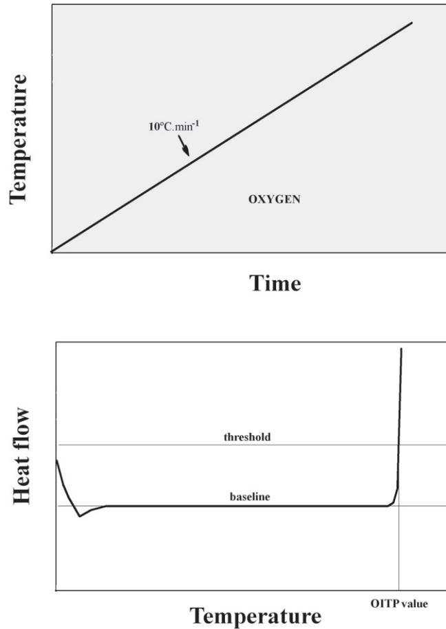
FIG. 133. Oxidation induction temperature measurements.
