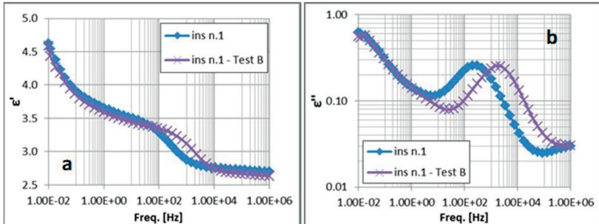
FIG. 29. University of Bologna results of dielectric spectroscopy performed on PEEK/XLPO (Habia) cable: (a) real part of permittivity. (b) imaginary part of permittivity. Frequency range  $10^{-2}$  Hz –  $10^6$  Hz.
