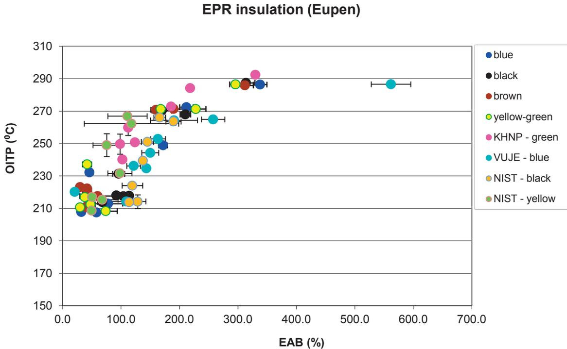
*FIG. 53. Cross-plot of OITP vs. EAB for EPR insulation (Eupen).*
