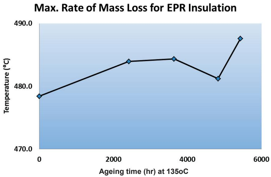
FIG. 127. Thermogravimetric analysis in case of max rate mass loss.
