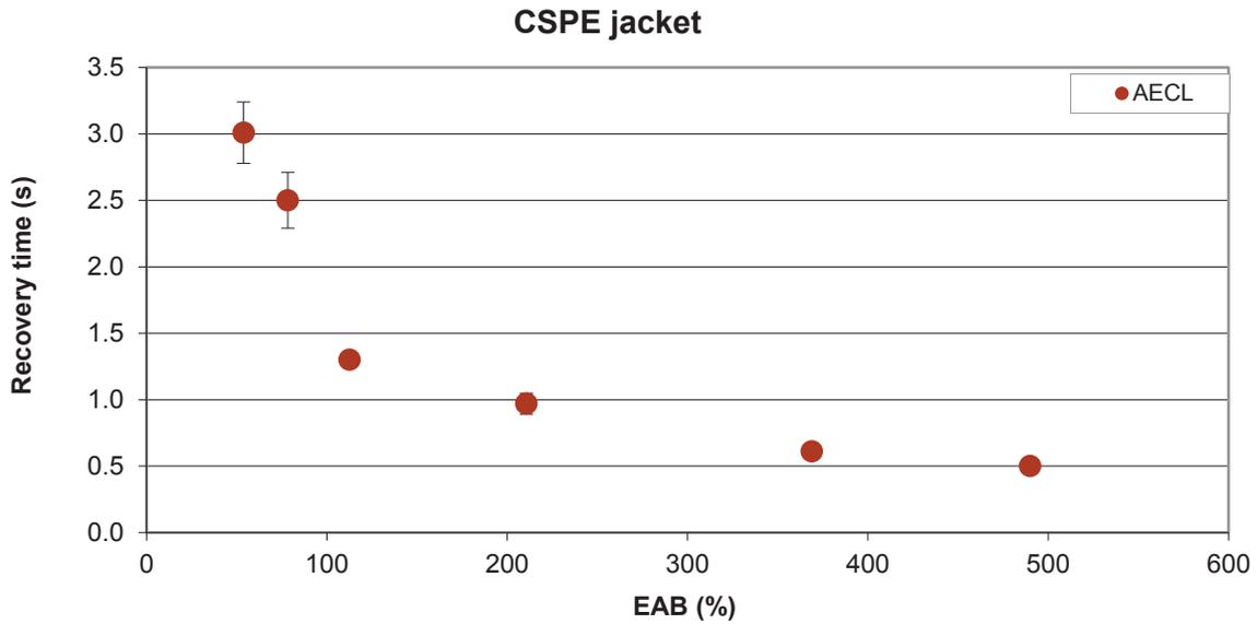
FIG. 62. Cross-plot of recovery time vs. EAB for CSPE jacket (Rockbestos).
