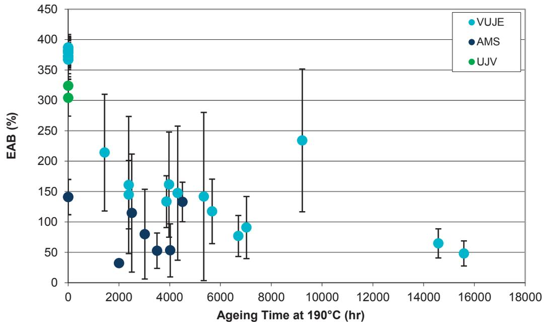
FIG. 32. EAB data for PEEK insulation.
