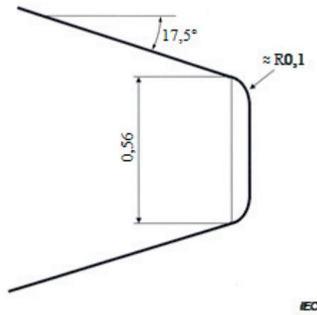
FIG. 130. Indenter (Dimensions in millimeters).
