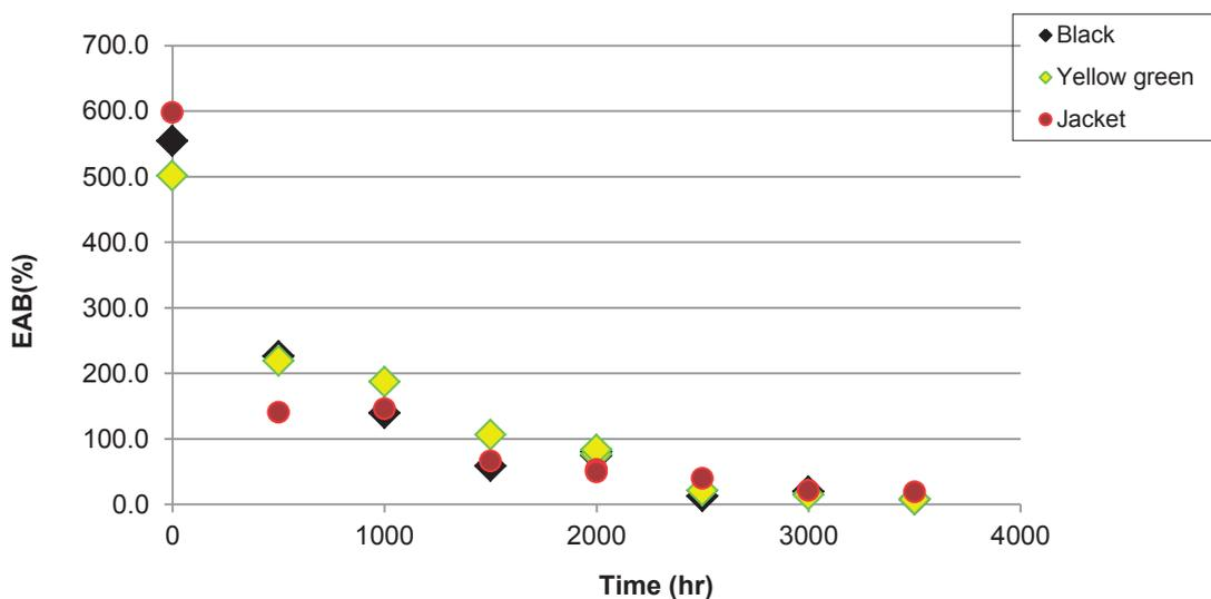
FIG. 93. EAB vs time for Hew insulation and jacket materials.
