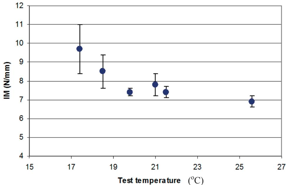
FIG. 36. Temperature variation of IM for EPR insulation.
