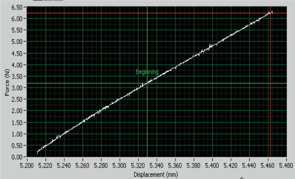
FIG. 83. Force-displacement curve for indentation of unaged Shanghai XLPO jacket.
