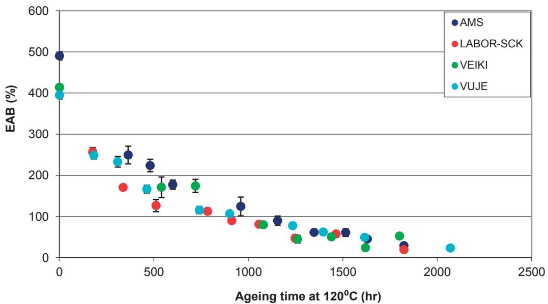
FIG. 34. EAB data for thermally aged CSPE jacket (Rockbestos).
