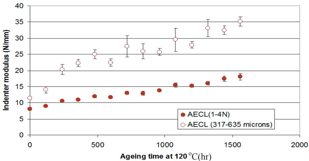
FIG. 38. Comparison of IM values for thermal ageing using 1-4 N force range and 317-635 micron depth range for the CSPE jacket (Rockbestos).
