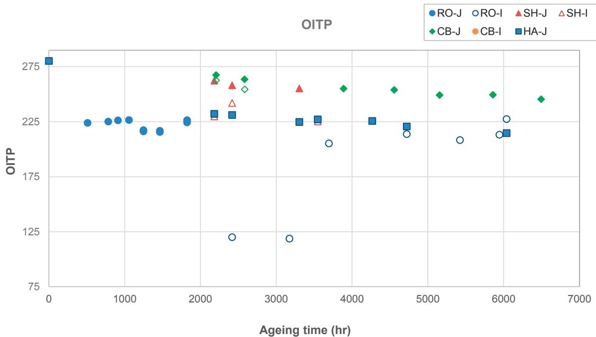
FIG. 121. OITP results for a series of thermally aged cable insulation and jackets.
