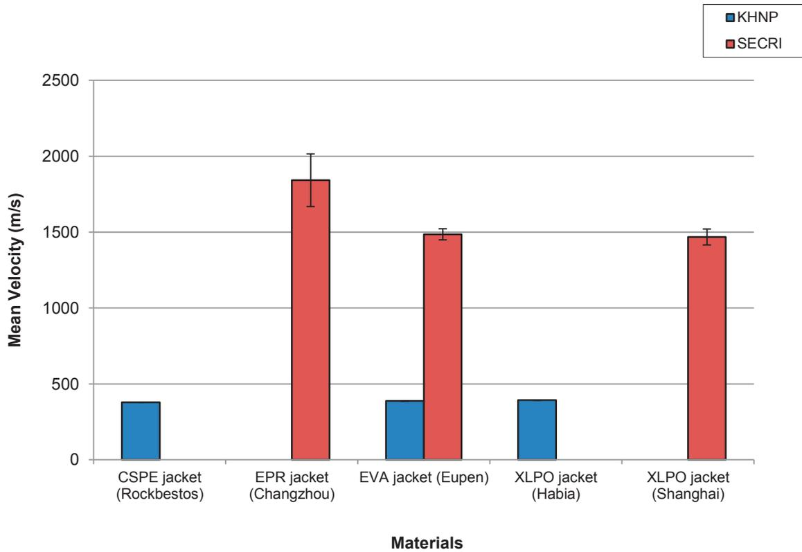
FIG. 27. Ultrasonic velocity for as-received samples.
