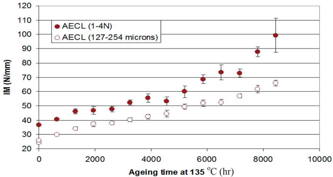
FIG. 37. Comparison of IM values for thermal ageing using 1-4 N force range and 127-254 micron depth range for the EPR jacket (Changzhou).
