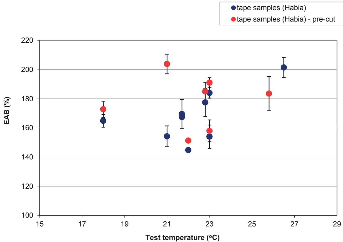
FIG. 20. Temperature variation of EAB for the Habia tape samples (each data point is for a different lab).
