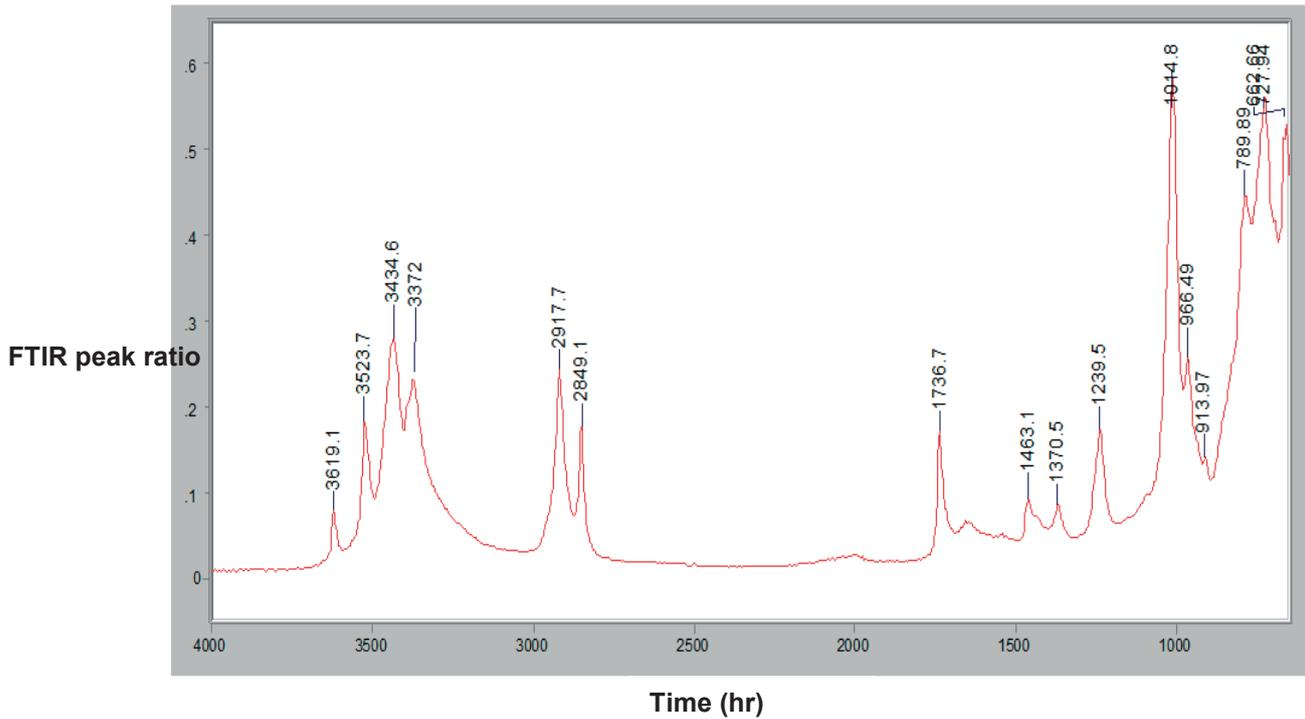
FIG. 13. Attenuated FTIR spectrum for the Habia XLPO jacket (Reproduced with permission courtesy of Korea Hydro Nuclear Power Company).
