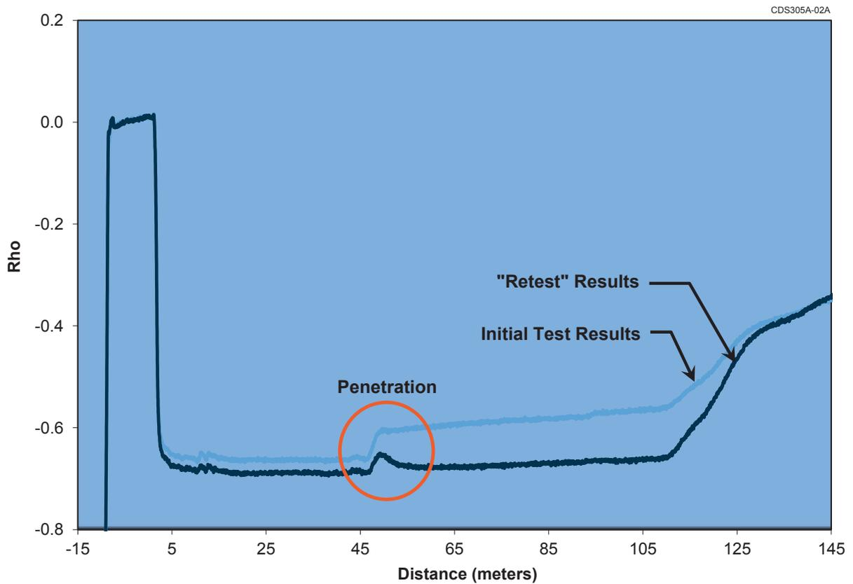
FIG. 4. TDR trace of NI circuit indicating a high impedance connection (initial test results) compared to TDR trace after the fault was repaired ('retest' results) (Reproduced with permission courtesy of AMS corporation).
