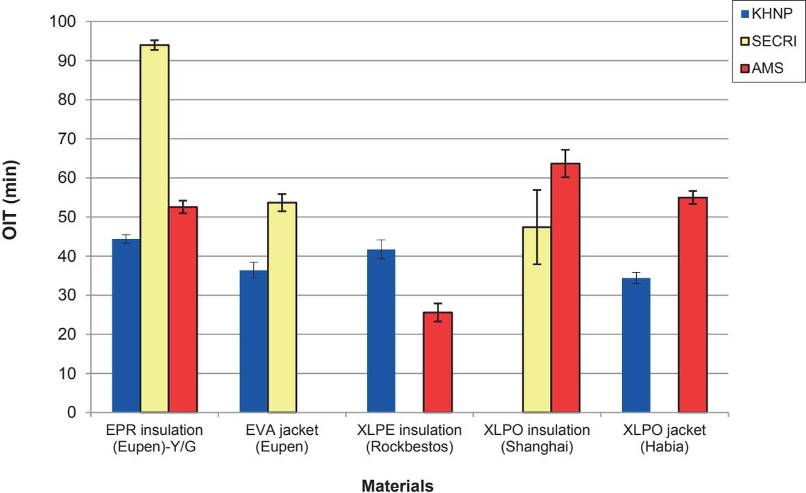
FIG. 22. Example of variability of OIT data for unaged samples.
