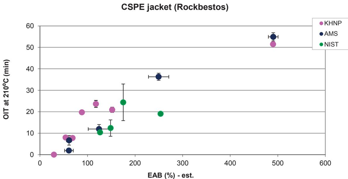
FIG. 63. Cross-plot of OIT vs. EAB for CSPE jacket (Rockbestos).
