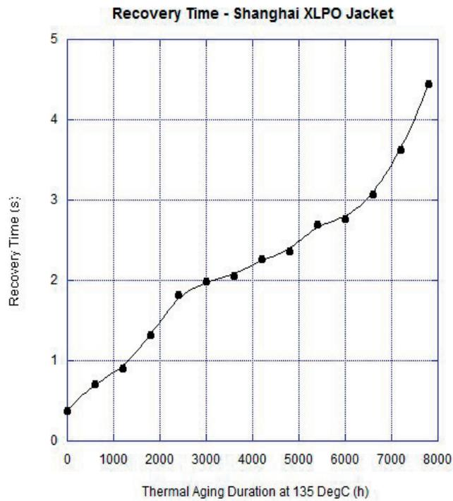
FIG. 91. IM and recovery time results for unaged and thermally aged Shanghai XLPO jacket samples.
