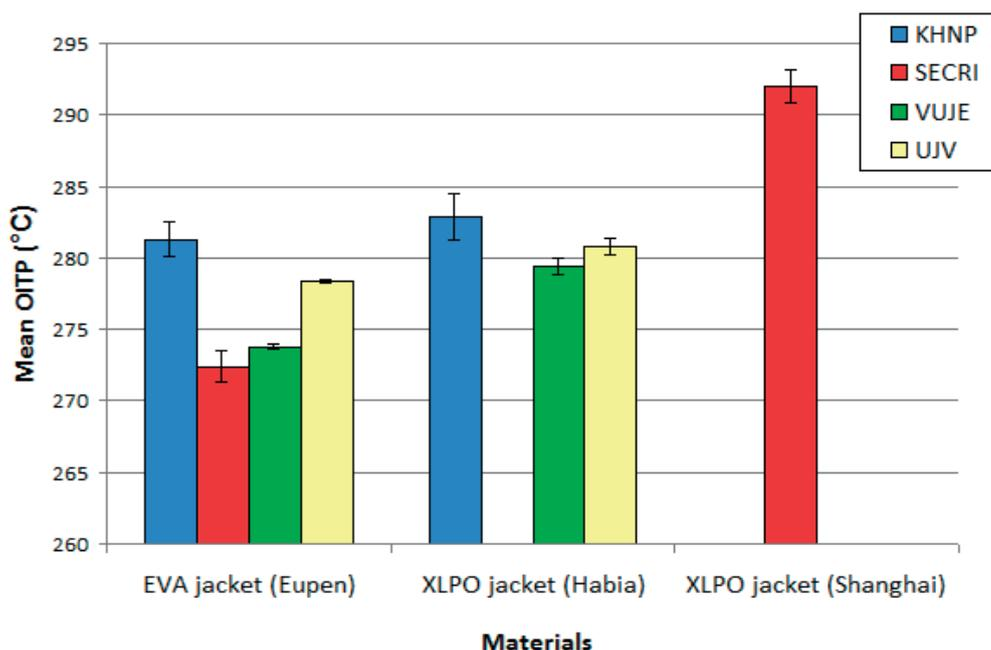
FIG. 23. Example of variability of OITP data for unaged samples for jackets.
