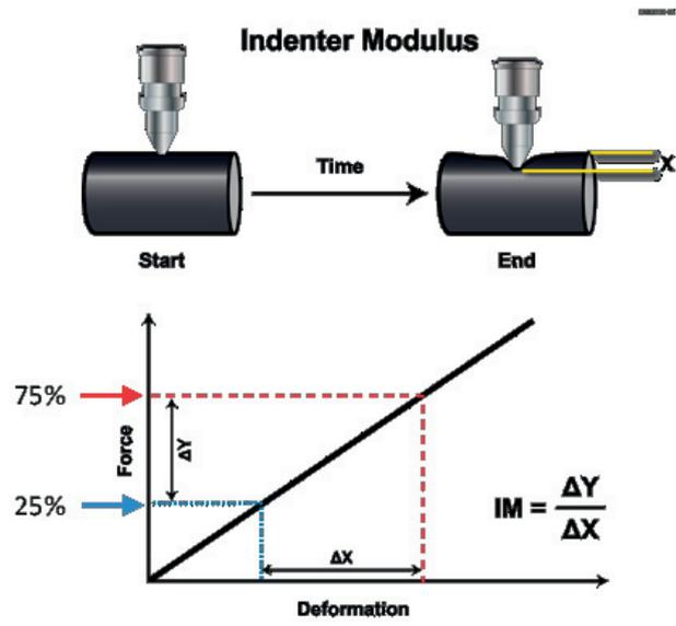
FIG. 7. Conceptual diagram showing the principle of the indenter modulus measurement (Reproduced with permission courtesy of AMS corporation).
