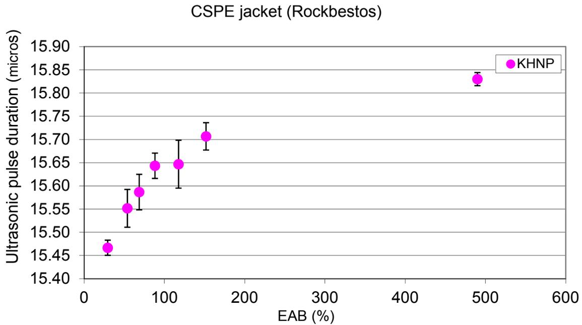
FIG. 65. Cross-plot of ultrasonic velocity vs. EAB for CSPE jacket (Rockbestos).
