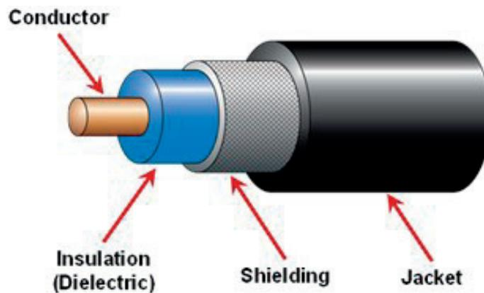
FIG. 1. Schematic of a typical cable (Reproduced with permission courtesy of AMS corporation).
