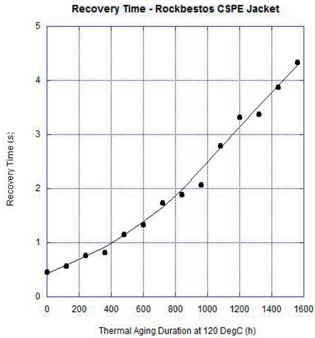
FIG. 87. IM and recovery time results for unaged and thermally aged Rockbestos CSPE jacket samples.
