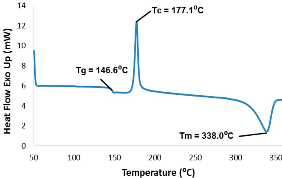
FIG. 12. DSC Curve showing transition temperatures of PEEK (Reproduced with permission courtesy of AMS corporation).
