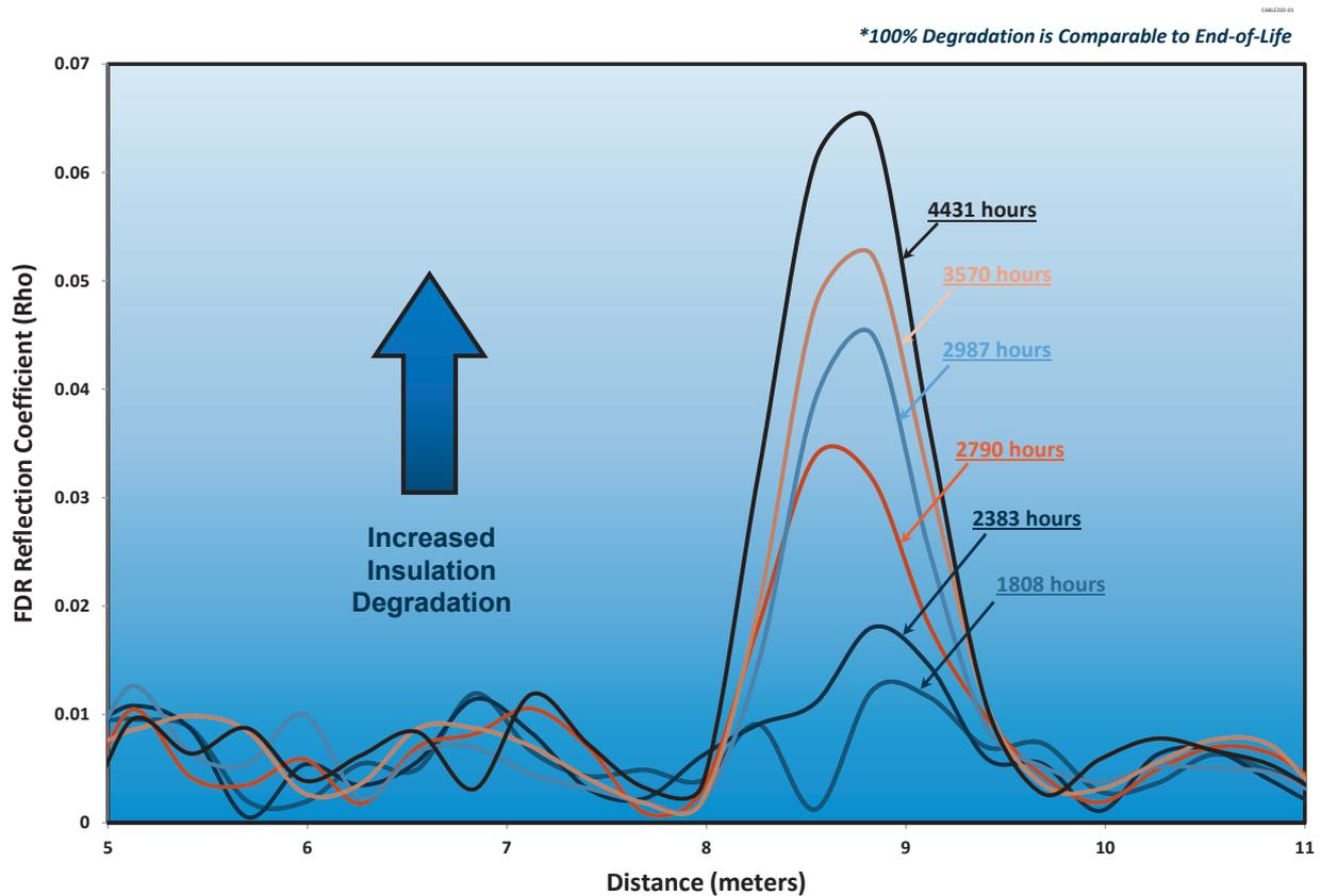
FIG. 5. Results of FDR testing of an EPR insulated cable after thermal ageing (Reproduced with permission courtesy of AMS corporation).
