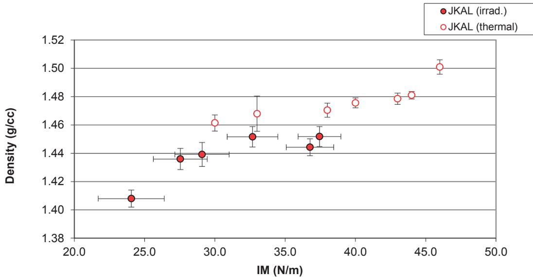
FIG. 74. Cross-plot of density vs. IM for EPR jacket (Changzhou Bai).
