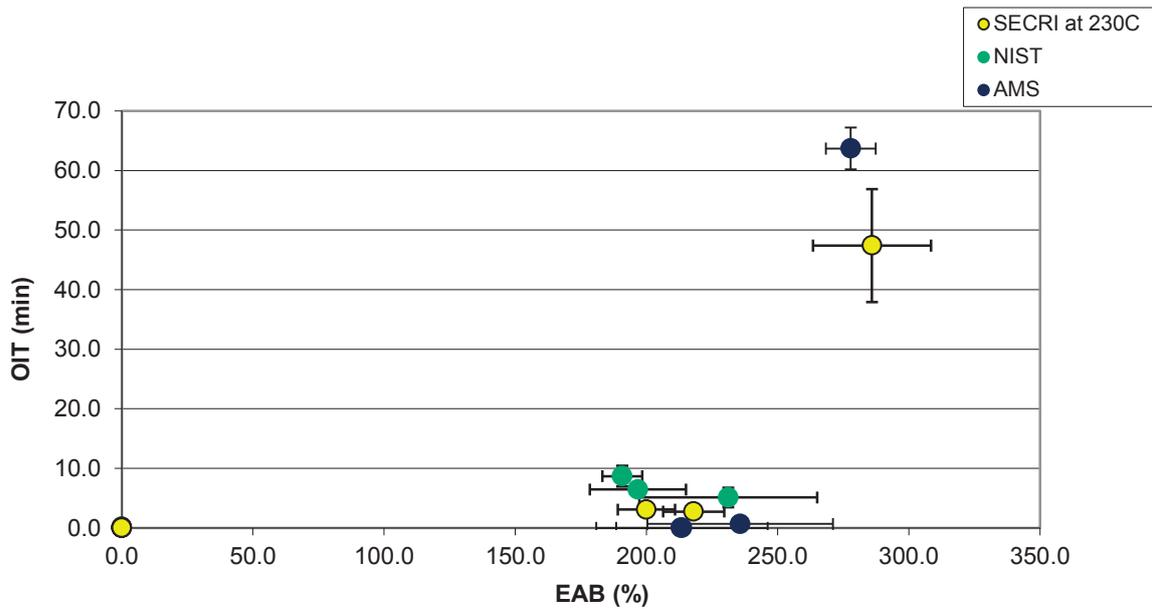
FIG. 77. Cross-plot of OIT vs. EAB for XLPO insulation (Shanghai).
