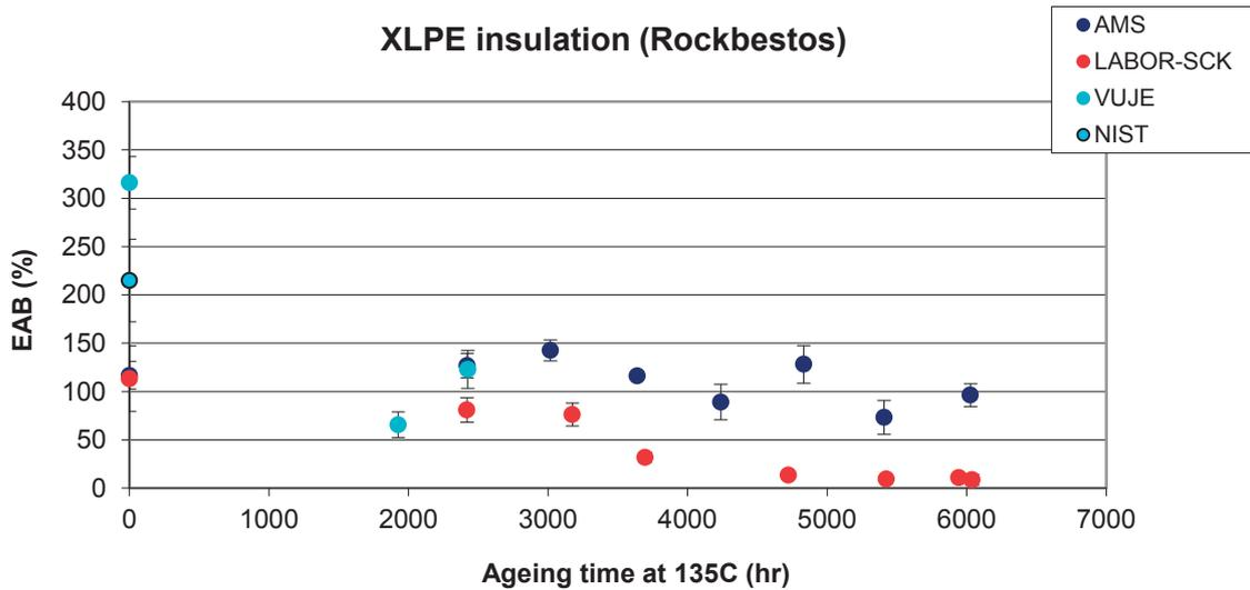
FIG. 59. EAB data for XLPE insulation (Rockbestos).
