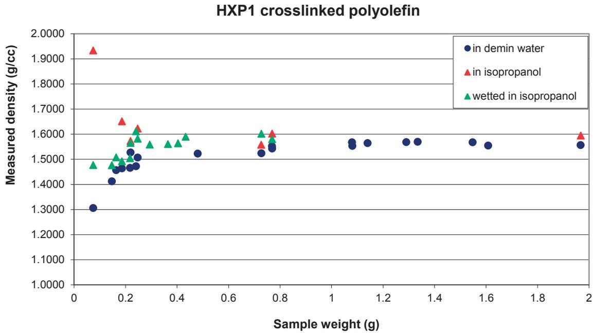
FIG. 113. Effect of sample size on density measurements.
