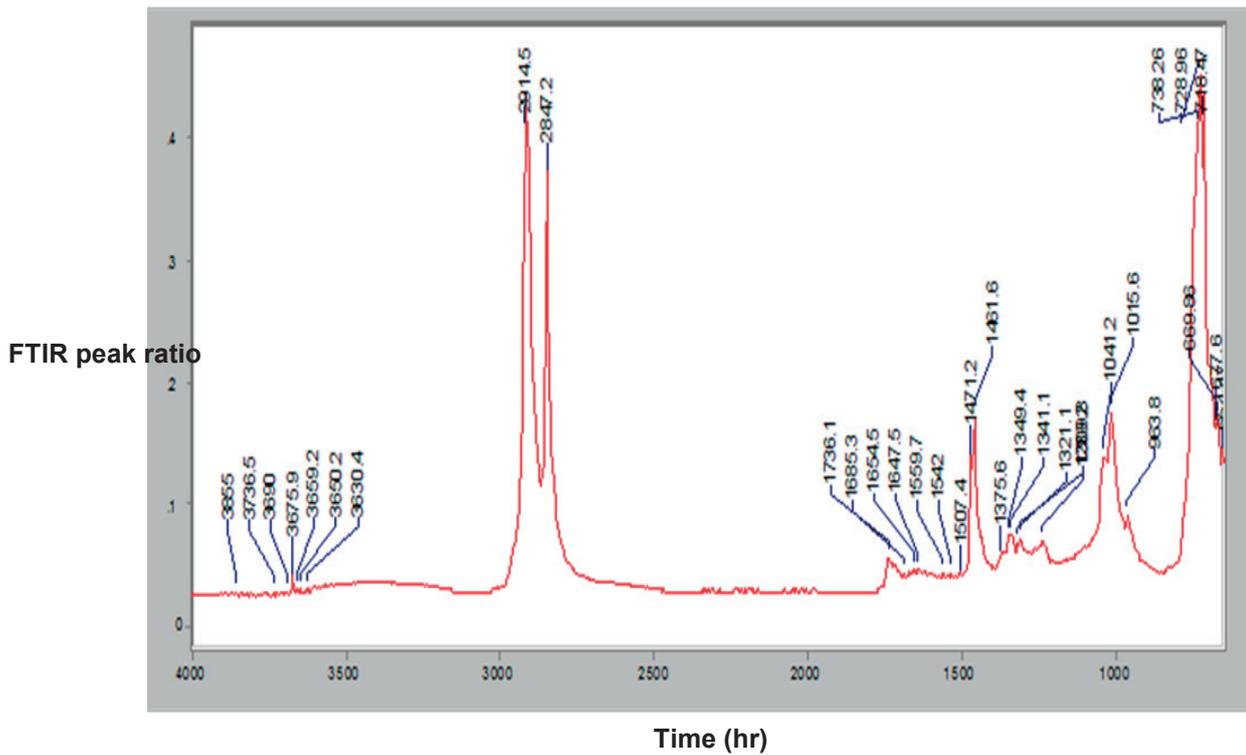
FIG. 26. Example of an FTIR spectrum for XLPE insulation (Rockbestos).
