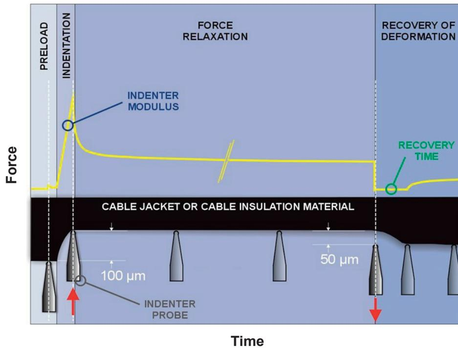
FIG. 9. Measurement procedure for recovery time (Reproduced with permission courtesy of AECL).
