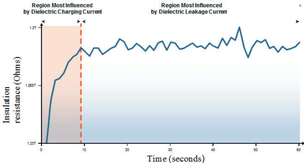
FIG. 6. Insulation resistance (IR) curve for a CRDM cable in NPP (Reproduced with permission courtesy of AMS corporation).
