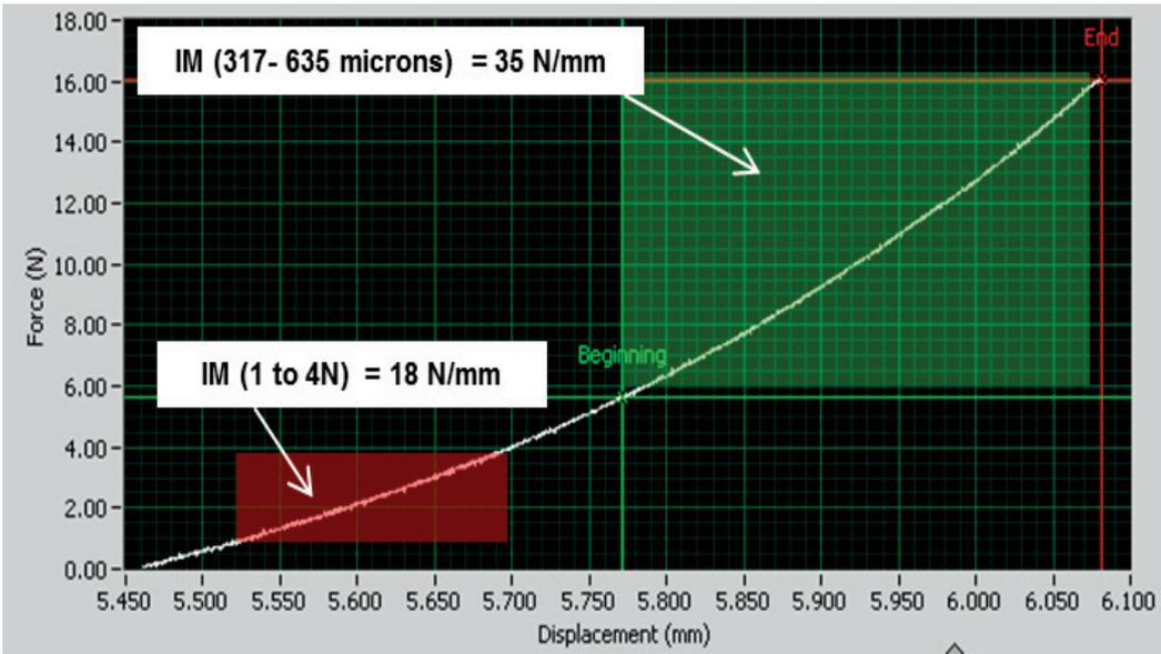
FIG. 86. 1560h thermally aged Rockbestos CSPE jacket.
