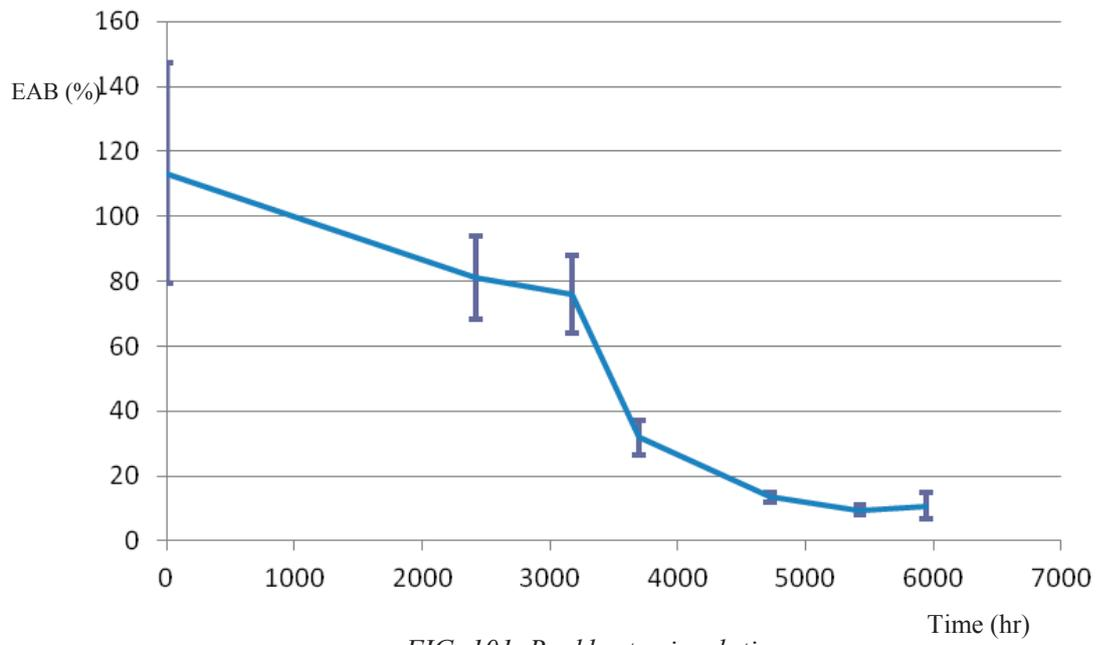
FIG. 101. Rockbestos insulation.
