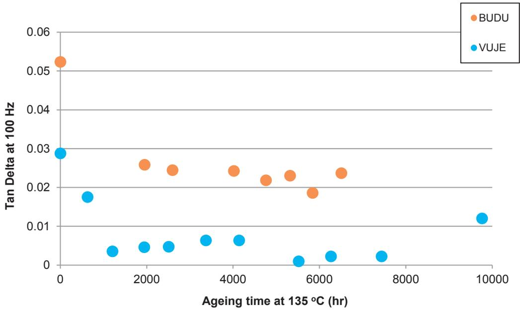
FIG. 42.  $\tan \delta$  data for thermally aged EPR insulation (Eupen) black/all.
