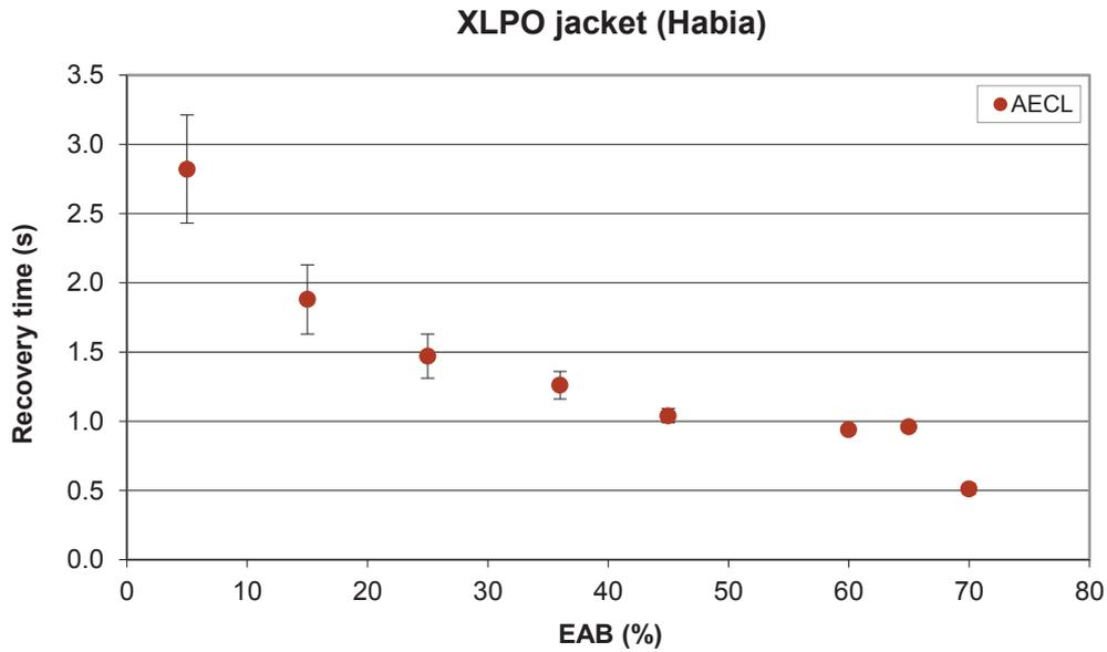
FIG. 49. Cross-plot of recovery time vs. EAB for XLPO jacket (Habia).
