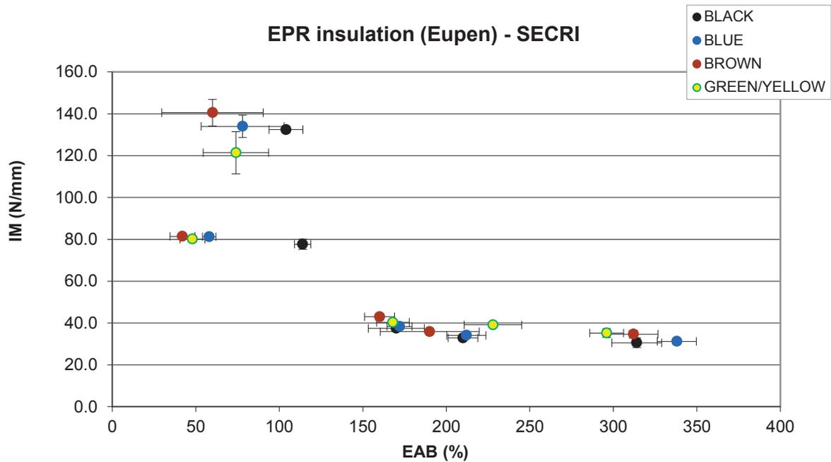
FIG. 52. Cross-plot of IM vs. EAB for EPR insulation (Eupen) – Shanghai Electric Cable Research Institute (SECRI) data.
