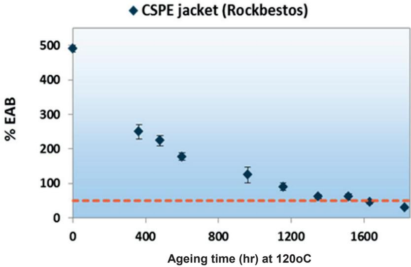
FIG. 124. CSPE jacket EAB test.
