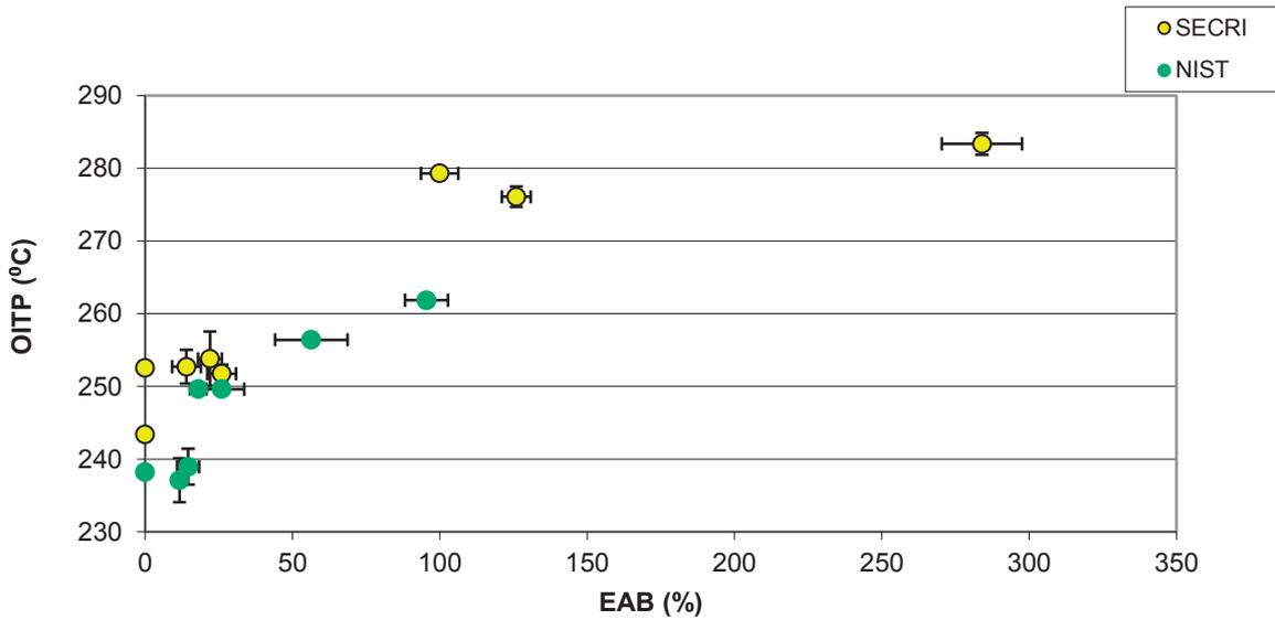
FIG. 69. Cross-plot of OITP vs. EAB for EPR insulation (Changzhou).
