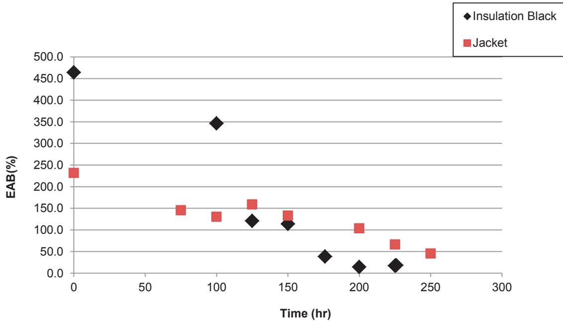
FIG. 94. EAB vs time for Shanghai insulation and jacket material.
