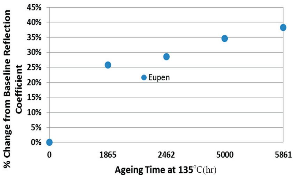
FIG. 46. FDR data for thermally aged Eupen insulation (EPR)
