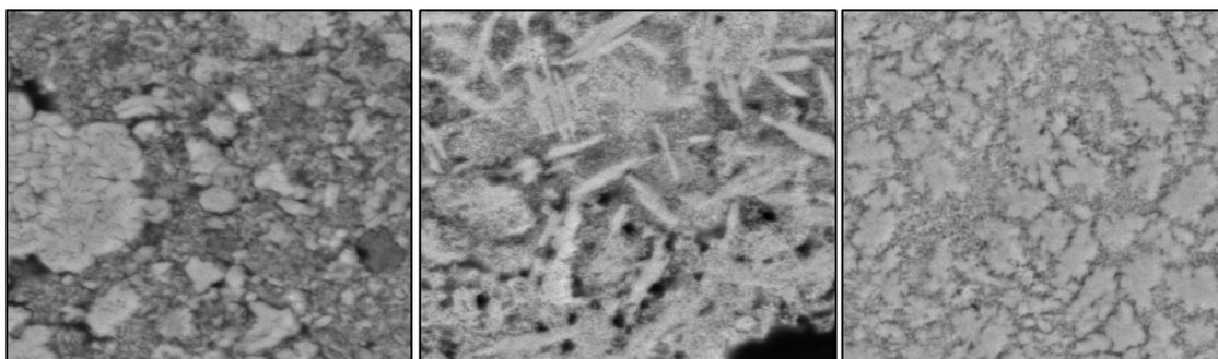
FIG 1. SEM images of epoxy mounted, polished and carbon coated UOC samples from Beverley (left), Ranger (centre) and Olympic Dam (right) at  $\times 1500$  magnification ( $15\ \mu\text{m}$  image width).
