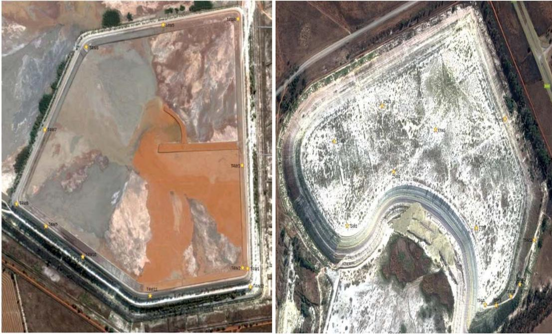
FIG. 2: Aerial photographs; on the left is the tailing dam showing the paddocks and on the right is the disused tailing dam. Yellow marks represent sampling points.
