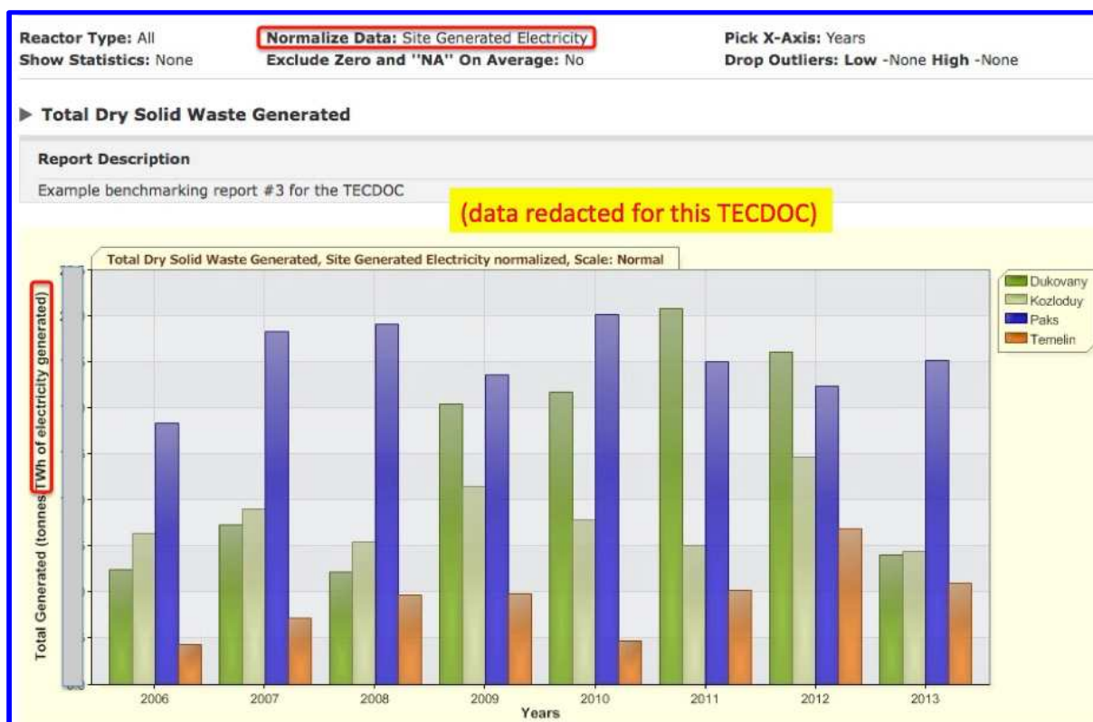
FIG. 21. "Must Have Report #3": Total Dry Solid Waste Generated.
