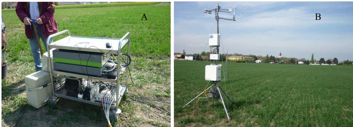
FIG. 1. (A) Picarro L1115-i water isotope analyzer connected to its 6 air intakes; (B) 3-D sonic anemometer and LI-COR 7500 water vapour sensor mounted at 2.5 m at top of mast.
