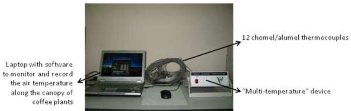
FIG. 3. ‘Multi-temperature’ device constructed by the INST’s engineers which functions like a psychrometer used for determination of the air humidity in meteorological observations.
