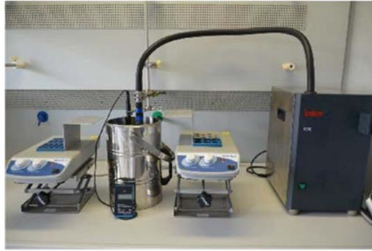
*FIG. 3. The vacuum distillation setup consists of heating blocks, Dewar cold bath, an immersion cooler and an electronic thermometer to monitor temperature of the cold bath.*
