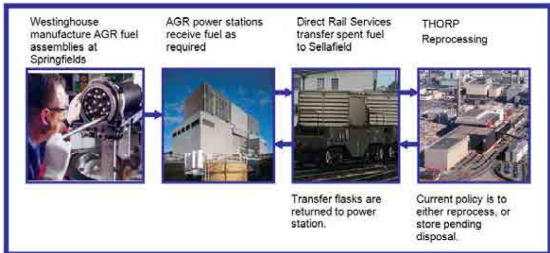
FIG. XIV-3. Interfaces between the front end and the back end of the AGR fuel cycle.
