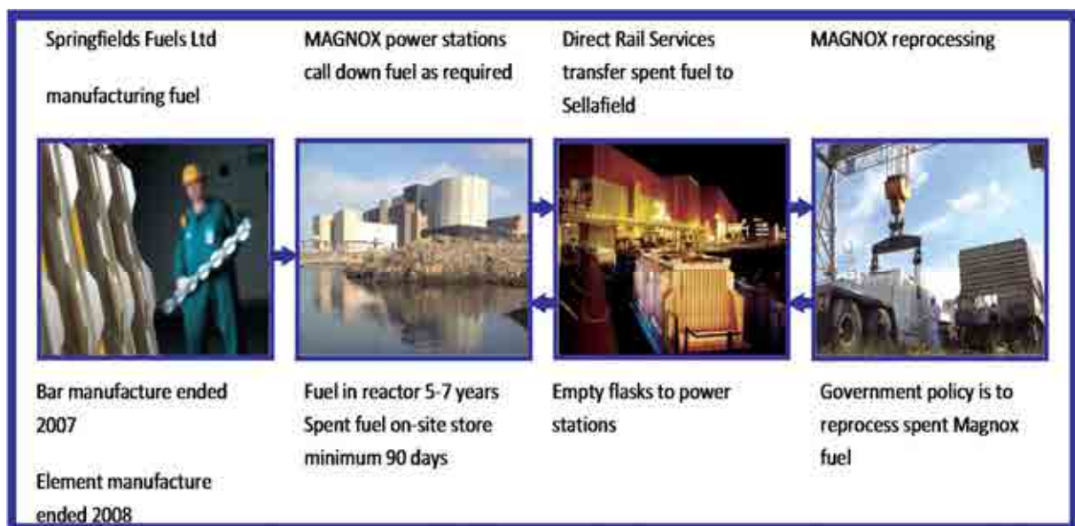
FIG. XIV-3.1. Interface between the front end and the back end of the MAGNOX fuel cycle.
