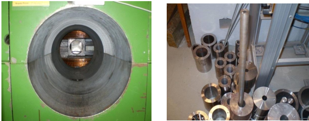
FIG. 3. The iron frontal wall and the largest collimator aperture (left panel); collimator inserts of different sizes (right panel).
