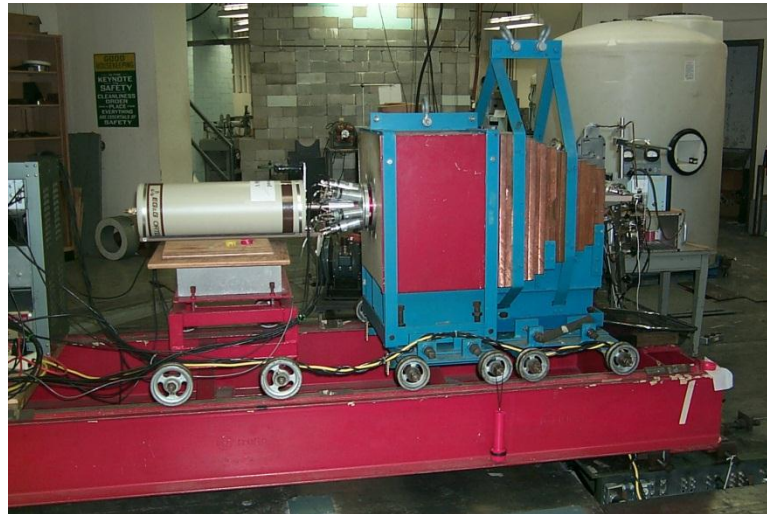
FIG. 8. Singles \gamma ray measurement configuration. The carriage is shown at 90^\circ to the beam direction.
