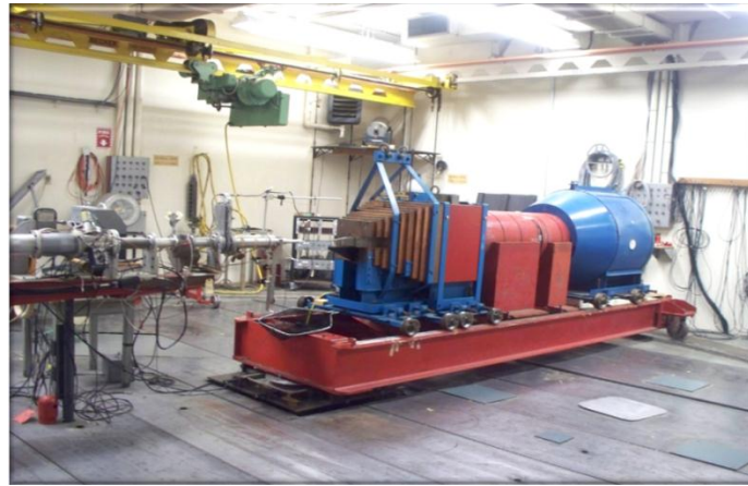
FIG. 3 Neutron time-of-flight end station pictured at \theta = 0^\circ . Copper is an effective shield for both neutrons and \gamma rays and is visible in the section nearest the gas cell [8]. The remaining red collimation is Li_2CO_3 -loaded paraffin with collimation rings. The 'MAIN' detector is housed in the last blue shield which is filled with loaded paraffin containing several Cd and Pb concentric rings to reduce thermal neutrons and photons in the vicinity of the detector.
