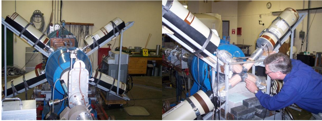
FIG. 9. Two views of the \gamma - \gamma coincidence configuration. The left photo shows the arrangement from the beam-line view. The blue collimator is placed over the gas cell and forms a \sim 2 cm diameter neutron “collimator”. A 10 cm thick lead wall just after the collimator attenuates \gamma rays generated in the collimator. Four HPGe detectors follow and are operated in a \gamma - \gamma coincidence arrangement. The right photo shows the arrangement from the detector viewpoint. The sample of interest is placed along the flux in the center of the 4 detectors.
