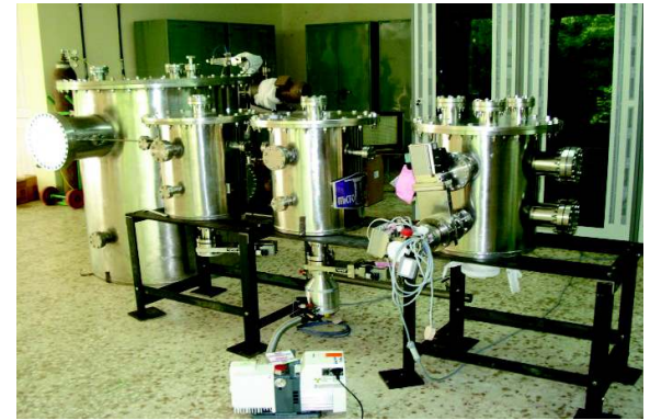
Pellet injector under commissioning
