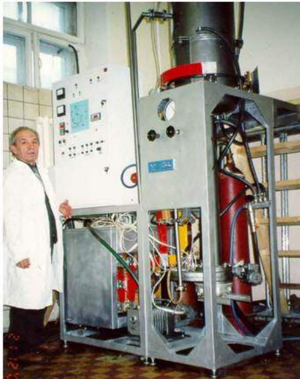
Gravity-type furnace for production of microspheres
