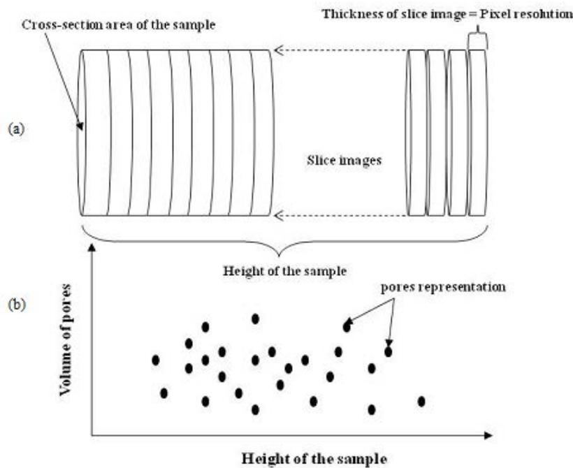
FIG. 9. (a) Schematic diagram showing the constitution of sample height from slice images and (b) presentation of pore size distribution as a function of sample height
