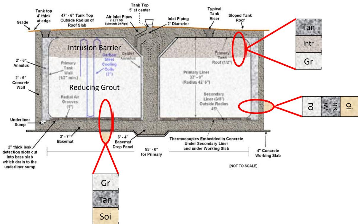
FIG 16. One dimensional conceptual model constructed to evaluate cementitious barrier performance associated with a waste tank.
