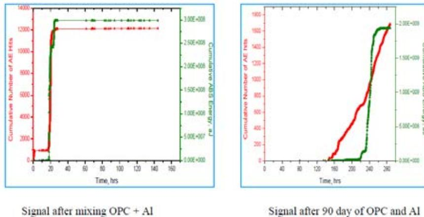
FIG. 11. Cumulative number of AE hits and associated ABS energy detected during the AE monitoring of the BFS/OPC samples with encapsulated Al.
