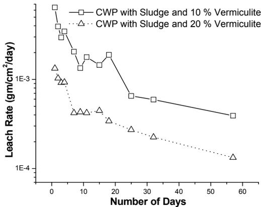
Leach rate of CWP prepared from sludge with various concentrations of Vermiculite
