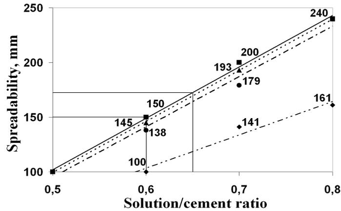
FIG. 1. Spreadability of fresh mixes, mm of slump Numbers on the figure refer to mixe designations. Spreadability relation of cement grouts of composition: water, portland cement, bentonite (■), solution of NaNO<sub>3</sub> with concentration of 300 g/l, PC, bentonite (▲), LRW of SUE SIA "Radon" with concentration of 250 g/l, PC, bentonite (●),LRW of Kalinin NPP with concentration of 500 g/l, PC, bentonite (◆) of the solution/cement ratio.
