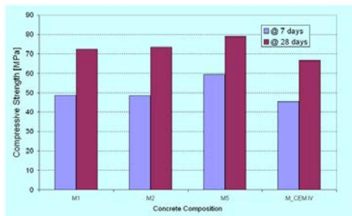
FIG. 6. Results of compressive strength measurements for 4 compositions for 2 time periods.
