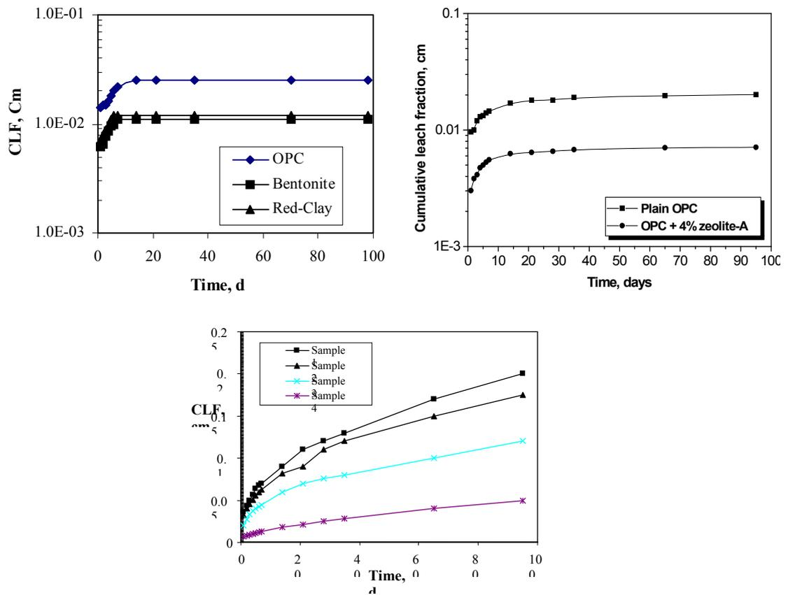
FIG. 4. Cumulative leached fraction from modified cement matrices.
