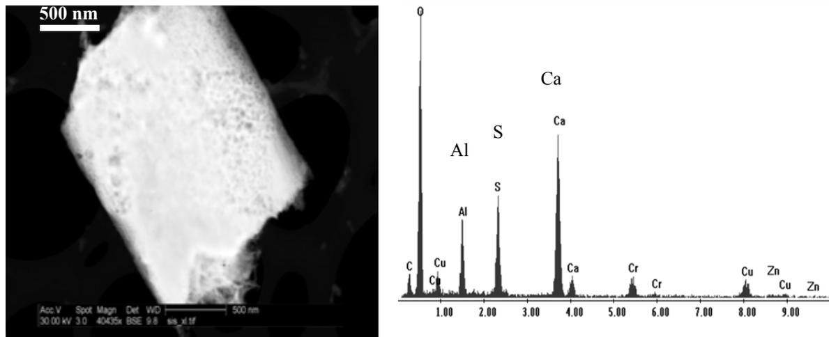
FIG. 12. STEM-in-SEM/EDX microanalysis of ettringite (carbon comes from the sample holder, Cu from the copper grid, and Cr from the detector).
