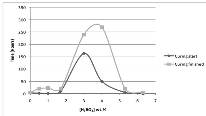
FIG. 2. Impact of borate waste content on time to initial and final set.
