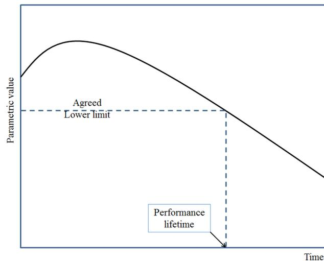
FIG. 18. Representation of durability and the relationship between parameters, time in service and performance lifetime.
