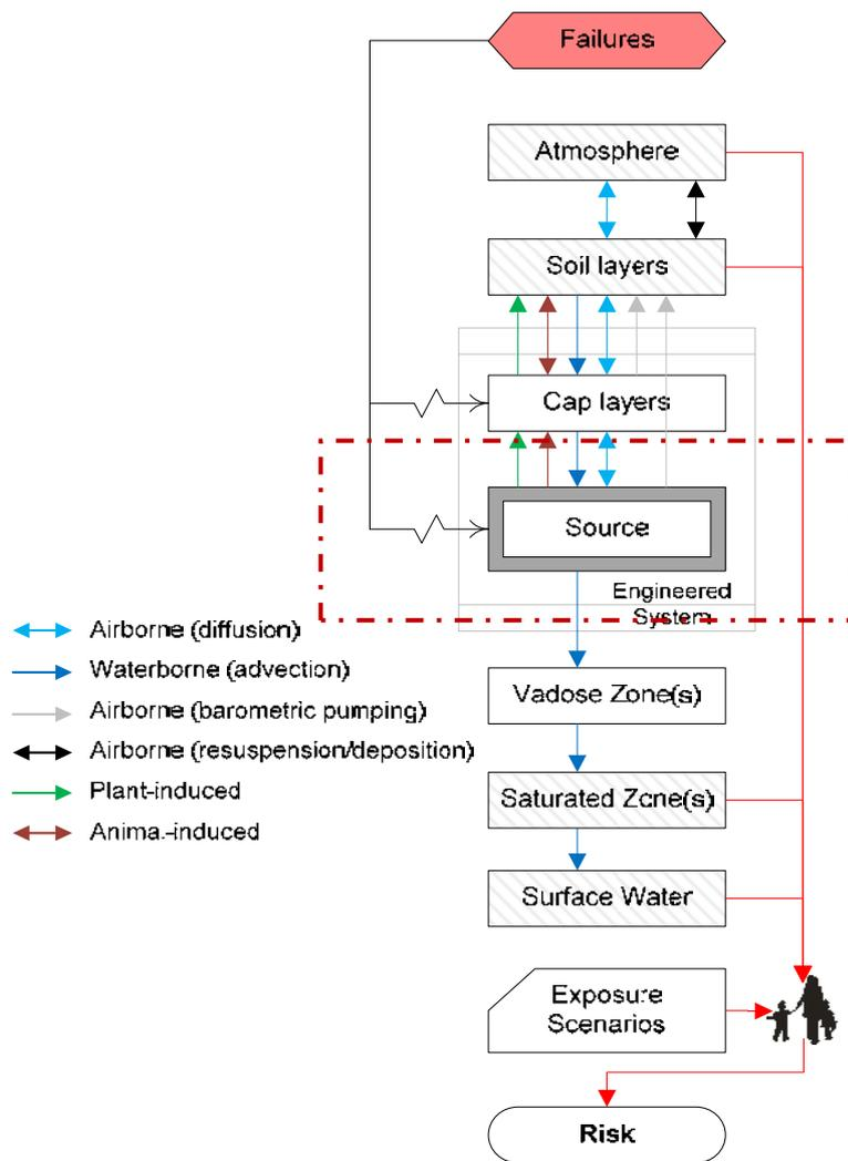
Cementitious wasteforms (PA source terms) and cementitious barriers (containers and containment structures) are part of engineered systems. Durability over time and changing conditions of these cementitious barriers are necessary inputs to disposal facility performance assessments.
