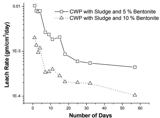
Leach rate of CWP prepared from sludge with various concentrations of Bentonite
