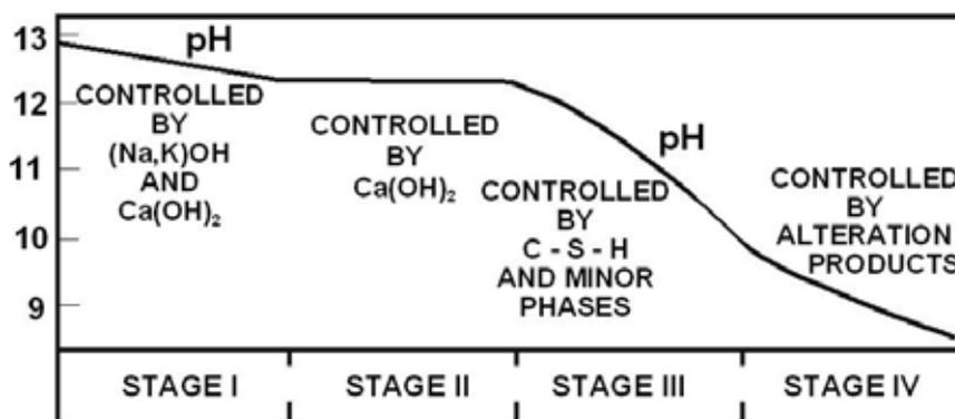
FIG. 15. Evolution of cements in a disposal environment.
