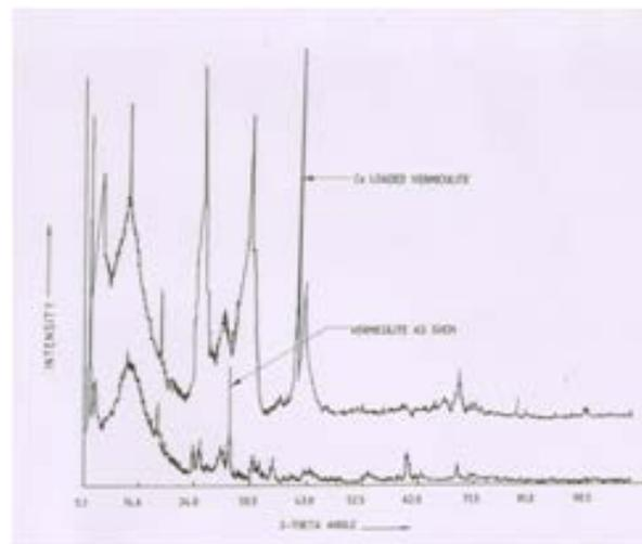
XRD pattern of Cs loaded and as such vermiculite
