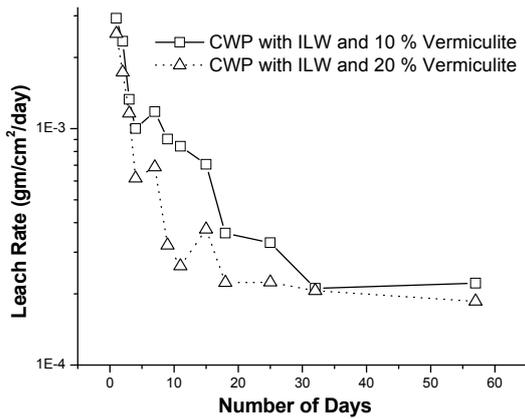
Leach rate of CWP prepared from ILW with various concentrations of Vermiculite
