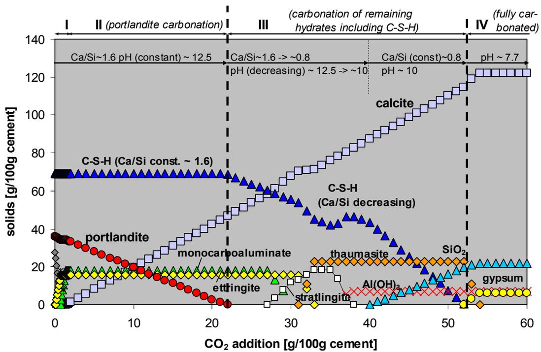
FIG. 17. Effect of carbonation on the mineralogy of hydrated ordinary Portland cement.
