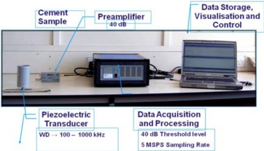
FIG. 10. Acoustic emission technique used in current CRP.
