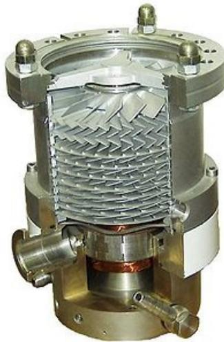
*FIG. 4.1. A cutaway view of a turbomolecular high vacuum pump.*
