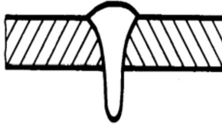
*FIG. 1.48. Excessive penetration.*
