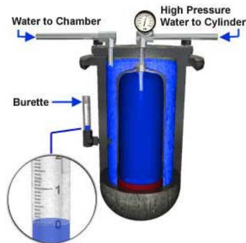
*FIG. 6.1. Water jacket test.*
