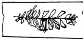
*FIG. 1.43. Piping in weld.*
