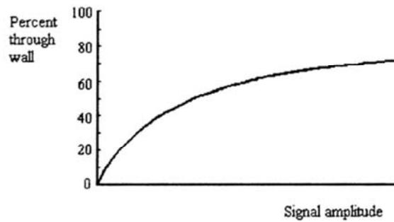
FIG. 5.40. Graph showing the correlation between signal amplitude and flaw depth for narrow circumferential flaws like fretting grooves.
