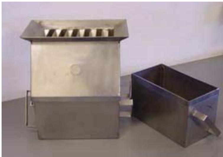
Figure 4.16 A type of sample splitter.
