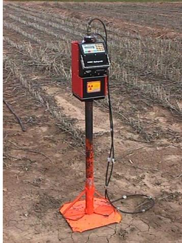
Figure 2.17. A CPN model 503DR neutron probe mounted on a stand, which has been placed over an access tube. The feet of the stand are designed to fit between plants in a row, yet provide enough surface area to not sink into the soil. The protrusion of the access tube above the soil surface prevents the stand from falling over (Evet, 2000).
