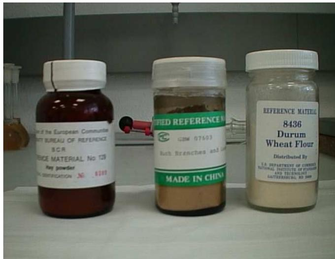
Figure 5.3. Certified reference materials for total N analysis.
