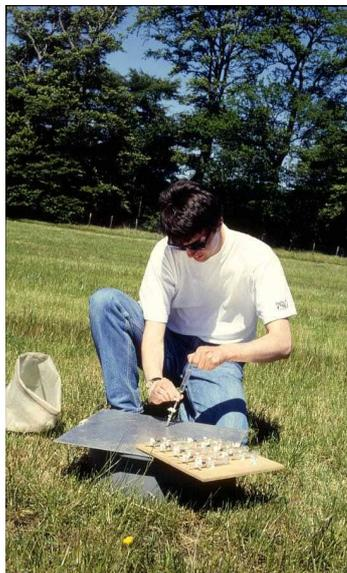
**Sampling head space gas from a chamber for denitrification experiments**
