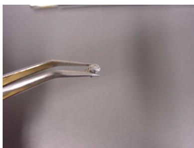
Figure 4.4. Tin cups being formed into a round shape.
