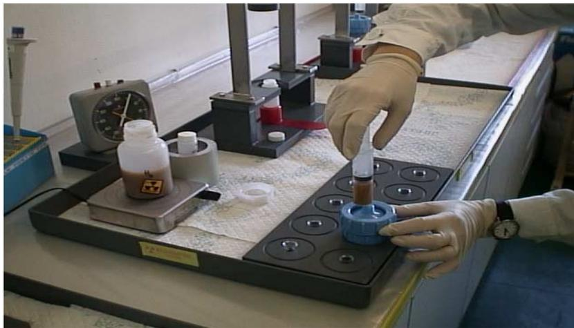
Figure 4.13. Filtration of labelled soil suspension for Cerenkov counting or LSC.
