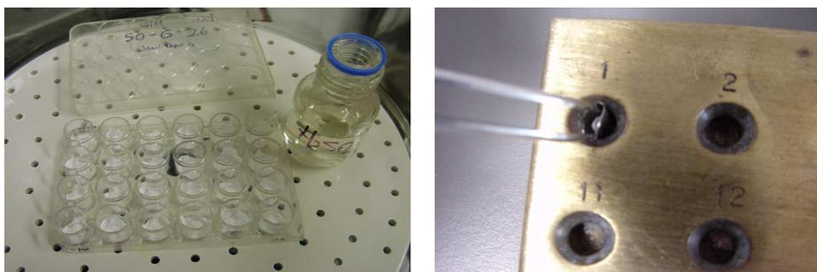
Figure 4.3. Filter papers being dried in the desiccator (left) and being placed in tin cups (right).
