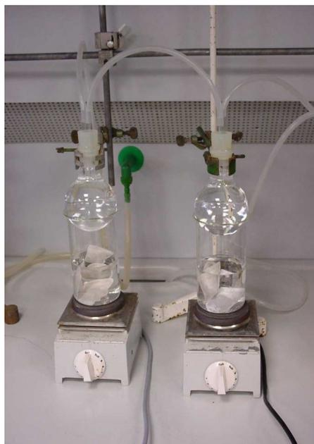
Figure 4.18. Apparatus for ADF determination.
