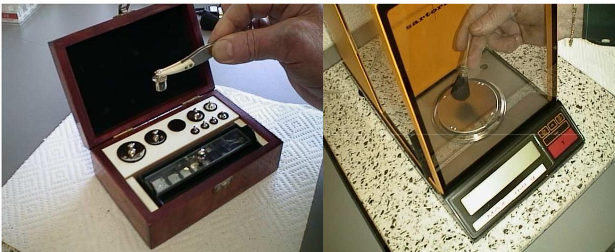
Figure 5.4. Certified reference weights (left) are used to calibrate the balance after careful cleaning (right).
