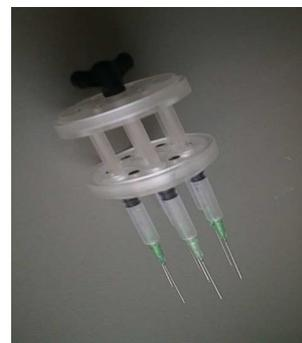
Simple soil solution injector
