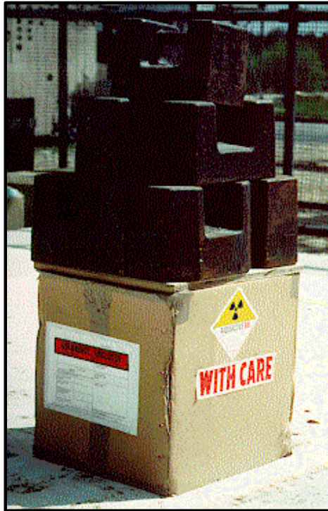
FIG. 8.15. Package stacking test
