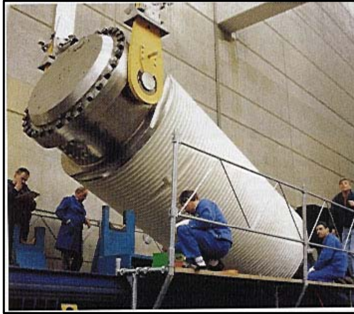
FIG. 8.11. Type B(U) irradiated LWR nuclear fuel package
