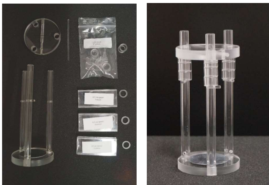
FIG. 1. Assembling of the IAEA electron standard holder for the TLD irradiation. (a) Holder in parts (b) Assembled holder, plate top at 2.8 cm depth
