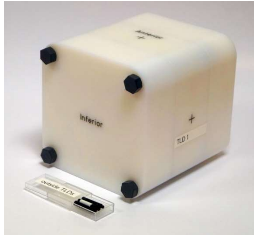
FIG.1. Phantom containing IMRT QA insert loaded with film and TLDs and a pillbox with TLDs to be affixed to the outside of the phantom.
