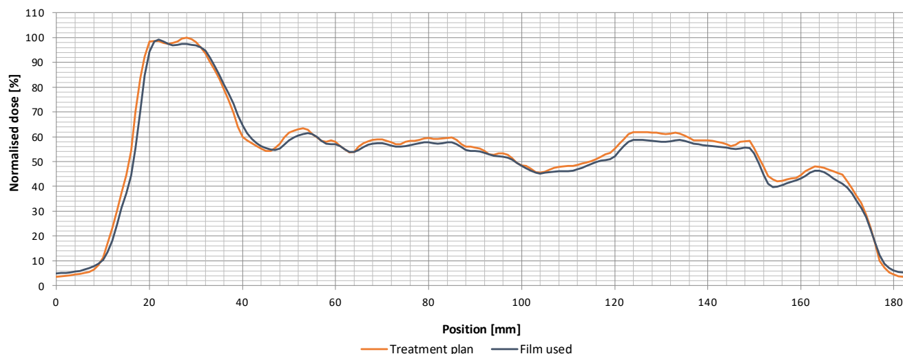
Figure 3. Vertical profile along the axis passing through the point of the reference dose.
