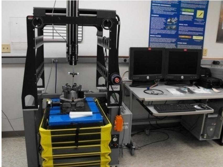
FIG. 3-87. Eddy current measurement instrumentation with scanning stage.
