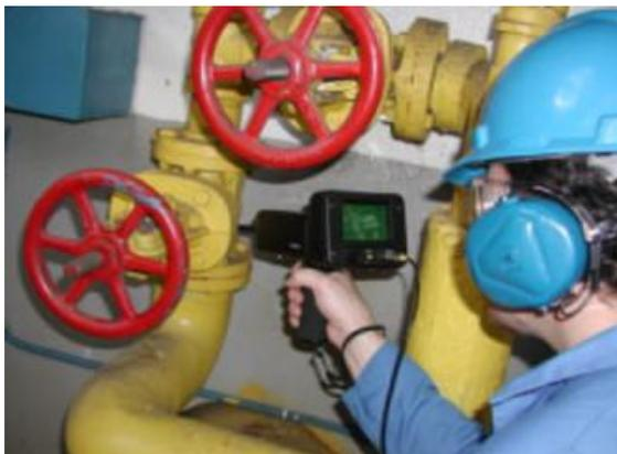
FIG. 2-79. Carrying out of measurements by ultrasonic locator Ultraprobe 10000.
