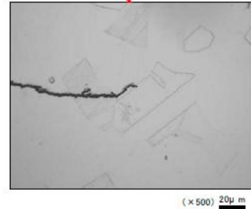
FIG. 3-15. Sectioning face observation by optical microscopy (Type 316NG) (TP No.:F1-S3NG-9, Fatigue usage 0.8).
