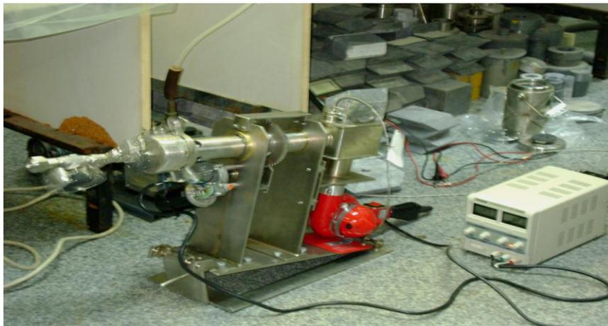
*FIG. 20. Uranium dissolution in the dissolver*
