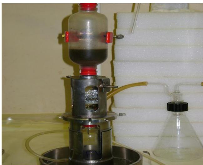
FIG. 23. Mo Precipitate Filtration
