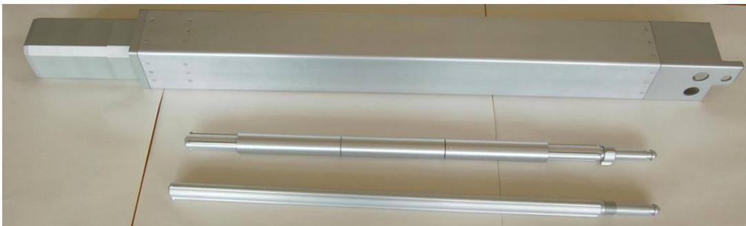
*FIG. 5. Irradiation device and target holder with 3 annular targets*
