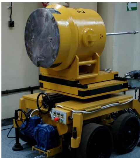
*FIG. 17. Transfer cask mounted on transport vehicle*
